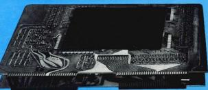
Also standard in 4K x 8 bit words and 2K x 8 or 9 bit words. For special data processing and collection systems, buffer-4K x 9 Card Set ing of 7 bit magnetic tape,
