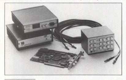
Fox Research's 10-NET fiber-optic boards support 1M bps communication using the Ethernet protocol; the 10-NET fiber hub (right) accommodates up to eight nodes. of fiber-based communications. Especially in personal computer networks, fiber-optic media play a more important role in extending the reach of networks that don't talk to the building next door and in immunizing those networks that suffer errors from EMI radiation. Cost also plays an important role.
