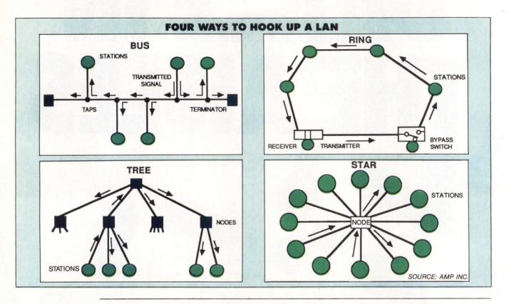
**Topology is destiny** in the choice of LANs. Two common arrangements are bus and ring. In the first, signals speed from the orginating station to all others on a common bus. In the second, a signal travels serially from station to station until it reaches its destination. The hierarchical tree arrangement is typical of the phone system. The central node in the star configuration can either serve the other nodes or simply be a passive transfer point.
