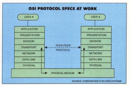
A typical seven-layer OSI connection between two computer systems would involve peer-to-peer communication with the top three layers dedicated to the user interface and the bottom three focused on the actual data link. This connection could be with two similar or dissimilar computer systems.
