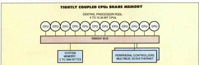
level by coupling a central processor through shared memory to multiple computers, each handling several databases and terminal-originated transactions.
