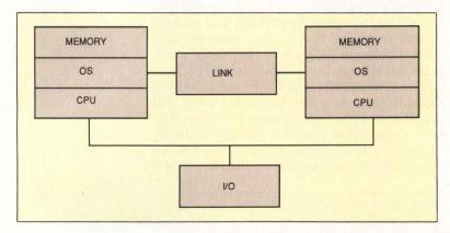
**Loosely coupled architectures** contain selfsufficent processors (above). Diagrammed below is the loosely coupled iPSC from Intel.
