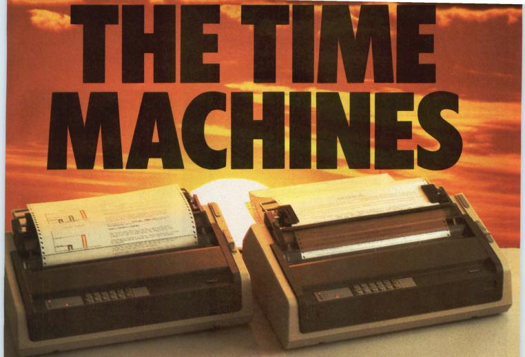
The Facit "C-line" includes the 400 cps, 15-color C7500 and the 250 cps, 7-color C5500
