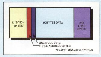
This example of a CDROM physical format uses spiral-track recording with the data arranged in packets consisting of 12 synchronization bytes, three address bytes, a mode byte and 2K bytes of data, followed by 288 bytes of error-detection and correction.
