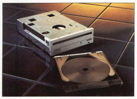
One Laser Magnetic half-height CDROM drive comes with a proprietary interface; the other with SCSI. Both read digital and audio disks.
