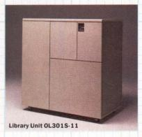
The 301 Series library unit provides as much as 83 gigabytes of on-line storage capacity. It incorporates a formatter/controller, one or two disk units, and an automatic changer for as many as 32 disk cartridges.
