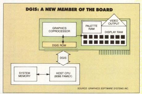
DGIS is a board-level interface that resides in ROM and works with a graphics coprocessor in IBM PCs and compatibles.
