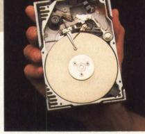
Shockproof 3.5-inch 20-Mbyte Winchesters that eliminate head-disk wear and stiction—completely.
