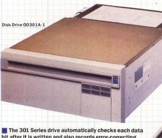
The 301 Series drive automatically checks each data bit after it is written and also records error-correcting bits. The combined use of read-after-write checking and error-correction codes reduces expected read errors to 10<sup>-12</sup>, allowing storage of both image and encoded data.
