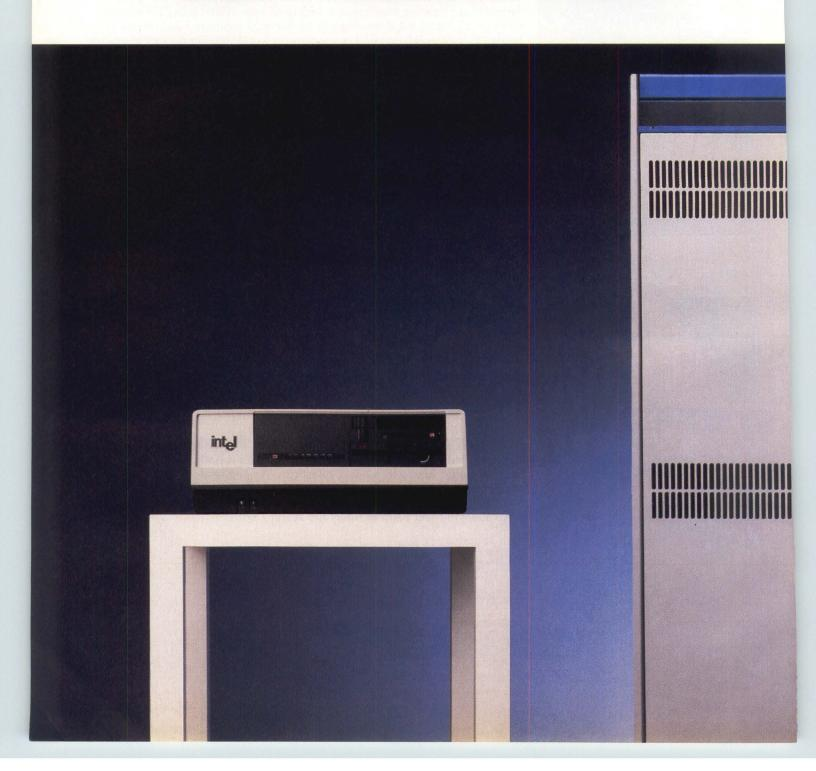
Its CPU performance is only marginally faster than the VAX\*-11/780 shown on the right, for example.
