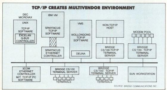
Many third-party vendors offer TCP/IP equipment that allows users to build a true multivendor environment. For example, a user at a terminal, personal computer or workstation has access to all network resources. The host computers also interchange files.
