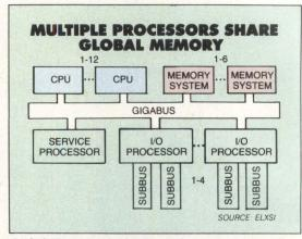
A tightly coupled, shared-memory configuration, such as Elxsi's 6400, is typical of many bus-oriented multiprocessors. Machines from Concurrent, Encore and Sequent use similar hardware architectures.
