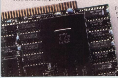
We designed this proprietary gate array chip (on your left) to let us fit a lot more capability in a lot less space. With more reliability, it was also the first chip designed exclusively for 3270 terminal emulation.
