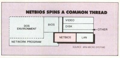
**NETBIOS** acts as an interface between MS-DOS 3.1 and a LAN. It allows the network, computers, peripherals and applications to use standard naming and command conventions.
