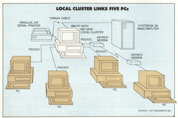
Cluster software and hardware, such as the AST-5250/ Local Cluster from AST Research, allow five IBM PCs to exchange files with a host minicomputer via the cluster product installed in one of the PCs. All 5250 boards allow for multiple LU sessions with the host, permitting a printer to operate concurrently with a workstation session. alter the nature of microcomputer-to-minicomputer and microcomputer-to-mainframe links.
