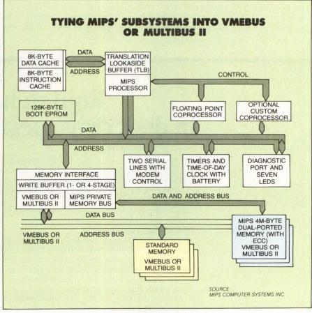
**The R2100 CPU board** from MIPS Computer Systems can operate at 3 million instructions per second using off-the-shelf VMEbus or Multibus II memory boards (yellow). The faster R2300 and R2600 CPU boards, running at 4.81 and 8 MIPS, respectively, require the company's proprietary R2350 4M-byte memory boards (blue).
