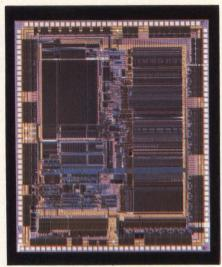
The backbone of MIPS Computer Systems' R2000 family of subsystems is this fully customized CMOS 32-bit processor chip with 4G bytes of virtual address space.
