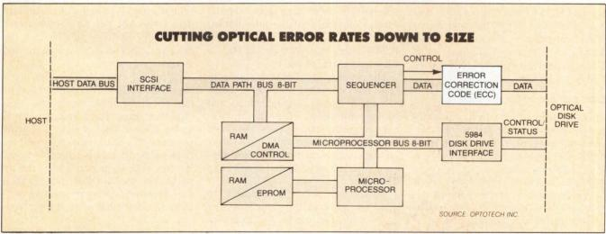
**Optotech's SCSI controller** uses an ECC to reduce raw bit-error rates to one in a billion over the 10-year life of an optical disk drive cartridge.
