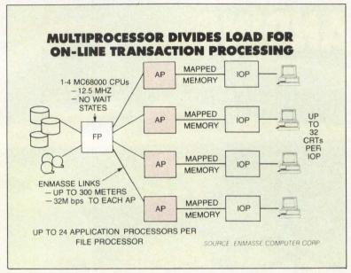
Targeting on-line transaction processing applications, EnMasse's multiprocessor system includes a file processor (FP) with up to four tightly coupled CPUs, which are in turn loosely coupled to as many as 24 application processors (APs).
