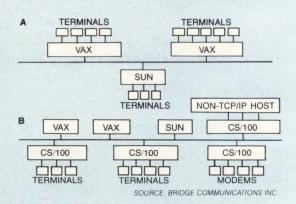
Conventional implementations of TCP/IP require terminal users to connect directly to a host (A), thus using the host's processing power even when accessing a remote host. With communications servers (B), the terminals access any host on the network without going through another host. Resources such as modems and non-TCP/IP hosts can also attach to the network.
