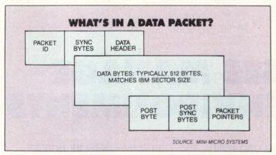
A data packet comprises three distinct subpackets: a header that tells the network what the packet is and what to do with it; the data, which is usually 512 bytes long to match the IBM PC sector size; and the post bytes and pointers.
