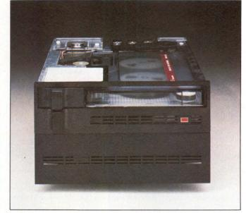
The Super Scorpion from Archive holds 125M bytes on DC600A cassettes and reads data already stored on smaller-capacity DC300XL cartridges.
