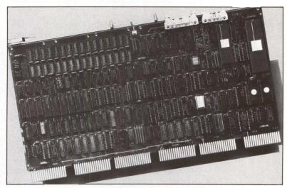
**Bridge's integrated VAX Ethernet** communications server (IVECS) fits into a single VAX Unibus slot.
