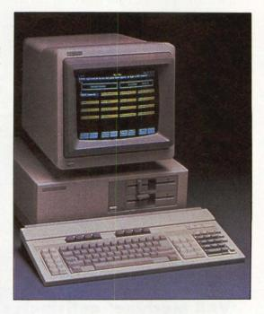
Offering IBM PC software compatibility, Hewlett-Packard's Vectra PC is also compatible with HP's minicomputer line.
