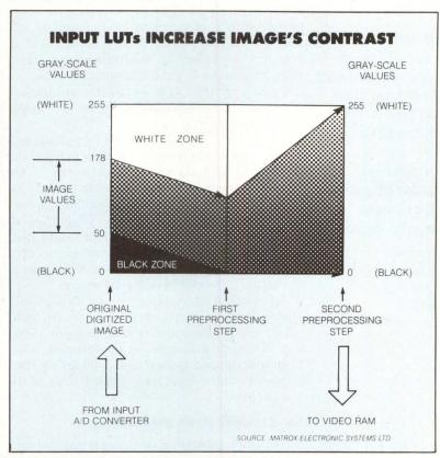
**Eight input RAM LUTs** on Matrox's PIP-512 image-processing board enhance contrast when most of the information is concentrated in a narrow range as, for example, between 50 and 178 input gray-scale values as shown. In the first preprocessing step, the lowest gray-scale value (50) for each pixel of the digitized image is mapped to zero (black). The other values shift correspondingly. The 128 gray-scale values are then mapped over an expanded 255-level range.
