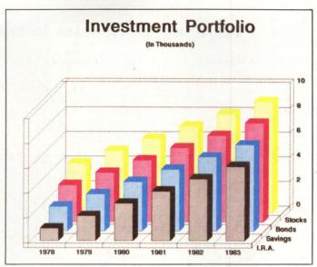
Twenty nozzles in the Xerox 4020 ink-jet printer deliver black, yellow, magenta and cyan inks. When combined, the inks produce seven colors in approximately 4,000 shades. This is an actual sample of the 4020's output.
