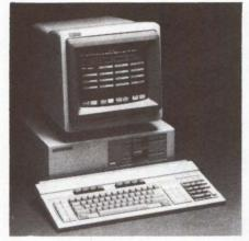
HP's Vectra personal computer is IBM PC/ AT-compatible and offers high-resolution text and graphics on its color and monochrome monitors.
