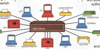
A special supervisory port lets you monitor activity on any other port, connect ports together, broadcast messages or designate the supervisory power to other ports.
