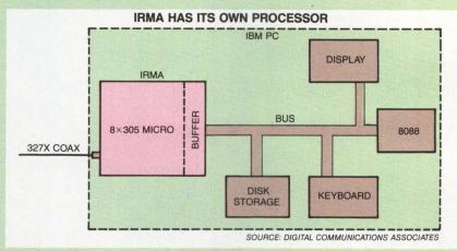
Digital Communications' Irma communications board features an on-board processor independent of the IBM PC's 8088 CPU. IBM's 3270-PC shares its 8088 between local and host communications.
