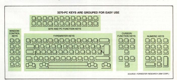
There are five key areas on the 3270-PC's keyboard—two sets of control keys for windows and for the cursor, a set of program function keys for 3270 and PC functions, a typewriter area and a numeric pad.
