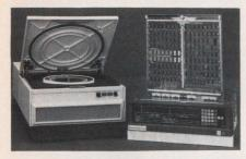
controller comes complete with cables to the first drive, a diagnostic/formatter package, and drivers for any current Interdata operating system. MiniComputer Technology, Mountain View, CA.
