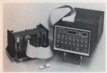
tem under test and the muPro-80-E. The modular package has a hexadecimal control/display console, the 8080 emulator, a power supply, two interchangeable 40-pin headers, interconnecting flat cable and user's manuals. Single unit price is \$3250. muPro, Inc., San Jose, CA.
