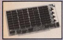
MITS and Imsai backplanes. The board has buffered address, memory protect and 450-nsec access.
