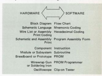
Fig. 1. Hardware and Software Counterparts
