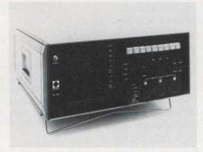
data can be stored in from 1K to 4K of memory. The CRT displays the nine-channel logic recorder levels as well as the ASCII, EBCDIC and hexidecimal codes. *EOTEC*, *Santa Clara*, *CA*.
