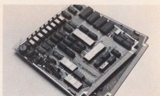
Zilog's microcomputer board set consists of a Z80 based microprocessor board, a disk controller, and a 16K byte random access memory card.
