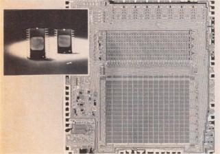
A 52-lead quad-in-line package is necessary on the PPS-8/2 microprocessor system to accommodate the "great functional density."
