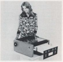
tear bar measures the forms length, ensures smooth forms feed, and eliminates jams. Tion Equipment Co., Oakland, CA.
