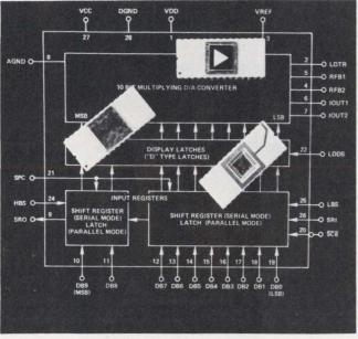
Analog Devices directly-interfaceable buffered D/A converter.
