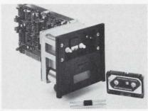
and a data transfer rate of 2400 bits per second. The cassette recorder consumes less than 2 watts of power, operating at 5.0 vdc. Designed specifically for use with microprocessors, the Mini-Raycorder is priced at \$225. Raymond Engineering, Inc., Middletown, CT.
