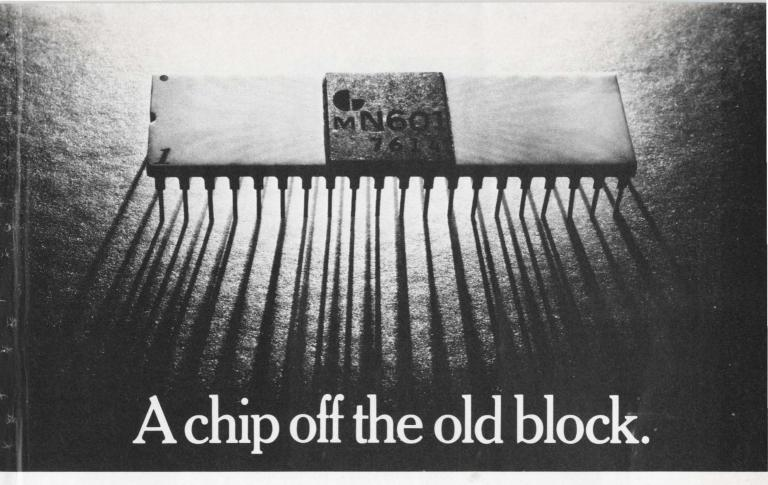
As you can see, this chip is housed in ceramic and mounted in a forty pin, dual in-line package.
