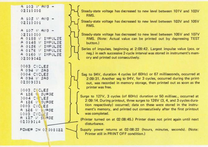
Fig. 4 - A section of a typical record printout with interpretation
