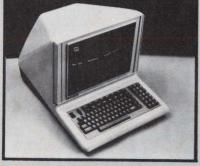
Scrolling and editing features are also included. Refresh memory stores up to 48 lines (two pages). Transmission rates to 2400 baud, asynchronous, are supported. Price in OEM quantities is \$3000.
