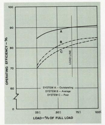
Fig. 1 — Efficiency deterioration curves for three systems from 25 percent to 100 percent of full load. Note rapid deterioration in efficiency of Systems B and C at fractional loads. System C is typical for the better motor-generator frequency converters.
