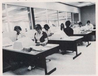
**KEY-TO-DISK IN ACTION.** An example of a shared-processor keyto-disk data entry system is the Entrex System 580 in operation at the VariTyper Division of Addressogrpah Multigraph Corp. With this Entrex System 580, department personnel at VariTyper have immediate access to a 2.5 million character Index Sequential Access Method (ISAM) master file containing information about all parts utilized in VariTyper's manufacturing process.
