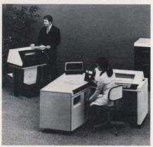
The performance of a B 80 basic system, with a 180 character-per-second console printer, is further increased by the addition of a 250-line per minute printer and two Burroughs dual-drive disk cartridge subsystems.
