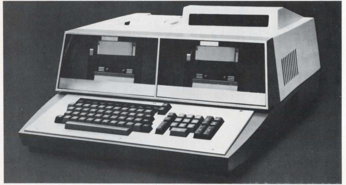
MSI's Source 7600 - A new multi-format data entry terminal from a (previously) fixed-format company.
