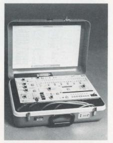
ing the calculation of block check characters. Intershake II offers the unskilled operator pushbutton selection of up to 15 protocol diagnostic routines. The skilled operator can structure these routines manually from a library of 100 programmable test steps including jump and branch instructions and loop instructions for software-like test programming. A CRT option allows simultaneous display of the full-duplex data stream, in clear text or hexadecimal.
