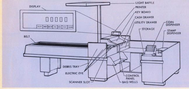
Fig. 1 - Schematic example of a POS checkout stand. (Courtesy of Sperry Univac)
