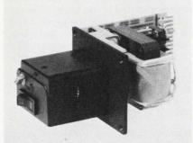
LED light sources and hermetically sealed phototransistors. Power requirements for the LEDs is 12 vdc. Price is \$151. Addmaster Corp., San Gabriel, California.
