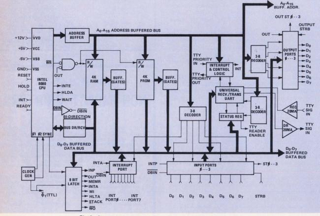
Fig. 2. System logic diagram of Data Numerics' DL8A microcomputer
