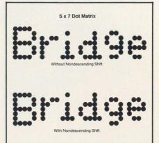
LEAR SIEGLER'S MODIFIED DOT MATRIX. By modifying the 5x7 dot matrix on its ADM-3 "Dumb" terminal, Lear Siegler now offers full lowercase capability. The retrofittable features works by shifting the nondescending characters up one line so the uppercase letters "straddle" the lowercase letters.
