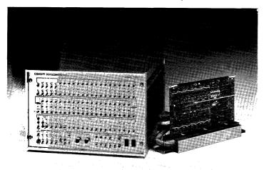
MHZ rate with out data breaks or cycle stealing. It includes six industry standard core and four semiconductor memory programs; all may be individually selected or sequenced automatically. The unit may incorporate up to fifteen mixed core and/or semiconductor programs.
