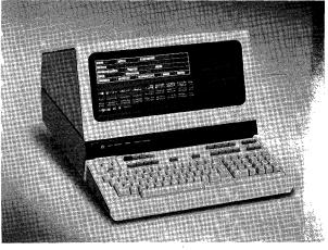
MSI's 3150 automatically generates 16 different character sizes, ranging from .111" to 1.776" high, or .095" to 1.520" high. It uses standard, pin-fed forms and prints an original with up to four copies (either carbon or carbonless). The printer employs a tractor feed, and its width is continuously adjustable to accept forms 4.0" to 14.875" wide.
