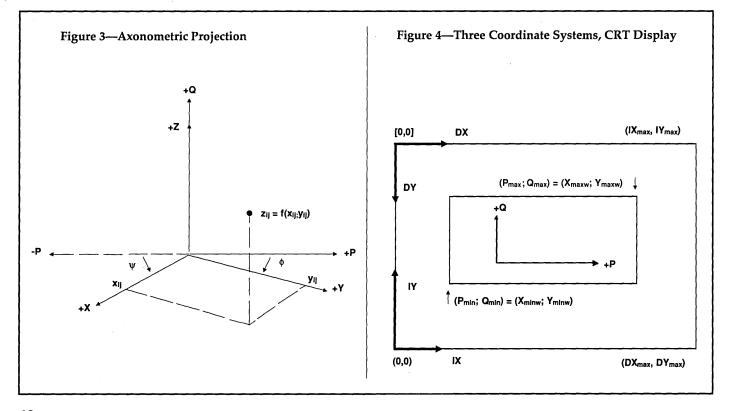
plane and its axial coordinates. The elements in square brackets correspond to matrix subscripts. You could, for example, store all the coordinates that describe the surface in arrays declared:
