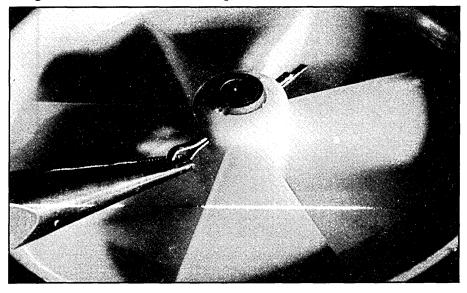
Inserting the Cotter Pin with Needle Nose Pliers
