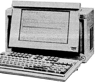
resolution 640x400 super twisted LCD with adjustable intensity and screen-angle. The screen size is 9.5"x6". It's as readable as a CRT. You can also plug in a digital or analog color monitor or a digital or composite
