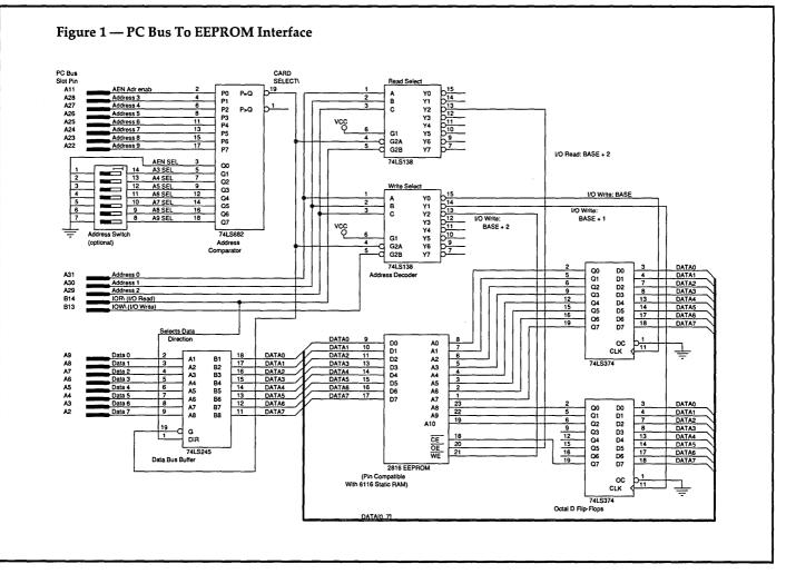
we can't dedicate any of the memory space to EEPROM so I've designed it to use the I/O space. Even then, there isn't enough free I/O space to support 2K bytes (only 10 lines, or 1 K, of I/O is brought out to the PC bus, with much of that dedicated to other purposes).
