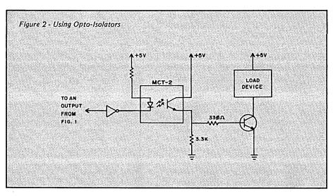
another without having any wires connected between them. Because there is no electrical connection between the two machines, each is safe from electrical malfunctions in the other. With opto-isolators, the only connection between the controller and the controlled is a beam of light. (For more info see Micro C issue #32, page 30.)
