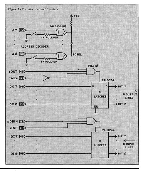
This circuit assumes that only 8-bit I/ O is used in the S-100 machine. (This is the case in most S-100's, although the IEEE-696 specification for the S-100 bus allows 8 or 16-bit I/O addressing.) This simple parallel I/O port also uses no interrupts, no DMA or TMA, and no exotic parts.
