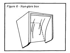
stage of construction (without the bottom, but with a piece of filter material temporarily in place). Finishing touches included spray-painting the inside of the box flat black, and the outside with aluminum paint. I sanded the aluminum paint lightly to remove raised grain, burnished it with the back of the sandpaper, and gave the outside a couple of coats of clear spray lacquer to keep aluminum flakes from getting loose.
