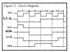
If memory (or an I/O device) isn't ready (or can't be interrupted), then it pulls the READY line low, and the 8088 simply marks time until READY goes high again. For example, if the 6845 video controller is accessing video memory when the 8088 wants to use it (video memory), the 6845 pulls the READY line low.
