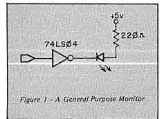
attached to any address or data line in an S-100 machine, and most of the status and control lines. For 25 cents, you can't go wrong.
