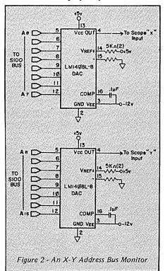
address bus activity. Although it is not as sophisticated as a \$10,000 state analyzer, it isn't as expensive, either. By watching the display when the machine is working properly, you can get a pretty good idea of what part of RAM the machine is operating in, and also see areas that the machine "hangs" in, or where the PC spends most of its time.
