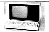
12" GREEN ball brothers TV-12 monitor in enclosure  $19 \times 16.5 \times 14$ ". Room for mounting BB1, BB2 & X820 type SBC's; 8" drive(s) & power supply (see below). Needs +15 Vdc @1.2 Amp, Non composite (separate sync) input. Used & 100%Tested.
