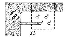
Gently scrape the green solder mask from the ground plane (large copper area) so you'll have a space to solder the capacitor leads. Keep the capacitor leads very short.
