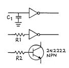
Figure 2 - Controlling Frequency Response
