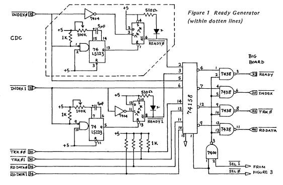
Figure 2 CDC to Shugart Signal Generator and Multiplexor
