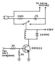
AC Motor Control Circuit
