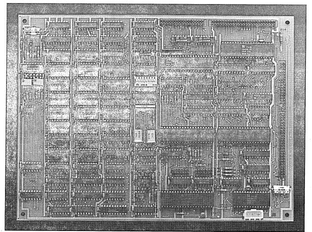
Insight Enterprises' 128-I Single Board Computer offers power, versatility, and speed while occupying no more space than a weekly news magazine. The heart of this board is the Zilog Z80-A 4MHz CPU and 128K of RAM. To further bolster its prowess, the entire Z80-A
