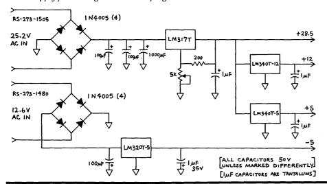
sure and mount LM340T-5 plus five volt regulator and the LM317T adjustable positive voltage regulator on heat sinks, using heat sink grease. The LM340T-12 twelve volt regulator and the LM320T-5 minus five volt regulator do not require heat sinks.
