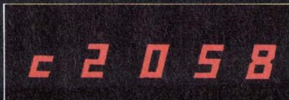
The event is located using the illustrated delay counter, which can be set to count up or down at an adjustable speed as low as one step every two seconds. Specific sections can thus be examined and the counting stopped and stepped back to pick up and locate any irregularities.
