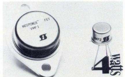
switching time of 4 nanoseconds at a drain current of 1 ampere. Other key specifications include a maximum continuous drain current of 2 amperes (for the 25-w VMP 1 series), and a typical input leakage current of less than 1 nanoampere.
