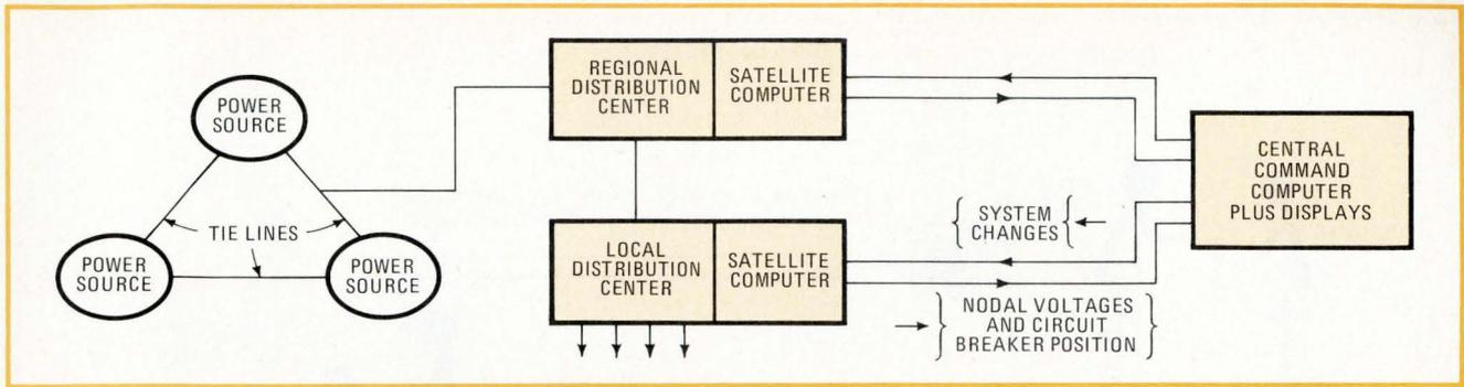
**5. Power generation.** Monitoring, managing, and control of a power grid is best done by a distributed network. A typical system will have a number of regional centers and associated local centers, all with processors tied into the central computer.
