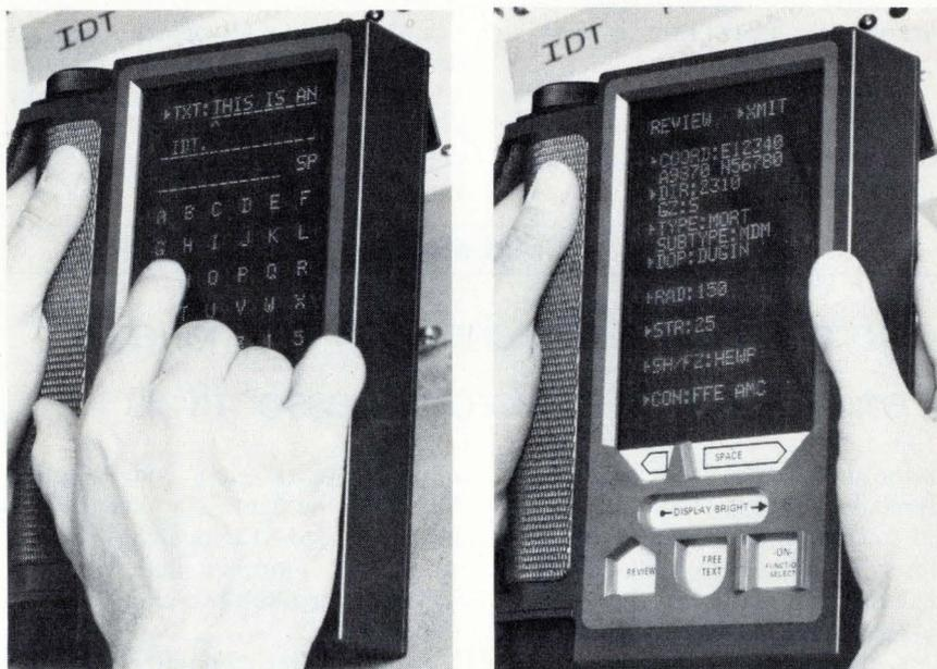
**Clear view.** Message keyed into interactive display terminal via transparent switch over light-emitting diodes (left) is reviewed for accuracy before being transmitted.
