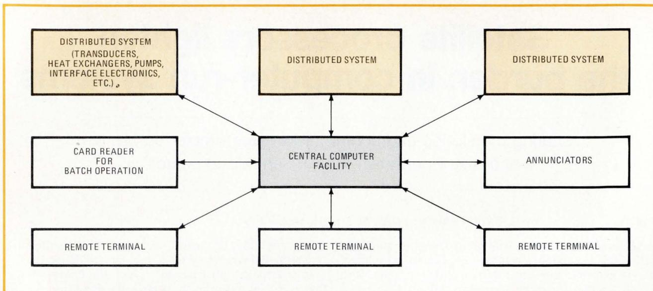
**3. Centralized control.** Multiple distributed systems can be controlled and monitored by one central computer. However, if a system of this type gets too large, real-time control may no longer be possible because of the resultant large time delays.
