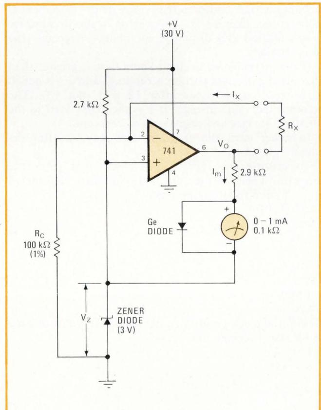
inverting and noninverting input terminals of the op amp must be equal,  $V_o R_c / (R_c + R_x)$  must equal  $V_z$ . Therefore:  $V_o = V_z(R_c + R_x) / R_c$ , or  $I_m = (V_z / R_m)(R_x / R_c)$ . The values of  $V_z$  and  $R_m$  shown yield:
