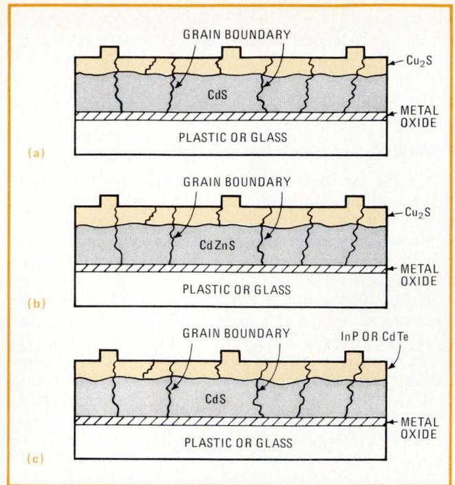
**3. Cadmium sulfide for low cost.** Although they deliver efficiencies of around only 6%, CdS solar cells are cheapest. They can be built on inexpensive substrates, like plastic or glass, with a cuprous-sulfide coating over either CdS (a) or cadmium zinc sulfide (b), or with either indium phosphide or cadmium telluride over CdS (c).
