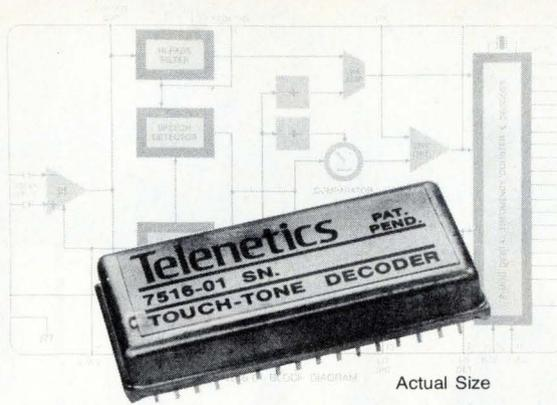
Telenetics' 7516-01 is a complete Touch-Tone Decoder in a  $\frac{1}{2}$  cubic inch, 32 pin DIP. Telephone Standard 2-of-8 tones are received, processed and decoded into discrete 1-of-16 or BCD (plus strobe) outputs. Input signal ranges  $-22$  to  $+4$  dBm with a balanced, capacitively coupled,  $50\text{ K}\Omega$  impedance. Operating voltage range is 8 to 28V dc (single supply); temperature range  $-30$  to  $70^{\circ}\text{C}$ .
