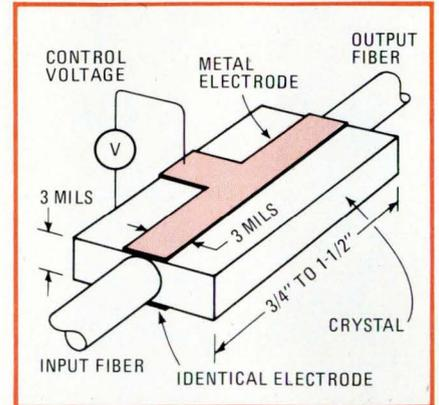
**Mod crystal.** Voltage applied across the surfaces of the electro-optic crystal modulates light in Sperry device. The longer the crystal, the deeper the modulation.
