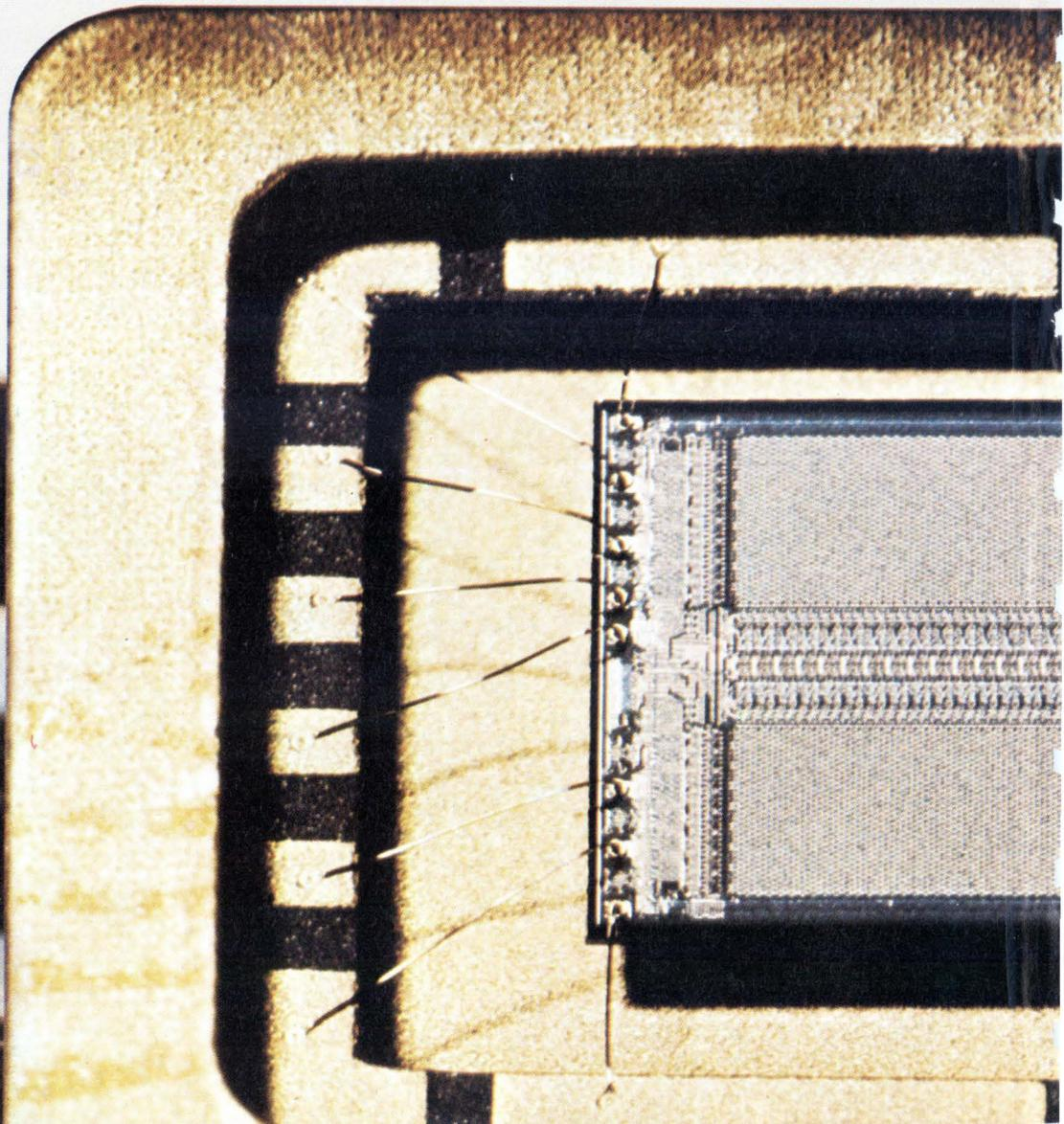
RAM — goes through an arduous series of screens and stresses: Full parametric pre-burn-in testing. Temperature cycling. Centrifuge. Dynamic burn-in at 125°C. And final test at high temperature with wide guardbands. Want proof? Ask our customers.
