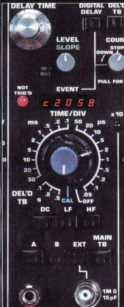
The PM 3261 is another world first. In addition to conventional triggering facilities, the instrument features a digitally delayed timebase that can be set to trigger on a particular pulse in a data stream, the position being displayed on the built-in, five-digit LED. This facility allows individual events to be located quickly and accurately in data streams of up to 100,000 bits and then be 'trapped' for detailed display.
