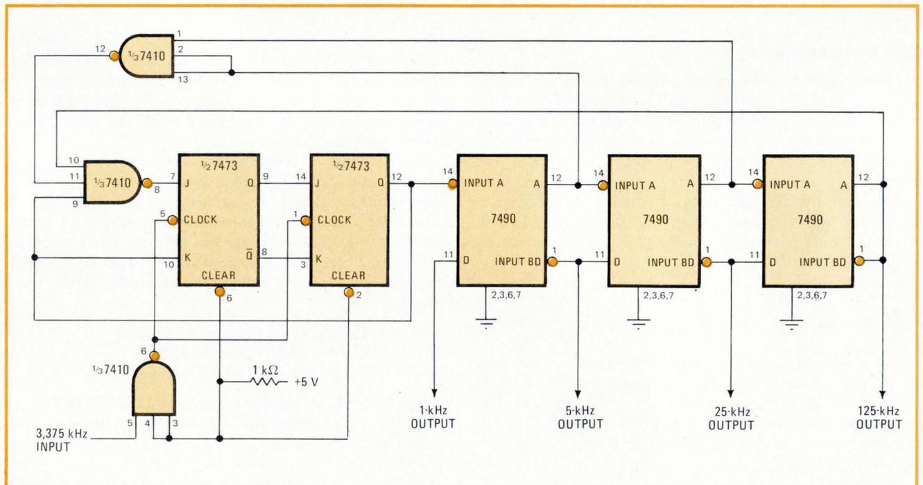
**Frequency divider.** This circuit uses a dual flip-flop and three divide-by-2 stages with feedback to divide the input frequency by 27. Three divide-by-5 stages then give further reductions. The input frequency of 3,375 kHz is convenient for use as a laboratory standard oscillator frequency because it has many useful submultiples and, besides, can be calibrated with great precision simply with a color-TV set.
