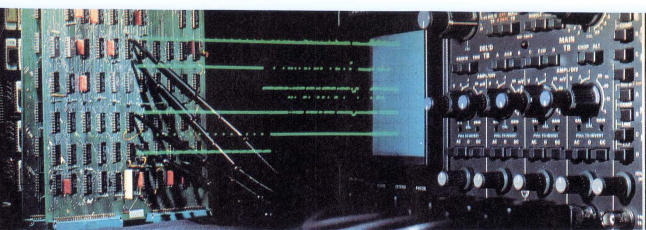
**Four 50 MHz channels. Unique triggering facilities.
