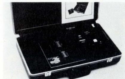
connecting the programmer with a teletypewriter or similar terminal through which it can be commanded to program, list, duplicate, and verify PROMs.
