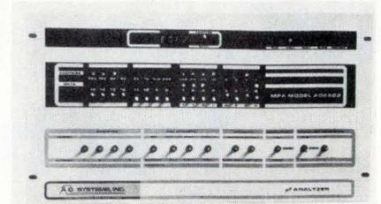
and program counter), examining and depositing data in memory, run/halt control, and single-step control. Readouts are provided to display system status, analyzer status, and the contents of the address bus and the data bus.
