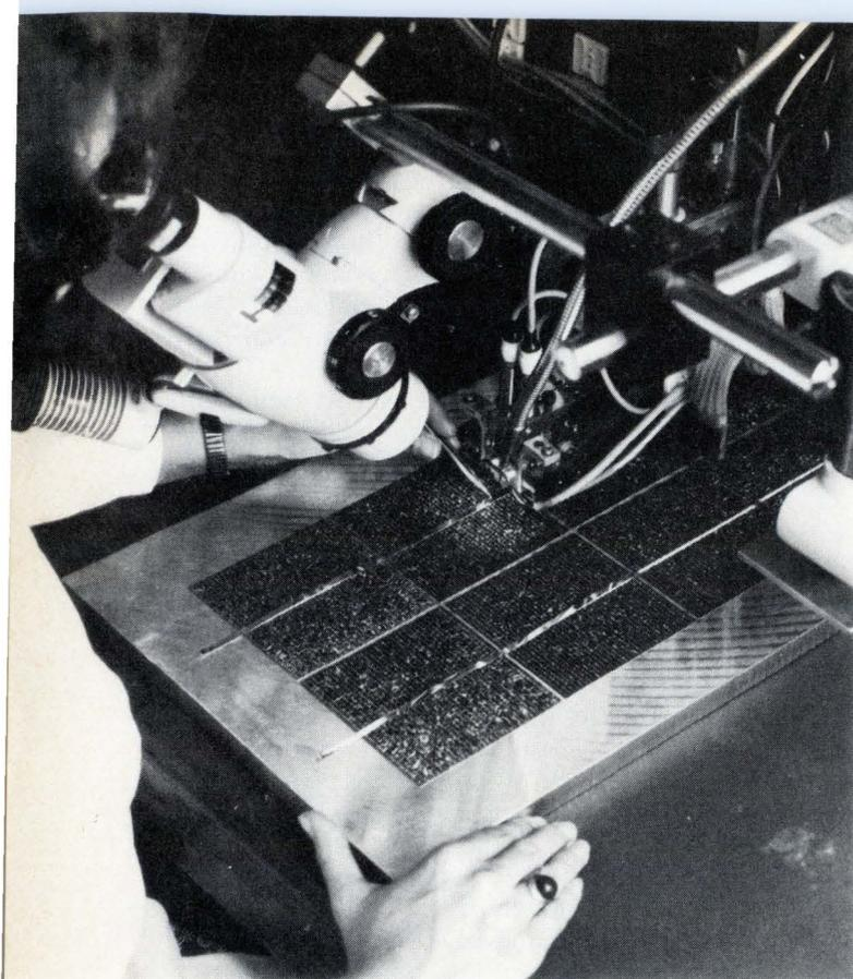
**1. Quantity counts.** A new polycrystalline material from Wacker-Chemitronic has enabled AEG-Telefunken to build experimental 10-by-10 centimeter cells with 10% efficiency. Here eight are being electrically welded into one module of a photovoltaic generator.
