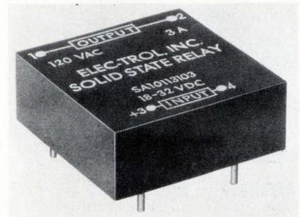
switch up to 3 amperes at 120 or 240 volts ac. Versions are available with input-voltage ranges of 3 to 8, 8 to 18, and 18 to 32 v dc. Capable of being driven directly by TTL levels, the relays offer zero-crossover switching and optical isolation between input and output. The price is \$5 each for 1,000 of the 1.5-ampere 120-volt version, and \$5.79 for the 3-A 120-v unit. Delivery time is six to eight weeks.
