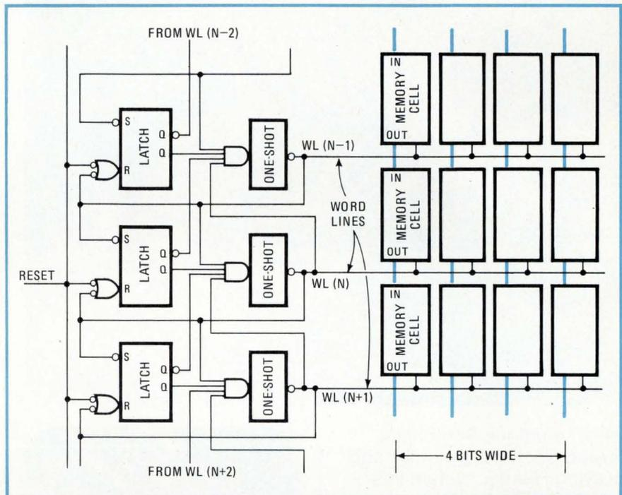
**Shift down.** Control circuitry for the 67401, comprising latch, AND gate, and one-shot, monitors cell contents and allows data to propagate from top to bottom. Data does not shift from word-line  $N-1$  into  $N$  unless the line is empty, having sent its contents to  $N+1$ .
