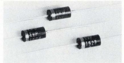
equipment from voltage surges. The devices, which are offered with breakdown voltages from 8.2 through 200 volts, have a clamping time of only 1 picosecond. All devices in the family can withstand temperatures to 400°C, and can be operated from -65°C to 175°C. In quantities of 100, they are priced at \$1.35 each and have a delivery time of six to eight weeks.
