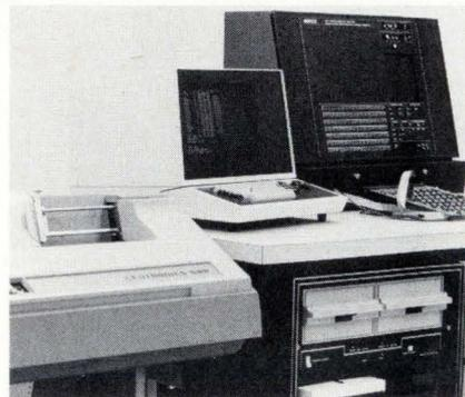
unskilled operators to isolate circuit-board faults. System hardware includes a 16-pin IC clip and a single-tip probe. Connected by cable to the 6500 test head, the clip and probe are positioned by the operator in accordance with instructions displayed on a CRT terminal. Both clip and probe are protected against overvoltages to  $\pm 30$  volts.
