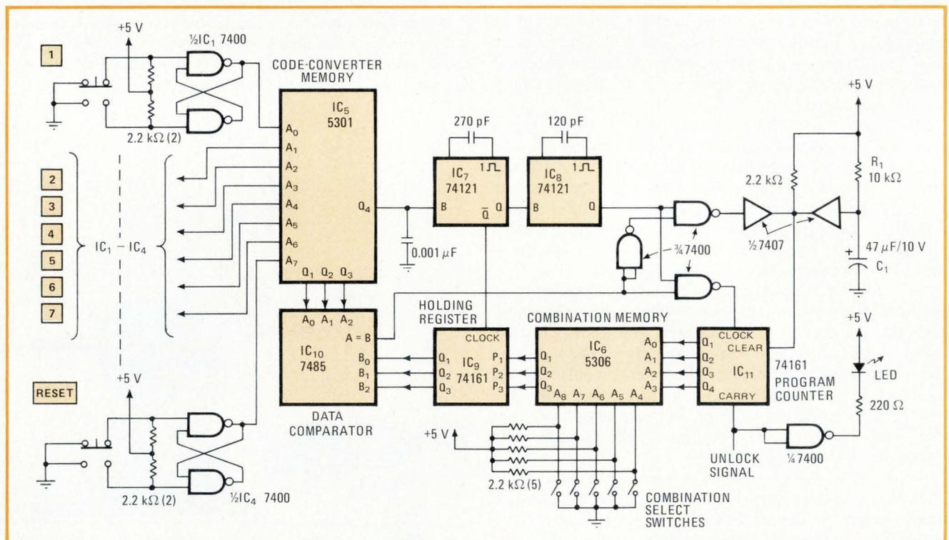
**Maximum security.** A total of 13 integrated circuits is used in this digital combination lock, which requires a sequence of 15 digits to open. The design permits easy changing of sequence length and number of possible digits, and the memory stores up to 32 combinations.
