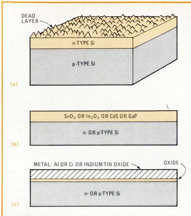
**2. Good efficiency with silicon.** Solar cells based on Si provide reasonable efficiencies—on the order of 15%—at reasonable cost. Several variations look quite promising—among them nonreflecting (a), heterojunction (b), and Schottky-barrier (c) structures.
