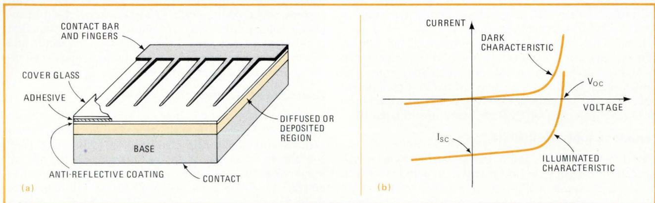
**1. Typical solar cell.** Essentially, a solar cell is a semiconductor photodiode. It is made up of seven structural elements (a), starting with a base contact and topped by a cover glass. Electrically (b), it behaves like a conventional junction diode when not illuminated. But when illuminated, it develops a small electrical signal, even though no external bias voltage or current is applied.
