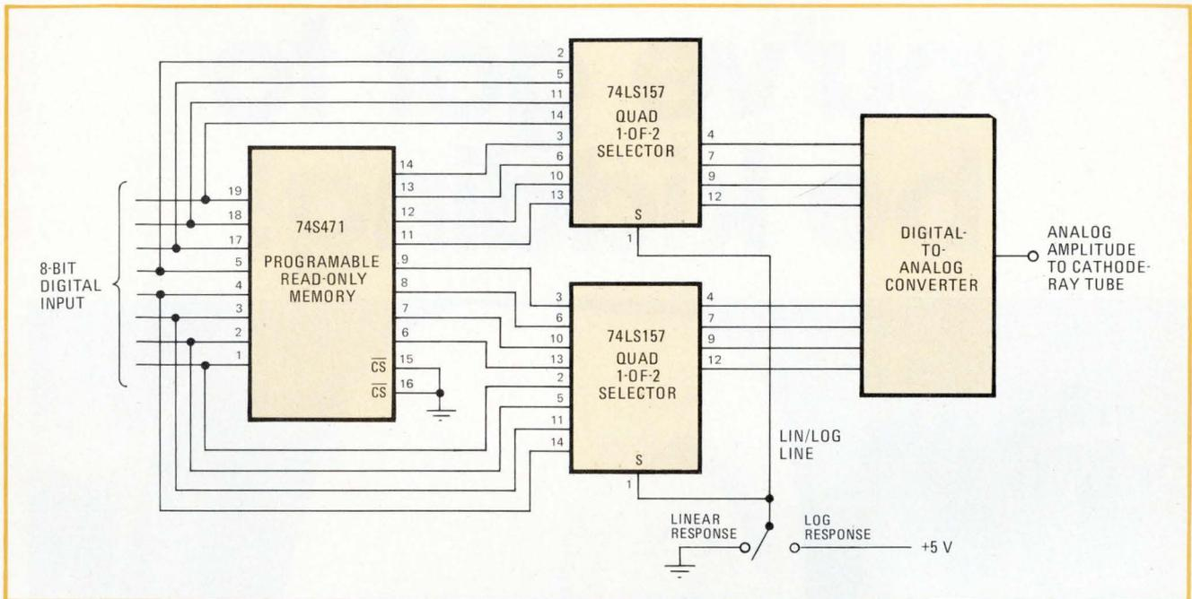
**1. Three ICs select response.** The 74LS157 quad two-line-to-one-line data selectors choose either the linear input code or the logarithmically scaled output from the 74S471 PROM and present it to the d-a converter for display on a scope.
