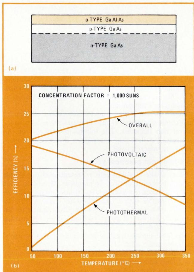
**4. For concentrated sunlight.** The high cost of fabricating gallium-arsenide cells (a) can be offset to a large extent by intensifying the sunlight that shines on them. What's more, concentrating sunlight raises cell operating temperature, so that both solar light energy and solar thermal energy can be converted into electrical power. The result, as shown in (b), is high overall efficiency.
