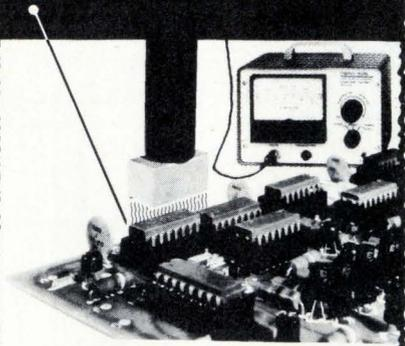
Heat any integrated circuit or electronic component to its rated temperature with a heat probe. Accuracy  $\pm 3^\circ\text{C}$  or better. Or check the component's temperature with a thermo-couple probe. Model 810 Thermo-Probe does both. Reads out directly in  $^\circ\text{C}$  and  $^\circ\text{F}$  on a large  $4\frac{1}{2}$ -inch meter.
