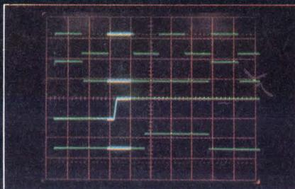
Here the main and delayed timebases are triggered from different channels, one example of the PM 3244's unique triggering facilities. Signals can therefore be shown even when they are not related to the main timebase.
