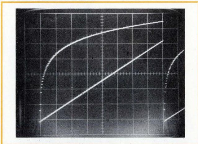
**2. Log response.** The logarithmic PROM output corresponding to a linear digital ramp input is shown in the top trace after conversion. The ramp input is shown in the lower trace. The scope is triggered by the overflow in the 8-bit counter that generates the ramp signal.
