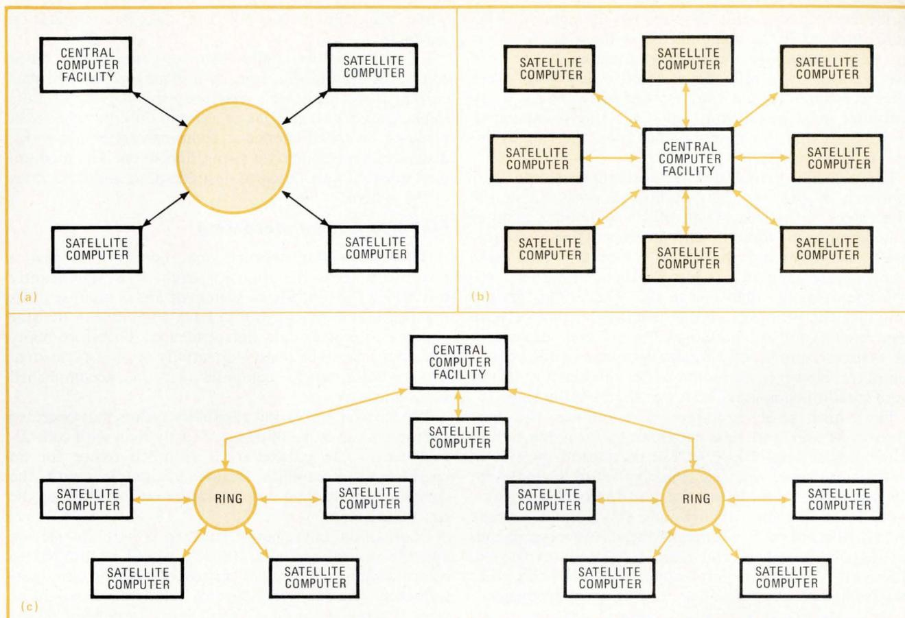
**4. Distributed-control setup.** A distributed-control system can take on three architectures: the ring (a), the star (b), and the hybrid (c). The star is most widely used since it is relatively simple to generate the hardware and software required.
