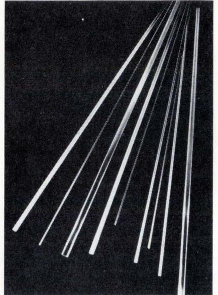
trical insulators, and similar applications that do not require optical transmission. It is offered in a variety of shapes—round, square, rectangular, elliptical, and triangular—in diameters from 0.01 to 0.2 inch. Available lengths vary from one inch to several hundred feet, depending upon diameter.
