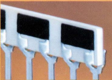
Bourns Krimp-Joint™ offers both a mechanical and electrical bond that lap or butt joint construction can't provide. The lead is crimped on the network element and a high-temp, reflow-resistant solder is used to prevent failure during wave soldering and in circuit thermal cycling and vibration.
