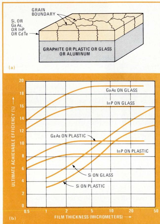
**5. Low cost but not yet practical.** Solar cells (a) made with thin films of polycrystalline semiconductors on inexpensive substrates hold the promise of reasonable efficiencies at low fabrication costs. The curves (b) show the theoretical efficiencies achievable for various combinations of substrates and semiconductor films, as a function of the thickness of the semiconductor film.
