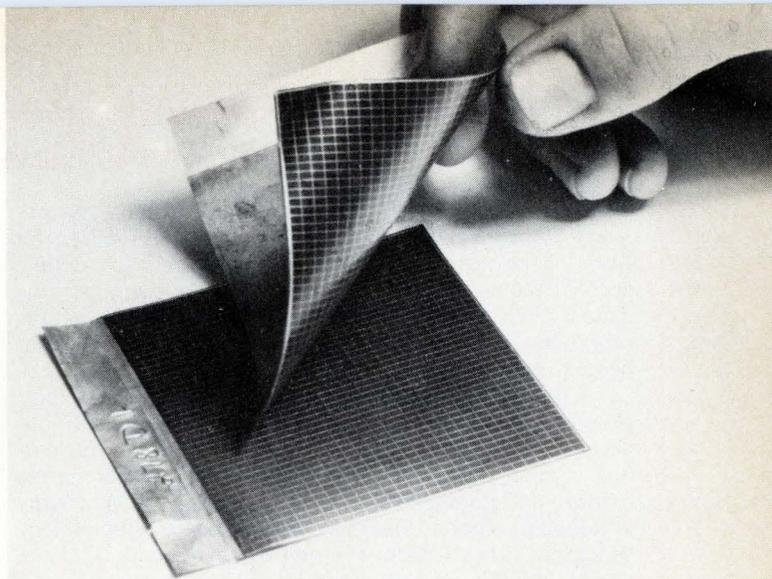
**2. Next generation.** Least expensive of photovoltaic materials, cadmium sulfide has a theoretical 20% conversion efficiency. These thin-film CdS cells, developed at the University of Delaware's Institute of Energy Conversion, have attained 7.8%, the highest yet.
