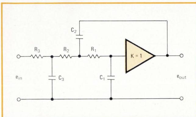
**1. Uses loose-tolerance components.** The performance of this three-pole low-pass active filter is insensitive to values of resistors and capacitors if the amplifier gain,  $K$ , is unity. Therefore inexpensive components with relatively loose tolerances can be used.
