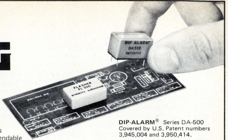
... this unique, miniature solid state sound device has unlimited applications. Plugs into 16 pin DIP sockets or PC boards. Rugged, reliable, loud. Models for 3, 5 and 12 vdc, 35 mA maximum current. Dependable solid state construction means no mechanical contacts, no arcing, no RF noise. 76 dbA at 400 Hz tone radiates in all directions for positive alarm, warning, fault detection.
