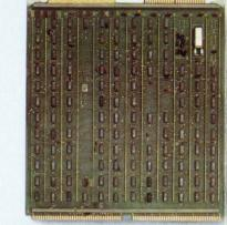
Magnetic Tape Controller. Model four 9-track standard tape units, or equivalent. Cabling separate.
