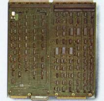
NAKED MINI LSI-2/10 CPU. Model 10600-00. 16-bit minicomputer processor offers twice the speed of LSI-3/05 processors. Includes Power Fail Restart option. See ALPHA LSI-2/10
