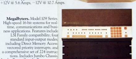
MegaByters. Model 109 Series. High-speed 16-bit systems for realtime, communications and business applications. Features include LSI Family compatibility; four standard input-output modes, including Direct Memory Access vectored priority interrupts; and a comprehensive set of 224 instructions. Includes Jumbo Chassis. Jumbo Power Supply, Programmer's
