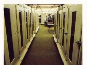
Temperature chambers stress computers to isolate marginal components. Computers are continuously tested during 72-hour burn-in at 50°C. Any error starts the test over from the beginning. To further stress the computer, power is cycled on and off approximately 2000 times during test.
