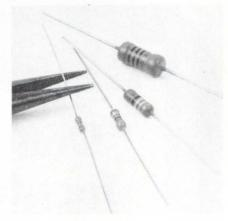
1.5 megohms. Designated type RTL, the Hokuriku Electric Industry Co. (HDK) resistors conform to MIL-R-22684B and are suitable for consumer and industrial electronic products. The resistors are available in four power ratings: 0.25, 0.5, 1, and 2 watts. The highly stable devices are fabricated by a patented process in which a tantalum film is sputtered onto a cylindrical ceramic substrate. Pricing on the resistors is as low as 5 cents apiece for certain 0.25-watt units.
