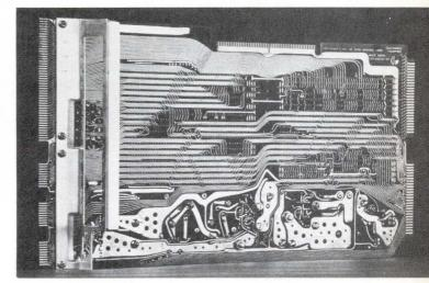
**Engineered efficiency.** When Data General put integrated power-supply circuitry into the backpanel on three Nova computers, backpanel wirewrapping was eliminated as well as much hand wiring.
