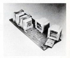
of the relays is 1 ampere at 24 volts dc.
