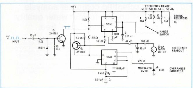
**Unambiguous.** Addition of overrange indicator to analog frequency meter warns when switch is set to wrong frequency range. Transistor Q<sub>2</sub> allows input signal to trigger LED monostable whenever input frequency is greater than meter range. Inexpensive and reliable circuit shown is useful from near dc to well over 20 kHz.
