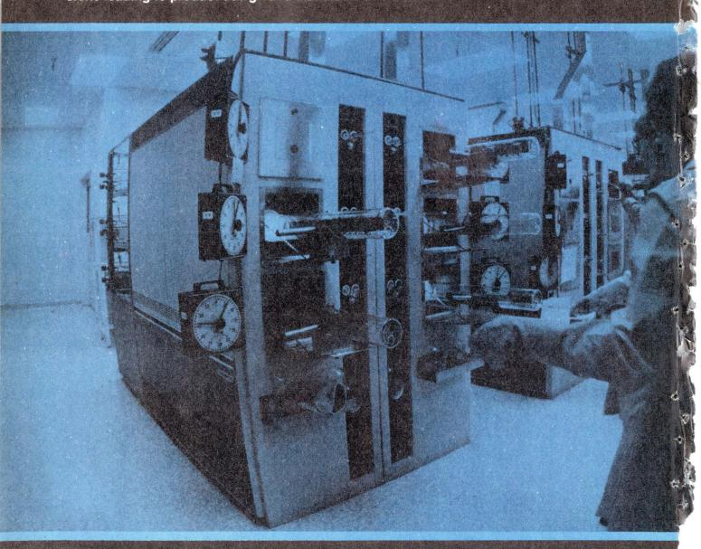
Semiconductor firms use variety of methods to increase yield and hence productivity. Left below, diffusion furnaces for 3-inch silicon wafers at National Semiconductor; right, automatic wire bonding and, below, wire bonds being stressed on centrifugal tester, also at National.
