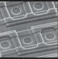
Contacts after etching and resist removal. Note absence of pinholing and sharp edge acuity.
