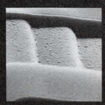
AZ-1350J allows "0" pinholing during etching.
