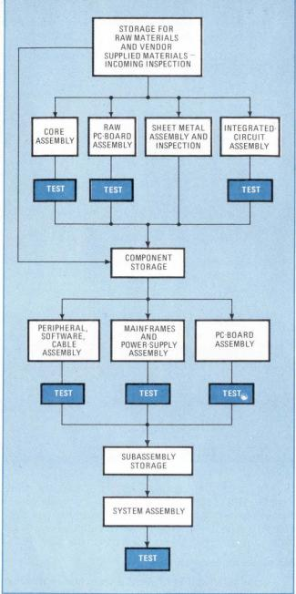
**Sub tests.** Subassemblies for minicomputers built at Data General are tested after nearly every step to assure that final assembly will work properly, cutting diagnostic work on assembled computers.
