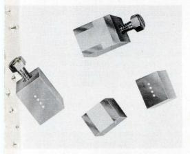
The chips are electromagnetically shielded for minimum coupling in densely packed circuits, and the platinum-gold pads on their undersides make them easy to bond to substrate metalization. Unusual in chip inductors, too, is the third terminal pad, which is connected to the adjustable core for more effective grounding and shielding of the component. The units measure 0.150 by
