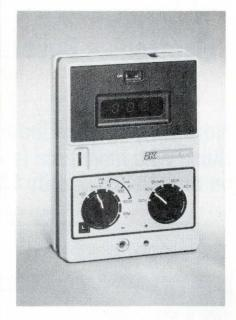
model 280 is within  $\pm 1\%$  of full scale on dc volts and within  $\pm 2\%$  of full scale on ac volts and ohms, except on the 10-megohm range where typical accuracy is specified as within  $\pm 2.5\%$ .
