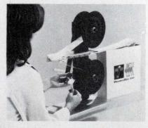
Semi-automatic *Insul-cote* dispensing machines are available for even faster installation. Activated by a ratchet handle, the machine presents the coated insulators one at a time for fast application.
