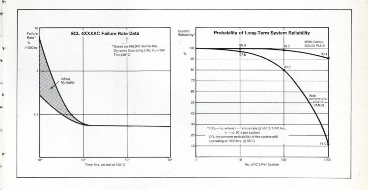
As shown in the Failure Rate curve, mortality of CMOS IC's is greatest in the first 100 hours of service. That's the stage of life where failures cost you most, for reworking during system burn-in, and for field failures within warranty.
