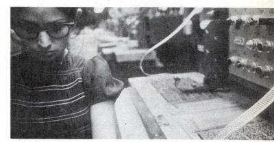
**Terminals.** Zenith Radio Corp. uses 25 Amp Inc. machines, controlled by DEC minicomputers, to insert terminals on pc boards.
