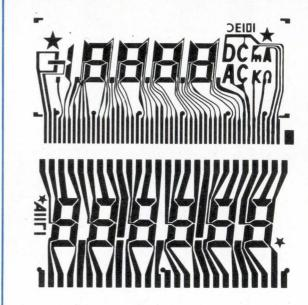
**Thicker and better.** Sometimes a redesign improves productivity by improving reliability. For instance, when Liquid Xtal changed the design of this display to permit conductive patterns to be short and thick, conductors no longer opened and yields went up.
