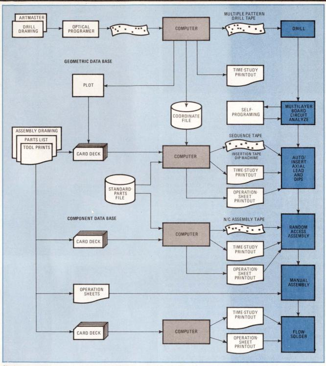
**Single source.** After printed-circuit artwork is digitized, computer at Bendix Corp. takes over to generate series of tapes used in such operations as pc board drilling and testing, and sequencing of components for automatic and semiautomatic insertion.
