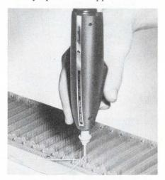
is priced at \$59.69 including wrapping bit, line cord, and recharging unit. The tool weighs only nine ounces, and can handle 26- to 30-gauge wire. Its Ni-Cad batteries have a nominal operating time of eight hours between charges. Recharging time is 14 to 16 hours, the company says. The P160-4 tool and P160-2 bit are available from stock. Vector Electronic Co. Inc., 12460 Gladstone Ave., Sylmar, Calif. 91342 [397]
