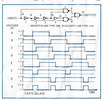
**Frequency doubler.** Propagation delays through inverters cause NAND gates 5 and 6 to go low for 60 nanoseconds following the rising and falling edges, respectively, of input pulse. Therefore output goes high twice as often as input.
