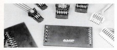
Reliability of the insulation-displacement method of terminating wires to connectors has long been proven in the telecommunications industry. A series of hermaphroditic contact connectors from AMP are supplied pre-loaded with contacts designed for this technique, which eliminates the time, expense, and tooling required for prestripping wires.
