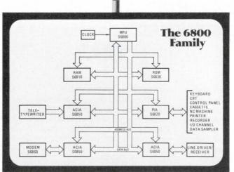
It's less costly because it requires fewer parts. It runs on just one +5V power supply instead of three. It has a more efficient instruction set, which reduces the number of locations needed in memory because of six memory addressing modes. And it needs no TTL to bring it together.
