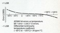
Three temperature ranges to choose from. You can specify the AD562 guaranteed for operation over three temperature ranges. The model K: 0 to +70°C. The model A: -25 to +85°C. And the model S: -55 to +125°C.
