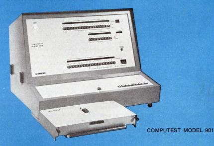
Semiconductor testing demands a practical low-cost solution. To check performance of semiconductor memory from the device through the system level requires memory-oriented addressing capability, a stable clock system, performance compatible device interface and real-time error detection. It's all found in the Computest Model 901 bench top memory tester.
