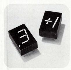
The new 5082-7750 series displays provide a high contrast ratio and wide viewing angle.
