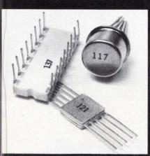
Each i38510 device is marked with its wafer-lot number and delivered with process documentation.
