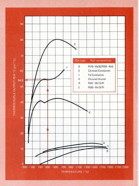
1. Thermocouples. For a type J thermocouple operating at a temperature of 300° C, the readout voltage resolution must be equal to the thermocouple output per °C (approximately 54.5 microvolts per °C from the graph) multiplied by the desired temperature resolution.
