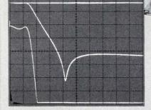
Spectrum analyzer displays of filter response at 10 dB/div and 2 dB/div using built-in tracking generator
