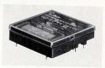
erations at no load to 50,000 operations at full rated load. Initial contact resistance is 50 milliohms or less. The contacts are made of gold-flashed silver and are rated at 0.1 to 3.0 amperes at 30 v dc resistive. Coil voltage ratings are 6, 12, 24, 36, and 48 v dc. The relay will pull in at 75% of the rated coil voltage and has a power requirement of 800 milliwatts. Pricing of the relay can be as low as \$3.06 in large quantities.
