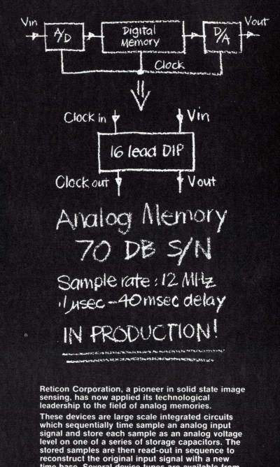
reconstruct the original input signal with a new time base. Several device types are available from inventory with up to 128 elements of storage.
