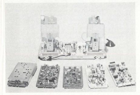
Savings in sight. Matsushita's new G4 chassis has five boards (left to right): video i-f amplifier; chroma circuit and video amplifier; audio amplifier and supply-line regulator; horizontal oscillator and drive circuit, and vertical oscillator and drive circuit. Chassis costs about 20% less to produce than previous types.
