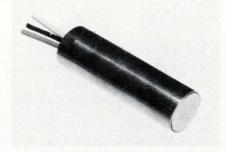
to 100 watts of power. The sensors are sensitive at their front faces only and are offered with both normally open and normally closed output contacts. Packaged in a steel housing 1 in. in diameter and 3.25 in. long, the switch will accept standard 0.5-in. conduit fittings.
