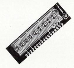
Nine digits, matched for brightness, are mounted on a single pc board.
