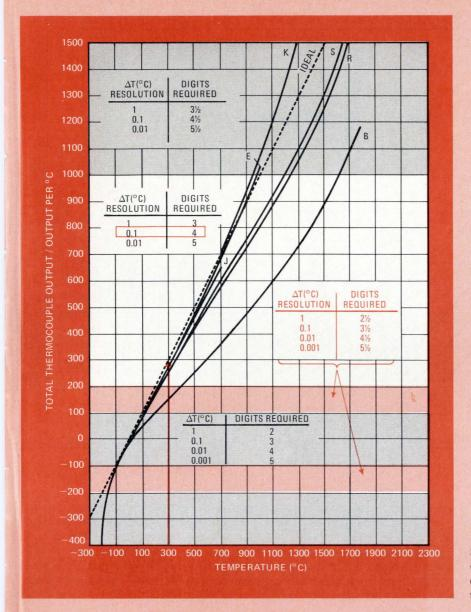
2. Required digits. Type J thermocouple operating at 300 °C requires at least four digits on a readout for a temperature resolution of 0.1° C.
