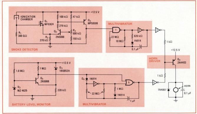
**Detector.** A MOS FET transistor,  $Q_1$ , with high input impedance monitors the voltage level at a divider, one half of which is an ionization chamber. Differential amplifier  $Q_1$ - $Q_2$  picks up any decrease in this voltage and triggers a multivibrator that sounds a pulsating alarm. Low battery voltage triggers a second multivibrator that uses the same horn to sound a "beep... beep. ... beep" warning.
