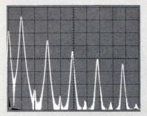
Spectrum analyzer display of square wave harmonics
