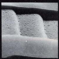
AZ-1350J allows "0" pinholing during etching.
