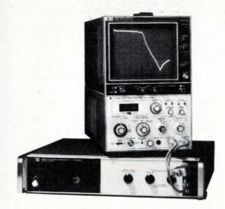
The HP 8558B RF spectrum analyzer now has a companion tracking generator for making swept-frequency response measurements from 500 kHz to 1300 MHz. The HP 8444A option 058 tracking generator's output signal is always the same frequency as the spectrum analyzer, making it possible to achieve more than 90 dB dynamic range in swept transmission and reflection measurements. The generator provides 0 dBm calibrated output with ±0.5 dB full band flatness.
