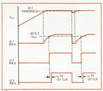
**2. Sequence.** When V $_{\rm cc}$  reaches a threshold defined by the setting of the 5-kilohm potentiometer, IC 1 turns on. Its rise is delayed by the RC network on IC 2. After one time constant, the clear input to IC 3 is released, and the flip-flop is set by the next clock pulse.
