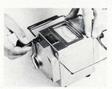
measuring element and a hand-powered generator for current supply. Measurements are made by connecting the terminals of the megohmmeter to those of the lines or wiring under test, and turning the crank. Resistance is read directly on a scale. Different models can apply voltages ranging from 250 to 2,500 volts and can measure resistances from 50 to 10,000 megohms.
