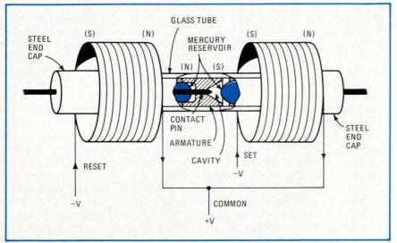
**Self-latching relay.** Switching mechanism of this axial relay is similar to that of the keyboard switch. When the relay latches, the armature moves towards the set coil, causing the mercury reservoir there to fill the tunnel cavity and contact the pin at the end of the cavity. This pin, which runs the length of the armature, is always in contact with the reset-coil side of the relay through the other mercury reservoir.
