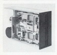
Now that flexible-disk drives are becoming popular in data applications, demand for lower costs is opening a market for dual drives. Dual drives, however, though less expensive than two singles, have disadvantages—notably an interdependence that means complete loss of disk capability if the drive fails.
