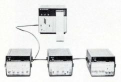
Low-cost data acquisition: three counters (with snap-on interface modules) send time interval, frequency, and voltage information to a thermal printer that also acts as a controller.
