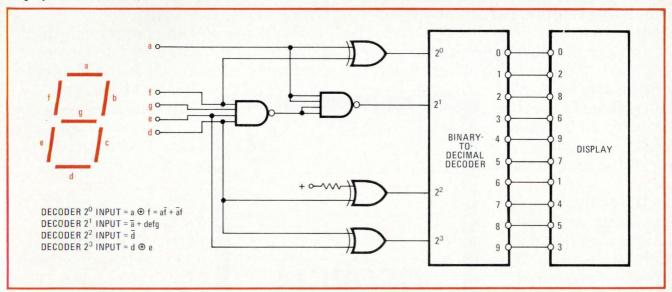
**Converter.** Seven-segment display code is converted into a 1-out-of-10 code for driving such things as indicator tubes, and uses only three integrated circuits. Decoder, external logic, and cross-wired outputs keep the IC count low.
