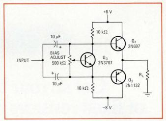
Crossover-distortion regulator. Complementary transistors Q1 and Q2 form a power amplifier stage in which the bias point is controlled closely through transistor Q3 acting as a voltage regulator. The biasadjusting potentiometer permits exact setting of the stage's bias point so that crossover distortion is held to a minimum. The transistor regulator also automatically compensates for varying temperature.
