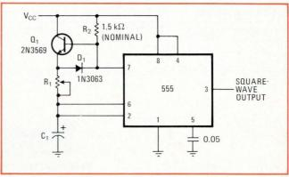
**Workhorse.** This configuration of the 555 timer can drive a heavy load without distorting its square-wave output, even over a very wide frequency range, unlike simpler hookups.
