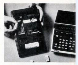
Sharp Electronics' model PC-1002 calculator is a scientific unit with four extra function keys that the user can define by plugging in the appropriate programable read-only memory. With different PROMs, the functions of the special keys are changed, converting the calculator to any application the user needs.
