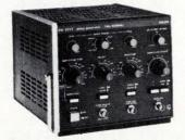
Philips PM5771, a pulse generator with < 2.4 nsec risetime designed for TTL/ECL work
