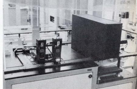
**6. Tests.** After leaving the warp detector, the wafers are visually inspected again. They then pass to stations that check the thickness and resistivity of the epitaxial layer. The units on left are four contact resistivity probes; at right is rapid-scan Michelson interferometer that checks thickness.
