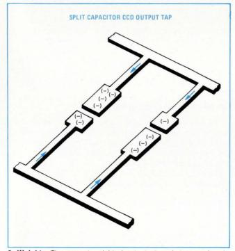
**3. Weighty.** The correct weighted output at each tap can be obtained by simply splitting the electrode at that position so that a fixed quantity of signal is detected. Summing all such taps produces the desired signal transformation.
