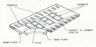
How they work. When the liquid is not electrically excited, its long cigar-shaped molecules are parallel to one another in a position perpendicular to the plates. The liquid appears transparent. When an electric current is applied, ion activity of the molecules leads to turbulence causing the liquid to scatter incident light. Depending on the type of nematic liquid used, either a dynamic scattering or field effect display results.
