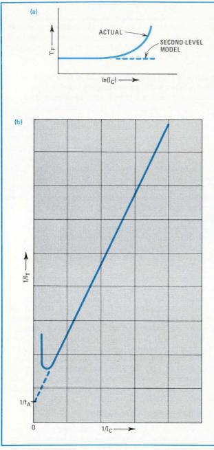
**7. Forward transit time.** For the second-level Ebers-Moll model, the total forward transit time,  $\tau_{\rm F}$ , is assumed to be constant, although it does vary with collector current, as indicated in (a). Generally,  $\tau_{\rm F}$  is computed from the measured value of the unity-gain bandwidth, f<sub>T</sub>. But if there is no quasi-constant f<sub>T</sub> region, an appropriate f<sub>T</sub> value can be found graphically from a plot (b) of  $1/f_{\rm I} \text{ vs } 1/I_{\rm C}$ .
