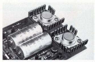
Lower cost per unit was result of replacing four TO-3s used in this 10-watt power supply with two TO-3s in UP3 dissipators. Dissipators allow two TO-3s to operate at 5 watts each with same 65°C case rise above ambient as four devices operated at 2.5 watts each. Low profile dissipators plus TO-3s were assembled in less space allotted to four transistors. New design saved money, improved reliability and eliminated troublesome charring of G-10 board.
