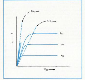
**4. Collector resistance.** The value of resistance  $r_{C'}$  can range from a few ohms to hundreds of ohms. It is measured by displaying the collector characteristics. In the normal active region,  $r_{C'}$  is the inverse slope of the dashed line  $(1/r_{C'max})$  through the knees of the curves. When the transistor is saturated, the value of  $r_{C'}$  increases. Its upper limit is noted here by the other dashed line  $(1/r_{C'min})$ .
