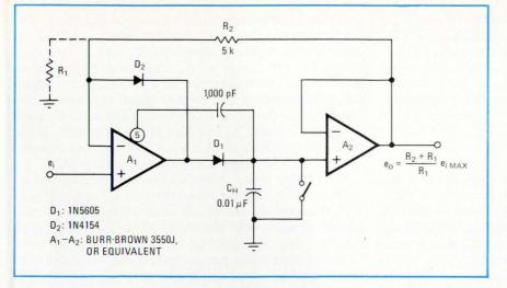
output resistance of this buffer. In the sample mode, feedback adjusts the capacitor voltage to counteract the buffer errors. In the hold mode, however, this error-correcting feedback is disabled because diode  $D_1$  no longer conducts, so any change in buffer offset or loading will create an uncompensated error. Accuracy then becomes dependent on stable FET temperatures and constant loading. The output resistance is  $R_s + 1/g_{fs}$ , where  $g_{fs}$  is the transconductance.
