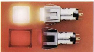
**513 SERIES** With bezel for snap-in panel mounting. Alternate, momentary and snap-action contacts with ratings to 5 amps. N.O., N.C. and two circuit (one N.O., one N.C.). Low level switches also available. Round, square and rectangular bezels in four colors; caps from  $\frac{1}{2}^{\prime\prime\prime}$  to  $\frac{1}{2}^{\prime\prime\prime}$  in more than 12 colors. Illuminated caps with or without legends. **UL listed**.
