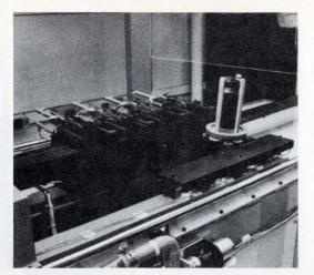
2. Cleaner. At this station, left, wafers are loaded in carriage. Modified LFE plasma cleaner then moves over the carriage to clean the wafers. LFE system is only commercial equipment in the entire Motorola epitaxial setup.
