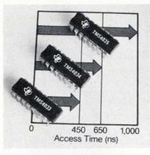
with the popular 2102-1, 2102-2, and 2102 RAMs, respectively, the TMS4033, TMS4034, and TMS4035 have respective access times of 450, 650, and 1,000 nanoseconds. Other features of the devices include full Series 74 TTL-compatibility, single 5-volt supply load, and three-state outputs for bus-driving capability. Delivery is from stock.
