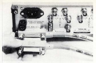
2. Connector. Cables used with the interface system have dual male-female connectors at each end so that they can be stacked, thus allowing more than one cable to be attached to any instrument. This permits either star or daisy-chain configurations.
