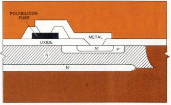
dissimilar metals, as you do in nichrome-aluminum interfaces, in our bipolar PROMs. The fuses are semiconductor material. And polysilicon is classically simple compared to blown junctions. Blown junctions miss the
