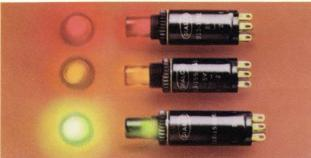
**913 SERIES** Miniature size, mount in 3%" hole. Red, green or yellow LED operates from 5VDC; Neon operates from 125 VAC. Momentary action. Choice of S.P.S.T. double break, N.O., N.C. or two circuits (one N.O., one N.C.). Life: 1,000,000 operations.
