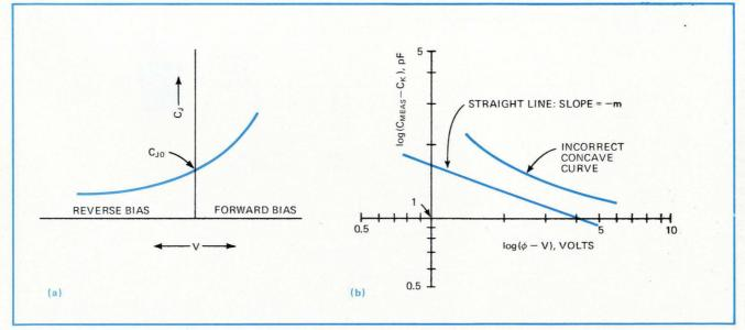
5. Junction capacitances. Both the emitter-base and collector-base junction capacitances ( $C_J$ ) are a function of their respective junction voltage (V), as shown in (a). These two capacitances can be measured with a bridge, but the extra capacitance ( $C_K$ ), mainly caused by pin, stray, and pad capacitances, must be accounted for. A graphical method for reducing the measured capacitance ( $C_{MEAS}$ ) is given in (b).
