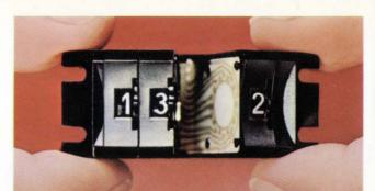
545 SERIES Low priced thumbwheel switches available in standard and miniature sizes with BCD or decimal format. Positive detents for easy action. Miniature switch snaps together, no tools or hardware needed, on  $\frac{3}{4}$ " centers. Gold bifucated contacts assure high reliability. Rugged design allows operation from  $-25^{\circ}$ C to  $+85^{\circ}$ C. Modern low profile—recessed on panel face to eliminate accidental activation.
