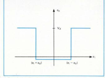
**2. Transfer function.** Output clamp keeps low level only a fraction of a volt below ground. The complementary function is obtainable by inverting the two input diodes and the reference voltage.
