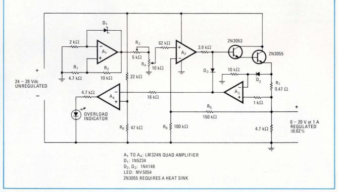
**Op amp regulator.** An unregulated 26-volt source becomes a 1-ampere 0-to-20-V supply regulated to within  $\pm 0.02\%$  by a simple quad operational amplifier. Input can vary between 24 V and 28 V, and quiescent current is less than 10 mA. A light-emitting diode gives an overload indication, the level of which depends on the value of resistor R<sub>8</sub>. Single power Darlington can replace the two transistors.
