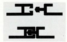
The tubing is supplied in flat, open form and can be wrapped around existing installations without re-wiring—an especially convenient feature when splices are required. Alpha Wire Corp., 711 Lidgerwood Ave., Elizabeth, N.J. 07207 [393]
