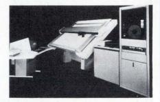
tem software allows the design engineer to make a preliminary drawing on a cathode-ray-tube display, look at the part from any angle, crosshatch, zoom, rotate, window, insert fillets, add standard parts from a library, and define jigs and motions for numerically controlled tools. Data can also be formatted for design analysis and simulation. The Computervision Corp., 201 Burlington
