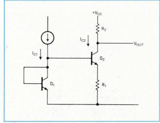
**1. Measuring temperature.** So long as  $Q_1$  and  $Q_2$  are a matched pair and  $I_{C1}$  and  $I_{C2}$  are not equal, the difference in the base-emitter drops across R1 is proportional to the absolute temperature.
