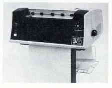
valuable in systems that combine CRT terminals and printers on one line. Since the interface contains a 1,024-character buffer, a Printec-100 can be printing a message while other terminals are being serviced by the computer. Price of the interface, complete with a Printec-100, is \$4,650.
