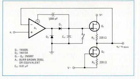
**2. An improvement.** Two FETs provide temperature compensated buffering at the output of the peak detector. Output current no longer drains the holding capacitor  $C_H$ . Offset shift in the buffer FET  $Q_1$  is compensated by biasing it with a matching FET  $Q_2$  and by enclosing  $Q_1$  in the feedback loop.
