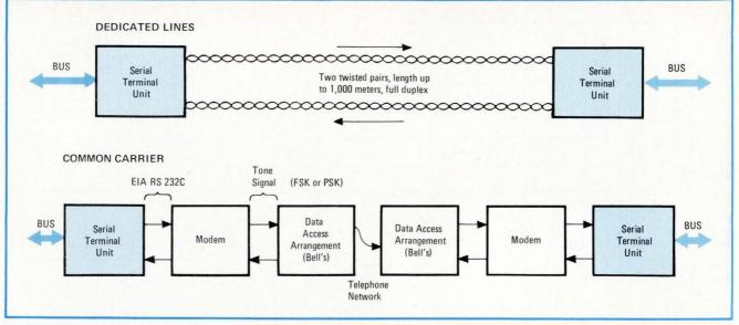
**8. Extension.** Serial terminal units may be used to extend the length of the data bus, either through dedicated lines or by common carrier. The units lower the cost of transmission by taking parallel data from the bus and converting it to serial form.
