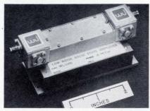
5300 series include: frequency of 7.25 or 8.4 gigahertz or 8 to 10 GHz, noise figure of 6.0 dB or 7.5 dB, small-signal gain of 30 dB or 27 dB, output power of +5 dBm or +6 dBm, and gain flatness of  $\pm 0.5$  dB or  $\pm 1$ dB.
