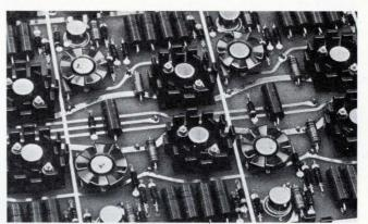
Temperature matching at varying power levels is easy with the wide variety of IERC dissipators. On this board problem was to keep TO-5s at approximately equal case temperatures although some were operated at 2.2 watts and others at 1 watt. Press-on Fan Tops costing pennies kept 1 watters at 55°C case rise above ambient while LP dissipators held 2.2-watt devices at nearly identical case temperatures. IERC Insulube® coating permits mounting LPs directly on printed circuit lines.
