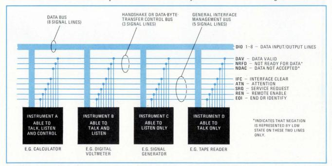
**1. Data bus.** The Hewlett-Packard bus uses a 16-line cable to quickly link up any instruments equipped with appropriate interface circuitry into a system. Data transfer is byte-serial, bit-parallel at rates as high as 1 megabit per second.
