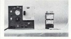
matograph. A worker wears only the first two items—the collector column on his collar, and the sample pump on his belt. After a period of time, the collector column is detached and placed in the flasher assembly, which is connected to the chromatograph. The flasher assembly heats the column and causes the collected sample to be passed through the chromatograph where it is analyzed in a matter of minutes.
