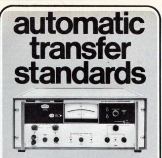
The 1600A Auto-Balance AC/DC Transfer Standard. Precise repeatable measurements every 30 seconds. Traceable to NBS. Takes tedium and guesswork out of 100 ppm transfer measurements in Lab, QA and production.
