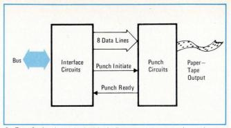
**6. Punch.** As shown by its block diagram, a tape punch can be partitioned into the punch circuits that will enable it to perform its functions as an instrument and the interface circuits that are necessary to connect it to the data bus.
