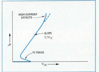
**1. Emitter resistance.** Constant value of emitter resistance  $(r_{E'})$  is obtained from a display of base current  $(l_B)$  as a function of collector-emitter voltage  $(V_{CE})$ . The  $r_{E'}$  value, typically around 1 ohm, is the inverse slope of this display at low currents.
