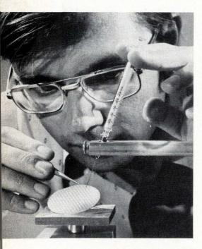
Conventional test equipment can determine whether an IC is functioning properly, but these tests may be of little value in determining exactly why and where an IC has failed. To solve this problem, scientists at the RCA Physical Electronics Research Laboratory in Princeton, N.J., say they have developed a nondestructive technique that enables both the electric fields and temperature distributions at the surface of an operating IC to be viewed through conventional optical microscopes.
