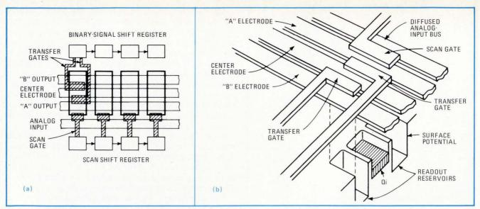
5. Making a transfer. In a charge-transfer device, readout of each charge sample is independently controlled by the voltage on the transfer gate of the cell. Readout is achieved when the gate voltage is sufficiently above a fixed threshold and when a signal proportional to the magnitude of the charge is induced by means of ac coupling in either "A" or "B" output circuit.
