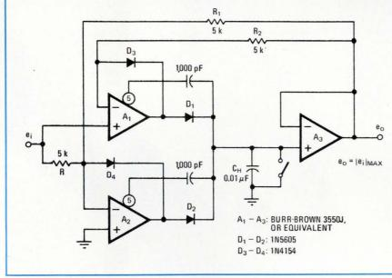
**5. Peak-to-peak.** A simplified peak-to-peak detector is formed by combining two simple peak detectors. A positive peak detector is formed by  $A_2$  and  $A_3$ , and a negative peak detector by  $A_1$  and  $A_3$ . Op amp  $A_3$  sums the peaks, positive and negative.
