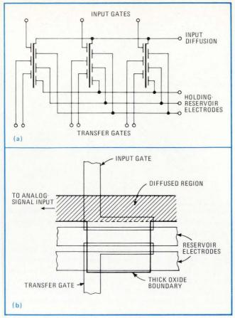
**4. New method.** In the CTD method of signal processing, the analog signal is connected to input diffusions (a) that are connected to all the charge-transfer cells, where they slosh back and forth until the desired output is achieved at that cell. A detail of the basic cell in a charge-sloshing structure is shown in (b).
