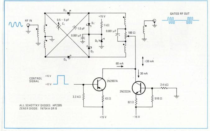
**High isolation.** Control signal (lower left) turns on pnp transistor, providing + 30 mA to gate circuit at top, to turn it off and block passage of rf signal to antenna. When control is up, npn device takes over, drawing -30 mA from gate and turning it on. Zener voltage minus positive swing of input signal establishes reverse bias on series diodes, achieving isolation of as much as 70 dB at 80 MHz.
