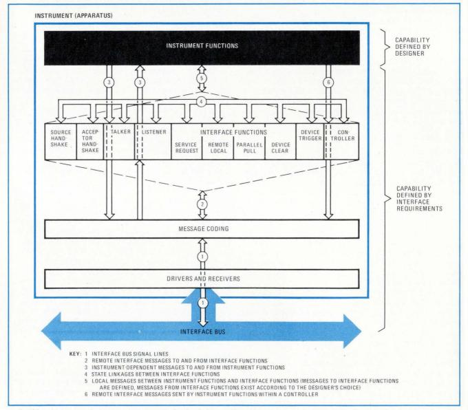
4. Partition. Instrument designs can be conceptualized as being partitioned into two areas: instrument functions and interface functions. But this division does not necessarily imply two separate physical layouts within the instrument.
