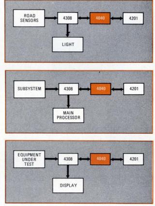
**Applications.** The 4040, with the 4308 ROM and the 4201 clock generator, could form a "smart" traffic controller (top), a preprocessor (middle), or a portable troubleshooter.
