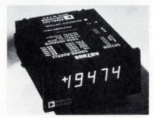
sign for 5-V DPMs has gained recognition as a standard, but until now the firm did not offer 120-V meters that could be mounted in a panel cutout that is the industry norm.
