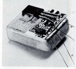
**Ovenized.** A transistor heats the crystal oven that is incorporated into high-stability versions of the PM6610 series.
