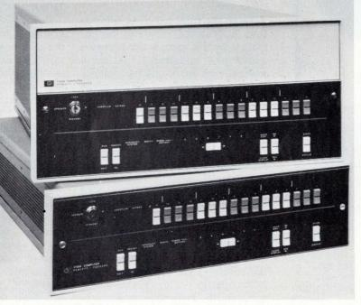
**Beginnings of family.** The model 2108A, at top, and the 2105A are the first in a line of minicomputers from Hewlett-Packard that uses 4,096-bit semiconductor memories for main storage. The machines are fully microprogramed with a 24-bit processor.
