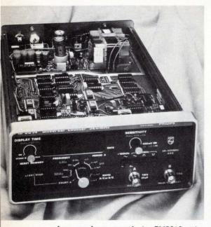
Low package count. In PM6610-series counters from Philips, four custom C-MOS circuits handle the functions that would otherwise require about 50 TTL packages.
