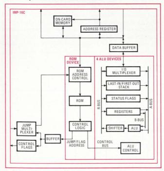
4. Sixteen bits on a board. National's IMP-16 architecture supplies a full 16-bit minicomputer capability on a single pc board. Microprogramable ROMs control the four 4-bit arithmetic logic units that do the processing. Four- and 8-bit versions are also available.
