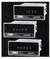
ment in the panel-mountable series contains a crystal-controlled clock and a programable divide-by-N chip which combine to yield a time base that can be varied from 0.05 millisecond to 13 seconds in steps of 0.05 ms. This enables standard transducers to produce readouts in any desired units-English today and, if necessary, metric tomorrowwhen some pin-to-pin wiring is changed.
