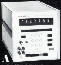
6-digit Model M106 A. Accuracy  $\pm 0.002\%$ . Range  $\pm 1$  microvolt to  $\pm 1,000$  VDC in 4 ranges. Solid-state voltage selections and digital display. Isolated remote BCD programming optional. A proven, versatile performer for bench, production or computer-controlled test systems . . . with a low basic price of \$2,375.
