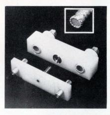
temperature rise in high-current applications—a 2,000-ampere load applied for one minute results in a 75millivolt drop through the helix connector. Insertion and retraction forces of 5 pounds nominal permit easy removal and insertion of the modular panels. 42
