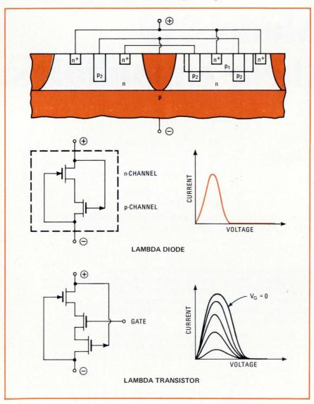
Peak-to-valley current ratios are in the order of  $10^5$  for practical devices, about  $10^4$  times greater than those for tunnel diodes. Peak voltages run in the range of 0.5 to 5 volts, and valley voltage thresholds in the range of 2.5 to 12 V, making for easy interface with other devices.
