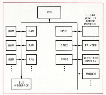
**3. Twice four is eight.** This 8-bit microprocessor chip set, which also is fabricated by Rockwell, contains more than 90 instructions with 4-microsecond execution times. All of the components shown work directly off the CPU.
