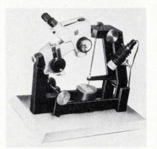
also be guided to shave parallel to conductors, eliminating smearing of gold materials and preventing remnants from building up and damaging the circuitry. The machine is suitable for use with multi-chip arrays since the scraper path operate within a controlled area. J. and A. Keller Machine Co. Inc., 2320 Milli-
