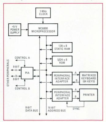
**1. Eight-bit family.** Motorola's M6800 family of components is organized around the concept of the parallel data bus. Consequently, all memory and peripheral interface adapter (PIA) chips are simply designed to hang on its CPU's eight bidirectional data lines.
