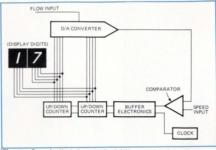
**Miles-per-gallon meter.** Key to the system is a hybrid pressure transducer with a vacuum reference etched on a silicon chip and a Wheatstone bridge composed of four resistors.
