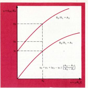
**3. Interpolation.** Family of Schade voltage curves shows how ratio of dc voltage to peak voltage (y-axis) varies with changes in the product of frequency, load resistance, and filter capacitance (x-axis) for different values of the ratio of source resistance to load resistance. For such values of  $R_s/R_L$  as  $A_2$ , for which no curve is plotted, the formula provides a linear interpolation that can greatly increase the accuracy of the calculated results.
