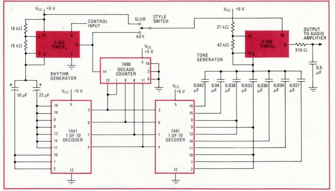
**Tuneful timers.** This music synthesizer, which relies on two IC timers, can play a simple 10-note song. Timer<sub>1</sub> generates the rhythm for the tune, while Timer<sub>2</sub> generates the tones. If the CONTROL INPUT is tied to the supply line, the tune recycles continuously. The position of the STYLE switch determines whether the tones are played individually or blended. This circuit plays "A Pretty Girl Is Like a Melody."
