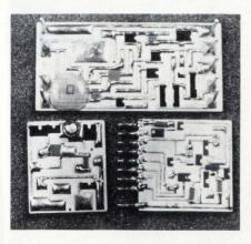
quirements of the circuit, and the user then bonds the semiconductors on the mounting pads provided. A wide variety of circuits can be developed this way, and in ordering, the customer need only furnish the circuit schematic with passive components identified, the quantity required, size limitations, maximum electrical and environmental stresses to be encountered, active devices to be bonded or not, and bonding technique preferred.
