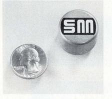
to 400 MHz with a nominal gain of 12 dB. Other specifications include a noise figure of 5 dB maximum, with the input-output impedance available in either 50 or 75 ohms. Constructed with solder pin connections, the enclosure is 1 by  $\frac{3}{4}$  inch. Price is \$27 in quantities up to 100. Delivery is from stock.
