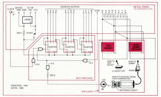
**Functional checkout.** Compact IC tester makes a complete functional check of many different logic circuits. The performance of the device under test is compared with that of a reference circuit. Series-connected decade counters provide the necessary binary inputs for the test device. A defective unit will light the display on the logic comparator. The assembled tester occupies a small metal panel (see photo).
