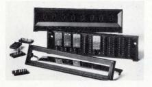
sembly has wire-wrapping terminations and a 20-pin capacity. Further, no mounting holes are needed other than a single panel cutout, and after installation of the bezel, the display package aligns itself. Industrial Electronic Engineers Inc., 7720-40 Lemona Ave., Van Nuys, Calif. 91405 [393]
