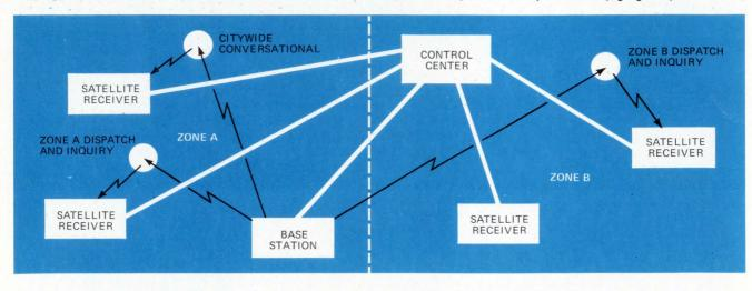
Keeping in touch. This sample digital police communication system uses phone lines (in white below) and rf links (zigzag lines).
