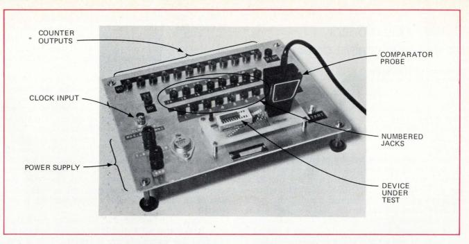
tween the counter output jacks and the numbered jacks to the inputs of the IC to be tested. Run another lead from the STOP jack to the jack following the last-used counter output. The clock signal generator can now be hooked up to the CLOCK jack. (The maximum clock amplitude should not exceed 5 v, nor the maximum clock frequency 10 megahertz.)
