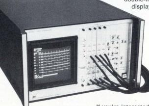
The Digiscope gives you eight channels of digital data simultaneously acquired at 50 MHz, up to 100 bits of pretrigger kokback, and single shot measurements without sacrificing critical analog information in the signals.
