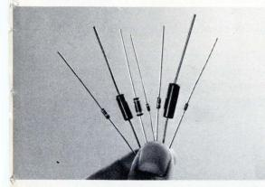
We are adding substantially increased capacity for precision parts with temperature coefficients of 50ppm/°C. And 25ppm/°C. parts are in the final stages of development. This will extend the range of our metal film performance capabilities significantly. As soon as samples of our 25 ppm resistors are available for evaluation, we'll let you know.
