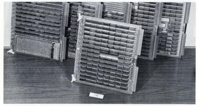
1. The big attraction. Built using standard TTL hardware, this microprogramable processor circuit requires 451 packages on five circuit boards. Using advanced MSI logic and read-only-memory programing, it requires 114 packages on one board. Yet the same circuit, when built with today's n-channel LSI techniques, can be packed into one 40-pin microprocessor package—Motorola's new M6800 system.
