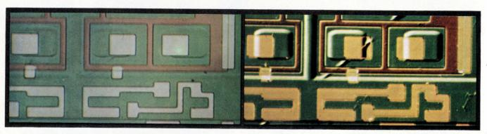
The AO DICV Series 10 Differential Interference Contrast Microscope can make a big difference. A standard brightfield microscope reveals only what is shown in the specimen on the left.
