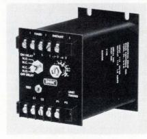
positive detent selector switch. Static output is rated for more than 100 million operations. The convertible unit also has an optically isolated ac control circuit with transient protection to 1,500 volts. Time ranges are from 0.02 to 2.6 seconds to 0.5 to 250 seconds.
