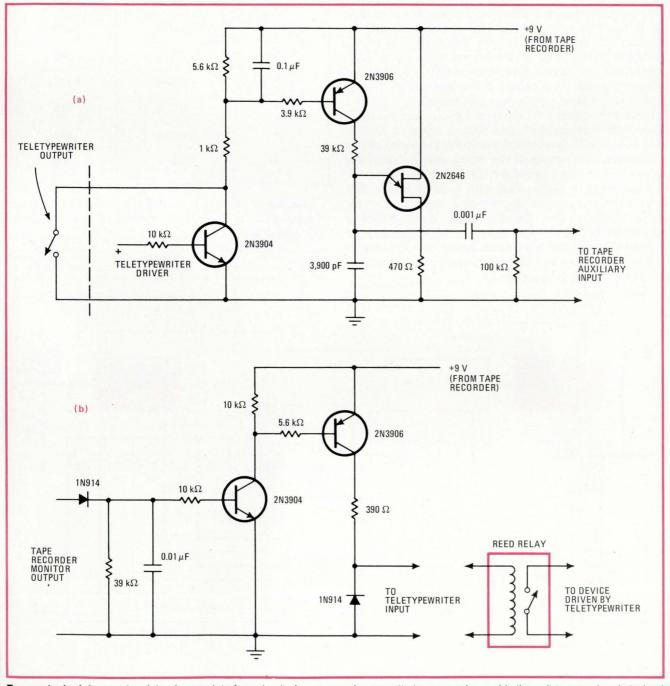
**Economical minicomputer data storage.** Interface circuits for an everyday cassette tape recorder enable the unit to record and playback teletypewriter information. The recording circuit (a) can be driven by either the teletypewriter itself or by a teletypewriter driver. The playback circuit (b) can drive the teletypewriter directly or interface with a relay driver. The recorder's battery can run both circuits.
