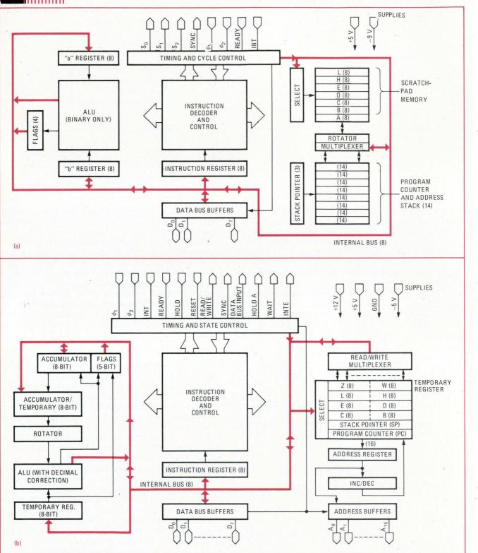
**1. Comparison.** Intel's earlier single-chip microprocessor, the 8008, has a separate scratch-pad memory and address stack (a). In the 8080, these have been combined into the six 16-bit registers (b). The accumulator has been moved into the arithmetic and logic unit, avoiding the use of the internal bus for data transfers between the scratch pad and the ALU during arithmetic and logic operations.
