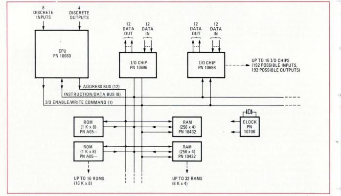
2. Four bits' worth. In Rockwell's self-contained 4-bit PPS system, versatility is a major design asset. Five compatible elements—CPU, RAM, ROM, a RAM-ROM combination chip, and an input/output buffer—provide up to 4,096 8-bit ROM words and 4,096 4-bit RAM words.
