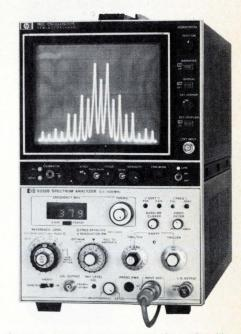
Accurate measurements are made easily with the economical 8558B spectrum analyzer (shown here in a 182C oscilloscope).
