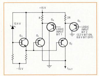
**3. Pnp-pnp.** Replacing diodes of Fig. 2 with transistors eliminates diode storage times and thus raises speed, but this change does not affect problems of changing current gain and base-emitter voltages.
