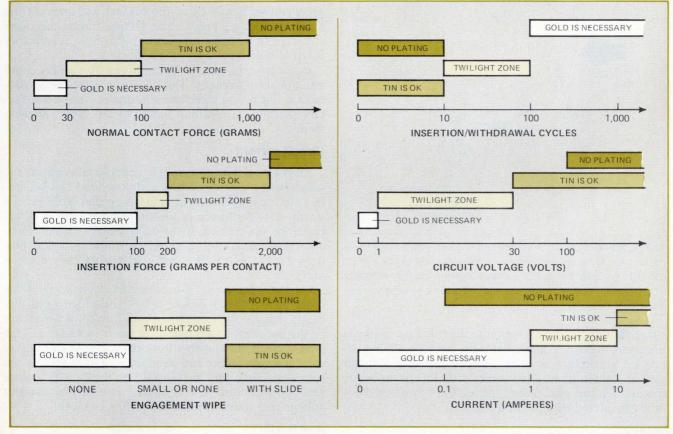
**3.** Plate it? These guidelines will help a designer to choose gold, tin, or no plate at all, for connector contacts. The recommendations relate the plating choice to both the design of the connector and the application for which the connector is intended.
