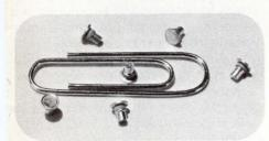
These developmental diodes have operating voltages from 100 to 143V, with operating current from 50 to 900 mA, depending upon frequency and power output.
