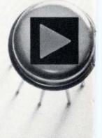
The first high accuracy FET-input op amp;  $I_b = 5pA max$ ,  $V_{os} = 1.0mV max$ ,  $\Delta V_{os} / \Delta T = 10 \mu V /^{\circ}C max$ . AD506.
