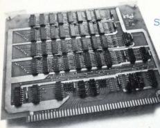
The 2102 is extremely simple to use because it requires no peripheral supporting circuits, no special supplies, nor does it require the extra design effort needed by most RAMs to interface with TTL.
