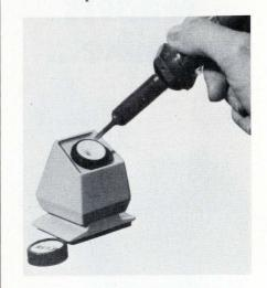
nates impurities at connections, allows irons to stay hot by absorbing a minimum amount of heat while working. No abrasives are used, and any shape of tip up to <sup>1</sup>/<sub>4</sub> inch in diameter can be handled. Re-Tip consists of a non-skid base and a replaceable cartridge.
