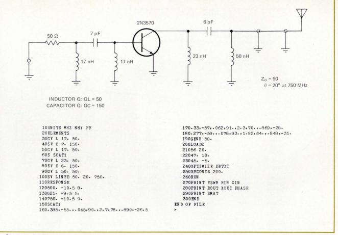
2. Starting point. The uhf amplifier is to be optimized for maximum power gain. In the Magic input data, circuit elements are listed from left to right. For inductors and capacitors, their values, as well as their Q factors, are given. S-parameters are used to characterize the transistor.
