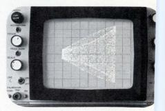
A non-triggered modulation trapezoid displa of a 1 GHz carrier modulated with a 12 MH sinewave.
