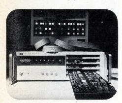
The 6145A digital current source has 200  $\mu$ s programming speed and 1  $\mu$ A (X1 range) or 10  $\mu$ A (X10 range) output accuracy.
