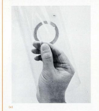
**4. Setting records.** Phase-contrast microphoto of the disk surface (a) shows the standard multiburst test video signal and the sync-tip interval (horizontal retrace pulse). At a lower magnification (b), it's possible to see the separate color bars and individual record tracks. One important advantage of the film disk (c) is that it can be handled without harming the recorded information.
