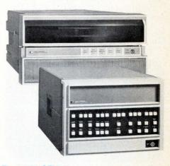
The 2123A OEM disc-based system has a data transfer rate of over a million 16-bit words per second.
