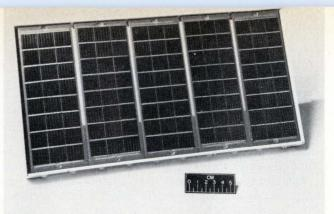
**2. Solar arrays.** Six 9<sup>3</sup>/<sub>4</sub>-by-18-inch modules are put (left) into a 50watt (at peak) array from Solarex Corp. NASA's Lewis Research Center is experimenting with encapsulating space-type solar cells between sheets of plastic for structural strength and easy handling.
