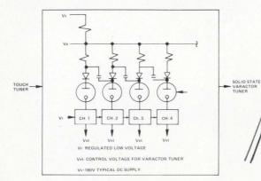
When the new varactor tuning systems for color TV sets were designed, components were required to perform two functions — illuminating the channel selector and transferring precise, regulated voltage to the solid state tuner. Reliable performance, long life and low cost were design objectives.
