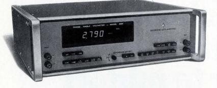
....This NEW DPAV provides complete analysis of complex AC waveforms at discrete frequencies and displays the results on a high readability  $4\frac{1}{2}$  digit display. Parameters measured are Total, Fundamental, In-Phase, and Quadrature voltage plus Phase Angle. Phase angle is displayed directly in degrees from 0° to 360° with a resolution of 0.1°.
