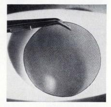
equipment. This will allow semiconductor manufacturers to supplement existing LED product lines. The wafers are made of monocrystalline GaP grown by the Czochralski method in high-pressure chambers using liquid encapsulation.
