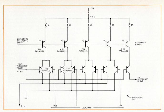
**6. Monolithic current-steering.** Current-source bit transistors  $Q_{1-4}$  operate continuously, while logic inputs switch currents from ground path to output line, thus avoiding thermal tails. Multiple transistors for each bit help assure base-emitter voltage-matching. A reference servo is also used in this circuit; it is not shown to minimize drawing complexity, but is similar to that in circuit of Fig. 5.
