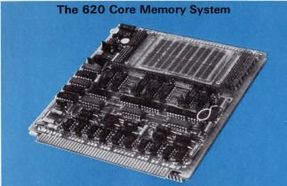
Capacity of 1,024 words by 10 bits on a single card. Planar 3-D, 4-wire configuration measures  $6.0 \times 6.4$  inches. Expandable. Access 'time: 350 nanoseconds. Full cycle time: 1.0 usec.
