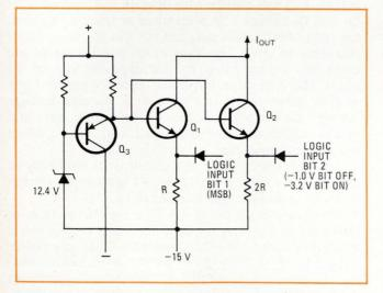
**1. Diode-npn switches.** Transistors  $Q_1$  and  $Q_2$  are switchable current sources whose currents are set by resistors R and 2R.  $Q_3$  transfers 12.4-V zener drop to resistors R and 2R to help set the individual currents. Output current  $I_{OUT}$  goes to a summing resistor. Unequal heating or cooling can cause imbalances in the base-emitter voltages of the transistors and also in the current gains, both of which affect accuracy. Logic inputs were not compatible with TTL levels.
