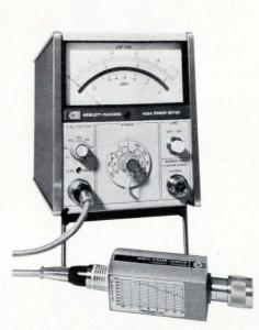
The 435A power meter's internal RF power reference provides added confidence in overall measurement accuracy.
