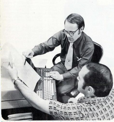
Simply input your specs (say, temperature rise, voltage and current requirements). The 9830 calculator automatically selects the fabrication parameters you need.
