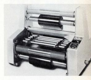
13 feet per minute. Normal working rate is 5 to 8 ft/min. By adding a 6in. core adaptor, available as an option, 1,000-ft rolls of film can be accommodated.
