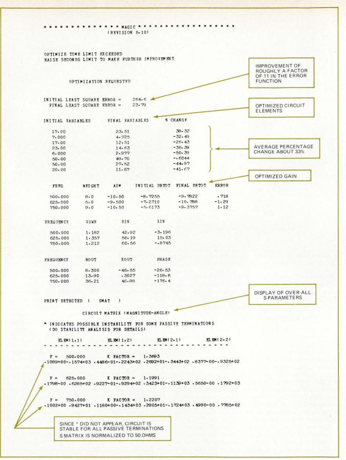
**3. Optimization run.** In a single computer run, Magic adjusts circuit-element values to achieve the desired amplifier performance. The optimized circuit produces a nominal gain of 10 decibels, which remains flat to within ±0.75 dB from 500 to 750 megahertz. The printout of the over-all S-parameters shows the amplifier to be stable. A second optimization run would further improve circuit performance.
