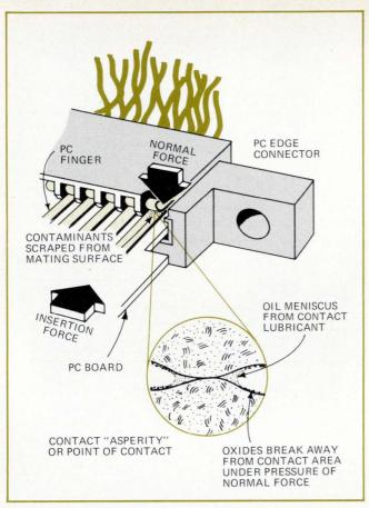
**4. The action.** Inserting a printed-circuit board into an edge connector causes the mating contacts to develop a normal force which depends on both the spring constant and the contact deflection when mated. Repeated insertions and withdrawals remove tiny particles from the surface of the pc-board fingers.
