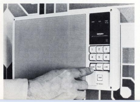
occupant to talk to the guard as soon as the burglar alarm is tripped. The idea is to provide human interruption in case of a false alarm caused by unintentional activation a major nuisance in all home security systems.
