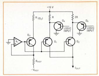
**4. Adding a reference servo.** Addition of an operational amplifier helps to compensate for changing current gain and base-emitter voltage. All bases are adjusted to maintain constant current through  $Q_3$ , and, if the transistors are matched, the currents through  $Q_1$  and  $Q_2$  are thus controlled by the operational amplifier.
