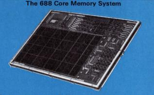
module capacity of 32,768 words by 20 bits on a single card, ndable to 64K, 128K, 256K or 512K by 10, 20 or 40 bits. Planar 3-wire configuration measures 15 x 21.5 inches. Access time: nanoseconds. Full cycle time: 1.2 microseconds. System options de: enclosures with printed circuit back panels, power supplies
