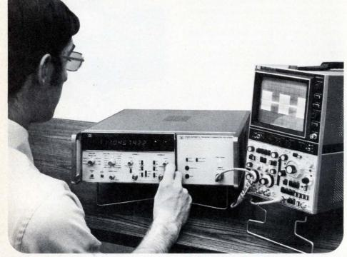
Pulsed RF and CW up to 4 GHz are measured automatically with a heterodyne converter plugged into the new counter.
