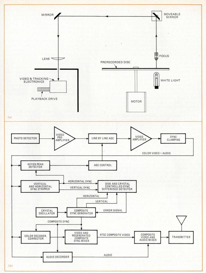
5. Recorded message. Using a white-light source and a carefully designed optics arrangement, the playback unit (a) can be built inexpensively. The electronics (b) is also simple and straightforward, but can be upgraded for improving picture quality.
