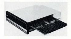
When used with a Nova 800, a 1,024 real-sample-time series can be transformed and the magnitude of the spectrum formed in 139 milliseconds. Time-domain signal-processing functions can be calculated at a rate of 2.8 microseconds per multiply-accumulate. Price is \$6,000. Elsytec Inc., 212 Michael Dr., Syosset, N.Y. 11791 [358]
