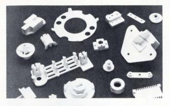
**Glass-reinforced polyester** for the fabrication of electronic parts is self-extinguishing. Applications are in circuit receptacles and circuit breakers, for example. Sizes range up to 5 by 3 by 1<sup>3</sup>/<sub>8</sub> inch in ivory or dyed colors. The material is said to surpass the characteristics of nylon, acetal and phenolic materials in certain applications.
