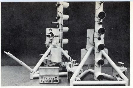
**Intruder detector.** Laser fence has six devices in vertical row. Their beams are picked up by optical receiver. Small instrument is local collector/display unit of the system.
