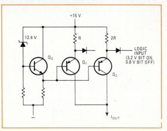
2. **Diode-pnp.** Nearly a mirror image of the circuit in Fig. 1, this circuit provides compatibility with TTL-logic inputs, but it still shows the same deficiencies in compensating for changes in transistor-current gains and base-emitter voltages.
