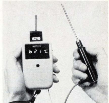
an analog-to-digital converter, MOS logic, and a small number of discrete items. There are three standard probes: chisel-end, flat-end, and a tube for holding liquids. The most likely use in electronics technology is in laboratories to check temperatures of heat sinks, transistor cans, and things like that. However, Ernest May, Kane-May managing director, expects to sell it for laboratory and production use throughout industry.
