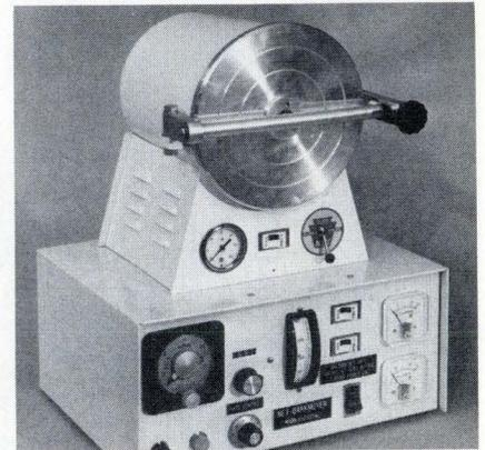
nickel-aluminum alloy. There are two heating chambers available, one measuring 4 by 4 by 10 inches, and the other, 8 by 4 by 8 in. The unit is transistorized, and the transistors are grouped into modules for easy repair.
