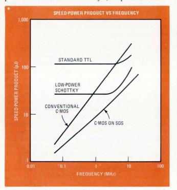
8. Power struggle. Low-power Schottky could take over some jobs from C-MOS. It operates at optimum speed-power tradeoffs for many applications, especially in the 100- to 500-kHz range, where it dissipates about twice the power of C-MOS but runs 10 times as fast.
