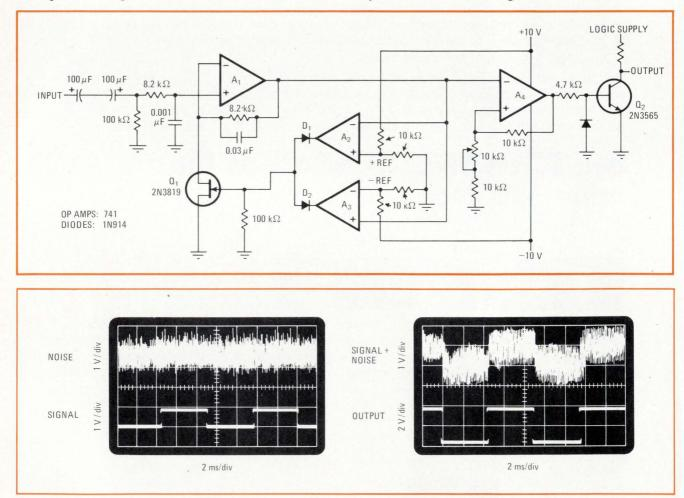
**Pulling the data out of the noise.** Adjustable-hysteresis voltage discriminator makes significant improvement in signal-to-noise ratios, as can be seen from the scope traces. The level of regenerative feedback of amplifier  $A_4$ , the voltage-discriminator stage, is adjusted to provide optimum noise immunity. The gain of amplifier  $A_1$  is controlled by transistor  $Q_1$ , which is operated as a voltage-variable resistor.
