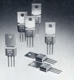
NEC's Models 2P05M, 2P1M, 2P2M, & 2P4M are P-gate all-diffused mold thyristors with an average on-state current of 2 Amps. ( $Tc=54^{\circ}C$ ). Surface treatment of the pellets with glassivation technique guarantees a high degree of reliability.
