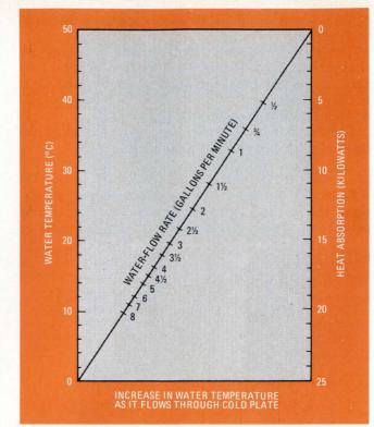
8. Warmup. By aligning a straight edge with values of the heat absorption and the water-flow rate in a cold plate, the temperature rise can be read from the scale at the left. A similar chart, found in heatexchanger manuals, enables the designer to determine the temperature rise through a heat exchanger.
