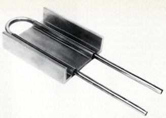
**4. Dense package.** This configuration is well suited for cooling TO-3 packages because the devices are placed directly over the coolant lines, ensuring short, efficient thermal paths to the coolant. Unit can dissipate 2 kilowatts, but occupies only 85 cubic inches.
