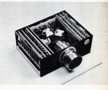
**Ring around a prism.** Bell Labs' CCD color camera of the Picturephone type has three CCD chips arranged around a prism to form the color images. Several other devices have been made using the three-level polysilicon approach.
