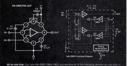
All on one chip: Our new HA-2900/2904/2905 incorporates all of the following devices on one chip in a TO-99 package with standard op amp pin out: two N-channel MOS input D.C. amplifiers, two sample and hold; one 750 Hz oscillator; four voltage comparators; and four N-channel MOS analog switches 160db. Together, these features permit design applications in precision linear systems not feasible before with conventional monolithic amplifiers and hybrids.
