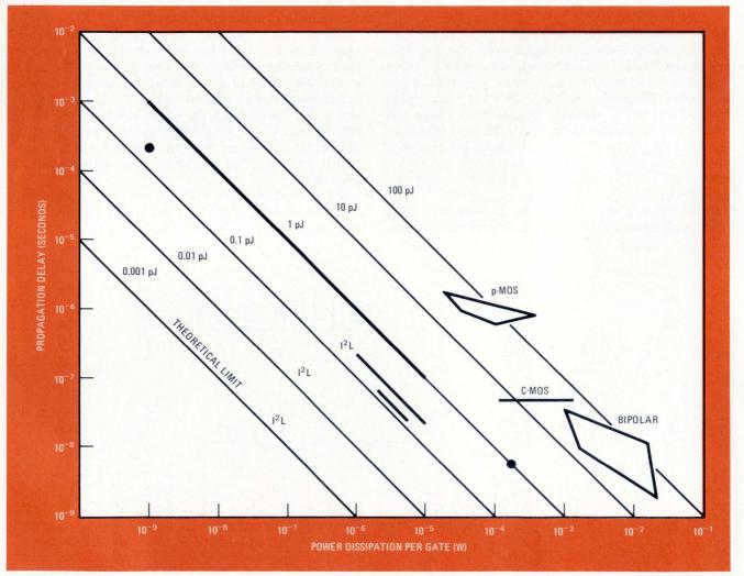
**13.** Far out. The performance of I<sup>2</sup>L far exceeds that of other logic families, MOS or bipolar, because it can operate at nanowatts per gate in less than 10 nanoseconds per gate. The projected speed-power product is less than 0.1 picojoule (for today's TTL, it is 100 pJ).
