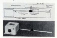
full scale. Several models are available, with displacement ranges of 0 to 12 inches and 0 to 60 in. Further, repeatability is better than 0.02%, and input is +15 volts at 250 milliamperes or -15 v at 25 mA. Tempo Instrument Inc., E. Bethpage Rd., Plainview, N.Y. 11803 [360]
