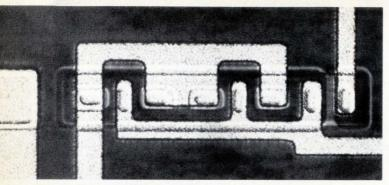
1. New gate. This I<sup>2</sup>L gate from IBM Boeblingen occupies space of one bipolar transistor, can operate at 0.1-pJ speed-power product.
