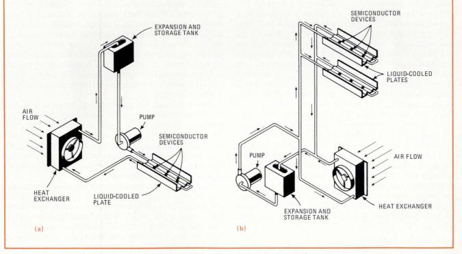
6. Flow system. A simple series-flow system is well suited for cooling a single cold plate (a). Connecting two or more liquid-cooled plates in a parallel-flow system (b) reduces the pressure drop so that a large-capacity pump isn't needed.
