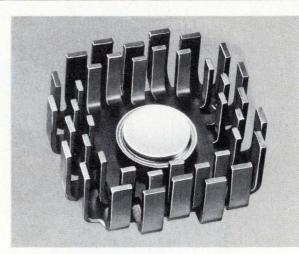
Design-to-cost criteria were missed in a touchy servo amplifier because 4 parallel devices required too much testing and matching. Designers went to single TO-6 cooled by nested HP1 and HP3 Staggered Finger dissipators. At 100°C case rise above ambient, the single TO-6 dissipates 36 watts, plenty for the application.
