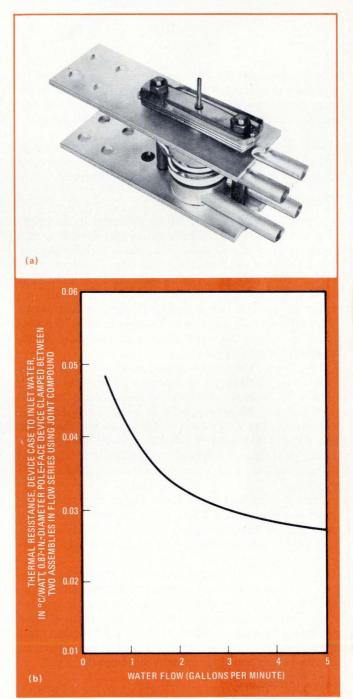
**3. Cool cooler.** The liquid-cooled solid-state copper blocks sandwiching the semiconductor device (a) provide two thermal paths (top and bottom) and dissipate 2 kilowatts. Clamp puts an 800- to 2,000-pound bite on the semiconductor device to assure a low thermal resistance—on the order of 0.034°C per watt at the interface (b).
