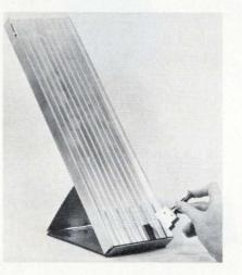
static-electricity problems often found in C-MOS devices. A flexible cable between the two tools is said to increase production rates and reduce possibility of device losses. The PIC-A-DIP works as both a 10-channel 0.3-inch dispenser or a fivechannel 0.6-inch dispenser made of unanodized aluminum. Price starts at \$87 each for single quantities. Micro Electronic Systems Inc., 8 Kevin Dr., Danbury, Conn. 06810 [395]
