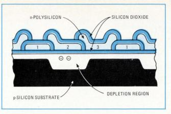
**3. Easy to manufacture.** Bell's CCD image structure, part of a Picturephone-type imager, has relaxed tolerances and high yields.
