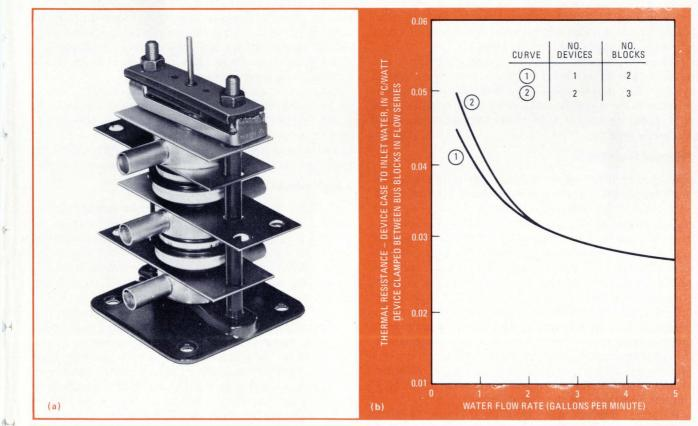
**Two stories.** Stacking two pressure-mounted devices, such as semiconductor rectitiers and thyristors, in a liquid-cooled assembly (a) is a compact technique for cooling kilowatt-level devices. Thermal resistance from the case to the coolant is low at low flow rates, and it diminishes little at flow rates above two gallons per minute (b). Adding the second device (curve 2) raises the thermal resistance a trifle (curve 1).
