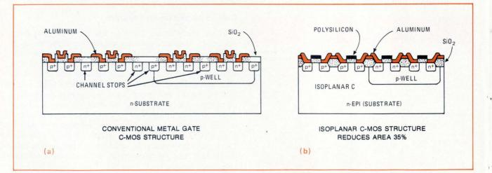
**9. Isolating C-MOS.** The active junctions that isolate devices in conventionally fabricated C-MOS (a) waste space. In Fairchild's oxide-isolated C-MOS structure, the heavily doped p $\vartheta$  guard rings are eliminated, reducing area and the capacitance that degrades speed.
