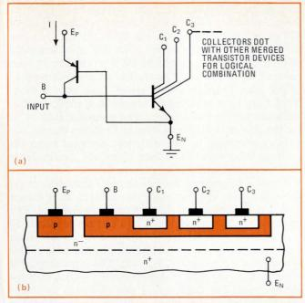
**11. Merging.** In the  $l^2L$  structure, the gate is reduced to a single complementary transistor pair, one of which is a vertical npn transistor with multiple collectors (a). As shown in this IBM structure, on silicon it merges into the space of just one device (b).
