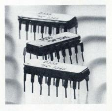
space, and reduces complexity in applications requiring two or more timer circuits. These include uses in sequential timing and synchronization, clock-pattern generation, and pulse modulation. The D555 can also be used in circuits for pulse shaping, frequency division, keyed oscillation, and other one-shot applications. Compatible with TTL,
