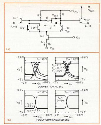
**3. Full compensation.** Fully compensated ECL circuits, the operation of which is not dependent on temperature and voltage changes, include a compensation network like the one shown in (a). This makes for a single switching characteristic (b).
