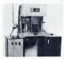
The company compares this operating rate to five conventional systems requiring 16 operators. The new system consists of an eight-ton hydraulic press and a progressive die containing a magazine with approximately 90 strips of devices, which are loaded into the press. Kras Corp., 99 Newbold Rd., Fairless Hills, Pa. 19030 [393]
