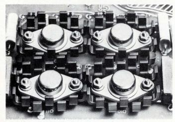
More power, higher reliability from the same TO-66s is a paradoxical requirement, but designer met it in this amplifier circuit with LB Series Staggered Finger dissipators. Nominal case rise above ambient of 90°C for bare case TO-66s permits 3 watts dissipation per device. Adding LB s doubled transistor life by giving 10°C temperature drop while increasing power to 5.5 watts per device.
