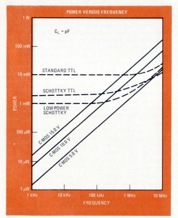
**6.** Low power, low frequency. At frequencies below 10 kHz, C-MOS can operate at dissipations of 10 microwatts per gate and is unbeatable by other logic families. But its power rates climb sharply at higher frequencies and above 100 kHz exceed those of TTL.
