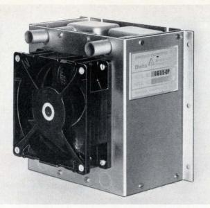
7. Cool exchanger. This double-pass heat exchanger transfers heat from the entering liquid to an air stream that is driven through the exchanger by a fan. The liquid enters and exits through the fittings above the fan. Raising the air and liquid-flow rates improves thermal performance. However, to minimize erosion and corrosion, liquid-flow rates through coolant lines should not exceed 10 feet per second.
