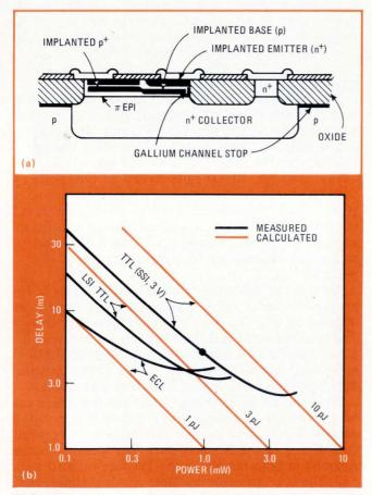
**4. Smaller, better.** Oxide isolation increases the density and speed of TTL and ECL circuits, especially when combined with ion implantation. Bell's OXIM transistor, with implanted base, emitter and collector (a), operates at very low speed-power levels (b).
