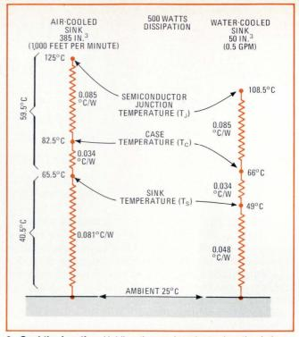
**2. Cool the junction.** Holding the semiconductor junction below a limiting temperature is crucial to thermal cooling—a key factor in long-term reliability. Here, circuit equivalents have been drawn for both an air- and a water-cooled sink dissipating 500 watts. The water-cooled system keeps the junction almost 17°C cooler and requires about one seventh the volume of the air-cooled sink.
