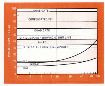
**2. Power tradeoff.** In the low and medium operating ranges, Schottky TTL operates at less power dissipation per gate than does ECL. But Schottky's power consumption goes up dramatically above 20 MHz, and in fact exceeds that of ECL at very high frequencies.
