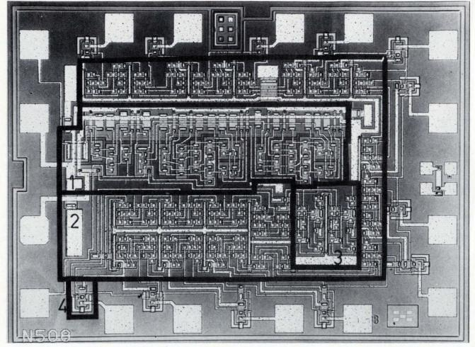
**16. Mixing it up.** In this  $2^{19}$  counter, the first two stages are built with MOS logic (region 1) and the remaining stages with  $l^2L$  (regions 2 and 3.) Note that the two  $l^2L$  flip-flops in region 3, with different layout rules from those of region 2, operate with different speeds.
