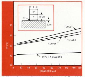
**3. Diamonds forever.** The best heat-sink material is Type IIA diamond. Other heat-sink materials are shown for comparison, however, since processing difficulties can wipe out diamond's advantages. Also emphasized is the effect of device diameter—the smaller the diameter, the less the change in temperature.
