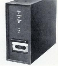
the drive system includes a controller and one bidirectional dual-differential capstan cassette transport with a speed of 6 inches per second. The system's packing density is 800 bits per inch with 8-bit characters. Read-write speed is 600 characters per second. Price is \$2,450. Cipher Data Products, 7655 Convoy Court,
