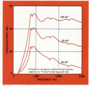
**B.** Noise mask. Minimum detectable signal intensity rises at frequencies near and above an 800-hertz interference signal. The masking effect is less significant at frequencies below that of the interfering tone. Notice the faster fall-off in detectable signal threshold at frequencies above 800 Hz when the weaker interfering signal levels are used.
