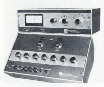
and inspection testing and includes a modified six-dial Wheatstone bridge, a linear amplifier, and a solid-state bridge power supply. The model 4271 is equipped with "low," "go," and "high-limit" lights, and provides 10 switch-selectable limit ranges. In addition to percentage
