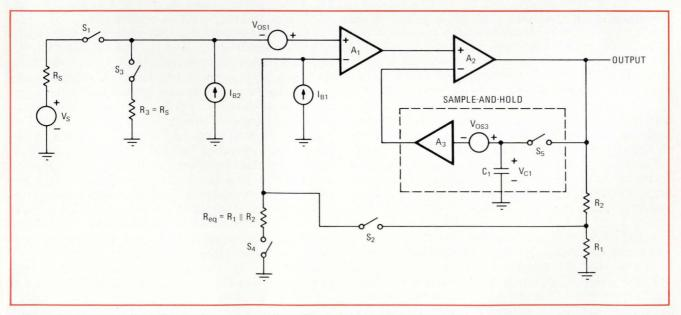
**1. Dynamic zero-correction.** Offset voltage of over-all amplifier is held to a few microvolts by inserting correction voltage at input of amplifier  $A_2$ . By applying correction voltage at interstage between  $A_1$  and  $A_2$ , errors due to sample-and-hold inaccuracies can be minimized. Sample-and-hold circuit stores correction voltage while over-all amplifier has its feedback loop open and is disconnected from source.
