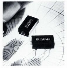
suitable for computers, computer peripheral equipment, and many types of instrumentation. Encased in a phenolic housing, the device is designed for 5-volt, 10-milliampere operation, with other voltages available.
