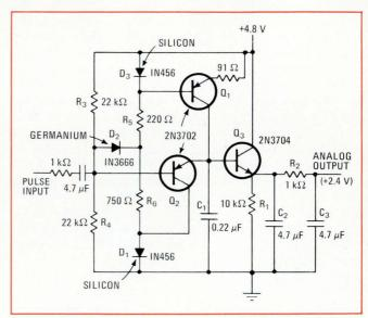
**PWM decoder.** Circuit detects pulse-width-modulated signals, supplying dc analog output over wide operating temperature range. If input control signal is interrupted, decoder output goes to preset fail-safe level. Transistors  $Q_1$  and  $Q_2$  and capacitor  $C_1$  make up sawtooth generator that drives transistor  $Q_3$ , which acts as peak-voltage detector.  $Q_2$  and  $Q_3$  are cascaded complementary emitter-followers.
