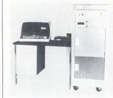
the Doctor 12 unit into a chip tester. Test programs are activated by a CRT-keyboard link, and both program and results are displayed on the CRT. In addition to go/no-go testing, the unit performs memory system debugging and engineering evaluation. Price is about \$25,000. Adar Associates Inc., 85 Bolton St., Cambridge, Mass. [394]
