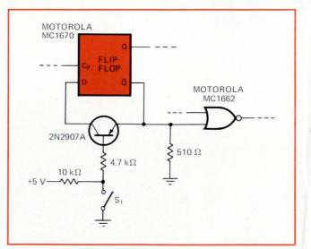
**Gating ECL signals.** Bipolar transistor gate can transfer logic signals with propagation delay of as little as 100 picoseconds. With switch closed, transistor saturates and gates signals from flip-flop's  $\overline{Q}$  output to its D input. When switch is open, transistor is cut off, and strong reverse bias at D input rejects all unwanted stray signals. The switch can be a pair of contacts or a TTL device.
