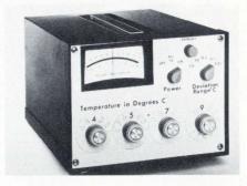
lution of  $0.001^{\circ}$ C, and long-term deviation from accuracy and stability is rated as  $\pm 0.01^{\circ}$ C. The thermometer, designated model LD-1, provides a 60-hertz rejection ratio of 70
