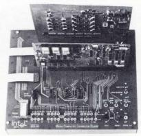
for the PROM being programed, a source of 50-v peak-to-peak programing voltages, and a 16-lead cable for direct connection to a teletypewriter, which is used to program the PROMs, test them and communicate with the microcomputer prototype. Price is \$375.
