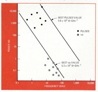
**4. More power to them.** Performance of a microwave source is rated by the product of its power and frequency squared (Pf<sup>2</sup>). This figure of merit has increased by orders of magnitude in the last two years. Present TE oscillators have achieved as much as 100,000 W-GHz<sup>2</sup> for pulsed devices, and 530 W-GHz<sup>2</sup> for cw operation.
