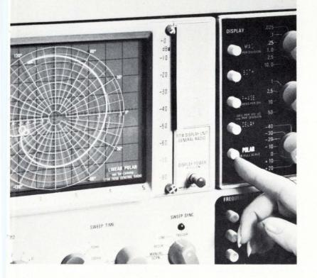
WHEN you need concise measurement data on antennas or rf cables, you'll see the value of polar (Smith-chart) displays of impedance versus frequency.
