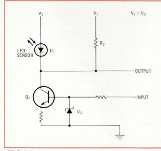
**LED Switch.** A few components can be added to enable the conventional LED to double as a photodetector.
