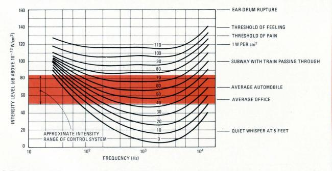
**A. Human response.** Human ears act as narrowband filters at very low signal intensities, but responses increase to a 3-dB bandwidth of several thousand hertz at an intensity of 1 watt per square centimeter.
