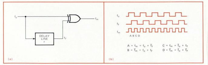
**1. Frequency doubler.** Basic multiplier circuit (a) consists of a delay line and a single exclusive-OR gate. Timing diagram (b) illustrates frequency-doubling operation. Any 2<sup>n</sup> multiple of f<sub>0</sub> is generated by cascading multiplier circuits.
