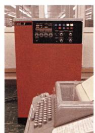
the subassemblies are entered at fourteen IBM 2796 Data Entry Units on the shop floor. The units are controlled by the System/7, which edits the data input
