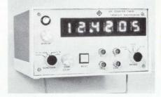
range and 0.01 second on the 1,000second range. Frequency of any ac or positive dc pulse may be measured to 2.5 MHz in three ranges. Price is \$400.
