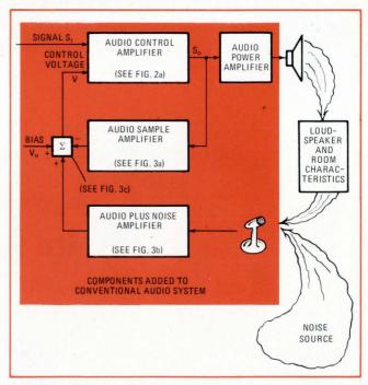
**1. Battle with noise.** Feedback system compares sampled signal output to ambient signal plus noise to generate a control voltage proportional to background-noise levels. The resulting speaker output is thus automatically adjusted to changing background noise.
