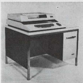
Data terminal EDX-1901 is for use in communications and data processing systems. The basic unit includes a keyboard, a page printer, a tape reader, and a tape reperfocator. It is designed for operation with the USASCII code and asynchronous operation at either 15 or 25 characters per second. General Dynamics, Electronics Division, P.O. Box 2566, Orlando, Fla. 32802 [425]
