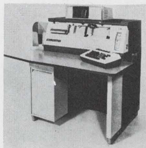
Card keypunch A150 is designed as a free-standing data input preparation device for use with electronic data processing systems. It punches and interprets standard 80-column cards. It incorporates both regular and alternate stacking pockets which are operator selectable. Unit punches and interprets at up to 20 card columns/sec. Burroughs Corp., Detroit, Mich. 48232 [427]
