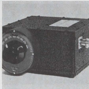
R-f filter model TTF-315-3-3EE is for the 210 to 420 Mhz telemetry band. It is a 3-section device having a 30-db form factor of 3. Typical insertion loss is 1.3 db at center frequency and average power rating is 30 w. If maximum stopband rejection is required the filter is also available in a 5-section version. Telonic Engineering Co., Box 277, Laguna Beach, Calif. [402]
