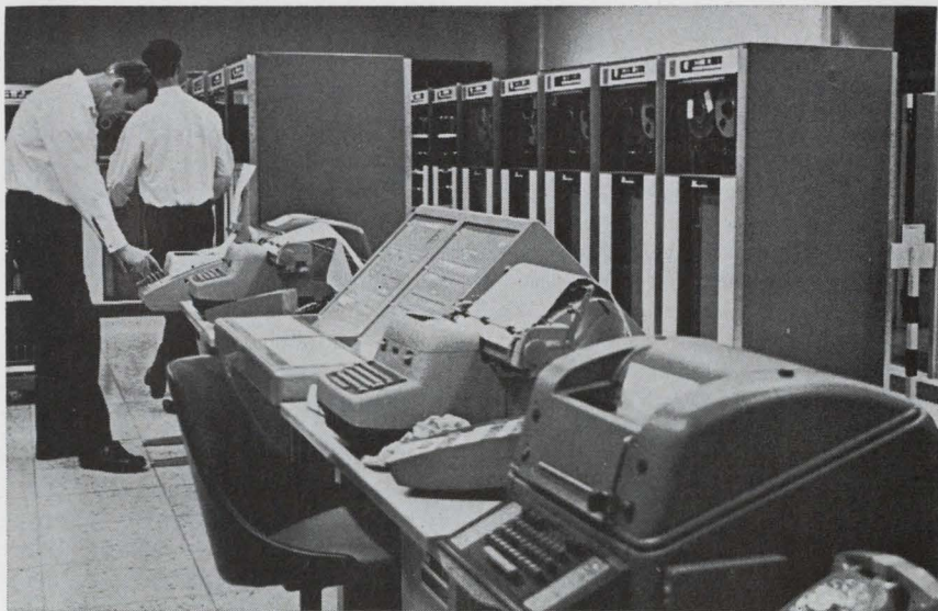
Close control. Operators in Santa Monica center mount tapes for the appropriate programs in use, and monitor the number of users in the system.
