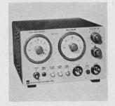
General purpose pulse generator type 1340 features wide ranges of pulse repetition frequency and pulse duration (both 108/1). Prf is as high as 20 Mhz or as low as 0.2 hz and pulse duration can be varied from 25 nsec to 2.5 sec. Ground-based positive and negative pulses are available simultaneously. Price \$395. General Radio Co., West Concord, Mass. 01781. [362]
