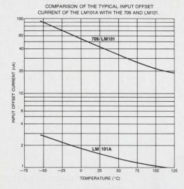
An order of magnitude improvement. The LM 101A has every advantage of the LM 101, but with 20 nA offset current and 100 nA bias current guaranteed over a  $-55^{\circ}$  to  $125^{\circ}$ C temperature range.
