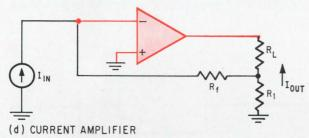
Applying controlled sources. Four basic types of controlled sources that use operational amplifiers are shown above. When combined with RC passive networks the system can be used to provide desired transfer functions, having adjustable complex poles.
