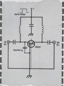
Turn this circuit off and the RF is shunted to ground through the FET's equivalent  $C_{\rm gs}$ . OFF attenuation is greater than 65 dB for small signals. ON loss is less than 6 dB. With the 2N5397 these figures hold true around 200 MHz.
