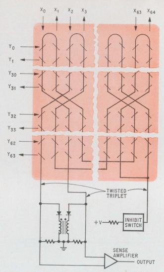
**Bow tie.** This sense winding pattern loads the driver symmetrically, and cancels most noise.
