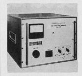
Pulse generator model 605P can provide 20 kw of power in pulse widths from 0.05 to 1,000 #sec. Pulse repetition rates can be varied from a single shot to 1,000,000 pps. Pulse amplitude is continuously variable to a maximum of 2,000 v. Standard rack mounted units are \$3,890; benchtop, \$3,990. Cober Electronics Inc., 9 Gleason Ave., Stamford, Conn. [363]
