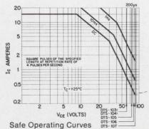
energy reliability that's needed for very tough switching jobs—resistive or inductive. The 28-volt shunt regulator above, for example, is amply handled by the DTS-103 ( $V_{\text{CEX}}$  of 80 volts). For complete data on this circuit, ask for our application note No. 42.
