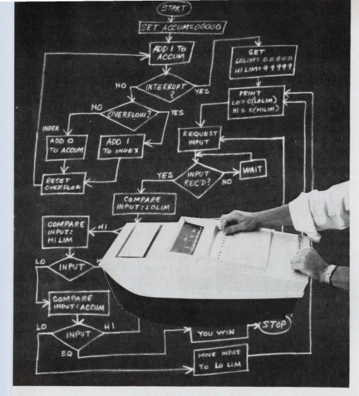
Mighty midget. Small though it is, the Nova has all the characteristics of a much larger computer, as the flow-chart in the background indicates. The chart itself represents the stored-program concept, the diamond-shaped decision blocks indicate conditional branches, and the operations at the upper left show how the program can modify itself. Strictly speaking, the read-only memory prevents direct modification, and current programing practice frowns on it, but the concept is still valid.
