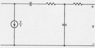
**Pairing.** Several groups of zero transmissions, including complex pairs, can be achieved with this active network. A controlled source is required for the transmission zero.
