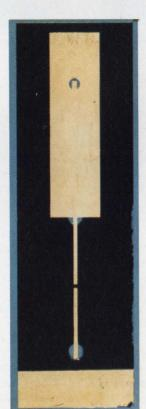
Pulser. This beam-lead microwave pluse generator was built at MIT.
