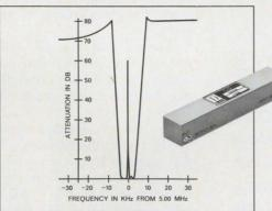
When it comes to rejecting clutter in a Doppler radar system, or the carrier in a suppressed-carrier communications system, the Damon Model 5200A Bandpass-Notch Filter gives you a double edge. It provides at least 50 db of clutter or carrier rejection — plus crystal bandpass filtering to eliminate unwanted sidebands.
