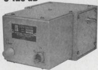
New Miniature Motorized Programmable Stepattenuators come with values as high as 129 dB in 1 and 10 dB steps. These 50 ohm series 96, 97 and 98 Stepattenuators come in a choice of 8 standard RF connector options (coaxial or waveguide); 5 standard frequency ranges; 17 standard insertion loss ranges; and single, double or triple drum assemblies internally connected in series with low reflection adapters to minimize mismatch errors.
