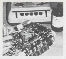
localized areas of electronic components can now be Dalic **Brush Plated** with most metalswithout dismantling!
