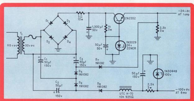
**Upstaging.** Capacitors  $C_1$ ,  $C_2$ , and  $C_3$  couple the transformer secondary to the multiplier diodes  $D_5$ ,  $D_6$ ,  $D_7$ , and  $D_8$ . Each multiplier stage will raise the no-load output voltage by about 1.4 times the rms voltage at the transformer output.
