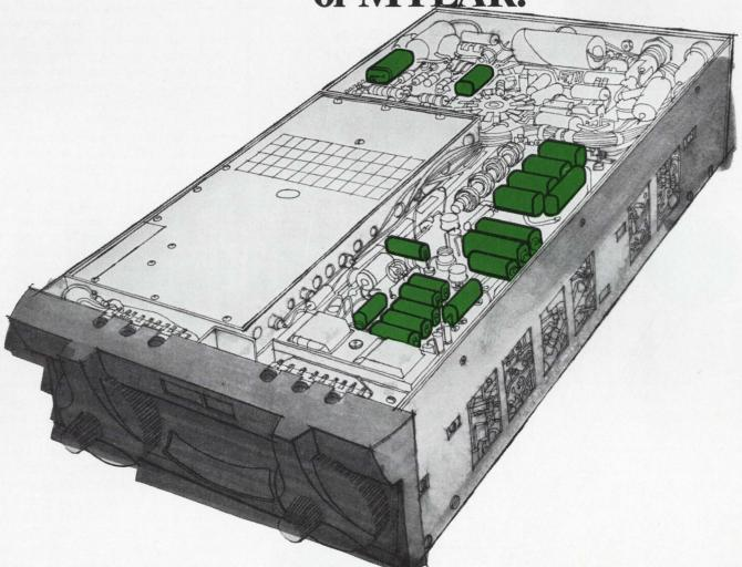
Strict aircraft safety standards require the most reliable navigation equipment available. That's why King Radio Corporation uses capacitors of MYLAR\* for their Distance Measuring Equipment. MYLAR can take temperature extremes from -60° to +150°C; MYLAR remains constantly stable under humid conditions.
