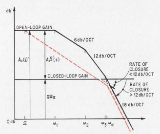
**Graphing the gains.** Bode plots for the open-loop and closed-loop gains of a typical operational amplifier. Dashed line represents the gain response of a modified op amp whose stability is assured by added RC components.
