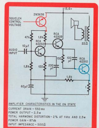
No bias. When the receiver is idle, the squelch gate ensures low standby current by removing the bias to the output stage.
