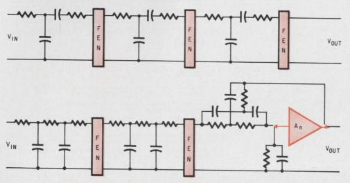
FEN filter synthesis. A sixth-order bandpass filter (top drawing) and a sixth-order elliptic lowpass filter (bottom drawing) are built with frequency emphasing networks (FEN's). These units provide the RC networks with resonance properties similar to those of LC networks.
