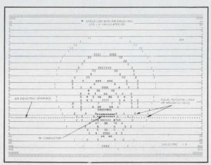
COMPUTER PLOT OF EQUAL-POTENTIAL SURFACES (RF MAGNETIC FIELD) AROUND MICROSTRIP LINE WITH &= 9
