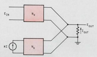
**Kuh's method.** An open-circuit voltage transfer function within a constant multiplier is made possible with a single control source and a few RC elements.
