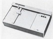
On record. The sensitivity can be set between 0.5 and 3 volts/inch.
