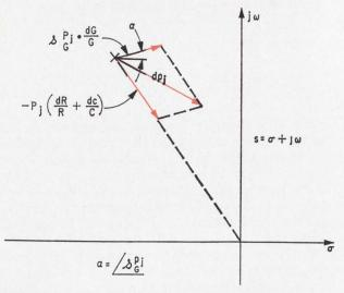
Pole displacement. The vector diagram represents the pole displacement for an active RC feedback network consisting of an active device G and resistors and capacitors. These passive components must track closely.
