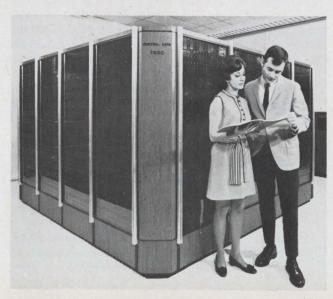
Big and small. Control Data's new computer, the 7600, is big enough for a man to step inside. And it uses tiny (16-mil) handwired arrays of toroidal cores in its memory. Despite its use of cores, the machine has a 275-nsec cycle
