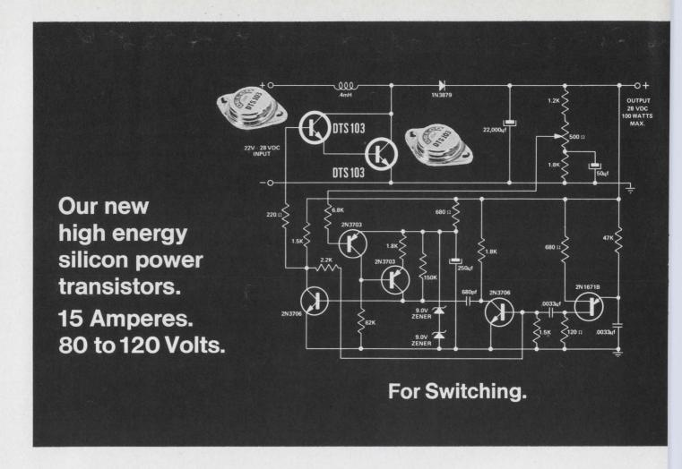
The Delco Radio DTS-100 series. NPN. Triple diffused. Rugged.
