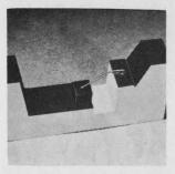
Schottky barrier mixer diode type CAY13A is a gallium arsenide device with an over-all noise figure of 6.5 db at X-band frequencies. Vswr is 2 max. I-f impedance is 350 ohms. Temperature range is —55° to —155°C. The unit is mounted on a ceramic carrier 1.9 x 0.8 x 0.35 mm. Metalized lands simplify bonding to substrate. Mullard Ltd., Mullard House, Torrington Place, London WC1, [440]
