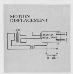
Linear variable differential transformers (LVDTs) can be used to provide the same type of signal system phase reversal.
