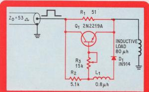
Anti-inductive.  $Q_1$  lowers the impedance of the network in proportion to the increased reactance across the load.
