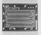
Two 64-bit shift registers, each with a single-phase clock, provide high speed operation from d-c to 1 Mhz and power consumption of less than 3 mw per bit. The MOS products are the 3305 quad 16-bit unit in a dual in-line package, and the 3306 dual 16-bit/single 32-bit unit in a TO-100 container. Fairchild Semiconductor, 313 Fairchild Dr., Mountain View, Calif. 04041. [442]
