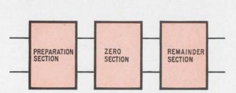
Cascading. Transmission zeros and driving-point admittance can be achieved simultaneously with a three-section arrangement connected in cascade.
