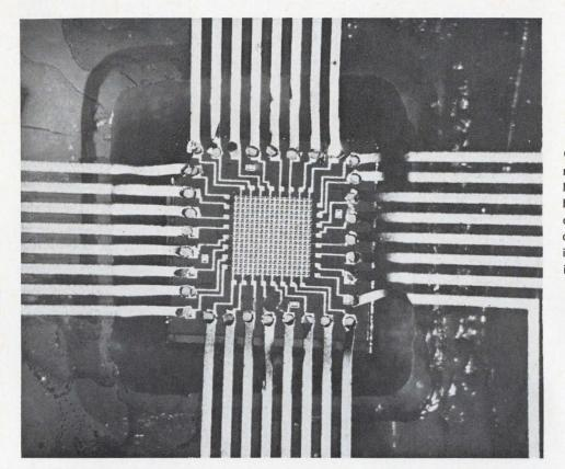
Over the edge. In this read-only memory from MIT's Lincoln Lab, the beam leads are formed on the substrate overhanging the cavity into which the chip is inserted.
