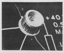
Norwegian hybrid. The trigger is a thinfilm IC made for counters and readers.
