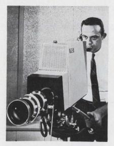
Two down. RCA's new color television camera has one pickup tube instead of the conventional three.
