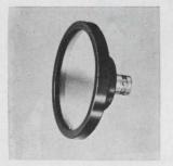
Silicon Schottky barrier photodiode PIN-25 has an active area of 7 cm². Response time is 5 nsec or less. Capacitance at 90 v is less than 100 pf/cm². Linearity of response extends over 8 decades. Noise equivalent power is 10—13w in a 1 hz bandwidth. Reverse leakage current is less than 10—7 amps cm². United Detector Technology, 1732 21st St., Santa Monica, Calif. [441]
