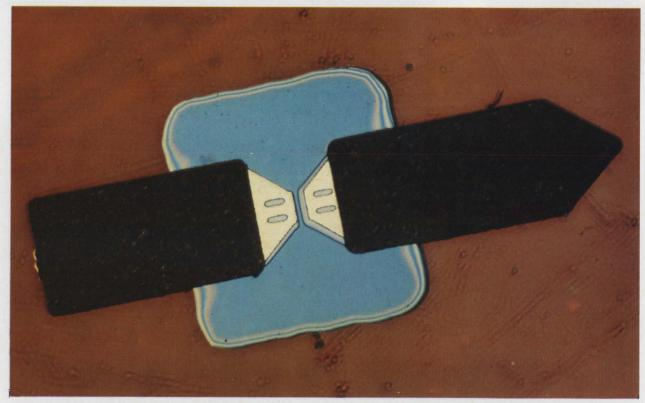
Isolationist. This surface-oriented pin diode, developed by Texas Instruments for use in the MERA program as a transmit-receive switch, has beam leads and provides better than 20-db isolation with an insertion loss of less than 0.5 db. Total capacitance is 0.1 pf and series resistance is 3 ohms.
