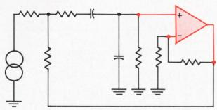
Second-order transfer functions. A typical circuit that can be used to produce second-order transfer functions is this one proposed by Sallen and Key. It assures stable frequency operation and is easily built with a small number of components.
