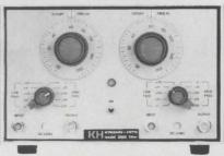
MODEL 3202 provides continuously adjustable high-pass, low-pass, bandpass and band-reject functions over frequency range of 20 Hz to 2 MHz. Two-channel bench unit shown; 51/4"x 85/6" x 151/4"-rack units available.
