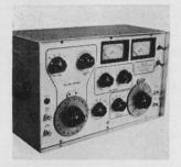
Power meter 6863-1 provides information on conducted EMI, displaying corrected EMI current, line impedance and calculated EMI power values. Current probes couple to the unknown impedance and measure impedance magnitudes from 0.3 to 1,000 ohms and phase angles ± 180° from 15 kbz to 30 Mhz. Solar Electronics Co., 901 Highland Ave., Hollywood, Calif. [361]
