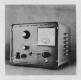
Model 222 Maxi-Max voltmeter accepts input transients and stores the peak value for reading on the built-in meter, or for plotting using the external output. It can describe the larger of the plus or minus peaks of a given transient. The voltmeter has a dynamic range of —50 db from 10 v. Price is \$1,500. Marshall Research and Development Corp., 15A St., Burlington, Mass. [365]
