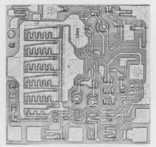
Steady climate. Compensation circuits keep drift down to  $\pm 0.002\%/^{\circ}C$ .
