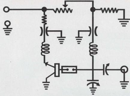
TA7403 is a new configuration... designed especially to simplify oscillator circuitry. Featuring 0.5 watt output at 2 GHz (at 21 V operation), this all-new RCA epitaxial silicon n-p-n transistor will be especially attractive to designers looking for a device that acts as a superior self-excited oscillator at L-band and higher microwave frequencies.
