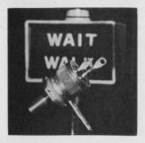
Bidirectional triode thyristors series BTV0400 handle up to 3,600 w and provide their own built-in electrical isolation. The case is fully insulated from the mounting stud. Five types are available for use with peak offstate voltages of 100 to 600 v. All types handle up to 10 amps of on-state rms current. Transitron Electronic Corp., 168 Albion St., Wakefield, Mass. [436]
