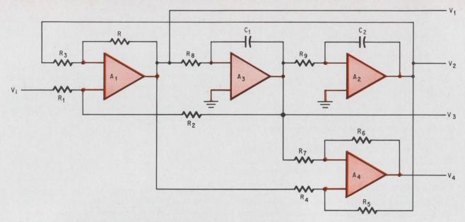
Miller integrator. One approach to achieving a desired transfer function is to use a basic Miller integrating network consisting of amplifier and RC network. Several such units are employed here to produce second-order transfer functions.
