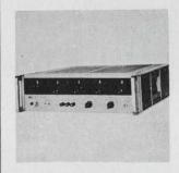
A-c calibrator 6921A has a 25-w output and supplies either a calibrated voltage or current to its load. The rms amplitude of its output is within  $\pm 0.25\%$  of selected value. The unit has 4 voltage ranges: 0 to 1.4, 14, 140, or 280 v rms. It has 5 current ranges: 0 to 1.4, 14, or 140 ma rms, or 0 to 1.4 or 5 amps rms. Hewlett-Packard Co., Locust Ave., Berkeley Heights, N.J. [366]
