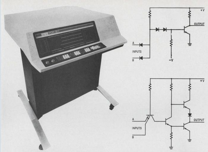
Little giant. This computer, the all-IC PDP-8/I, can be more powerful than the discrete version because it has room inside for several optional features. It's small enough for a desk top.
