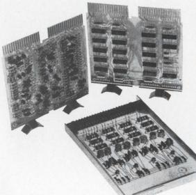
**Evolution.** Three stages in the development of DEC's line of circuit modules; the system modules at bottom, R series at left, and new M series at right.
