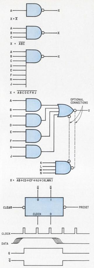
Logic configurations. All these gate forms are available in TTL circuits.
