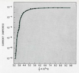
**Threshold.** Plot of electrical conductivity in sodiumdoped CdS tap crystal against reciprocal temperature shows a gradual decay of current as temperature rises until a sudden drop point is reached. Temperature range covers 115° to 300°.
