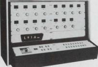
New <u>automatic</u> Linear IC Tester offers simple, <u>pre</u>programmed operation
