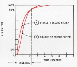
**Rise-time measurement.** Rise time of the d-c output response is the time it takes the curve to go from 10% to 90% of its maximum value. Rise time is the same for both filters, but the double-filter section reaches the 99% point faster than the single-filter section.
