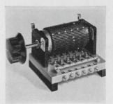
R-f programing switch has six normally-open contacts that can be arranged in any combination of fan-in and fan-out groups. Maximum crosstalk is 80 db; insertion loss, 0.4 db. Up to 270 Mhz minimum isolation is 60 db and maximum vswr is 1.09; up to 500 Mhz, minimum isolation is 45 db and maximum vswr is 1.30. Sealectro Corp., 225 Hoyt St., Mamaroneck, N.Y. 10543 [424]
