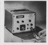
Go/no-go noise limit tester 60-2300 can be used to inspect precision or trimmer, wirewound or film potentiometers. The unit contains a constant current source to energize the wiper and a high input impedance adjustable limit detector to monitor wiper voitage. A panel light indicates when a preset limit is exceeded. Solatron Enterprises, Venice, Calif. [363]
