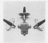
Airborne antenna array type 56360 may be mounted on missiles with diameters of less than 18 in. It consists of 3 low-silhouette monopole antennas and a 3-way power divider. It provides an omnidirectional pattern in the frequency band 1.435 to 1.540 Ghz, and operates at altitudes to 100,000 ft, and at air speed of Mach 2. Andrew Corp., 10500 W. 153rd St., Orland Park, III. [404]
