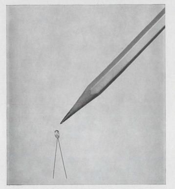
The new T-3/4 lamps used in Tung-Sol readouts, both digital and alphanumeric, provide important performance advantages without loss of effective brilliance. The low-power factor is especially advantageous where energy-source weight must be minimized—such as in aircraft and space vehicles.
