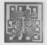
High-speed TTL one-shot circuit, or monostable multivibrator type TT $\mu$ L9601 features a retriggerable design. It provides a stable and accurate output pulse adjustable from 50 nsec to any width within the range of practical capacitor values. Input circuitry has a max. repetition rate greater than 10 Mhz. Fairchild Semiconductor, 313 Fairchild Dr., Mtn. View, Calif. [443]
