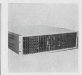
Magnetic core memory model DC-32 is a medium speed 3D unit with 4,096 and 8,192 word basic modules available from 4 to 26 bits in 2-bit increments. Full cycle time of typical 4096 x 8 unit is 1.5 µsec and will vary up to 40% in larger configurations. Access time is 600 nesc. Prices start at \$3,350. Datacraft Corp., P.O. Box 23550, Ft. Lauderdale, Fla. 33307. [383]
