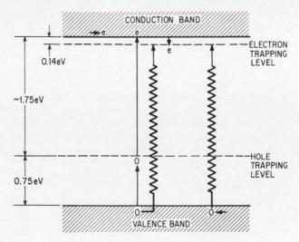
**Energy model.** Wavy arrows represent radiative transitions, solid arrows those of stimulating energy in this representation of tap storage mechanism.
