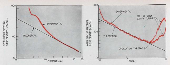
Regular curves. TI's double epitaxial diode (right) shows the uniformity of breakdown of guard ring diode.
