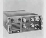
Ten-watt portable single-sideband radiotelephone and radiotelegraph unit operates up to two independent and two dependent channels in the 1.6 to 15 Mhz range. It can be powered by "D" batteries, alkaline cells, or nickel-cadmium batteries which may be recharged from a 12-volt auto electrical system. Kaar Electronics Corp., 1203 W. St. Georges Ave., Linden, N.J. 07036 [428]
