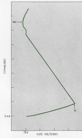
Negative resistance. Oscillograph of the current voltage characteristic of a sodium-doped CdS crystal at 4.2°K shows negative resistance. Values of V<sub>t</sub> and V<sub>m</sub> are, respectively, 145 v (I=7ma and 75 v (I=29ma). Tap crystals are unique because their negative resistance depends on the intensity and duration of stimulation.
