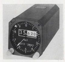
Twice told. Unit indicates altitude with both a pointer and a digital display.
