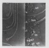
Copper-clad laminate Micarta 65M27 eliminates "measling" (shown at right in photo) in the normal manufacture of printed circuits. It meets requirements of Mil-P-13949. It is translucent light green and ranges in thicknesses from 1/32 to 3/4 in. The laminate is available in standard sheet sizes with copper on 1 or both sides. Westinghouse Electric Corp., Hampton, S.C. [345]
