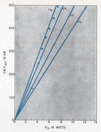
Ins and outs. Dots show efficiencies of about 9 Ghz for TI diodes while lines show projected efficiencies.
