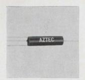
Subminiature case style C reed relay is designed for high speed switching applications. It features axial leads and is available as an unshielded model in Form A and C. Reed package is hermetically sealed, gas filled. Contact rating of Form A is 500 ma and Form C withstands currents up to 100 ma. Aztec Electronics Inc., 163 Liberty Ave., Anaheim, Calif. 92801. **[341]**
