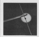
Microminiature forward regulator diodes, with from 1 to 6 individual junctions offer low voltage and low dynamic impedance. Four discrete voltage ranges are offered from 0.470 to 3.0 v, with or without controlled stored charge. Units may be operated with forward current from 0.1 to 10.0 ma. Reverse voltage at 10 u.a is 10 v. Computer Diode Corp., Fair Lawn, N.J. [442]
