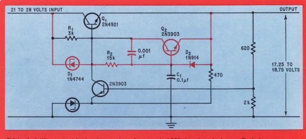
**Sidetracked.** When output load resistance drops from nominal 360 ohms to a short, zener  $D_1$  starts conducting. This causes  $Q_2$  to conduct and shorts out  $Q_1$ 's base-emitter junction. The zener's high reverse resistance and  $R_2$  limit the load current until the short is removed.
