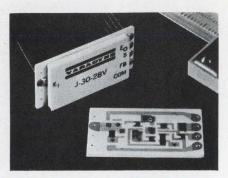
is 80 decibels at 10 kilohertz, and the device can be used from 10 hertz to 600 khz. Peak deliverable power is 10 watts normally, and 24 watts if the regulator is coupled to a 36°C heat sink. The active element in the device is a Motorola operational amplifier.
