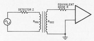
**Impedance matching.** If the detector impedance is lower than the amplifier noise resistance, a transformer is required to increase the detector impedance.
