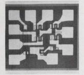
R-f/i-f amplifier LM171 is a versatile circuit that can be used in the emitter-coupled or cascode configuration from d-c to 250 Mhz. In the cascode configuration it provides 100 Mhz tuned power gain of 27.5 db. In the emittercoupled configuration it provides 100 Mhz tuned power gain of 24.6 db. National Semiconductor Corp., 2950 San Ysidro Way, Santa Clara, Calif. [436]
