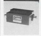
The 1,750-1,850 Mhz and 2,200-2,300 Mhz telemetry bands are efficiently diplexed using the F173A. Consisting of 2 bandpass filters, the unit is suited to both transmit-receive diplexing and signal separating or combing. Insertion loss in each band is under 0.35 db; isolation between bands, over 60 db. Peninsula Microwave Laboratories, 855 Maude Ave., Mtn. View, Calif. [407]
