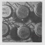
Three families of dual MOS transistors are offered with and without diode gate protection. Minimum source-drain breakdown voltage for the SD5014/15 is 120 v; for the SD5012/13, 65 v; for the SD5010/11, 30 v. Threshold voltages are typically.4 v; transconductance ratios, 0.8 to 1.0. Solid State Scientific Corp., Commerce Drive, Montgomery, Pa. 18936. [441]
