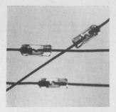
Epitaxiai silicon tuning varactors series MA-45000 are 75 and 110 v units designed for large capacitance variation with bias. Typical performance is shown by the MA-45011, which has a typical r-f input power of 5.0 w, minimum breakdown voltage of 75 v, and a power dissipation of 350 mw. Units have wide applications for vhf-uhf. Microwave Associates Inc., Burlington, Mass. **[440]**
