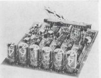
**On its own.** The counter, with no power source, amplifier or controls, is intended for design into new systems.
