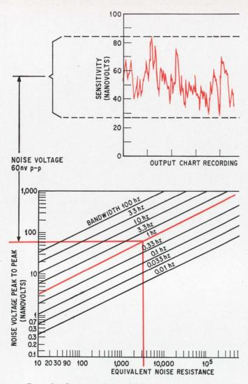
**Example.** Designer plots a 3-kilohm noise resistance and reads the value of noise voltage obtained where this line intersects 1 hertz. In this example, the value is 60 nanovolts. Then he checks the peak-to-peak value of the output chart to be sure that the value doesn't exceed 60 nanovolts.
