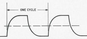
**Charging signal.** Shunting a high-resistance signal by stray capacitance produces an exponential waveform.
