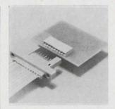
Flexible nat cable connectors called AMP-UNYT use an insulation-piercing crimp to make physical and electrical contact with the cable. Designed for use with cables meeting NAS729 (0.063 in. wide conductors on 0.100 in. centers), these connectors are available in cable-tocable, cable-to-wire, and cableto-board configurations. AMP Inc., Harrisburg, Pa. [342]
