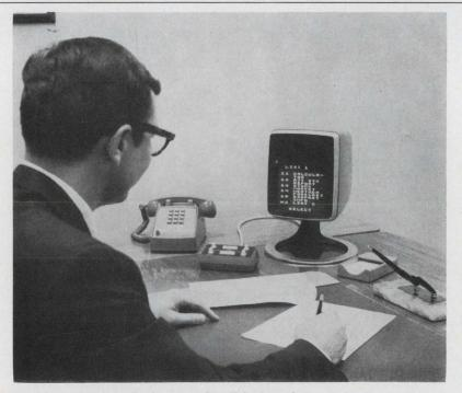
**Ring up a computer.** Engineers at Bell Telephone Laboratories in an in-house experiment, linked an unmodified commercial computer to this Picturephone so their device could be used as a desk terminal to display data on such things as inventories and news, stock, and weather. Bell plans additional tests; no marketing plans have been made.
