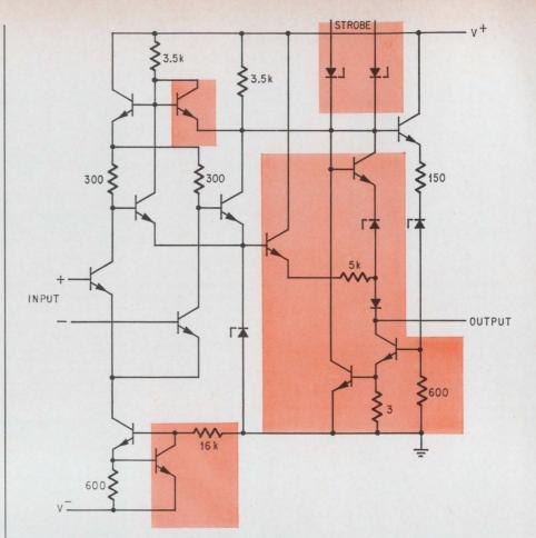
**Second thoughts.** Circuitry in the shaded areas has been added by Robert Widlar to his original design for an IC voltage comparator.
