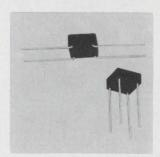
Single-phase-bridge, silicon rectifiers model B172 offer reduced space requirements by handling maximum power per unit size. Units include double diffused, passivated junctions. in a cold case design for high reliability. Current rating is 2 amps with free air mounting. Voltage ratings range from 50 to 1,200 v piv. Edal Industries Inc., East Haven, Conn. [439]
