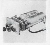
Master oscillator-power amplifier cascade subsystem 10078 is for drone control use. It consists of a pulsed master oscillator tetrode cavity, driving a Class C power amplifier tetrode cavity rated at 14 kw output. Operating range is 410 to 460 Mhz. Duty cycle is 0.00015; output impedance, 50 ohms. Microwave Cavity Laboratories Inc., 10 N. Beach Ave., La-Grange, III. [405]
