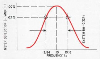
**System bandwidth.** Bandwidth for output response is found by measuring the width of the curve at the 70.7% values; for this curve, the bandwidth is 0.32 hz.
