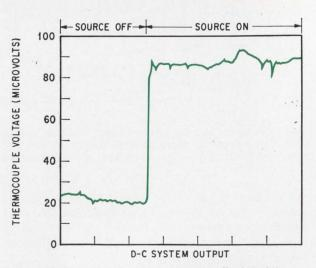
**D-c output.** Even though the source is off, plot of the d-c output indicates an error voltage due to the ambient temperature of the thermocouple junction.
