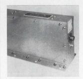
Amplifier-multiplier subsystem, packaged as a single unit features a bandwidth of 750 Mhz and operates over a temperature range from 0° to 70°C. It has a multiplication ratio of 36 to 1, requires no tuning, and operates with an output frequency of 8.375 to 9.125 Ghz from an input of 233.6 to 253.4 Mhz. Applied Research Inc., 76 S. Bayles Ave., Port Washington, N.Y. **[408]**
