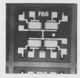
Monolithic MOSFET quad device HRM8052D is packaged in a  $\frac{1}{4} \times \frac{1}{6}$  in. flatpack. Each of the FET's in the chip is a P-channel, enhancement mode, diode protected, insulated gate device optimized for multichannel commutation applications. Each device has a typical channel resistance of 300 ohms with a -10 v bias. Hughes Aircraft Co., Newport Beach, Calif. [438]
