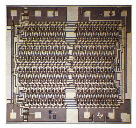
This is a photomicrograph of the longest static shift register available in a production device today. It's TI's new dual 50-bit MOS IC...one of eight new computer-designed circuits. Companions include three other dual SRs (32, 25 and 16 bit), a six-channel analog switch, an audio amplifier, a dual full adder, and a dual 3-input NOR gate.
