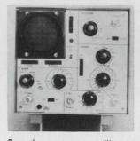
General purpose oscilloscope model 101 is suited for applications on CATV sites, remote communications sites, flight lines, ship-board and field use. It combines 50 mv/cm sensitivity and d-c to 20 Mhz bandwidth. The unit measures 9 x  $8\frac{1}{2}$  x 15 in. and weighs 17 lbs. Price is \$665; delivery, from stock. Texscan Technical Products Corp., Indianapolis. [367]
