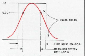
**Equivalent noise bandwidth.** By definition, true noise bandwidth is 1.57 times the measured bandwidth. In this case, the measured bandwidth is 0.32 hz, so the noise is 0.5 hz.
