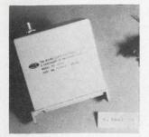
Ku-band tunnel diode amplifier model NC-12001 operates at 12 to 12.3 Ghz, with a noise figure of 6 db max. and intermodulation distortion in the third order not greater than -35 db relative to either of two signals at -50 db max. input. Input vswr is 1.20 and supply voltage is 18 v d-c. Micro State Electronics Operation, Raytheon Co., 152 Floral Ave., New Providence, N.J. [401]
