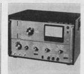
Modulation meter model 409 provides wide carrier ranges—a-m: 3 to 1,200 Mhz; f-m: 3 to 1,500 Mhz—and measures percentages of amplitude modulation in 3 ranges, and f-m deviation up to  $\pm 600$  khz in 6 ranges. A-m measurement accuracy is better than  $\pm 3\%$  to 5 khz; f-m, better than  $\pm 5\%$  to 50 khz. Winslow Tele-Tronics Inc., 1005 First Ave., Asbury Park, N.J. 07712. [364]
