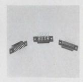
Dual-in-line IC sockets are available in the W series for hard wiring and the S series for solder type terminations. All types accept any dip with round, square, rectangular, hollow or solid leads with a cross section of 0.008 in. to 0.023 in. and 0.090 in. minimum lead length. Body material meets MIL-M-14F. Robinson-Nugent Inc., New Albany, Ind. 47150. [348]
