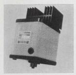
Four a-c to d-c plug-in power supplies have a current rating of 3 amps at output voltages ranging from 6 to 10 v. Line regulation is  $\pm 0.05\%$  and load regulation is either  $\pm 0.5\%$  or  $\pm 0.25\%$  depending on the model. Designed for use in an ambient temperature range from 0 to  $55^{\circ}$ C, the units require no additional heat sinking. Acoplan Corp., Easton, Pa. 18042. [381]
