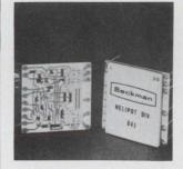
Miniature, hybrid, cermet thickfilm ladder switch model 841 is designed for use in digital to analog conversion systems. It offers 4 switching sections, each using 2 bipolar transistors. Rise and fall time is typically 200 nsec, and load range is 0 to 5 ma. Operating temperature range is -55° to +125°C. Beckman Instruments Inc., 2500 Harbor Blvd., Fullerton, Calif. [347]
