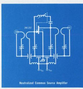
High  $g_m - 6000 \mu$ mho min – and low  $C_{rss} - 1.2$  pF max – combine to give these results in a neutralized common source amplifier. But if you're against neutralizer twiddling then design a common gate circuit. With the 2N5397 it'll be unconditionally stable up to 800 MHz and, at 450 MHz, still have 13 dB power gain with NF less than 4 dB. Used either way – CS or CG – the FET's "square law" character reduces inter- and cross-
