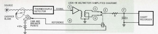
**Synchronous system.** Lock-in voltmeter, in color, replaces amplifier in basic sync system; chopper blade is rotated at a constant speed between the source and detector. At input A, detector produces a square-wave voltage, with amplitude proportional to radiant energy, superimposed on d-c and noise voltages.
