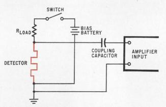
Semiconductor bias. Battery enables an engineer to vary the resistance of a semiconductor in proportion to the level of incident radiant energy. The battery also makes it possible to produce an a-c signal voltage when the radiant energy is chopped.
