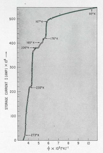
**Current curve.** In sodium-doped ZnO tap crystals that have been thermally stimulated electrical conductivity increases, remaining high at low temperatures. But current drops sharply at about 167°K and picks up briefly at 176°, 185°, 206° and 2,350°K. Curve starts at 77°K and extends to room temperature.
