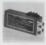
Pulse amplifier model 1002A is designed for MOS driver applications. With a +2 to 5v pulse into its 50 ohm imput, from a word or pulse generator, and a -22 v d-c supply voltage, it supplies a pulse with a minimum of -15 v into a 200 ohm load with 50 pf across its output. Unit measures 1 x 2 $\frac{1}{2}$  x 5 in. Price is \$150. Multi-Phase Electronics, Van Nuys, Calif. **[388]**
