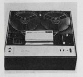
Stereo tape recorder has three heads for sound-on-sound and special-effects recording. Sony 355 operates at three speeds ( $74_2$ ,  $33_4$ ,  $17_6$  ips), and has a 7-in.-reel capacity. Features include noise suppressor, tape-source monitor, scrape-flutter filter. The unit retails for less than \$229.50. Superscope Inc., 8150 Vineland Ave., Sun Valley, Calif. 91352. **[421]**
