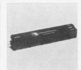
Transistor amplifiers ranging from 1 Ghz to 1.8 Ghz deliver output powers of 1 to 3 w depending on center frequenc and bandwidth. Typical model 1600-40-1.5-25D has a center frequency of 1.6 Ghz and a minimum 1 db bandwidth of 40 Mhz at a power output of 1.5 w with 25 db gain. Dimensions are 2 x 15/8 x 9 in. Microwave Power Devices Inc., Lynbrook, N.Y. [402]
