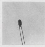
Measuring only 0.005 in. in diameter, the Micro-Bead thermistor is designed for measurement and control of temperature and of liquid or gas flow in any application where the mass of a larger element can not be tolerated. Response time is 0.12 sec in still air at 25°C. Dissipation constant is 0.04 mw/°C. Victory Engineering Corp., Springfield Ave., Springfield, N.J. [437]
