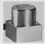
High level d-c output ( $\pm$ 1.5 v) linear accelerometer model 100 has an output accurately proportional to the sensed acceleration vector with ranges of  $\pm$ 1 g to  $\pm$ 259 g. Power input is 6 ffv d-c. The self-contained transducer measures 1 in. square by 1½ in. high, and weighs approximately 3 oz. Price is \$345. Setra Inc., 12 Huron Drive, Natick, Mass. 01760. [362]
