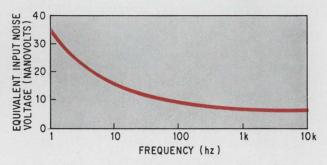
Flicker noise. Plotting the equivalent noise voltage at several frequencies reveals that the noise amplitude increases at low frequencies because of flicker noise.
