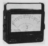
Battery-operated, 50,000 ohmsper-volt multitester measures resistance in four ranges up to 10 megohms. Meter has 5¼ in. face, spring-backed jewels and self-shielded movement. It's useable at frequencies up to 100 khz, has built-in overload protection. Price is \$19.95. Lafayette Radio Electronics Corp., 111 Jericho Turnpike, Syossett, N.Y. 11791 [425]
