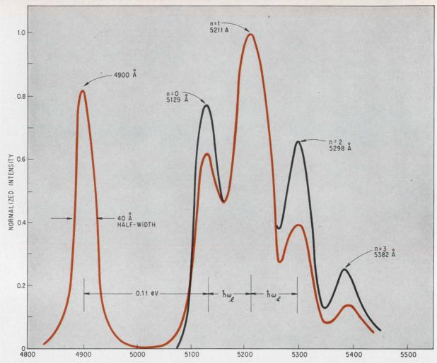
**Tap colors.** Spectra from mechanically-excited CdS tap crystal (color) and ultraviolet-excited crystal are similar. Most striking difference is the sharp peak at 4,900 angstroms in the mechanically-excited spectrum.
