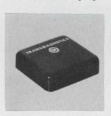
Solid sate device model 678 converts 3-wire synchro input to linear d-c voltage at high speed. It provides an output from -10 to +10 v linear to angles from 0° to 360°. It samples as many as 100 synchros 25 times per sec each in multiplexed systems. Unit costs \$1,125 (1-9), is available on a stock to 10 days basis. Transmagnetics Inc., Flushing, N.Y.[387]
