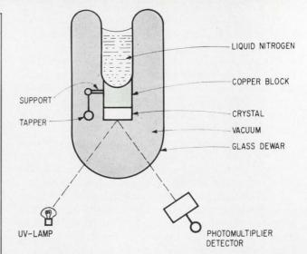
Storage device. This simple arrangement could form basis of memories, image intensifiers, or light meters.
