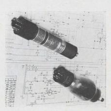
**Rookie and vet.** Solid state thyratron, top, is designed to duplicate mercury tube physically and electrically.
