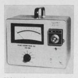
Lightweight vibration monitor model VM-10M can be used with any piezoelectric accelerometer with sensitivities from 1 mv/g to 100 mv/g. Features include high input impedance of 1,000 megohms, 6 full-scale acceleration ranges of 1, 3, 10, 30, 100 and 300 g, and a constant 10 mv/g output. Price is \$395. Agac-Derritron Inc., P.O. Box 358, Alexandria, Va. 22313. [365]
