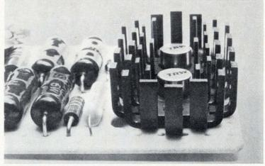
To cool off low-to-medium power transistors in TO-5 and TO-18 cases, use IERC's efficient LP's. Patented, staggered-finger design maximizes radiation and convection efficiency, radiates heat directly to ambient. Available in single or dual mounting for thermal mating of matched transistors.
