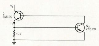
**Triggering.** Current  $I_1$  flows in the direction indicated after the reverse-biased base-emitter junction of  $Q_1$  breaks down.
