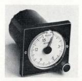
A plug-in industrial reset timer provides instant interchangeability for circuit testing and maintenance. Model 400 has time ranges from 6 sec to 96 hours, accuracy within 0.25%, and 2 load and 2 instantaneous switches. Applications include control of machine tools, induction heating equipment, and conveyor controls. Cramer Division, Conrac Corp., Old Saybrook, Conn. [342]
