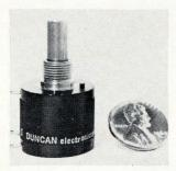
Ten-turn wirewound pot model 3253 PixiePot is  $7/8 \times 3/4$  in. and weighs  $1/2 \times 3/4$  oz. Resistance tolerance is  $\pm 5\%$  over 100 ohms to 100 kilohms. Linearity is  $\pm 0.25\%$  and resolution is typically 0.222. Units are rated at 2w at 25°C. Price is \$5.95 in lots of 1 to 24; less than \$4 in production quantities. Duncan Electronics Inc., 2865 Fairview Rd., Costa Mesa, Calif. [353]
