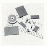
Ceramic chip capacitors are moisture resistant and contamination free in small rectangular, large rectangular, square, and monolithic disk feed-through configurations. Type K-1200 series, available in 51 models, ranges from 10 pf to 1.5  $\mu$ f. They operate from —55° to 125°C. D-c working voltages are 50, 100, and 200. Monolithic Dielectrics Inc., Box 647, Burbank, Calif. [3461]
