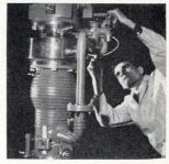
Vacuum pumping module 3352 pumps about 900 liters per sec. This allows more rapid production operations in vacuum metalizing, IC deposition, high temperature furnaces, and space simulation equipment. The module measures 35½ x 21½ x 27 in. It uses a 6-in. diffusion pump. Price is about \$2,000. National Research Corp., 160 Charlemont St., Newton, Mass. 02161. [424]
