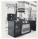
Designated the Plasma Vac AST1 300, a reactive sputtering system features 2 parallel-mounted water-cooled disk electrodes. The target electrode and discharge suppressor are in the upper position and the substrate-table electrode in the lower. An r-f supported plasma discharge is used to ionize the gas. Consolidated Vacuum Corp., 1775 Mt. Read Blvd., Rochester, N.Y. [428]
