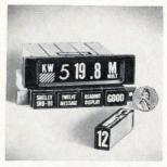
Ultraminiature rear projection readout SR-90 has 12-message capability. It reads out symbols, characters, or up to 4-line messages 0.1 in. high. Front dimensions are 0.650 x 0.460 in. Lamp replacement is accomplished from the front panel, by removing the readout from the housing assembly. Shelly Associates Inc., 111 Eucalyptus Dr., El Segundo, Calif. 90246. [344]
