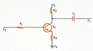
Force analogy. Contact points  $P_1$ ,  $P_2$ ,  $P_3$ , and  $P_4$  in this single-transistor circuit are fixed to components  $C_1$ ,  $R_1$ ,  $R_2$ , and  $R_3$ , shown in color, whose leads are assumed to be elastic. If the components are allowed to assume a position in which the net forces acting on each component are zero, the elements come to rest. The relative position of the components at this time becomes a possible board layout.
