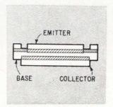
Utilizing the ADE (alloy diffused epitaxial) construction process, the MP2200A-2400A germanium transistors are suited for core driving, power conversion, and high-voltage switching where high power handling capability (80 to 120 v minimum at 8 amps) is needed. Prices range from \$2.25 to \$2.60. Motorola Semiconductor Products Inc., P.O. Box 995, Phoenix, Ariz. 85001. [442]
