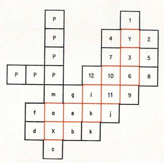
Step selection. With the X and Y squares representing the peaks between which a path is to be completed, the computer scans the area between them. Steps are chosen in the most downward direction from both X and Y. The squares surrounding the two peaks represent various lower altitudes. Steps can only be taken vertically or horizontally. They can neither be on or adjacent to steps of a different path nor retrace a previous step. The completed path is shown in color.
