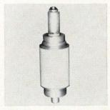
Variable capacitor CAQA-200 utilizes ceramic and copper materials with a vacuum dielectric. It handles 50 amps rms at 16 Mhz. Temperature rating is 120°C. Capacitance range is 10 to 200 pf. Over-all length is 3.75 in., diameter 1.31 in. The CAQA-200 makes possible the design of compact transmitter tank circuits. Jennings Division, ITT Corp., Box 1278, San Jose, Calif. [349]
