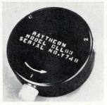
Coaxial L-band circulator model CLL-83 operates at 1.2 to 1.4 Ghz. It has a maximum vswr of 1.20, maximum insertion loss of 0.3 db, and minimum isolation of 20 db. The unit has a Y package configuration. It can also be supplied with 1 port terminated for isolator uses. The circulator is 3½ in. in diameter, 15½ in. thick. Raytheon Co., 130 Second Ave., Waltham, Mass. [407]
