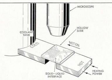
Experimental setup in which photographs such as that below were taken. The glass slide or cell—containing a liquid which freezes like a metal—is placed between hot and cold blocks of brass. This produces a temperature difference along the slide. A solid-liquid interface then forms between the two blocks. By moving the slide toward the cold block at a constant rate, one can observe the steady growth of the crystal under the microscope.
