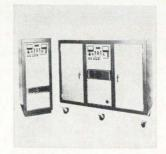
Laser power supplies for use with pulsed ruby and glass lasers range from 2.5 to 30 kw output. They are suited to high repetition operation in both the normal and Q-switched modes. All systems have solid state components including 20 amp, 7200 v piv singlephase, full-wave h-v rectifier. Prices from \$4,600. Spacerays Inc., Northwest Industrial Park, Burlington, Mass. [387]
