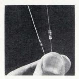
Mini-Mono, whiskerless glass diodes 1N5315 and 1N5316 are less than 36th of the standard subminiature D0-7 glass package. Minimum breakdown voltage at 10  $\mu$ a is 100 v. Forward voltage drop at 10 ma is 0.650 and 0.690 v minimum for the 5315 and 5316. Reverse current at 50 v is 50 na. Continental Device Corp., 12515 Chadron Ave., Hawthorne, Calif. 90250. [441]
