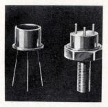
Silicon npn transistors A200/A201/A202 serve as class C r-f amplifiers. Power output is 1w, 7 w, and 12 w; gain is 10 db, 6 db, and 6 db, respectively. The inherently fail-safe units are intended for use in 12 v, battery-operated 175 Mhz mobile communication systems. Semiconductor and Receiving Tube Division, Amperex Electronic Corp., Slaters-ville, R.I. 02876. [4361]
