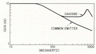
Resonant peak. Unlike the single common-emitter stage, whose frequency response is fairly flat, the cascode amplifier has a resonant peak. A variable capacitor,  $C_1$  controls peak position. When  $C_1$  is increased, the resonance is shifted to a lower frequency and a higher amplitude. This circuit has an 18-db gain and a 550-Mhz bandwidth.
