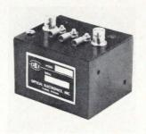
Analog peak sense and hold modules measure the amplitude of transients, obtain a peak noise voltage level, and measure the peak of a complex waveform. Operation up to 10 Mhz and accuracies as high as 0.01% full scale are provided by models 5138/5139 and 5146/5147. Prices are \$360 and \$400, respectively. Optical Electronics Inc., Box 11140, Tucson, Ariz. 85706. [375]
