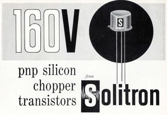
Solitron, now in full production of small signal transistors, has a complete line of PNP Silicon Choppers with voltage capabilities up to 160 Volts. Identified as the SSS 1001-4 Series, these devices are available in the TO-5 package. They offer high reliability, low saturation voltages and can be purchased as pairs with offset voltages matched to  $100 \,\mu\text{V}$  Ta=25°C. A few of their many circuit applications include modulators, servos, telemetry and multiplexing.
