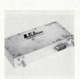
Logarithmic amplifier ITL-5, for microwave receivers, provides a log video output with a 70-db input dynamic range. Video output is proportional, within ±2 db, to the log of the input from —60 to +10 dbm. The unit is available at 30-or 60-Mhz center frequency, 4- or 8-Mhz bandwidth. It operates in a 50-ohm i-f system. Price is \$325. LEL Division, Varian Associates, Akron St., Copiague, N.Y. [405]
