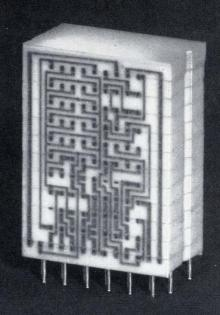
If you are working with a single chip or with complex circuit networks, Coors micro-ceramic modules offer you high reliability packaging. In the example above, the design engineer utilized base, frame, and lid modules to form a universal stacked package that can grow to fit any circuit density required. Each module is approximately 5/16" wide, 11/16" long and .050" high – indexed for high speed assembly. Because of the unique properties of Coors Ceramics, modules can be
