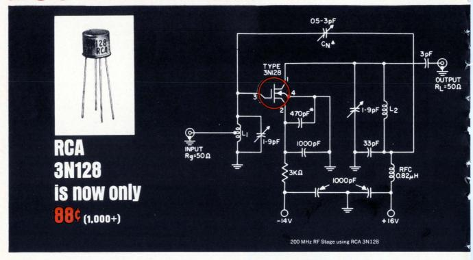
RCA's 3N128 N-channel, depletion-type MOS field-effect transistor actually offers dynamic range 10 times greater than conventional bipolar transistors. Because of the resulting improvement in cross modulation and spurious response, the 3N128 is recommended as an RF amplifier and a mixer to further improve performance in these areas. You can use standard vacuum-tube-type biasing and AGC requires virtually no power.
