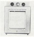
A dual-range Speedomax recorder measures molten-metal temperatures with the Temtip expandable immersion thermocouple, as well as carbon equivalent (or other analyses) with the Tectip thermalanalysis detector. This offers a savings for foundries and meltshops over the 2 recorders normally required. Leeds & Northrup Co., 4901 Stenton Ave., Philadelphia. L3641
