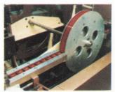
rects the circuits to any of 20 bins, according to the computer's priority programs. You get only circuits that are fully guaranteed at temperature extremes—not at just room temperature only.
