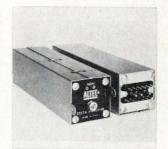
Amplifier model 2227A is a 15-pin device for voice frequency repeater systems. The low-frequency response may be adjusted for a flat characteristic or a roll-off at 200 hz. The unit has an input-output impedance of 600/1,200 ohms and operates on either 48 to 52 or 24 to 26 v d-c. Altec Lansing Division, LTV Ling Altec Inc., 1515 S. Manchester Ave., Anaheim, Calif. [383]
