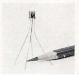
Silicon planar npn Darlington transistors 2N2723-4-5 are 2 transistor chips mounted in either a 3- or 4-lead TO-18 package. Characteristics include  $h_{\rm FE}$  within 10%,  $V_{\rm BE}$  matched within 30 mv, and temperature tracking within 100  $\mu$ v/°C. Applications are constant-current supplies and voltage comparators. Solitron Devices Inc., 1177 Blue Heron Blvd., Riviera Beach, Fla. [439]
