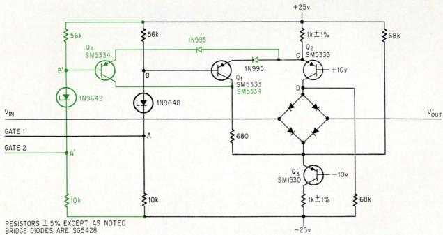
**Diamond gate.** A simple diode bridge transmits an analog voltage unchanged when an input gating signal is a binary 1. When the gating signal is 0, the output floats regardless of what the analog input is. The more complex diamond gate (with circuitry in color) used in the interpolator needs two digital gating signals to transmit the analog voltage.
