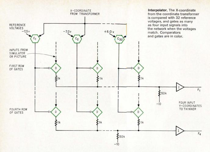
except the interpolator has a single digital control input. An AND circuit controls the bypass action in the other type, which gates the potentiometer voltages in the interpolator to shut off an unused input.
