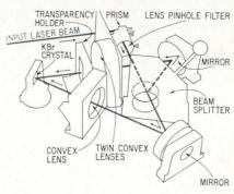
Crystal set. Diagram shows how light travels among prototype components set up in photo at left to record analog data such as photos or drawings. After exposure, a joy stick is used to lift the beam splitter out of optical path. and the crystal can be viewed from the rear. In this early model, the stepping motor for the KBR crystal holder is below the table.
