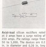
Axial-lead silicon rectifiers rated at 2 amps have a surge rating of 200 amps. Piv ratings range from 50 to 1,200. The devices are 0.2 in. in diameter and 0.38 in. long with a transfer molded, void-free body. They replace 1/16-in. stud units and eliminate heat sinks. Price of a typical unit—the MIBO (200v)—is 64 cents each. Electronic Devices Inc., 21 Gray Oaks Avenue, Yonkers, N.Y. [437]
