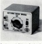
Amateur and Citizens Band radio operators can measure noise, resonant frequency, and operating impedance of whip antennas, dipoles, beams, and quads using an antenna noise bridge and a receiver that tunes the range of interest. Operating range is 0.5 to 150 MHz, from 0 to 100 ohms. Price is \$24.95. Omega-t Systems Inc. 516 W. Belt Line Rd., Richardson, Texas. [362]
