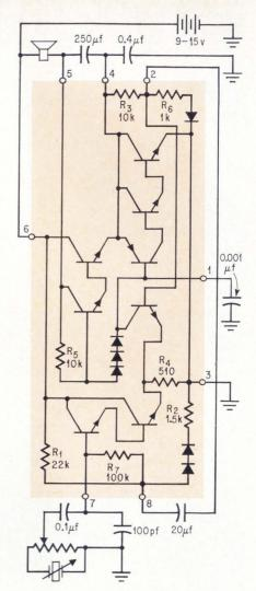
Push-pull. Output stage delivers more than a watt to speaker.
