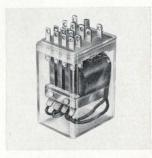
Magnetic latching relay type RR is offered in voltages ranging from 24 to 220 v a-c, and 12 to 110 v d-c. Standard design incorporates 4PDT contacts in fine silver, silver-cadmium oxide, gold nickel, silver palladium (60/40), and silver palladium (30/70). Mechanical life is 100 million operations. Schrack Electrical Sales Corp., 1140 Broadway, New York 10001. [356]
