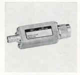
R-f voltage detector model 8029 has a vswr rating specified at less than 1.2:1, with typical values of 1.05:1. It is designed for c-w and swept applications, as well as general purpose usage, covering 10 khz to 3 Ghz. Square-law sensitivity is typically 0.3 mv/ $\mu$ w; flatness,  $\pm$ 0.5 db. Input impedance is 50 ohms. Price is \$95. Telonic Instruments Inc., 60 N. First Ave., Beech Grove, Ind. [408]
