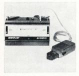
ServiVar is a battery-operated instrument that measures a-c voltage from 25 to 600 v at frequencies from 25 to 500 hz; a-c current, from 0.2 to 100 amps at 60 hz; and resistance, from 50 to 100,000 ohms. A snap-around probe allows readings in hard-to-reach locations. It accommodates wire up to 0.5 in. Bacharach Instrument Co., 200 N. Braddock Ave., Pittsburgh, Pa. [365]
