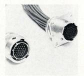
Circular connectors type ESM are bayonet locking, subminiature, and have a high contact density (0.080 in. center-to-center). They come in a 37-contact version in a No. 12 shell, and a 92-contact type in a No. 18 shell. Contacts are rated at 5 amps. They accept 22-, 24- or 26-gauge wire and are accessible from the rear of the connector. Elco Corp., Willow Grove, Pa. 19090. [348]
