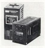
A universal dual-output power supply named Unitwin-164 meets MIL-E-5272 and related specs. It provides 2 voltage outputs adjustable between 0 and 25 v at 0.750-amp capacity for each section. Regulation is better than ±0.005% or 1 mv for line and load. Output impedance is 0.0032 ohm or less to 1 khz. Power/Mate Corp., 163 Clay St., Hackensack, N.J. 07601. [381]
