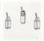
Rfi-shielded toggle switches attenuate conduction and radiation in the 0.14-to 200-Mhz range. They are suitable for radiation-free airborne electronic equipment conforming to MIL-I-26600. Series TR2100, 2150, and 3100 have an operating torque of 20 in.-oz max. Prices start at \$7.56. Control Switch Division, Controls Co. of America, 1420 Delmar Dr., Folcroft, Pa. [343]
