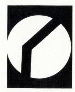
Sharp lines. Blown-up drawing of two typical line widths. Vertical line at left is generated by the y motion of the table. Diagonal line is achieved with successive x and y motions because the table can only move along one axis at a time.
