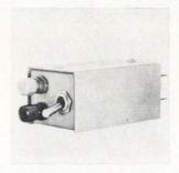
A plug-in thermocouple reference junction converts millivolt recorders to thermocouple recorders. The JR393 measures any temperature with any thermocouple. Over the 55° to 90°F range, its accuracy is  $\pm 1/2$ °F. Temperature range is -15° to +200°F. Consolidated Ohmic Devices Division, Consolidated Airborne Systems Inc., 115 Old Country Rd., Carle Place, N.Y. [371]
