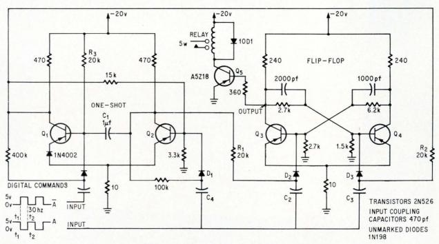
Operating sequence. Leading edge of  $\overrightarrow{A}$  at  $t_1$  triggers the one shot to start the timing. If the command pulse is short,  $Q_5$  turns on and fires the relay.
