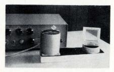
Playing the angles. Crystal at right is rotated by stepping motor whose controller is at the rear. Six arc minutes of rotation change incidence angle of laser beam enough to separate holograms.
