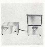
Ultrasonic cleaners for p-c boards and components come in tank capacities of ½ and 1 gallon. Each cleaner consists of the tank (detachable for cleaning); the transducer assembly, which induces cavitation in the tank; and the generator, which powers the transducer. The tank is for use with water-base detergents. Blackstone Ultrasonics Inc., 25 Barrett St., Sheffield, Pa. [425]
