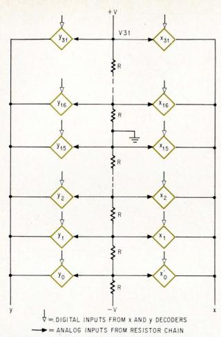
**Digital-to-analog converter.** Diamond gates (color) convert each of the x and y input coordinates from the digital decoder into an analog voltage.
