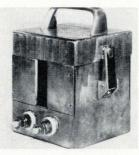
An injection-current probe can be clamped around d-c, 60 hz or 400 hz power lines carrying up to 300 amps, without altering their transfer characteristics. Designated GIP7418, it is also capable of injecting 1 amp from 100 hz to 100 khz into a circuit using an audio amplifier as the source. Genistron Division, Genisco Technology Corp., 18435 Susana Rd., Compton, Calif. [366]
