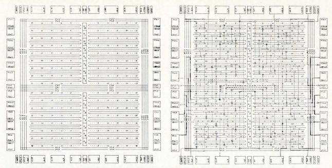
Mask layout. Both placement and wiring are layed out at left to indicate a final circuit scheme. Horizontal rows of dots indicate the vertical wiring positions; three solid lines between these rows indicate dual NOR circuits. By adding metal and diffused lines, the designer defines his final layout. Rectangles represent inputs to the circuit.
