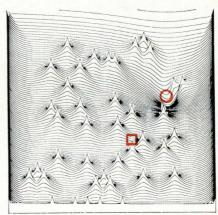
Sidestepping. Path shown in color indicates the connection between the two peaks. Sidestepping is caused by obstacles along the way. At right, target peak is again pulled down at a later stage of the process and the terrain examined for other connecting paths. Heavy black vertical lines and horizontal plateaus indicate several paths already completed.
