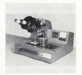
Ultrasonic die bonder DU-6 attaches dice to devices ranging from large stud packages to small headers or flatpacks. Ultrasonic energy is supplied by a 10-watt 40-khz generator. The dice are picked up by vacuum and a slide with the heater column holding the work is moved rapidly into place for bonding. Axion Corp., 6 Commerce Park, Danbury, Conn. [4221]
