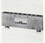
Coaxial bandpass filter model BK-51FN, covering 2.2 to 2.3 Ghz, is useful in telemetry receivers and down-converters. It offers high rejection-band characteristics—50 db at 2.04 and 2.46 Ghz—with 80 db image rejection. Insertion loss is 0.5 db, and vswr is 1.5 max. Price is \$275. The unit is available from stock. Microlab/FXR, 10 Microlab Rd., Livingston, N.J. 07039. [406]
