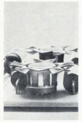
Fan-top dissipators for TO-5 and TO-18 cases drop temperatures dramatically; cost just pennies. T-shape adds almost nothing to board height; allows components to snuggle close to transistors. Spring fingers provide fast, press-on installation.
