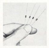
Subminiature ceramic tubular capacitors series CT07 are rated at 50 v d-c over a temperature range of -55° to +125° C. Capacitance values are from 10 to 10,000 pf in tolerances of +10% and +20%. The capacitors exceed the requirements of MIL-C-11015. They measure 0.165 x 0.095 in. Gulton Industries Inc., 212 Durham Ave., Metuchen, N.J. [341]
