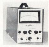
Portable strain gauge and transducer indicator model 1-115SI is an input conditioning module with integral power supply, amplifier, and meter readout. It accepts inputs from 1, 2, and 4 active arm bridges using input wiring up to 8 wires, plus shield. Accuracy is ±0.5% full scale in 4 ranges to 20 mv. Price is \$475. B&F Instruments Inc., Cornwells Heights, Pa. 19020. [372]
