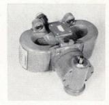
Tunable coaxial magnetron SFD-325, for airborne and ground-based radar systems, has a frequency range of 16 to 17 Ghz, and peak output power of 75 kw. Compatibility of the tube with modulators delivering widely varied pulse shapes is assured by the low pushing factor (60 khz/amp). Duty factor is 0.001. S-F-D Laboratories Inc., 800 Rahway Ave., Union, N.J. [403]
