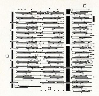
**Generated artwork.** Interconnection pattern for 122-element logic chip is generated 10 times oversize. Typical line width is 0.4 mil.
