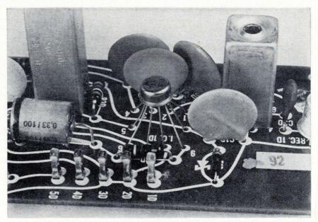
Replacement part. Audio IC in Motorola color-tv set replaced 15 discrete components; chip incorporates 15 resistors, 12 transistors, and 12 diodes.
