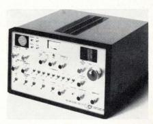
**Display.** Oscilloscope is provided to facilitate tuning.
