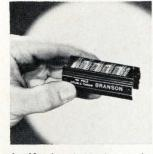
A 40-pole, double-throw relay package has 2-amp, 28 v d-c resistive contacts. The SR package eases replacement of individual switching units, eliminating the need to replace the complete unit. The sealed relays operate in a —65° to +125°C range, withstand 50 g shock for 11 msec, 20 y vibration from 10 to 2,000 hz. Branson Corp., Vanderhoof Ave., Denville, N.J. [350]
