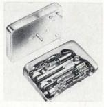
Tuning-fork oscillator LCG-2 is offered in discrete frequencies from 400 to 8,000 hz. Accuracy is 0.050% at 25°C. Output voltage at nominal d-c input is 6 v peak-to-peak 50% clipped sinewave into 6,000 ohms through an external d-c blocking capacitor. D-c input voltage is 12 v at 3,33 ma. Price is under \$32. Philamon Laboratories Inc., 90 Hopper St., Westbury, N.Y. 11590. [385]
