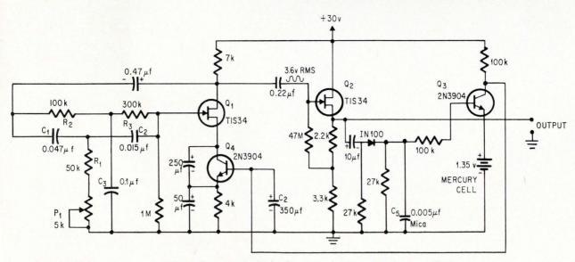
Stabilized oscillator. Output of FET oscillator  $Q_1$  feeds buffer stage  $Q_2$ . Signal is then rectified.
