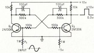
Adjustable hysteresis. Input signals, which exceed the threshold level set by potentiometer  $P_1$ , turn  $Q_1$  on and  $Q_2$  off, generating an output step.
