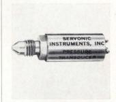
The Miniduser measures 0.5 x 1 in. and is available in pressure ranges from 0-500 to 0-10,000 psia and psig. Used primarily for airborne telemetry and control, it monitors air, fuel, and other media compatible with its NiSpanC sensing element. Over-all accuracy is ±1.75%. Servonic Instruments, subsidiary of Gulton Industries Inc., 1644 Whittier Ave., Costa Mesa, Calif. [376]
