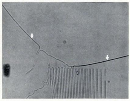
Bell Laboratories' model (200x) permits physical simulation of a <u>eutectic phase diagram</u> for an alloy such as lead-tin. Diagram relates liquid proportions (horizontal scale) to temperature (vertical).
