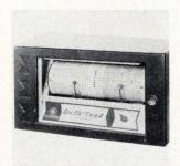
Data-Trak 5110-2P is an electrostatic curve follower with 2 curvesensing probes which track the individual x and y coordinate data plotted on a Mylar chart. A precision pot is servocoupled to each probe to translate graphical data to equivalent electrical outputs. The unit is suited to any process requiring 2 synchronized and programed signals. Research Inc., Box 6164, Minneapolis. [369]
