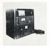
Magnetic stabilizer model MS-10 fully charges and stabilizes metallic alloy magnets up to 1/4 lb with a stabilization accuracy within 2%. It is capable of up to 1,000 charging cycles per hour. It is available in 115-v or 230-v models with single pushbutton or foot pedal operation. Instrumentation Division, Thomas & Skinner Inc., 1120 E. 23d St., Indianapolis, 46207. [361]
