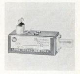
Fundamental voltage-tuned oscillator model ETS3152 has a tuning range of 1.2 to 1.8 Ghz. Linearity is within ±1% over 75% of the range. The devices, 1 x 1 x 2¼ in. provide a power output of 50 mw c-w. Noise is —70db, and harmonics approximately —15 db, Microwave Products Division, Consolidated Airborne Systems Inc., 115 Old Country Rd., Carle Place, N.Y. L4041
