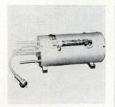
Class C pulse-cavity oscillator 11005 is a 2.5-kw unit that is tuned manually and covers 410 to 460 Mhz. Applications include drone control circuitry and a h-f test source. The unit is rated at 35% efficiency and has a duty cycle of 0.00015. Maximum input vswr is 2:1. Dimensions are 119/16 x 31/2 in. Microwave Cavity Laboratories Inc., 10 N. Beach Ave., LaGrange, III. **E4021**
