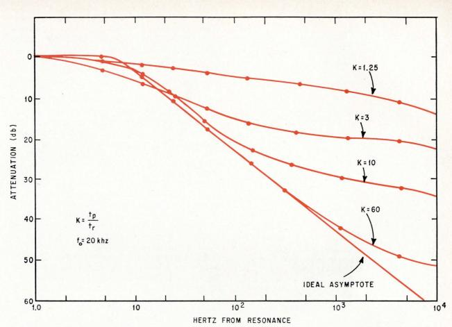
**Varying k.** As the ratio of pulse time to rise time increases, the shape of the frequency-response curve changes. Plots are obtained for a digital filter centered at 20 kilohertz.
