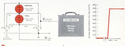
The Bissett-Berman E-CELL<sup>®</sup> is a unique "liquid state" electrochemical timing and integrating component now being manufactured in high volume on fully automatic production lines. E-CELLs are designed for single use or re-cycling, can be set or re-set in the field, and are furnished in wirelead or plug-in versions. A multiple electrode E-CELL enables complex functions such as two-phase timing – or subtotaling and totaling – with
