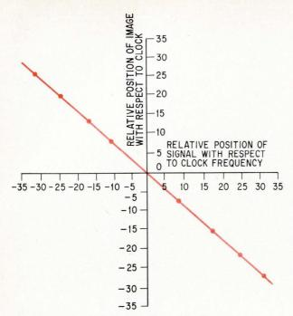
**Image response.** Relative location of the image frequency is plotted with respect to the clock frequency to enable the designer to locate a third-order image response.
