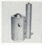
Pulse-amplifier cavity model 11026 can be used in phasedarray and broadband-radar systems. It is rated at 10-kw output and operates in L band. Basic frequency is 425 Mhz and it is tuned manually. Bandwidth is 50 Mhz at 1.0-db points. Power input is 2.5 kw peak; maximum input vswr, 1.5:1. Microwave Cavity Laboratories Inc., 10 North Beach Ave., LaGrange, III. [414]
