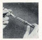
**Precision** connectors assure rated voltage standoff in mated or unmated condition. Recessed center contacts and precontact grounding are for safe handling. Maximum leakage across the interface is less than 1  $\mu$ a at 20 kv d-c and sea level pressures. The rated voltage is for limited pulse use. Reynolds Industries Inc., 2105 Colorado Ave., Santa Monica, Calif. [**341**]
