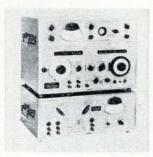
Twenty-seven controls and a crt provide versatility and ease of balance on the 2702 inductance bridge. The unit has a range from  $0.3 \ \mu$ h to 21,000 henrys, with internal frequencies of 10 khz, 1 khz, and 60 hz. The crt display indicates direction of inductor balance and reports at test frequency. Marconi Instruments, 111 Cedar Lane, Englewood, N.J. [365]
