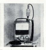
Charge detector CM467 measures electrostatic fields. Two interchangeable sensor probes are available. One measures charges in the  $10^{-9}$  coulomb range by direct contact. The other measures charges as low as  $10^{-12}$  coulombs, and is used for remote monitoring. Price of the Coulometer, with either probe is \$195. Metronics Associates Inc., 3201 Porter Drive, Palo Alto, Calif. [373]
