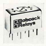
Half-size crystal can relays incorporate a magnetic circuit that locates the armature inside the coil, reducing leakage and coil power requirements for switching. Units, designated BR17 and BR16 for latching and nonlatching versions, require only 175 mw pull-in power to switch any load from dry circuit to 2 amps. Babcock Electroncost a Mesa, Calif. [347]
