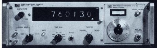
Model 5246L Counter with new 5254B Frequency Converter
