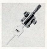
Model 410-A09 automatic frequency control and monitor cavity has a stability of  $\pm 1$  Mhz from  $-30^{\circ}$  to 75° C. It can be used to stabilize klystrons in discriminator circuits. The cavity offers a tuning resolution of  $\pm 0.5$  Mhz from 5.9 to 7.4 Ghz. A locking device protects the frequency setting against accidental change. Microlab/FXR, 10 Microlab Rd., Livingston, N.J. [416]
