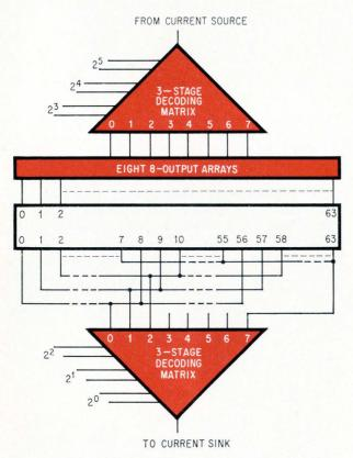
**Double-ended decoder.** Two 3-stage matrixes and eight 8output arrays can provide complete memory address decoding and driving cheaply. All the stages shown in color would be glass-switch arrays.
