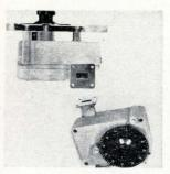
Eight compact, direct-reading attenuators span 7.05 to 90 Ghz. Attenuation range of each unit is 0 to 50 db. Vswr of 1.15, accuracies to  $\pm$ 0.5 db, and maximum insertion losses of 0.5 db are attained. The units, all panelmountable, range in price from \$350 to \$700. DeMornay-Bonardi division, Datapulse Inc., 1313 N. Lincoln Ave., Pasadena, Calif. 91103. [405]
