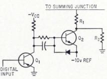
Sums current. A single current-summing stage consists of amplifying transistor  $Q_1$  driving switch  $Q_2$ . Resistor  $R_2$ shunts  $Q_3$ 's leakage current and is a low-impedance path for the discharge of stray capacitance.  $R_1$  is a precision resistor.
