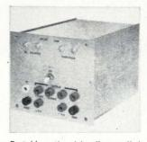
Portable active delay lines, called Delay Long, have applications in low-frequency signal-processing fields. Model APD 120 provides a delay of 120 msec. Delay to rise time ratio is 5:1. Input impedance is 1 megohm; output impedance, 4,000 ohms; maximum signal level,  $\pm 4$  v. Size is 45% x 51/4 x 65% in; price, \$650. A.P. Circuit Corp., 865 West End Ave., New York, [391]
