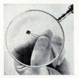
**Ceramic-encapsulated** platinum temperature transducer 5001-19 is designed for surface measurement over a range of  $-260^{\circ}$  to  $+400^{\circ}$ C. Resistance at  $32^{\circ}$ C is 500 ohms  $\pm 1^{\circ}$ , and resistancevs.-temperature relationship is linear over the entire temperature range. Time constant is 250 msec; repeatability,  $\pm 0.1^{\circ}$ C. Thermal Systems Inc., 13920 S. Broadway, Gardena, Calif. **[370]**
