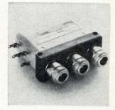
Coaxial latching switches of the MA-7524 series are for channel selection in military and commercial communications and radar equipment where space is limited. They feature 60-db interposition isolation from d-c to 12.4 Ghz and vswr of 1.5. Maximum insertion loss at 11 Ghz is 0.5 db. Maximum switching time is 0.015 sec. Microwave Associates Inc., Burlington, Mass. [412]
