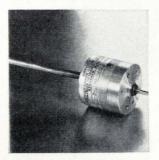
Model 15 shaft-angle encoder uses low-voltage light sources and wideaperture optics. Standard units can be supplied with resolutions up to 6,000 counts per shaft revolution. Starting torque is 0.02 oz-in. Voltage levels are 200 mv peak-to-peak minimum into a 2,000-ohm load. Options include an internal amplifier shaper. Dynamics Research Corp., 38 Montvale Ave., Stoneham, Mass. [390]
