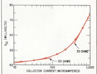
**Voltage-current plot.** Saturation resistance of the transistor varies from 30 to 50 ohms as the collector-to-emitter voltage is increased from 40 to 70 millivolts. The collector current through the transistor is in the microampere range.
