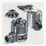
Suited for the chemical and aerospace fields where high pressures are to be monitored, series 250 transducers are available in 6 ranges from 0 to 5,000 to 0 to 20,000 psig. Housing and pressure cavity are of stainless steel and electrical components are sealed from the pressure media by stainless steel diaphragms. Taber Instruments, 455 Bryant St., North Tonawanda, N.Y. [361]
