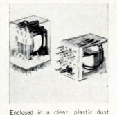
cover, a 1.281 x 1.109 x 0.859in., 4-pole relay is available in a-c and d-c versions. Model KHU has gold-plated silver contacts rated 3 amps 120 v a-c, 3 amps 28 v d-c, and ¼<sub>0</sub> hp 120 v a-c. Coil ratings are to 120 v 60 hz, and to 120 v d-c. The relays have computer and switching applications. American Machine & Foundry Co., Princeton, Ind. [243]
