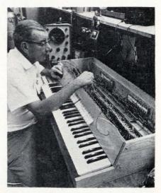
**On the inside.** Motorola engineers built this organ with a 5-octave, 61-note keyboard, and 18 function and voicing stops, to demonstrate what its new MOS IC's could do.
