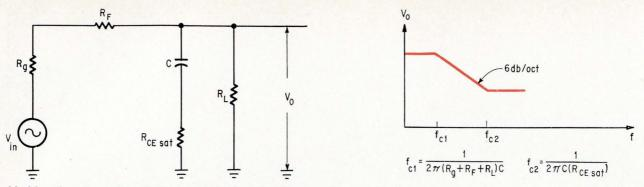
**Limiting the attenuation.** By including the transistor's saturation resistance into the equivalent circuit of the digital filter, the designer obtains an additional break point in the filter's response curve. Thus, he is able to limit the maximum attenuation.
