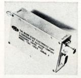
An L-band transistor amplifier is stable in an airborne rocket environment under all conditions of vswr and phase at the input and output. It has a gain of 17 db, 3-db bandwidht of 40 Mhz, and dynamic range of 60 db. With a center frequency of 1 Ghz, it includes a 10-db image reject filter at 1,120 Mhz. Micro State Electronics Corp., 152 Floral Ave., Murray Hill, N.J. [409]
