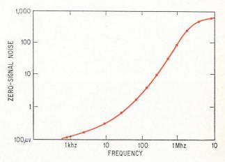
Shifting center frequency. As  $f_{\circ}$  increases, the zero-signal noise increases rapidly.
