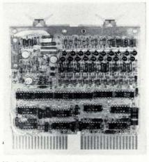
Machine built. Entire A/D converter is built on a double-sided board, using plated-through holes. Most components are inserted by machine.
