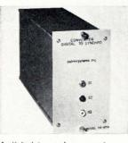
A digital-to-synchro converter accepts a parallel 10-bit binary angle and delivers a synchro signal equal to the digital input. Inputs of the DS800 are compatible with IC logic levels at updating speeds to 10,000 words/sec. Accuracy, no load to full load, is better than 0.5°. The unit's front panel is  $5½ \times 3½ \times 8$  in. Astrosystems Inc., 6 Nevada Dr., New Hyde Park, N.Y. [393]
