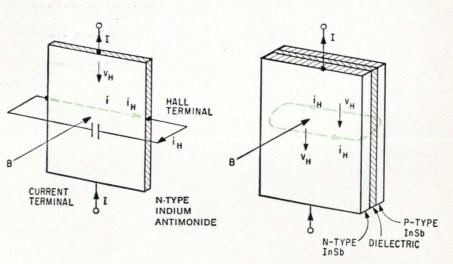
**Inductive slab.** Basic solid-state inductor (left) consists of InSb slab with external capacitor connected to two of its four terminals. Dielectric sandwiched between two slabs gives device internal capacitor.
