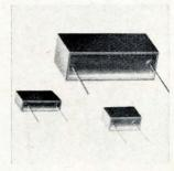
Epoxy-encased metalized mylar capacitors in a molded thin-rectangular configuration with radial leads are designed for high-density circuits. Series 17N is available in 100-, 200-, 400-, and 600-v sizes in capacitance values from 0.001 to 5  $\mu$ f with 20% to 1% tolerances. Operating temperature is from -55° to +125° C. SEI Mfg. Co., 18800 Parthenia St., Northridge, Calif. 91324. [348]
