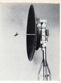
... Receiver dish. Receiver converter is also mounted right behind dish.
