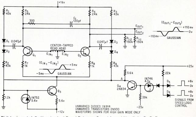
**Digital gain control.** Positive signals at  $D_5$  and  $D_6$  turn on  $Q_4$ , and forward bias diodes  $D_1$ ,  $D_2$ ,  $D_3$ , and  $D_4$  so that resistors  $R_1$ ,  $R_2$ ,  $R_3$ , and  $R_4$  load the amplifier and reduce its gain.
