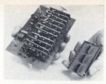
Simplicity in IC's. Subsystem (right) built with MOS IC's, which are packaged in plastic, takes only one-tenth the space of an equivalent unit (left) built with discrete devices.
