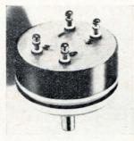
Custom-engineered pots made of conductive plastic, have 0.5% absolute linearity in the centers of their operational range, tapering to 0.15% in their end regions. Model 14C-1 offers a resistance of 100 to 20,000 ohms  $\pm 10\%$ ; power capability, 1.3 w at 25° C; torque, 0.2 oz maximum; minimum life, 5 million cycles. Gamewell division, E. W. Bliss Co., 1238 Chestnut St., Newton, Mass. [346]
