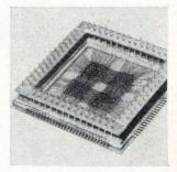
**Core memory** storage planes called Platrices can be used in memory systems for digital instrumentation and control equipment. A stack of Platrices is mounted on a p-c board through connection pins at the bottom of the stack. Units are available in 8 standard configurations with bit capacities ranging from 256 to 1,024. Ferroxcube Corp., Saugerties, N.Y. 12477. [352]
