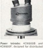
4CW800F, designed for distributed amplifier applications, feature 4 individual circuit connectors to the active part of the grid. Filament voltage ratings are 6 v and 26.5 v, respectively. Units are capable of 1,000-w output. Minimum selfresonant frequency is over 900 Mhz. Eimac division, Varian Associates, 301 Industrial Way, San Carlos, Calif. [403]
