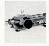
Precision 7-mm coaxial slotted line type 2852-05 is equipped with an APC-7 connector. It uses compensated dielectric pins in stead of a conventional bead to support the inner conductor. Rated residual swr is under 1.025 up to 18 Ghz. Over-all dimensions are 2.7 x 3.6 x 10.6 in. Weight is 2.7 lbs. Price is \$1,140. Alford Manufacturing Co., 120 Cross St., Winchester, Mass. [415]
