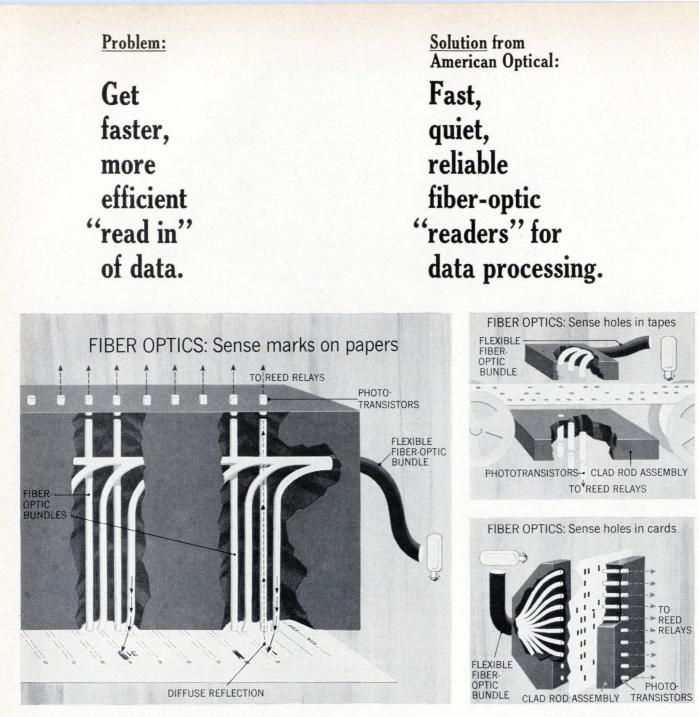
Electro-optical systems incorporating fiber optics are operating at up to four times the speed of electromechanical systems. When a combination of fiber optics, phototransistors, and reed relays is used, reading of basic data is not controlled by mechanical limitations. The use of fiber optics allows wide design freedom to increase system operating speed.
