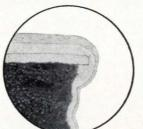
(a) Typical section of an electroplated hole, showing heavy buildup of metal plating at the orifice.
