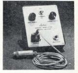
Compatible with most data recording systems, model SC1100 solid state bridge amplifier features a voltage output of 10 v full scale. Its 5-ma output current can drive most galvanometers directly without additional amplification. Continuously adjustable linear gain is  $\pm 0.5\%$  from 0 to 10 v. Price is \$95. Statham Instruments Inc., 12401 W. Olympic Blvd., Los Angeles. [392]
