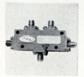
Solid state switch S001350, single pole, double throw, has a switching speed of 100 nsec. Its guaranteed high isolation value is 50 db to 2 Ghz, 46 db to 4 Ghz and low insertion loss of a maximum of 2 db to 2 Ghz, 2.8 db to 4 Ghz. R-f handling capacity is 2 w c-w. The switch weighs under 2 oz. Price is \$375 each. American Electronic Laboratories Inc., Colmar, Pa. [413]
