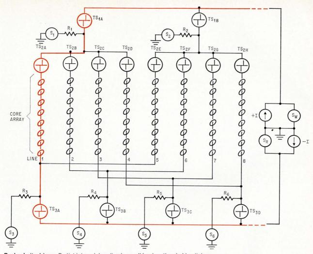
**Dual-polarity drivers.** Partial internal decoding is possible when threshold switches are applied as dual-polarity drivers. External decoding is still required for switches at bottom. One complete loop for a half-select current is shown in color.
