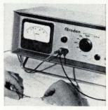
Ohmmeters for production lines have easy-to-read linear meters. Operational amplifier circuitry allows full-scale accuracy of 0.5%. Current through the item under test is 3 ma max on the 0-to-1ohm scale. Model 40 has resistance scales of 0 to 1, 0 to 10, 0 to 100, 0 to 1,000, 0 to 10,000, and 0 to 100,000 ohms. Price is \$245. Faradan Corp., 4130 Mennes Ave., Riverside, Calif. [376]
