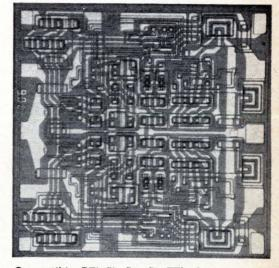
Compatible. DTL flip-flop fits TTL pins.
