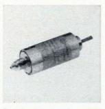
Potentiometric transducer 2101 operates in the ranges of 0 to 350 through 0 to 20,000 psi. It has an over-all accuracy of  $\pm 1\%$ at vibrations of 50 g. Normally used for control and telemetry, the unit will measure and monitor air, fuel, lubricants, and hydraulic fluids. It weighs 2 oz. and measures 0.75 x 1.5 in. Servonic Instruments Inc., 1644 Whittier Ave., Costa Mesa, Calif. [366]
