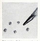
Hot-carrier diodes are packaged to permit use in circuits operating at frequencies up to 12.4 Ghz. Model 2701 has a single sideband noise figure of less than 6 db with a carrier frequency of 9.375 Ghz (local oscillator power, 1 mw). Model 2702 has a noise figure of 6.5 db; and model 2703, 7 db. Hewlett-Packard Co., 1501 Page Mill Rd., Palo Alto, Calif. [440]
