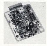
Video amplifier VA1367 is a d-c coupled, 10 Mhz, solid state plugin unit featuring a gamma-corrected transfer function to produce a linear relationship between crt light output and input-video drive. It employs feedback and temperature compensation to provide optimum gain stability and temperature independence. Beta Instrument Corp., 377 Elliot St., Newton Upper Falls, Mass. [383]
