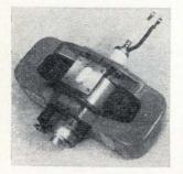
Mechanically tuned, coaxial magnetron model 304 is for use in airborne and ground-based radar systems. It develops 250 kw peak power across the 8.5- to 9.6-Ghz range. The 19-lb, air-cooled tube can be used in existing systems using the 6249 family of tubes. Dimensions are  $93/4 \times 101/4 \times 41/2$  in. SFD Laboratories Inc., 800 Rahway Ave., Union, N.J. [401]
