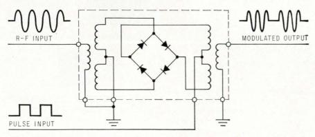
Power saver. Bridge of hot carrier diodes needs no power supply.
