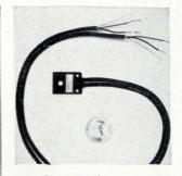
Hall-effect transducers measure steady-state, pulse, or transient currents without connection to the conductor under test. The CT-7W offers a rise time less than 1  $\mu$ sec, dynamic range of less than 1 ma to 30 amps peak, and frequency response flat to over 1 Mhz. It measures 1<sup>3</sup>/<sub>4</sub> x <sup>3</sup>/<sub>8</sub> in. with a <sup>3</sup>/<sub>16</sub>-in.-diameter opening. Ohio Semitronics Inc., 1205 Chesapeake Ave., Columbus, Ohio. [363]
