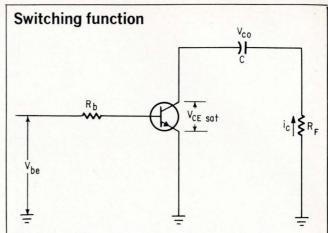
**Circuit operation.** An a-c switch requires current flow in both directions to charge and discharge the capacitor properly. When both the collectorand emitter-base diodes are switched from reversebias potentials to their forward-bias values the transistor is turned on. To turn the transistor off, the charged stored in the base is removed and both the collector and emitter are reverse biased.
