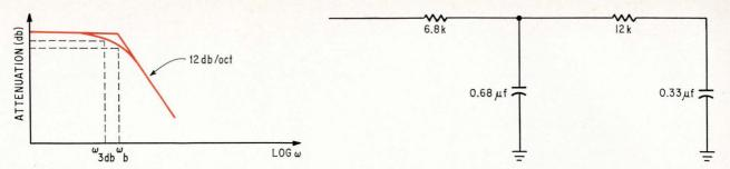
Altering the response. By changing the number of RC sections in a series-switched digital filter the engineer controls the shape of the frequency response. For a two-section filter the falloff is 12 decibels per octave.
