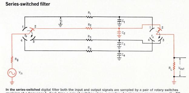
revolving at a frequency  $f_0$ . Each time a pair of switches close, a quarter of a sine wave appears across the RC filter arm of the circuit. The output is the voltage developed across the grounded capacitor,  $C_2$ .
