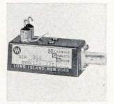
Voltage-tunable over half an octave, the ETS3152 is a 1.2- to 1.8-Ghz fundamental oscillator that offers greater than 50 mw of output power. Control voltage is 0 to 20 v. The unit measures 1 x  $1\frac{1}{5}$  x  $2\frac{1}{4}$  in. It will meet its specifications in  $-50^{\circ}$  to  $+70^{\circ}$ C environments. Delivery takes about 45 days. Consolidated Airborne Systems Inc., 115 Old Country Rd., Carle Place, N.Y. [404]
