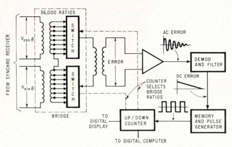
**Imbalance at work.** Error voltage caused by bridge imbalance drives pulse generator. Output pulses feed an up-down counter to advance digital display.
