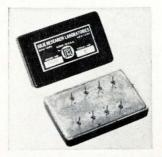
Precision resistor networks designed for plug-in to p-c boards cover a range from 10 ohms to 1 megohm. The line is available in accuracies from 0.0005% to 0.1% absolute and  $\pm 0.0002\%$  to  $\pm 0.1\%$  ratio. Stability is  $\pm 0.0015\%$  per year absolute and  $\pm 0.0002\%$  ratio. Price varies from \$20 to \$200. Julie Research Laboratories Inc., 211 W. 61st St., New York. [389]
