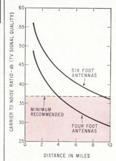
Minimums. Relay can operate at distances above the red area.
