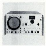
A spectrum analyzer designed for the community-antenna tv industry covers a range of 1 to 300 Mhz. A sensitivity of -90 dbm, flat responses, high stability, and spurious-free displays characterize its design. The Mark I analyzer has a 60-db display dynamic range and a 46-db distortion dynamic range. Price is \$1,500. Nelson-Ross Electronics Inc., 5-05 Burns Ave., Hicksville, N.Y. [368]
