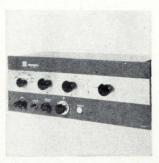
Panel-mounted potentiometers feature central readout window and an 11-position switch for selecting inputs. Two models are 3-dial instruments with a limitof-error of  $\pm 0.03\%$  of reading. Others have one decade switch plus a 27.5-in. calibrated slidewire scale with a limit-of-error of either  $\pm 0.1\%$  or  $\pm 0.2\%$ . Leeds & Northrup Co., 4901 Stenton Ave., Philadelphia. [369]
