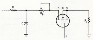
**Reducing noise.** For the FET, a balance network incorporating a potentiometer reduces the zero-signal voltage to below 50 microvolts.
