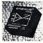
FET input operational amplifier QFT-5 provides  $10^{10}$  ohms differential and common mode impedances, less than 1 nanoamp of input offset current, 6 db/octave roll-off and high tolerance to capacitive loads. Output voltage is  $\pm 11 v$  at  $\pm 5.5 ma$ . Frequency (full output) is 50 khz. Price (1 to 9) is \$29 each. Nexus Research Laboratory Inc., 480 Neponset St., Canton, Mass. [395]
