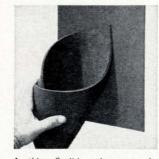
A thin, flexible microwave absorber based on silicone rubber, Eccosorb FGM has an average reflectivity of 12 db down from 2 to 12 Ghz over a wide range of incidence angles. It is usable up to 425°F continuously, and up to 500°F for short times. It weighs less than 2 lbs per sq ft. Price is in the \$50 per sq ft range. Emerson & Cuming Inc., Canton, Mass. **[407]**
