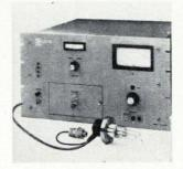
The Helmer gauge measures pressures obtained by vacuum equipment accurately down to  $1 \times 10^{-10}$  torr because the ion collector is optically shielded from the main source of X-ray current with no sacrifice in gauge sensitivity. Pressure is displayed on a single meter with a one-cycle logarithmic scale. Vacuum division, Varian Associates, 611 Hansen Way, Palo Alto, Calif. [371]
