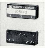
Double-balanced mixer 10514B, measuring  $1.63 \times 0.70 \times 0.43$  in., mounts on p-c boards. Range is 0.2 to 500 Mhz at I-o and signal ports; third port is d-c coupled. Conversion loss is less than 9 db over full range. Uses include pulse modulators, and current-controlled attenuators. Price is \$150. Delivery is from stock. Hewlett-Packard Co., 1501 Page Mill Rd., Palo Alto, Calif. [408]
