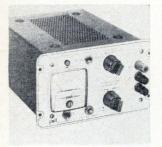
Regulated supply model 630 is suited for applications involving digital or linear IC's. It provides a continuously adjustable output voltage from 0 to 6 v at a maximum current of 3 amps. Dual concentric coarse and fine voltage controls enable voltage adjustment resolution of better than 1 mv. Power Designs Inc., 1700 Shames Dr., Westbury, N.Y. [385]
