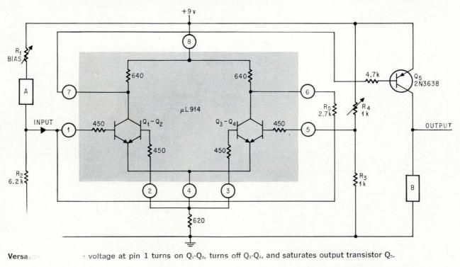
tor at A and a relay at B. If, however, A is a phototransistor and B a load resistor, the circuit becomes a light-sensing preamplifier with a digital readout.
