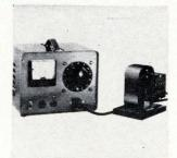
Portable a-c field demagnetizers are designed and built to user's specifications. The laminated core structure permits continuous-duty operation without heating. Peak field strengths are from 0 to 10,000 oersteds, infinitely adjustable. Units are available for 115-v or 230-v operation. Instrumentation division, Thomas & Skinner Inc., 1120 E. 23rd St., Indianapolis 46207. [384]
