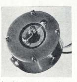
A solid state pulser provides up to 250 amps for driving laser diodes at room temperature. It uses avalanche-transistor techniques to produce 70-nsec pulses with 7- to 10-nsec rise times. Pulse repetition is adjustable from 300 hz to 10 khz. Volume of a 150-amp unit with a 10-khz driving oscillator is 1 cu. in. Austron Inc., 10214 N. Interregional Highway, Austin, Texas. [394]
