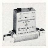
Two 50-ohm feed units provide a means of separating the d-c bias circuit from the r-f measuring circuit. Maximum bias current is 2.5 amps with voltage across the capacitor limited to 150 v d-c. The BN35616/6N/50 spans 30 to 100 Mhz, with vswr of 1.04:1; the 7N, 300 to 3,000 Mhz, with vswr of 1.06:1 at 3 Ghz. Rohde & Schwarz Sales Co., 111 Lexington Ave., Passaic, N.J. [402]
