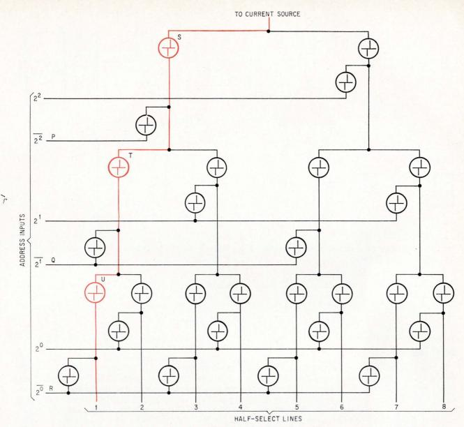
Alternative design. Binary decoder that doesn't require external resistors is made with doubled number of threshold switches, still in single monolithic array. Again, the first half-select line is picked by the switch routing shown in color.
