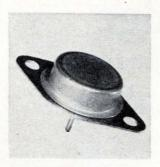
Six pnp silicon transistors are available at 200, 300, and 400 VCER, with either 1- or 2-amp beta ratings. The 200-v units have a 200 VCEO(sus), the 300-v units have a 325VCEO(sus), and the 400-v units have a 400VCEO (sus). The entire line of triplediffused devices has a power rating of 75 watts. Industro Transistor Corp., 35-10 36th Ave., Long Island City, N.Y. [437]
