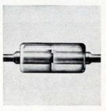
Whiskerless, voltage-variable capacitance diodes cover 3 to 18 pf. The Q's exceed 500 at 50 Mhz. Inductance is less than 0.5 nh; package capacitance, 0.2 pf. The diffused planar silicon units offer leakage under 100 na at 20-v reverse voltage. Double-plug construction gives reliability; the D0-35 package, high density. MSI Electronics Inc., 34-32 57th St., Woodside, N.Y. [443]
