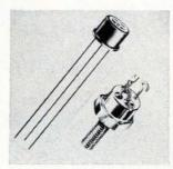
Triple-diffused, planar npn silicon transistors, designated 2400-6 (T0-5 case) anl 2800-6 (T0-59 case), are rated 7.5 amps. They range from 30 to 150 v with a typical frequency of 25 Mhz. The T0-5 units, at 10 w, cost from \$6.60 to \$21.40 each on orders of 100. Prices of the T0-59's range from \$8 to \$24. Silicon Transistor Corp., East Gate Blvd., Garden City, N.Y. [439]
