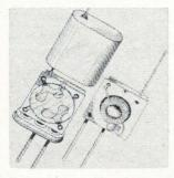
A six-pole quartz filter for use at or above 8 Mhz is contained in an HC 6/U package. The filter network is prepared using vacuum deposition with all resonators on a single quartz wafer. Foil leads are attached to the wafer and these leads, in turn, to the terminals of a p-c board. This allows 2 half-lattice sections on the wafer. Clevite Corp., 232 Forbes Rd., Bedford, Ohio. [353]
