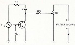
**Balance network.** To reduce zero-signal voltage of a shunt-switched filter, a nulling arrangement is applied.
