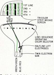
**Double-barreled.** Jatron color-tv tube has only two guns instead of the usual three, and strips instead of phosphor dots.
