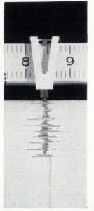
voltage electric writing method gives you sharp and clear printing on unique electrosensitive paper—and with instant start-up.
