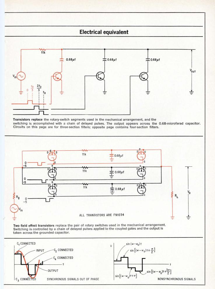
similar to that of a single-section LC filter. In its simplest form, the shunt-switched filter is represented by several parallel capacitors connected to segments of a rotary switch and returned to ground through the switch contact. The switch, which needn't be mechanical, rotates at a commutating frequency,  $f_{o}$ .
