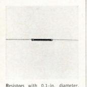
Residus values from 10 to 5,000 megohms in the ¼-watt size, type HACW, and 10 to 10,000 megohms in the ¼-watt size, type HADW. They are rated at 1,000 v and 5,000 v maximum, respectively. Both are terminated with 1½-in., No. 20 tinned-copper leads. Prices start at \$2.50. Resistance Products Co., Harrisburg, Pa. [345]
