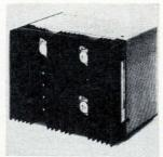
High-voltage d-c power supply modules include units to 410 v. Voltage regulation of 0.01% is provided in the BX series and 0.5% in the BC series. Both have plug-in p-c board construction, automatic overload and shortcircuit protection, remote sensing, and remote voltage adjustment or programing. ACDC Electronics, 2979 N. Ontario St., Burbank, Calif. [387]
