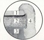
(b) Typical section of an NT-1 plated hole with uniform electro-less deposition of copper.
