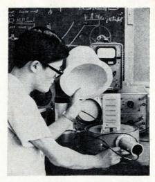
**On the block.** Yagi antenna for doppler-radar traffic sensor is made of foil strips cemented to polystyrene foam block. The "hat" is antenna's radome.
