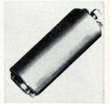
Infrared detector QKN1304 is for airborne and lab use. It uses an N-type indium-antimonide detector element that is sensitive in the 300-micron to 8-mm-long wavelength region, with 250-nsec response time. Standard aperture area is 4-mm diameter. Price is \$5,590; delivery time, from 30 to 60 days. Raytheon Co., 130 Second Ave., Waltham, Mass. 02154. [372]
