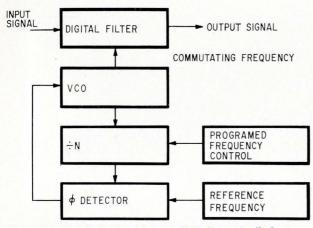
**Frequency hopping.** Stages for a digitally controlled system indicate the operation sequence. By regulating the voltage-controlled oscillator from the phase detector, the commutating frequency changes, thereby retuning the digital filter.
