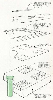
the Singer Co., says the process, called coplanar integration, casts chips in the ceramic substrate so that their faces are up and on the same level as the substrate surface. Friden inverts the package by placing the interconnecting grid of microscopic wires and two insulating silcon dioxide layers over the face-up chips.
