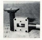
Frequency converter CX-7 has 8 to 12 Ghz (r-f) and 2 to 6 Ghz (i-f) bandwidths. Noise figure is 8 db; conversion loss, 7 db average. Harmonically related spurs are 30 db, other spurs 70 db below desired output for an input level of 3 mw or less. An l-o de-livering 3 mw for low level and 20 mw for high level use at 14 Ghz is required. Spacekom Inc., Box 235, Goleta, Calif. [410]
