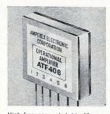
High-frequency, hybrid IC operational amplifiers are designated types ATF406 and ATF408. The thin-film circuits are fully frequency compensated at 25 khz for 6 db/octave rolloff. Open-loop gain is 100,000. Gain bandwidth product is 5 Mhz. Noise voltage is 10  $\mu$ v maximum. Micro-electronics division, Amperex Electronic Corp., Slaters-ville, R.I. [438]
