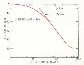
Slope variation. In the measured frequency response of a two-section series-switched filter the asymptotic slope is 10 decibels per octave instead of the theoretical value of 12 db per octave. This is due to a residual charge acquired by the network capacitors when the filter is switched into the circuit.
