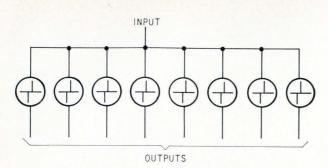
**Multiple array.** Proposed eight-output threshold switch array could be batch-fabricated on a single monolithic chip.
