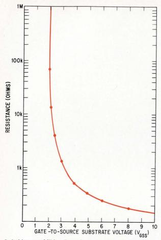
Switching capabilities. Plot of gate-to-source substrate voltage versus resistance for an MOS field effect transistor indicates a value of 200 ohms when  $V_{\rm GSS}$  equals 5 volts. Resistance increases infinitely at V<sub>GSS</sub> of 2 volts.
