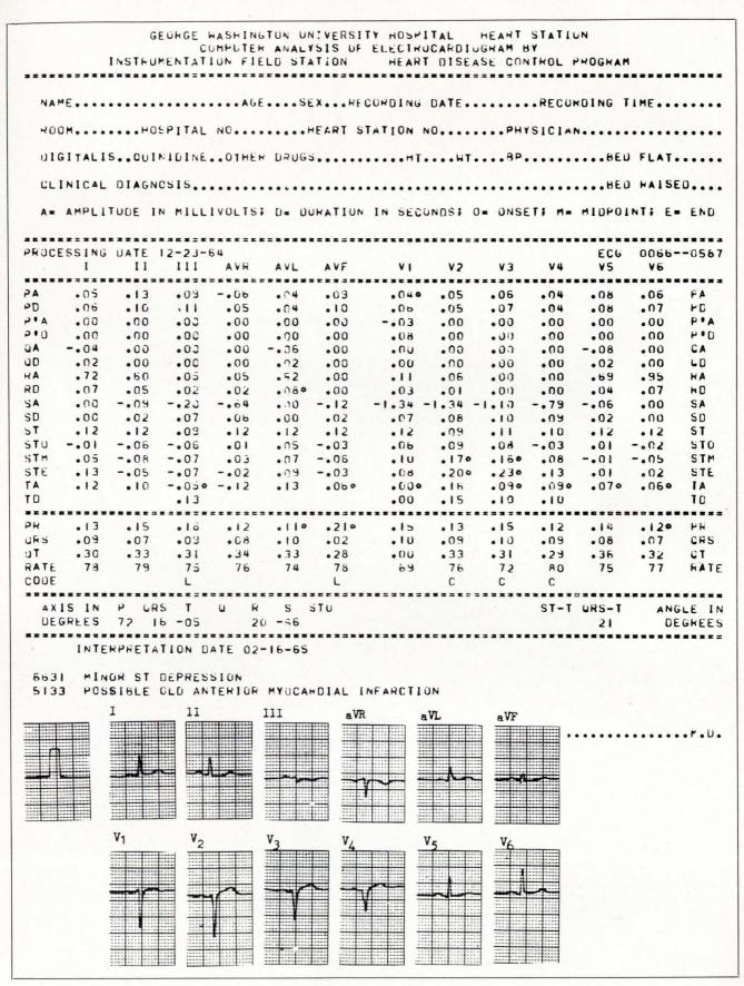
**Printout.** The amplitude (A) and duration (D) of the heart cycle's phases for each of 12 lead arrangements are calculated and tabulated by the computer. Asterisks (\*) mark suspicious values found by the computer as it compared the recording to a prestored table. The computer's diagnosis appears at the bottom of the printout.
