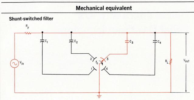
A simple shunt-switched digital filter is formed by connecting several capacitors in parallel to segments of a rotary switch. The circuit is returned to ground through a series resistor,  $R_{\rm F}$ , and the switch. Output is the voltage developed across the grounded capacitor,  $C_{\rm S}$ . Color indicates grounded capacitors in all diagrams.
