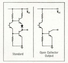
Before this circuit was developed, "Wire-OR" logic could only be used with DTL and RTL circuits. Now system designers can take advantage of this simplification and still benefit from the speed, economy and noise immunity of TTL.
