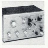
Transistor curve tracer CTA-2 displays a family of curves for both bipolar and field effect devices when used with any general purpose d-c scope. Base current steps of 20, 100, and 200 #a are provided with 4 ranges of sweep voltage to 240 v. Voltage steps for FET testing are continuously adjustable. Price is \$435. Rameco Corp., Box 580, Deerfield Beach, Fla. [362]
