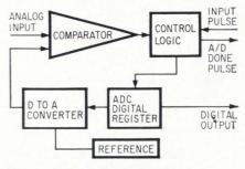
Comparison made. An input pulse triggers the control logic to set the most significant bit of the digital register. The bit is changed to a binary-weighted current in the digital-to-analog converter. The D/A current is then compared to the analog input, and the bit is either kept or rejected, depending on its size relative to the input current.
