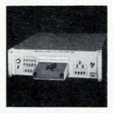
Analog measurements are made of digital IC's automatically by instrument 133. It can do up to 10,000 parameter measurements in 1,000 steps in  $\frac{1}{100}$  sec. Up to 15 readings can be made at a 10-#sec logical step. Programing is by two 5 x 6 in. circuit cards; one covering all devices in a family, the other the type to be tested. Teradyne Inc., 183 Essex St., Boston. [**367**]
