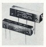
Standard resistance range of the models 3012 and 3052 Palirium cermet adjustment pots have been expanded from 10 ohms to 1 megohm. Operating temperature range is  $-65^{\circ}$  to  $+175^{\circ}$  C; contact resistance variation, 2.5%; and power rating, 1 w at 70° C. The Palirium cermet provides infinite resolution. Bourns Inc., 1200 Columbia Ave., Riverside, Calif. 92507. [356]
