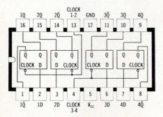
This specialized circuit was designed for readout tube applications. When used with the SN7490 decade counter and the SN7441 decoder/driver, the SN7475 will enable you to realize substantial savings in overall system costs.
