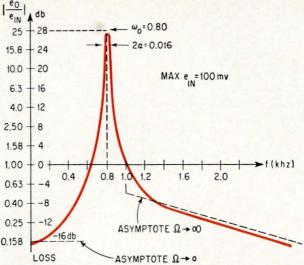
Selective amplifier at the top left is tuned in this example to 800 hz with Q equal to 50. All poles in the diagram at the lower left are in the left side of the complex plane together with two zeros on the sigma axis. Frequency response plotted above reaches a resonance at 0.8 khz.
