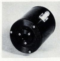
Precise, electronically controlled Q-switching at high repetitive frequencies is offered by a dual-crystal light modulator. The unit, a Pockels cell, can be used as a Qswitch, optical modulator, or shutter. It features low driving voltage and a high frequency response. Modulator performance is inde-pendent of temperature, because two electro-optical crystals mounted in temperature-insensitive crystal holders are employed.
