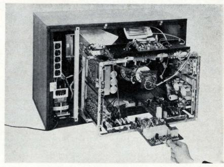
**Fast service.** Thorn opted for an easily serviced modular design for its all-transistor color-tv set. Most of the components are contained in 10 circuit boards that plug into a metal frame that slides out for servicing.
