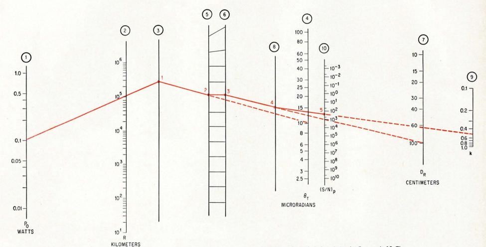
**Signal-to-noise ratio** is found at point 5 on scale 10. The points in color are determined by the values of the laser power,  $P_0$ , the distance between receiver and transmitter, R, the laser's beamwidth,  $\theta_T$ , the diameter of the receiver's collecting aperture,  $D_R$ , and the index of amplitude modulation, k.
