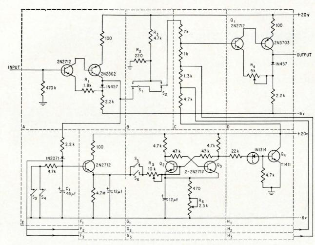
Scale factors are established when the outputs from H automatically change grounding points on the divider in stage C. Stage E detects the peak input voltage and con trols the outputs from the H stages.
