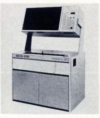
The first of a new family of incremental plotters operates at 800 steps per second. The series features high speed and accuracy,
