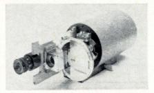
and then decreases to its original value as the rotation continues to 360°. It is possible to put octave infrared bandwidths on smaller segments of the filter wheel, resulting in one-, two-, three-, or fouroctave bandwidths at infrared wavelengths on only one CVF.
