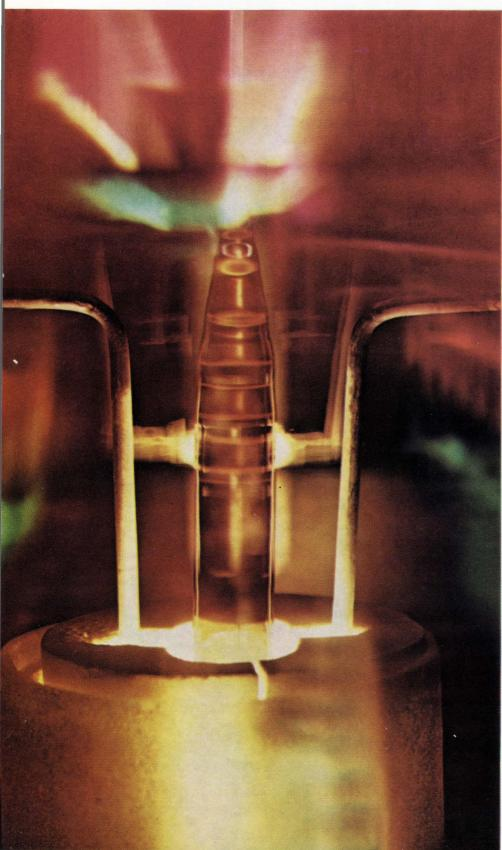
We grow the crystals. In fact, we grow more laser crystals than any other company in the world. So, when you're looking for higher laser efficiency, greater output, narrower beam divergence, increased brightness, or a new laser frequency—chances are, we grow the crystals that will give you what you want.
