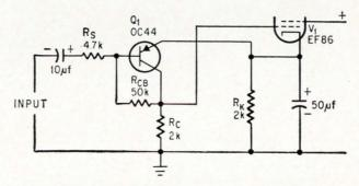
**Cathode bias** from tube  $V_1$  is the supply voltage for transistor  $Q_1$ . This preamplifier boosts the gain by 10.
