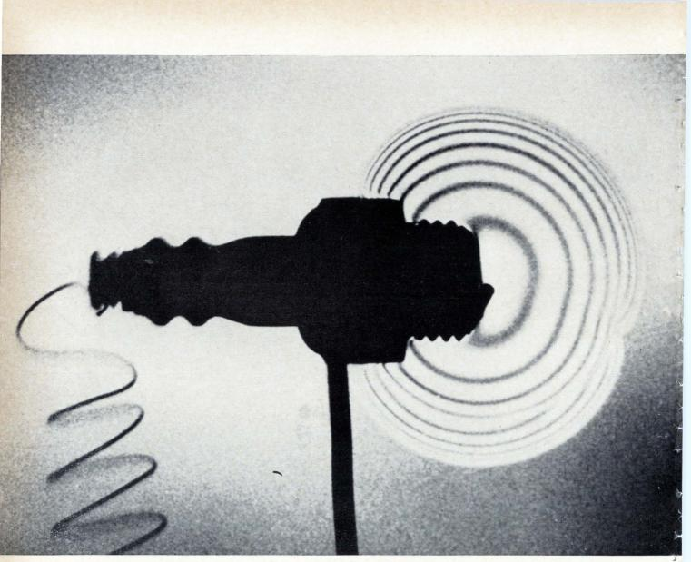
Holographic interferogram shows moving combustion front after spark plug ignites acetylene-air mixture.
