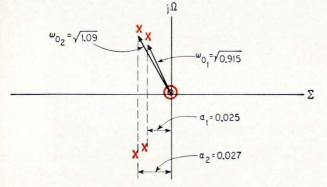
Location of the poles and zeros for unit  $M_1$  indicates both pole pairs are to the left of the j $\Omega$ -axis.
