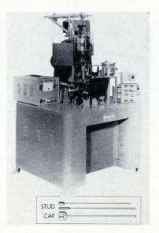
A high-precision stud welder produces a two-piece lead wire by butt welding a precut molybdenum slug to a Dumet wire. The slug is automatically fed into a six-head indexing turret, and the wire is then straightened, cut, and welded to the slug. The machine produces two-piece lead wires with the components in various lengths, diameters, and materials.
