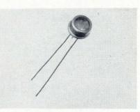
Resistive photocells combine cadmium sulfide and cadmium selenide to achieve the high stability of
