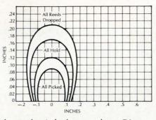
dry reed switch glass envelope. Dimensions shown along both axes represent displacement from the center of the magnet in alignment with the center of the reed switch.
