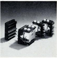
IBM wire contact relays can perform in excess of 200 million operations with an operate speed as fast as 4.5 ms, a release time of 5 ms maximum. The product line includes 4-, 6-, and 12-pole Form C relays, 4- and 6-pole latch models, all with compact, solderless, pluggable mountings—with coil-voltages up to 100 VDC.
