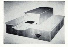
Quick, low-resistance connections to internal test points on p-c and multilayer interconnection boards are provided by a test adapter that checks for both continuity and insulation resistance. The Model TA101 connects to both sides of a four-layer board, checking the two sides simultaneously by means of some 700 plated-through holes on 0.100-in. centers.
