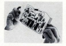
Extensive printed circuit applications are anticipated for a thermopoxy compound that is also an effective coating for electronic components where resistance to moisture, humidity, and vibration is required.
