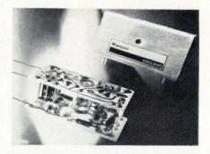
A self-contained oscillator has been designed primarily for use in portable test equipment. The unit, designated type F 3181, uses an integrated circuit as a heating element for temperature stabilization. The IC is enclosed in a tiny transistor can, together with a temperaturesensing device and the quartz crystal that controls the frequency of the oscillator.
