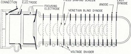
**Down the pipe.** Photomultiplier tube has 14 venetian-blind dynodes that amplify the electron beam through a series of secondary emission steps. The quadrants can be used with individual filters to sense the intensity of four color components of a light source. The tube is about  $6\frac{1}{2}$  inches long and 2 inches in diameter.
