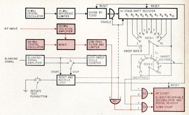
After mixing and filtering, modulator's r-f output passes through AND gates into the digital test set's count accumulator. Sweep rate (average slope) measurements are made by putting  $S_2$  in the sweep rate position and averaging the transmitter frequency over one cycle. This determines the most significant digits. Averaging the frequency over 1,000 cycles determines the least significant digits.
