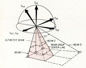
Radar velocity sensor's beam 1 geometry is typical of the landing radar's four beam patterns.
