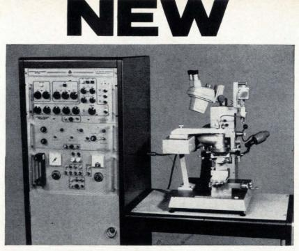
Airbrasive<sup>®</sup> Resistor Trimming System:
