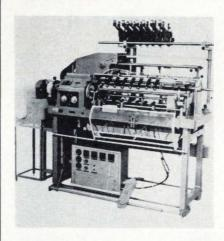
A new ballast-transformer winder uses an automatic paper-insertion technique that eliminates paper wrinkles and speeds the winding process. The paper is fed laterally so that its fibers are always kept parallel to the winding arbor, or coil stick, preventing wrinkles. Paper length is preset simply by adjusting a dial.
