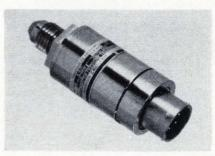
sure transducer designed for aerospace applications. The type 4-420 has an output range of 250 mv d-c for an excitation voltage of 10 v d-c or a-c rms. Units come with integral electronics for an output of 0 to 5 v d-c and an isolated input of 28 v d-c. Weight is less than 3 oz.
