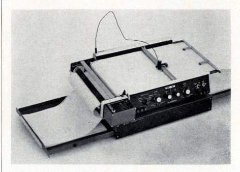
With a new automatic paper advance unit, x-y recorders can be made to perform many other functions besides x-y plotting. The unit allows the recorder to operate in three different modes: incremental paper advance, continuous stripchart action, and frame-by-frame paper advance, a new mode.
