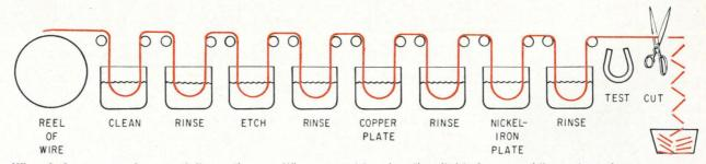
**Wire plating process** is essentially continuous. Wires are cut to a length suitable for assembling onto a plane, except when flaws are detected. Defective wires are cut at the flaw and the pieces are always shorter than good wires, hence easily separated.
