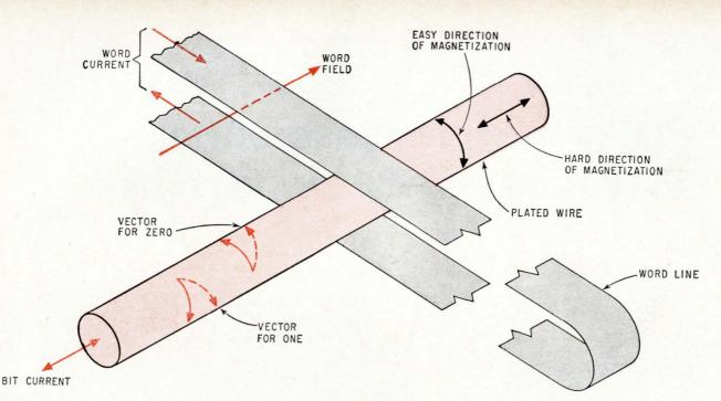
**In a plated-wire memory,** the word line forms a one-turn coil around several wires. A current in the word line tilts the vector magnetization from its rest position, shown in solid lines, toward the hard axis of magnetization, generating a pulse in the plated wire.
