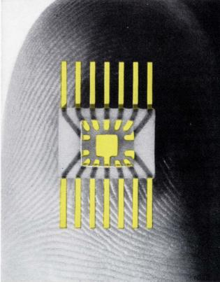
It's Sel-Rex Temperex<sup>®</sup> 'S', 99.99+ gold. And it will pack a lot more reliability into your integrated circuit manufacture. Temperex 'S' deposits withstand  $500^{\circ}$ C in air for five minutes with ease. There's no discoloration of the semi-bright gold because there isn't a trace of contaminants.
