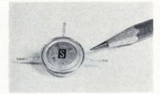
**Useful in military** and aerospace applications, a 10-amp silicon Darlington amplifier series in <sup>3</sup>/<sub>4</sub>-in. flatpacks is also adaptable to many commercial and industrial circuits.
