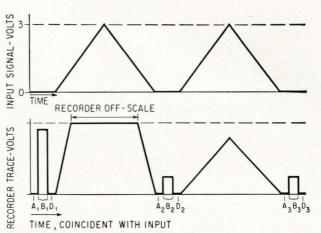
An off-scale trace is obtained on the recorder when the peak input exceeds 1 volt. The smaller calibration pulse at  $B_2$  indicates that the recorder scale is increased by a factor of 4, yielding a subsequent on-scale trace for the same peak input.
