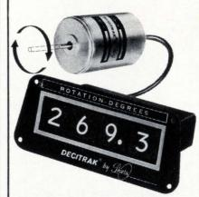
DECITRAK® is the only complete system, encoder plus all electronics, for transforming shaft rotation as well as synchro/resolver outputs into digital readout. Low-cost DECITRAK systems are available in 3-digit to 6-digit versions with 523 solid-state accessories. They interface precisely with most digital computers . . . also offer digital outputs for sequencing, motor control and set-point programming. All have extraordinarily long life. Fast delivery, too!
