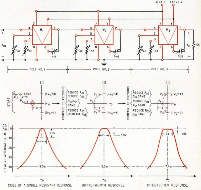
**Cascaded Minactors** produce a variety of responses ranging from a single resonance to a Butterworth response, or to an equal-ripple Chebyschev pattern. All the Minactor units are nominally the same, but  $M_1$  is tuned to the desired center frequency and adjusted for maximum gain. Other units are adjusted to provide unity gain at their respective resonances.
