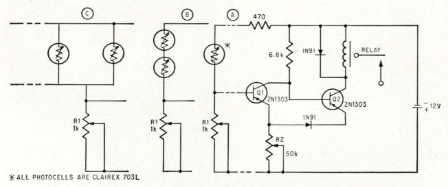
**Photoconductive cells** supply varying base drive to  $Q_1$  as light intensity changes. When  $Q_1$  cuts off with low base drive,  $Q_2$  conducts, energizing the relay.
