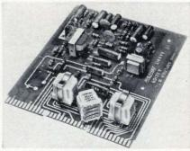
Four-pole standard and latching magnetic relays can switch up to 4 Form A (make) plus 4 Form B (break) in separate circuits, or up to 4 Form C (transfer) contacts, or any combination thereof. The switching versatility of the Printact relay eliminates the need to stock a variety of different units and cuts costs. Among other savings claimed for the relay are space, weight and production time.
