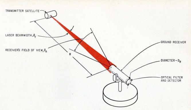
**Optical communications** detector receives not only the laser beam, but any background noise that falls within its field of view,  $\theta_{R}$ .
