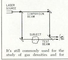
tests in wind tunnels and shock tubes. Its square configuration allows wide separation of the test and comparison beams; often the comparison beam can be routed around the subject.
