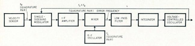
LM's frequency tracker is a closed loop servosystem that processes sensor and reference signals.
