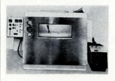
Silicon wafers and substrates of glass, ceramic, and thin-films of any size and shape can be automatically coated with photoresist on a large-scale production basis by a vapor carrier system. The process applies pure, uniform coatings in the angstrom range, thereby assuring fine line definition.
