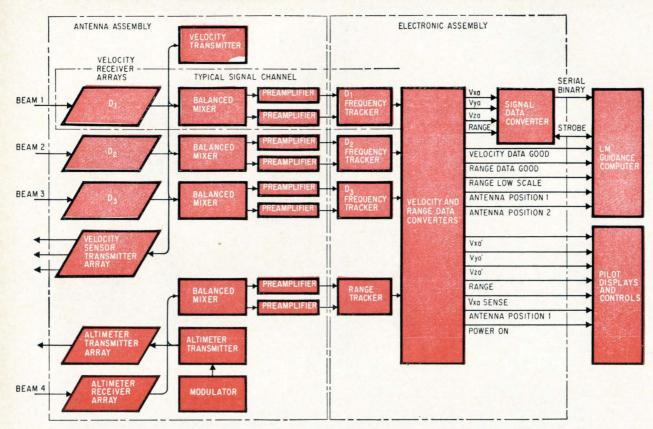
Lunar module's landing radar combines transmitter velocity and altimeter signals with the signals in return beams to produce doppler frequencies proportional to the spacecraft's velocity and range from the moon. Data converters break down the doppler signals into velocity components in the X, Y, and Z direction. These are input signals for the module's guidance computer.
