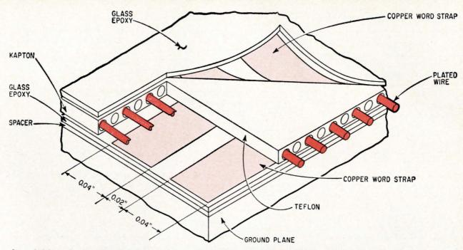
A sandwich made of plated wires between two layers of plastic insulates the wires from the word straps. The ground plane is a copper-clad glass epoxy board like those used for printed circuits.
