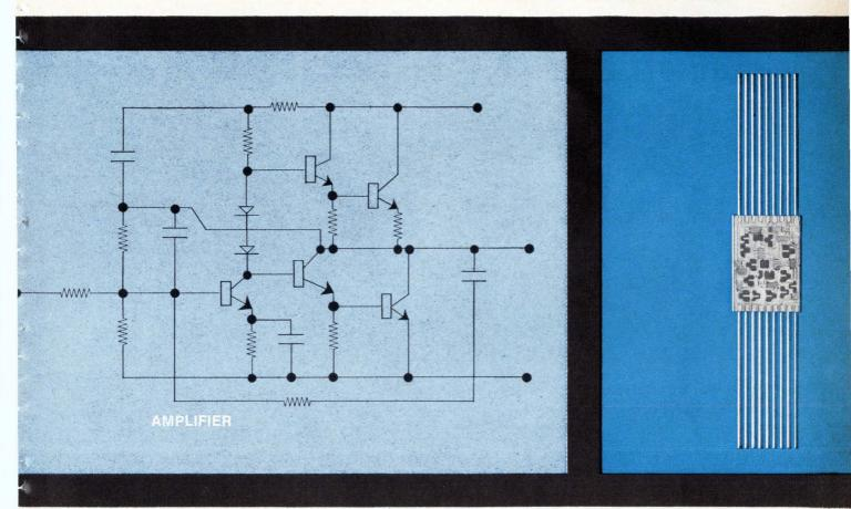
Volume microcircuit production of your analog or digital circuit is accomplished at Mepco by HYBRIDIZATION. The ability to manufacture precision passive film components is complemented by a wide variety of semiconductor attachment techniques. These capabilities provide the required flexibility to microminiaturize your circuit at the lowest possible cost. Consider these exceptional performance characteristics.
