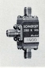
**Once limited** to moderate bandwidths, miniature switches can now range across the 1- to 18-gigahertz microwave band. Somerset Radiation Laboratory Inc. claims that it has the first microwave switch that can cover this frequency range in a single unit.
