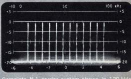
Complete N-1 carrier system shown in 120-kHz sweep width mode. Slope is 0 db, all carriers present, channels 2-13, high group.
