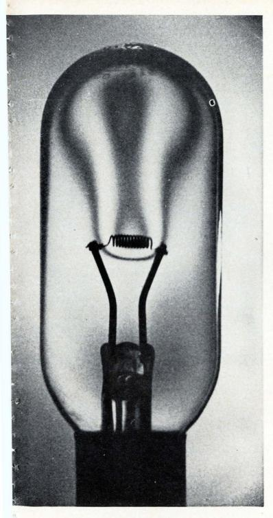
Differential interferometric measurements using double-exposure hologram of a light bulb. One exposure is made with the filament cold, the second with the filament heated. The difference between the two exposures is due only to the density changes in the gas inside the envelope. The interferogram is clear despite the poor optical quality of the glass bulb.
