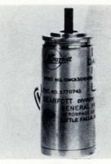
A size 8 inertial damped servomotor is suited for high-gain or high-speed servosystem applications. Weighing only 2.6 oz, the component is totally enclosed within a single stainless steel housing measuring only 1.68 in. in length. A rugged and reliable 400hz unit, the motor has two windings on the control phase, permitting either series or parallel operation. Stainless steel, high-precision bearings assure long, trouble-free service.
