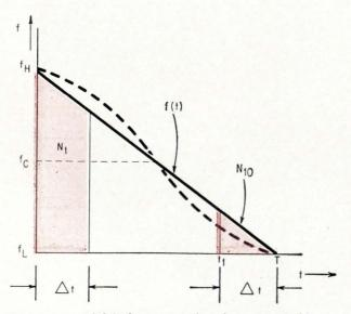
**Frequency modulator's** average slope is represented by the solid line between  $f_{\rm H}$  and  $f_{\rm L}$ . Nonlinearities are depicted by the dashed inverted S-curve. The tinted areas are equivalent to the change in transmitter frequency during pulse sample intervals N<sub>1</sub> and N<sub>10</sub>.
