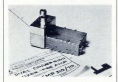
Mixer-preamplifiers offering dual conversion feature two intermediate frequencies that provide high selectivity and gain at a low i-f while reducing image frequencies of the high i-f. Dual conversion simplifies systems requiring a frequency synthesizer as a local oscillator. A vhf synthesizer can be used as the second l-o, with a crystal-controlled microwave source as first l-o, eliminating the need for an expensive, complex microwave synthesizer.
