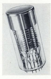
Recent advances in photocathode design have made possible photomultipliers with improved characteristics. According to the manufacturer, quantum efficiency has been almost doubled and now approaches 30%; the bialkali cathode has a sensitivity of 65  $\mu$ a/lumen; and, when the tube is operated at maximum gain, the dark current is less than 10<sup>-9</sup> amp. Spectral range is 3,400 to 6,500 angstroms, peaking at 4,000.
