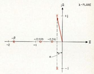
**Normalized Minactor function**, M ( $\lambda$ ), is plotted in the complex  $\lambda$ -plane. Crosses represent the poles of the function, circles represent the zeros. The angular frequency  $\omega_0$  is a vector drawn from the origin to the pole. By adjusting  $R_0$  the designer can shift the poles horizontally. Varying  $C_0$  shifts the poles vertically. Shifting the zeros doesn't affect resonance.
