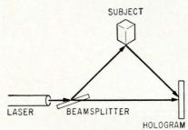
angle between the two beams. For the typical 30-degree beam angle, the spacing is twice the wavelength. The hologram's interference pattern shouldn't be confused with the pattern in the interferometer. In an interferometer, the beams are nearly parallel ( $a = 0^\circ$ ), so that fringe spacing is much greater and can be analyzed with the unaided eye.
