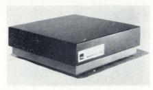
Transmission of digital data at a 4,800-bit-per-second clip over unconditioned Schedule 4 telephone lines is the key ability of a new data set. The unit, called the Model 4400/48 uses a relatively narrow bandwidth to transmit over the lowest cost lines. It avoids the frequencies that are severely distorted on such lines.
