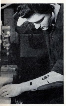
**Steady.** Electromyographic-controlled artificial hand manufactured in Austria has selective amplifier circuits that protect users from spurious finger movements.
