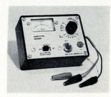
A go-no-go type, battery-operated instrument determines whether transistors are operational or faulty. Model 20 will show, in two steps, whether the transistor type is npn or pnp, if it is operating properly, and its d-c beta.
