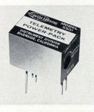
Transducer excitation in advanced instrumentation applications is provided by a telemetry power supply that measures  $0.73 \times 0.52 \times$ 0.50 in. and weighs 0.24 oz. It features reversible polarity, overvoltage and short-circuit protection. It also has adjustable output voltage, isolation of output from input and
