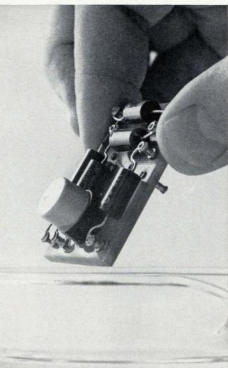
Temperature test your integrated or hybrid circuits in a 3M Brand Inert Fluorochemical Liquid and it'll drain clean, dry immediately and leave no residue.
