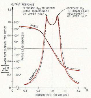
Filters can be synthesized directly from a given transfer function. Here the theoretical (color lines) and actual (dashed lines) curves are the output plots. Adjustments of the components can easily correct the small error caused by approximation of  $\lambda^2$ . Adjustments between the two curves can be made by tuning the Q of each pole.
