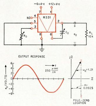
Design of this local oscillator requires a Model M331 unit connected as shown. Poles of the assembly are in the right half of the  $\lambda$ -plane. Negative portion of the output waveshape is slightly clipped due to the cutoff in the output stage of the Minactor amplifier.
