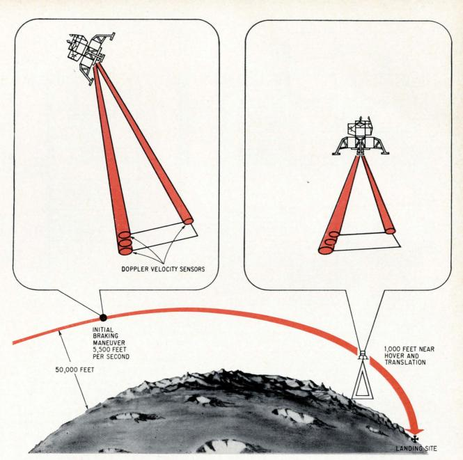
**Powered descent** begins when lunar module's altitude is about 50,000 feet. Throughout the tilt maneuver, the four radar beams are kept pointing at the lunar surface automatically by the guidance computer. The repositioning is accomplished by rotating the antenna of the landing radar around the Y axis into either of two positions.
