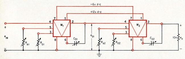
Cascade arrangement of two Minactors are used to reproduce the transfer function of equation 25.
