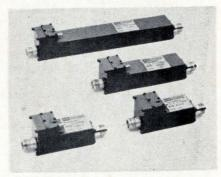
Precision directional r-f samplers covering 0.25 to 2.4 Ghz in four octave bands have an amplitude variation less than  $\pm 0.3$  db and calibrated detection sensitivity of 10 mv/mw up to 20 mw. Designated models 1009, 1010, 1011, and 1012, each consists of a directional coupler, a built-in crystal detector and a low-pass input filter. The frequency ranges are 250 to 500 Mhz, 0.5 to 1 Ghz, 1 to 2 Ghz, and 1.4 to 2.4 Ghz.
