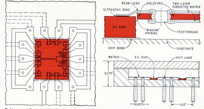
Tight squeeze. Beam-lead bonds and feedthrough eyelets of interconnection matrixes are shown in plan and cross-section in the sketches on the left and at the top. At the bottom is one package design ITT plans to use for chip assemblies.
