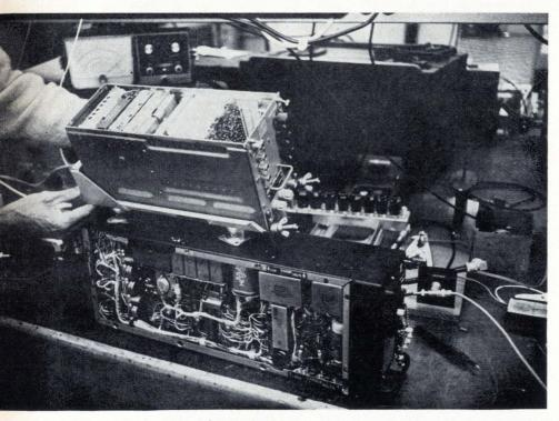
**Tri-service.** Mohawk's AN/APX-44 IFF (identification, friend or foe) system (below) will be replaced by the APX-68 (above) or the APX-72; eventually, all three services will standardize on a single unit.
