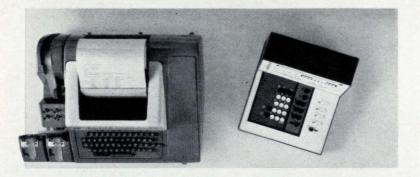
Name familiar but you can't remember the face? The insides of this new Mathatron computer calculator are different, too. Log, antilog, sine, cosine, and arctan are performed at the touch of a button. Storage 4000 bits. Simplified program control. And the price-performance ratio is higher than any other computer/ calculator. Starts at \$6990.
