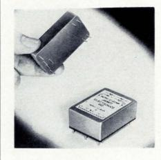
**Six 2pdt and 3pdt** with sealedmercury-wetted capsule high-speed relays have been introduced for p-c board mounting. Called Merc-O-Scan, they are designed for lowand medium-level switching applications. Typical uses include industrial process control systems, data acquisition, multiplexing, analog instrumentation, and sensing devices such as thermocouples.
