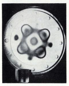
**Mode pattern** of a vibrating membrane of a sonar transducer. The vibration frequency increases from top to bottom in the experiment performed by R.L. Powell of the University of Michigan. quality optical elements for good results, precision is necessary in the positioning and holding of the hologram plate. To eliminate the chance of bending or distortion, thick photographic plates—of quarter-inch glass, for example—must be used and carefully processed.
