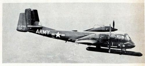
Success story. Army's Mohawk surveillance aircraft can data-link infrared and side-looking radar pictures of targets back to base almost immediately.
