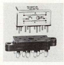
Low-cost switching devices permit electrical isolation between input and output circuits with a lamp-tophotocell light-beam coupling. Insulation resistance is about 10<sup>9</sup> ohms with smooth turn-on and turn-off. Input and output voltages may be either a-c or d-c. Voltage gain is high, with signals as low as 6 v capable of controlling output circuits rated to 250 v.
