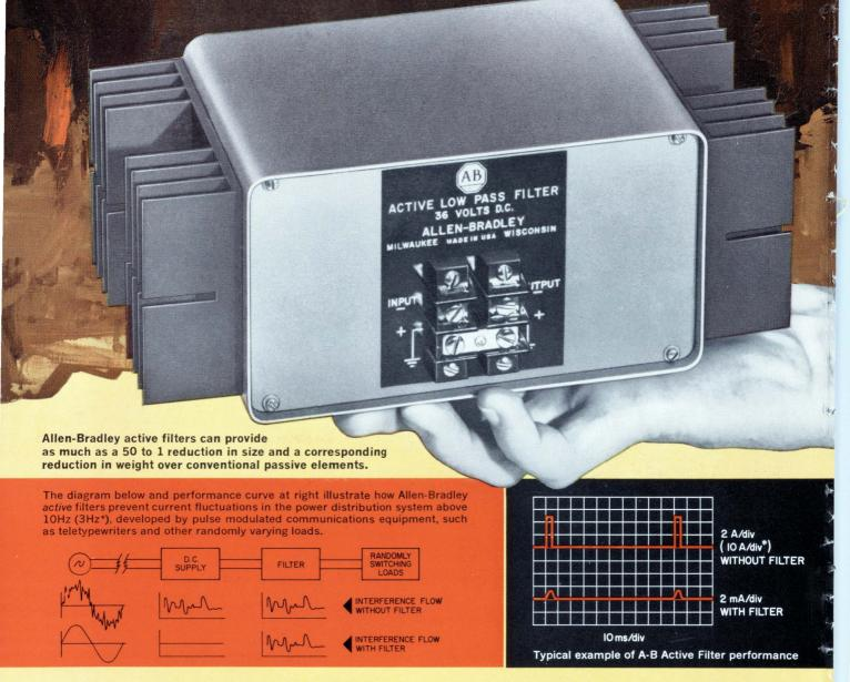
■ Directly as the result of some new ideas applied to the field of ElectroMagnetic Compatibility, Allen-Bradley has been able to produce a new *active* low pass filter that provides an attenuation of greater than 60 db over the range of 10Hz (3Hz\*) to 100KHz. The maximum dc component of the load current is 5 amperes.
