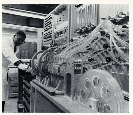
Apparatus for plating wire is capable of plating three strands at once —as indicated by the three holes at the entrance to the first cell. The supply reel is in the foreground and the cutting and testing station at the far end.
