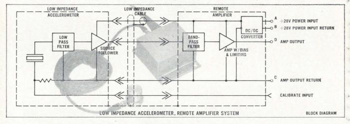
A new CEC Low Impedance Piezoelectric Accelerometer System, especially designed to operate in a high thermal and mechanical transient environment, has been selected for America's most advanced new missile.
