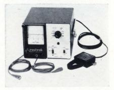
A portable power tester and recorder handles voltage, current, or both. The instrument features a time-sharing system that permits the stylus to record independent traces for both voltage and current. This system provides full chartwidth resolution with voltage plotted as a continuous trace and current as an interrupted trace for easy identification.
