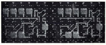
**Unmasked.** Standard Telecommunications Laboratories is working on a lasermachining technique that deposits—without using masks—interconnection patterns on large-scale integrated circuit arrays.
