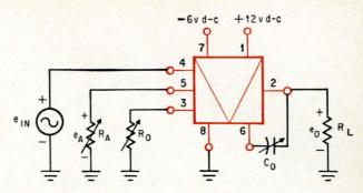
**Connection diagram** for normal operation of the Minactor shows pin 8 as the reference, and pin 4 as the input control. Elements  $R_A$ ,  $R_0$ , and  $C_0$  tune the filter.
