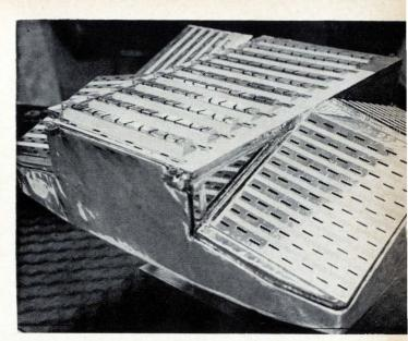
Landing radar antenna is covered with special thermal finish to protect it against extreme temperatures in space. The center section contains the altimeter and velocity sensor transmitting antennas. The outrigger antennas at either side of the center section are for the receivers.
