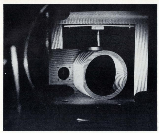
**Real-time interferometry** technique in which the comparison beam is stored on a hologram and the test beam is actual. In this arrangement, developed by K.A. Haines and B.P. Hildebrand of the University of Michigan, deformations caused by the applied load set up an interference pattern.
