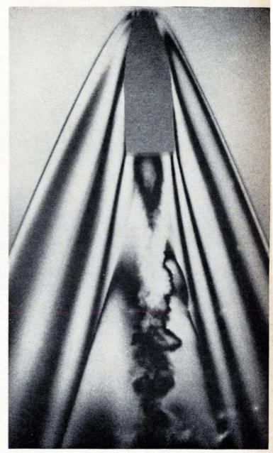
**Shock layer** surrounding a .22 caliber bullet traveling at 3,500 feet per second is shown in double-exposure holographic interferogram. The relatively long exposure time, 0.25 microseconds, causes a slight blurring of the bullet image.
