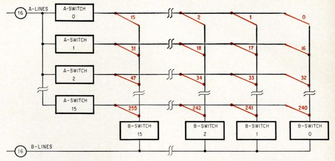
Sixteen A-switches and 16 B-switches provide a matrix that selects one of 256 word lines, shown in color. Each word line forms a one-turn solenoid around a group of 144 plated wires containing 16 nine-bit words. Four planes with four sets of B-switches and a common set of A-switches make up the complete plated-wire memory.
