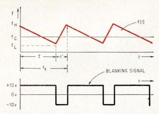
Frequency of Apollo radar altimeter's modulator varies as a sawtooth function with a center frequency of 99.79 Mhz. A blanking pulse synchronized to the r-f wave is also produced. Frequencies  $f_{\rm II}$  and  $f_{\rm L}$  are the upper and lower band limits of the sawtooth; and T and t' are the downsweep and upsweep pulse periods.
