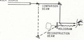
**Test beam** in the Mach-Zehnder interferometer can by synthetically generated with a hologram. The viewer then sees the interference pattern between the comparison beam and the test beam, released from the hologram with an auxiliary beam.
