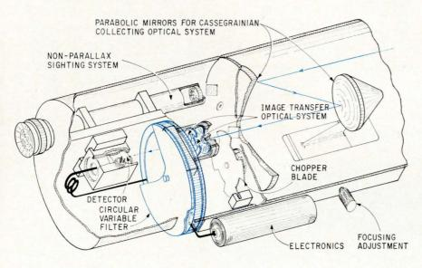
The key element in a spectral radiometer that makes continuous measurements of infrared radiation is a circular variable filter. This component is an optical interference filter whose transmission wavelength varies with the filter's angle of rotation.
