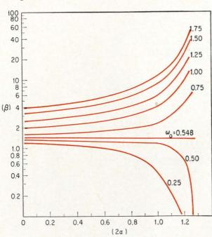
**Values for**  $\beta$  are determined from this plot when the designer inserts  $\omega_{2}$  and  $\alpha$ . The  $\beta$  value is used to locate the filter's pole along the real axis.
