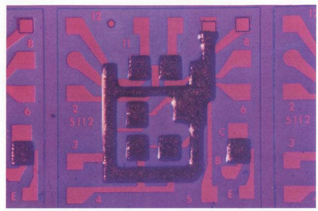
Chunky portions of Decal circuit are pieces of silicon isolated by etching and held together by a glass substrate.
