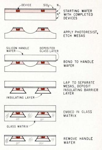
Handle wafer holds isolated islands in position on a silicon wafer until they are embedded in a dielectric matrix.
