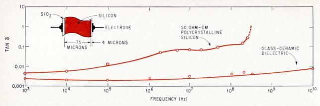
**Glass-ceramic dielectric** of the mosaic wafers has a low loss tangent at microwave frequencies. A conventional type of isolation, polycrystalline silicon refill, appears to be useless at about 250 Mhz. Refill is approximated by the sample configuration.
