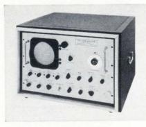
Using a comb of frequencies for accuracy measurements, a sonic spectrum analyzer covers the 0 to 50 khz range with a frequency accuracy to better than 10 hz. Model SS50-S is a valuable tool in the field of vibration, noise, dis-
