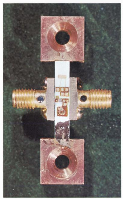
Lumped element amplifier will measure only about 0.1 inch square. This breadboard version's substrate is about  $\frac{1}{2}$  inch long. Used as a power amplifier at a frequency of 2 Ghz, it has an output of  $\frac{1}{2}$  watt with a gain of about 4 db. Its components are lumped inductors and capacitors.
