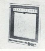
Capable of measuring 2, 3, 4, 6, or 12 inputs, a compact multipoint recorder has a full 6<sup>1</sup>/<sub>2</sub>-in. scale. The face area of the instrument is approximately 2<sup>1</sup>/<sub>2</sub> times smaller than a conventional 12-point unit which uses a 12-in. chart. Two of the series RD5 recorders can be mounted side by side in a standard 19-in. panel.
