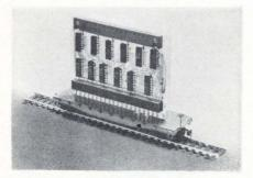
Two series have been added to the MoniLogic line of integrated-circuit logic cards. The dual in-line diode-transistor-logic (DTL) and transistor - transistor - logic (TTL) cards are called Series 8D and 8T, respectively. Savings afforded by the use of dual in-line IC's can run as high as 40%, according to the manufacturer.
