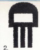
PET TO-5 is rated from 550 mW to 1.2 W at 25°C (chip dependent).
