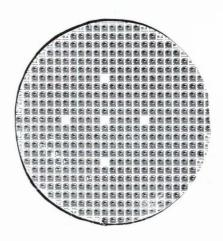
**Mosaic wafer** allows the diffusion of active devices and their interconnection after isolation processing to make the circuits seen on page 99. Each tiny dot is an island of silicon, surrounded by dielectric.
