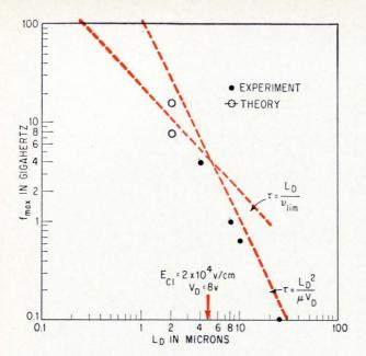
Thin-film triodes with a source-to-drain separation,  $L_{\rm D}$ , of 4 microns have a maximum frequency response of 4 Ghz. Halving the source-drain length again will probably extend the response to 8 Ghz rather than 16 Ghz because the critical field (arrow) is exceeded at this point in very small devices, and electrons reach their limiting velocity.
