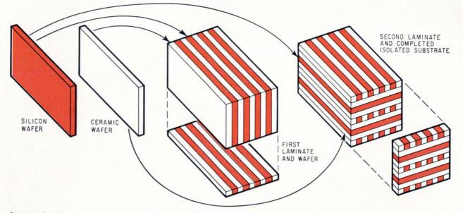
Layers of silicon and ceramic are bounded together, then sliced and laminated again to form a sandwich matrix of isolated silicon blocks. This technique can be used when arrays of field-effect transistors are needed. Thicker ceramic wafers provide a broader substrate area for thin-film devices.
