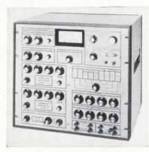
built with solid state devices, which operates over the frequency range from 4 khz to 500 khz.
