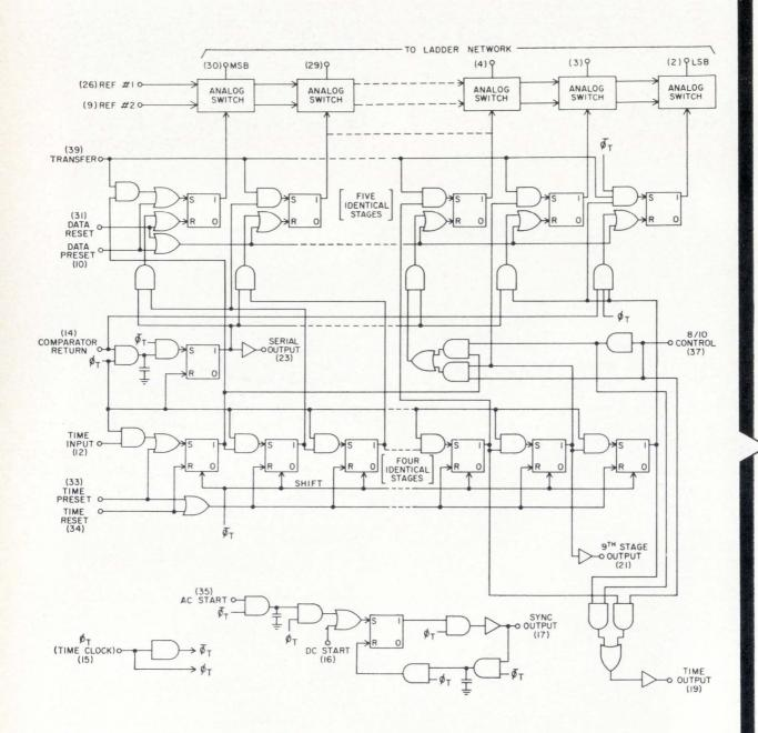
**Another ATOS First...** This Monolithic A/D-D/A Converter incorporates General Instrument's exclusive MTOS (Metal-<u>Thick</u>-Oxide-Silicon) process which provides Large Scale Integration without the need for high-cost discretionary wiring.
