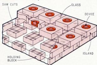
Matrixes can be made by sawing the wafer into squares . . .
