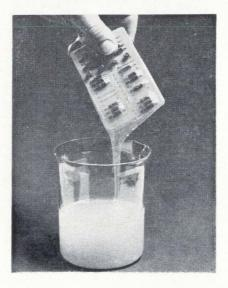
**Two new single-component** RTV (room-temperature vulcanizing) silicone rubber materials—a clear conformal coating and a highstrength sealant—are cured by a system that doesn't give off corrosive by-products. Previously available materials of this type, according to the producer, gave off a small amount of acetic acid during the cure, and this acid by-product could cause corrosion of copper during the curing period under humid conditions.
