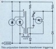
circuit is a typical application for Type 11Z13 Trigate Pulse Transformers.
