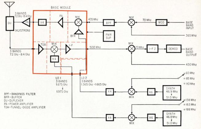
**Communications systems** would be made of one, or a few, modules supplemented by signal sources, modulators and demodulators that adapt the module operation to the specific system needs. With the klystron power amplifier, power could be boosted to the level required for troposcatter transmission.
