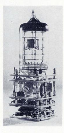
An unusual miniature oscillator uses an integrated circuit to stabilize the temperature of its crystal assembly for ambients of  $-55^{\circ}$  to  $+90^{\circ}$ C. The oscillator can be preset and supplied at any frequency between 10 and 15 megahertz. Since only 500 milliwatts are consumed at the worst-case ambient of  $-55^{\circ}$ C, applications in airborne equipment and manpack receivers are possible.
