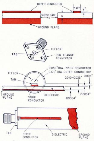
**Microstrip transmission line,** shown in cross-section at the top can be extremely small. However, it must be coupled to relatively large external connections. Below it is a transition that joins the microstrip to a miniature coaxial connector.
