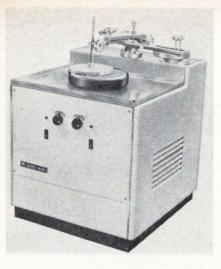
The Model PA818 is powered by a <sup>3</sup>/<sub>4</sub>-horsepower motor with continuous variable speed control up to 175 rpm. The 18-in. stainless steel wheel rests on a heavy duty 8-in. thrust bearing. The polishing wheel will accommodate four 63/4-in.-diameter pressure plates that can be independently driven to accelerate the polishing action.
