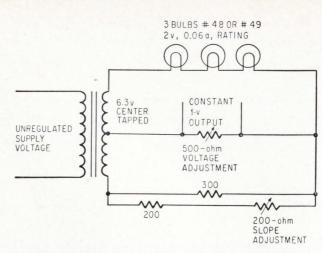
**Bulb resistance increases** to maintain a constant voltage across the load lamp of a bridge when supply voltage goes up.
