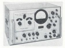
Automatic scanning is featured in a solid state noise and field intensity meter. The instrument is designed to meet the requirements of all applicable federal and military standards and specifications.
