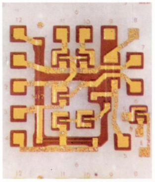
**Diffusion and metalization** processes similar to those used to make conventional IC's have converted the mosaic into a radio-frequency mixer circuit. The isolation between devices allows this circuit to operate at higher frequencies than can regular IC's.
