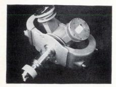
**High-gain**, crossed-field amplifier tubes deliver 1 megawatt peak power (3.5 kw average) over a 5.45 to 5.825 Ghz band. The SFD-231 amplifier, designed for pulsed coherent and frequency-agile systems, will amplify a signal without adding significant phase noise or phase distortion. Pulse width is 10  $\mu sec.$  Duty factor is 0.0035 maximum.
