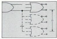
The capability of MECL II current-mode logic to fan-out up to 25 makes it superior in this category to all other available integrated circuit digital systems.
