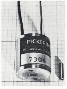
Conversion of motion to linear d-c output from 6-v d-c input is achieved by a linear variable differential transformer. Besides measuring, detecting, and controlling linear motion from a d-c supply, the unit can also be used for force and pressure measurement.
