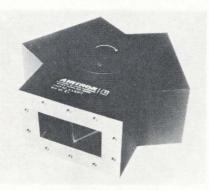
Application of a high-power ferrite material makes possible a junction circulator that can handle 5 kilowatts c-w at 2.4 to 2.5 Ghz. This is reportedly about 10 times the capability of previous units. The necessary electrical symmetry is provided by a Y-junction.
