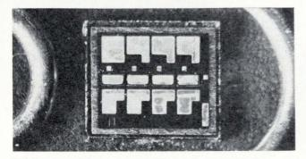
Wideband amplifiers are made 42 at a time on an inchsquare sapphire wafer. Chip transistors will be added.
