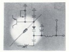
Voltage-variable capacitance diodes feature a high Q and high tuning ratio. The MV1720 through MV1750 series of silicon Epicaps cover a capacitance range of 6.8 to 100 picofarads with a capacitance tolerance of 10% and a re-
