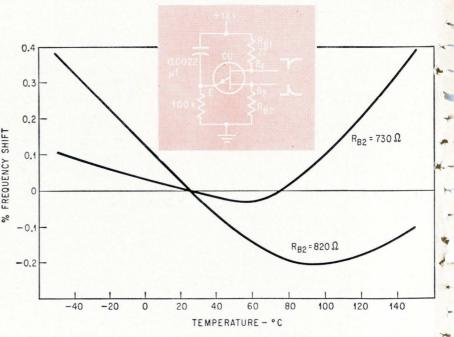
**Despite wide change** in value of base-2 bias resistor the frequency shifts less than 0.5% in a 5-khz relaxation oscillator built using GE's new unijunction transistor. Bias resistor is selected to get curve closest to zero frequency shift line.
