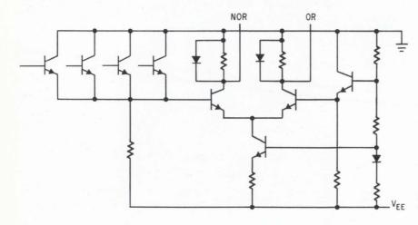
**From its very name,** one might suspect that emitter-emitter coupled logic might be superior to ordinary emitter-coupled logic. And it is, says the Westinghouse Electric Corp.'s Molecular Electronics division, which has just started to market integrated circuits that have emitter-to-emitter input coupling. The E<sup>2</sup>CL line has typical switching speeds of 2 to 3 nanoseconds with a fan-out of 3, compared to the 5 nsec that have been achieved with ECL counterparts.
