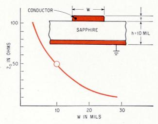
Sapphire acts as a high-quality dielectric for microstrip interconnections. Line impedance is typically 50 ohms when the sapphire is 10 mils thick and the conductor is 10 mils wide.
