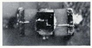
Another transistor mount. This one can be soldered directly to a microstrip transmission line.
