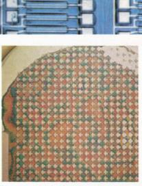
Close shave of wafer yields isolated transistor collector regions whose depths vary less than  $\pm\,$  0.3 microns. Color fringes confirm accuracy.
