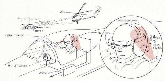
**Using his head.** When helicopter pilot has target lined up in sight, he flips on-off switch and then computer system aims weapons or reconnaissance cameras automatically.
