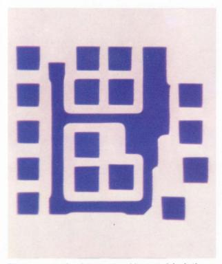
**Glass and ceramic mixture**—the white material—is the matrix that isolates the islands of silicon and keeps them in place during the high-temperature processing needed to fabricate an integrated circuit. Only enough silicon for a circuit remains after isolation etching.
