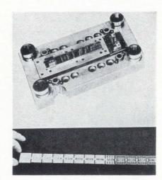
New carbide dies make possible the production of precise, subminiature frames for integrated circuits by stamping at rates of up to 200 pieces per minute. In their first application, the dies were used to make IC frames of 0.010-in.-thick Kovar, a soft magnetic material with high nickel and manganese content.
