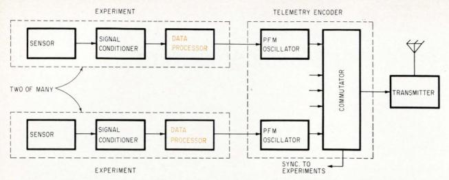
A single channel encoder replacing multitudinous pulse-frequency modulated oscillators is a step in the right direction, but still requires the inefficient special-purpose processors.
