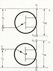
**Complementary unijunction,** top, has all currents and voltages reversed from standard unijunction. The complementary unit is made in IC form.
