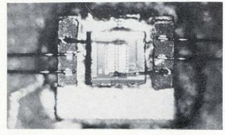
Mount for an r-f transistor. The opening is 0.020 inch square. The leads to the mount are wires.
