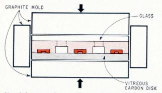
**Glass is hot pressed** around the squares or mesas, and the excess silicon at the back of the wafer is removed.
