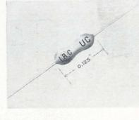
Bridging the gap between available discrete resistors and micro-circuitry is a new metal film resistor that satisfies the requirements of MIL-R-10509, and is believed to be the smallest commercially available. The UC resistor measures 0.125 in. long and 0.047 in. in diameter. It has No. 30 Awg (0.010 in.) gold-plated dumet leads.
