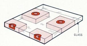
**Devices in the silicon islands** are isolated by the glass, on which thin-film wiring and components can be deposited.
