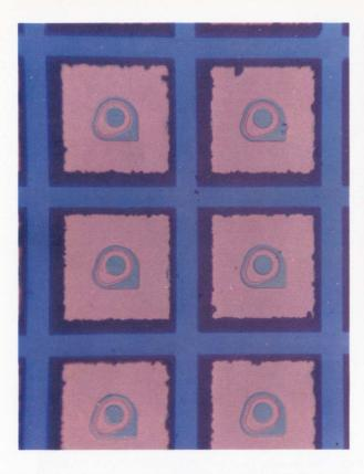
and switching times achieved with monolithic IC's. Radiation resistance of dielectrically isolated circuits should be superior to that of monolithic IC's, since the isolation junction is the monolithic element most sensitive to radiation damage.<sup>4</sup> The thermal problems that arise when a relatively high-power device is included in the monolithic silicon structure can also be significantly reduced.
