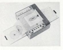
Consecutive records without individual hand loading of sheets are possible with an x-y recorder that uses fan-fold paper. The paper may be loaded or unloaded in midrecord and each record can be torn out as an individual sheet at the perforations. Both forward and reverse advance is inherent and can be controlled automatically by programing. Each record is capable of automatic advance when the extreme margin is reached.
