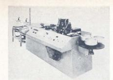
ters over the entire length of the wire; on 2-in. centers on the leading and trailing ends (up to 36 inches); and on 2-in. centers on the ends and on 15-in. centers over the remainder of the wire. The machine works on 115 v, 60 hz, and requires 100 psi air at 5 cfm.
