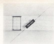
lead that is attached to a multifingered fixed wiper and is insulated on one side. The resistance element consists of fine wire closely wound on a metal mandrel. High-density winding and the design of the wiper afford high resolution with the wirewound element.
