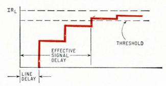
In nonmatched system, line reaches stable value after several reflections. Curve shows how effective delay of signal is greater than line delay alone.
