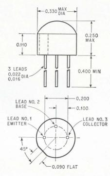
**Circuit designers,** pleased that epoxy packaging cuts the cost of transistors, also want performance that competes with the more expensive encapsulation. One attempt to meet the challenge is a new pnp transistor from the semiconductor division of the Fairchild Camera & Instrument Corp.
