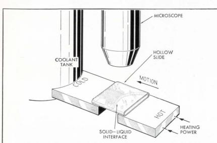
Experimental setup in which photographs such as that below were taken. The glass slide or cell-containing a liquid which freezes like a metal-is placed between hot and cold blocks of brass. This produces a temperature difference along the slide. A solid-liquid interface then forms between the two blocks. By moving the slide toward the cold block at a constant rate, one can observe the steady growth of the crystal under the microscope.
