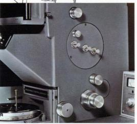
All features you want are built-in, at your fingertips. They can be used while you're comfortably seated. Conveniently reached control zone. Focusable stage.  $.5 \times .3 \times$  zooming variable magnification. Exclusive high-power stereo viewing. Visual observation, projection or photomicrography. Built-in shutter controls. Selector for transposable camera and viewing screen.
