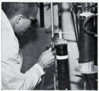
while one half inch away the same quartz tube is cooled by liquid nitrogen to -196°C. In half an inch, G-E fused quartz accepts a temperature gradient of 1994°C. Remember this fantastic capability of G-E quartz as you, in your own field, seek solutions to the uncommon challenge. Circle 575 on reader service card
