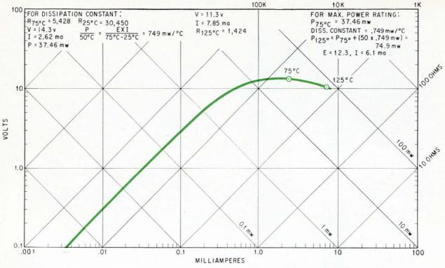
**Typical voltage current** characteristic for a beryllium oxide substrate. Maximum power rating for this unit is 75 milliwatts.
