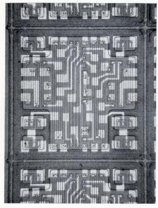
Production dielectrically isolated integrated circuits. The chips were developed from breadboards like this.
