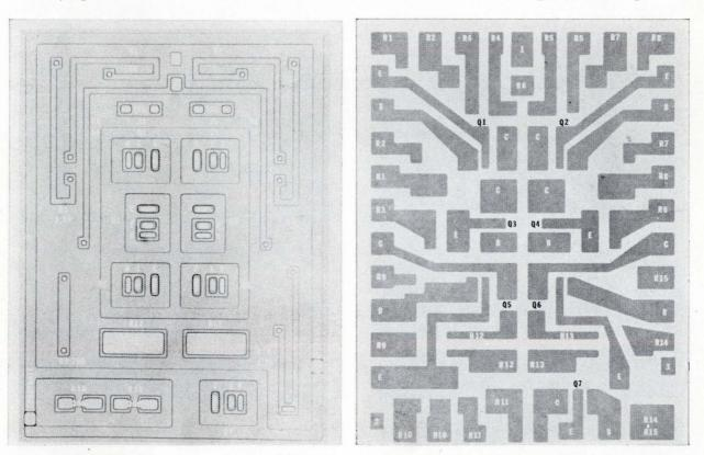
Master dice breadboard has six transistors and 33 resistors varying in value from 75 ohms to 10,000 ohms. Aluminum bonding pads shown in photo at right are connected to each resistor and to the emitter, base, and collector of each transistor.
