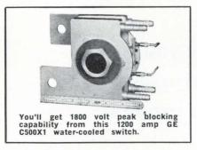
RMS with peak blocking capability to 1800 volts in both directions. Surge ratings are 4000 amperes peak for ten cycles and 7000 amperes for one cycle. The device can be used directly in 440 or 550 volt a-c service. Circle number 811.
