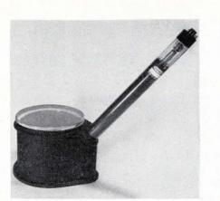
New Raytheon Projectoray\* Tube produces more than double the light output of standard projection-type cathode ray tubes. The tube's light output is 30,000 foot lamberts, which results in a light level of 15-foot lamberts on a 3' x 4' lenticular screen.
