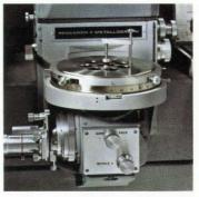
The exclusive Bausch & Lomb Foster Calcite Prism ... your assurance of the finest results in polarized light...also provides vertical illumination for built-in bright field, sensitive tint, phase contrast and high power stereo viewing. A second prism produces an optimum level of dark field illumination.
