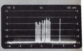
Three L-3 carrier channels shown in 12-kHz sweep width mode: teletype signals on center channel, 2600-Hz ''on hook'' tone on right channel, left channel idle.
