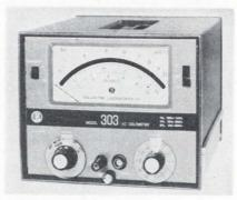
An analog meter capable of measuring a-c voltages from 2 hertz to 6 megahertz will be introduced at the EEE show by Ballantine Laboratories Inc. The company's president, A.W. Parkes Jr. reports it is the first transistorized analog instrument capable of operating at such a low frequency.
