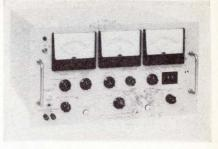
unavailable. Instruments manufactured in Germany cover only portions of the range. Now, a device developed by the Wiltron Co., employs crystal controlled frequency and counter techniques to obtain very stable and accurate time delay measurements. The instrument is specifically designed for delay distortion application.
