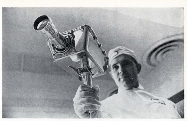
Apollo television camera with telephoto lens attached is held by Westinghouse engineer. Handle also serves as an electrical connector that can be engaged and disengaged without the contacts welding in the moon's vacuum environment. Cable in handle carries d-c voltages to camera and video output to transmitter in the spacecraft. All the electronics are mounted on the top plate. Bottom pan is an enclosure. Thick casing is for protection from meteors.
