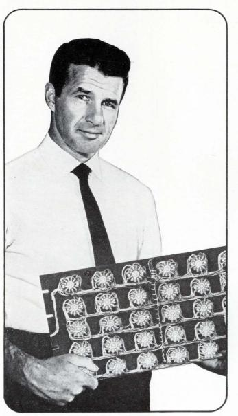
**USING ROTARY SWITCHES** requires 330 soldered joints . . . over 8 hours of labor . . . occupies 293 square inches of panel space . . . costs \$88.00 installed. (*That's* \$0.29 per switching point.)
