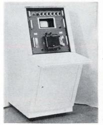
. . from an indium antimonide cell paints a picture with 10 black-to-white ranges on the monitor console's oscilloscope. A built-in Polaroid camera makes a permanent record of the scope's traces.
