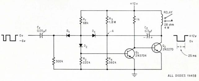
Modified circuit generates a fixed output pulse of 25 milliseconds for each input pulse.
