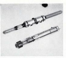
**Recording Storage Tubes.** The miniature tubes shown here are Raytheon's single-gun (CK1516) and dual-gun (CK1519). They provide high resolution, long storage, and fast erase capability.
