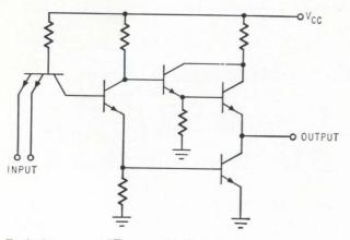
Typical two input TTL gate circuit used in the new high-speed Texas Instruments' Series 54H logic line.
