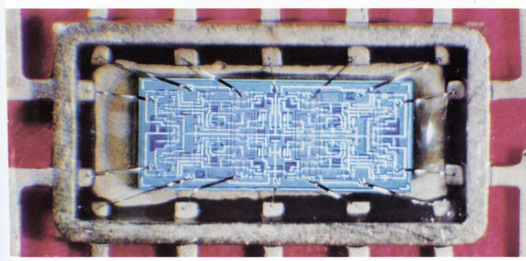
**One of modified-DTL devices** used in Cincinnati Milling Machine numerical control system is this dual J-K flip-flop, part of TI's series 73. Silicon slice contains total of 80 transistors, resistors, and capacitors.
