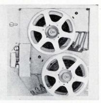
A compact, punched-tape reader and spooler reads 500 characters per second optically, and winds the tape on 10<sup>1</sup>/<sub>2</sub>-inch reels at 50 inches per second. The unit is only 21 inches high.
