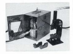
Both the inner and outer shields of multiconductor shielded cable are terminated by a new lightweight crimping tool. The Y40LH 'Hypress
