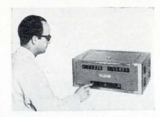
Bidirectional counters furnish accurate, high-speed determination of dimension, travel or position along one or two axes of motion. Primary application is for machine tools, layout and plotting machines and similar equipment where lead screw rotation can be monitored to provide a direct and continuous display between stationary and movable members.
