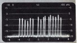
Center channel above expanded to 3.6-kHz sweep width mode: 17 teletype carriers, 1 missing, 2 showing "mark-space" information.
