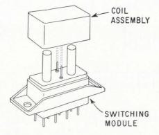
**The organic contaminants** given off by conventional insulators for magnet wires can, if they form a film, interfere with the operation of an electromechanical relay's contacts.
