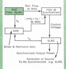
The Type XUC is the only true UHF-Synthesizer. It is the only single instrument to provide output frequencies to 1 GHz with 3V and 80 dB suppression of spurious. Generation of ultra-stable microwave frequencies is simplified and can be accomplished in two ways:
