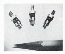
square wave frequencies as high as 40 khz, or even higher sine wave frequencies for new miniature rectifiers. They offer a 9-amp current rating and peak inverse voltage up to 400 v with all models having controlled avalanche characteristics. Surge ratings are as high as 150 amps for one cycle.
