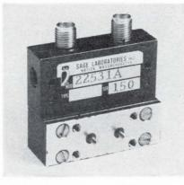
An expanded line of miniature balanced mixers now includes eight models with replaceable diodes. Called the M-LINE the new devices cover 1 to 4 Ghz in two bands. In each band, dual and single i-f outputs are available with ¼-36 connectors or solder lugs.
