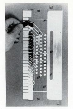
Plating tape is applied behind contacts to form one plating electrode.
