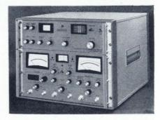
A new test receiver for measuring antenna patterns has taken its cue from sophisticated telemetry gear. The receiver employs coherent conversion techniques and phase locked loops to increase sensitivity by 30 db and improve phase accu-
