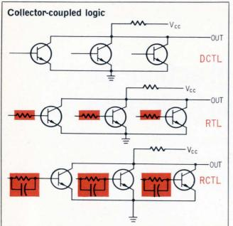
**Collector-coupled** or current-sourcing logic types include, from top to bottom, direct-coupled, resistor-coupled, and resistor-capacitor coupled transistor logic, abbreviated DCTL, RTL, and RCTL, respectively. The resistors in RTL overcome current hogging, while the RC input in RCTL avoids current hogging and, theoretically, improves speed. lithic IC, a separate power supply is used, connected to the bottom of  $R_3$ , to provide turnoff drive at the base of  $Q_1$ .
