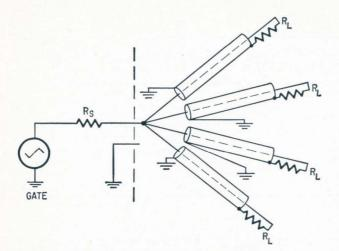
In the radial fan-out method, inputs to the logic circuits must be matched to the transmission line.
