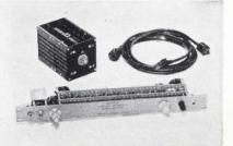
Nine high-gain solid state amplifiers can be used with acoustical instrument systems in the geophysical field and other applications. Series 505 amplifiers feature a wide dynamic range of 60 db which allows reception of greatly attenuated signals. The units can also handle large signals (200% overload) without blocking.
