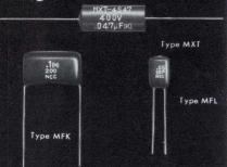
POLYESTER FILM CAPACITORS. Type MXT In Plastic Tube. Capacitance Range : .001 MFD to .22 MFD. Voltages : 100v, 200v, 400v, 600v DC. Type MFK Dipped Flat Shape. NOn-Inductive Construction Capacitance Range : .01 MFD to .22 MFD. Voltages : 100v, 200v, 400v, 600v DC. Type MFL **Dipped Flat Shape** Capacitance Range : .001 MFD to .47 MFD. Voltages : 35v, 50v, 100v, 200v, DC.
