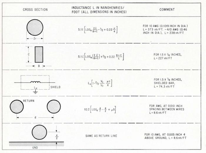
**Specific transmission** line formats will yield these values of inductance per foot. In the last six cases in the table,  $\mu$  is assumed to be that of air, and no fringing is assumed.
