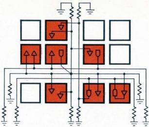
In this example of tree method, one gate is seen to drive both horizontal and vertical lines fanning out to flatpacks. All lines are terminated in characteristic impedance.
