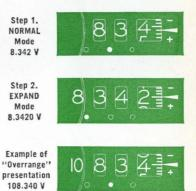
Note these other interesting features of the new 353: a left-to-right digital readout; an automatic display of "mV" or "V"; proper placement of the decimal point; 10 megohms input resistance; an automatic disabling of the motor during the "expand" dialing; a red light to indicate overrange or wrong polarity; and provision for a foot-operated switch for a "read" or "hold" function.
