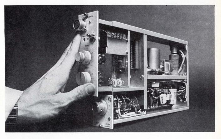
Record directly...strain...pressure...displacement... temperature...or any other phenomena that can be transduced into an electrical signal. The Beckman 9800 Series Input Couplers (over 30 of them) plug directly into the preamplifier in the Dynograph<sup>®</sup> Recorder, averting heavy expenditures for specialized amplifier systems when your application needs change.
