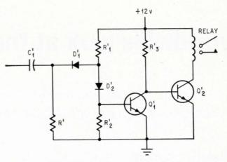
**Conventional high-gain** pulse amplifier generates output pulses whose duration is determined by the time and amplitude of input pulses together with time constant  $R'_{a}C'_{1}$ .
