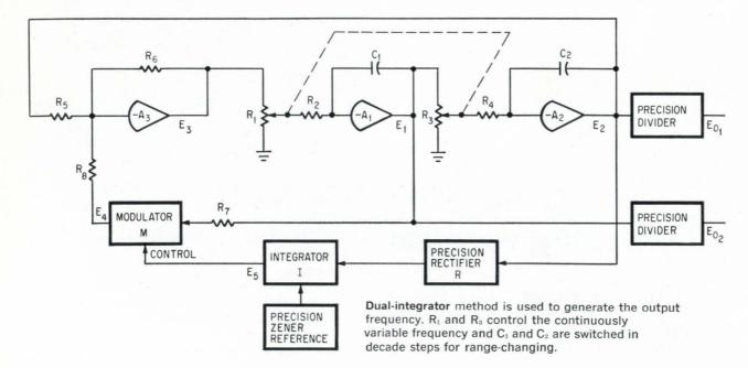
output dividers to provide flexibility when using the instrument in both one-and two-phase applications.
