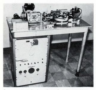
**Tape control unit** fits beneath a coil winding machine, and sequences any number of winding operations while controlling auxiliary assembly and test functions as well. dle all of the operations required for automatic assembly and testing of coils. It can be used with any of the company's standard turret-transfer coil winding machines.
