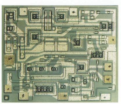
**Modified-DTL**, in which input diodes are replaced by transistors, forms the output of this monolithic sense amplifier. Built by Motorola Semiconductor for 0.5  $\mu$ sec-cycle core memories, its high and low output levels are 5.9 volts and 0.35 volts, respectively.
