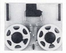
cuit holds the output transistor switches closed until the tape is positioned for reading the next frame. This eliminates all off time during tape advance. The reader retains information from the last frame while it is advancing the tape to the next frame. Updating to the new frame is instantaneous.
