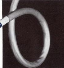
This multiple pair, Beldfoil shielded cable is typical of the types of Belden cable used in recording critical measurements on the Goldstone tracking antenna.
