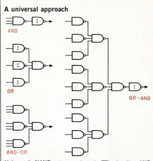
**Using only NAND** gates, such as in TTL circuitry, AND gate, OR gate, AND-OR, and OR-AND can be produced. For the AND, a NAND is followed by an inverter; in the OR, inverters precede a NAND; and AND-OR is made up entirely of NAND's; and the OR-AND is three stages of NAND's followed by an inverter.
