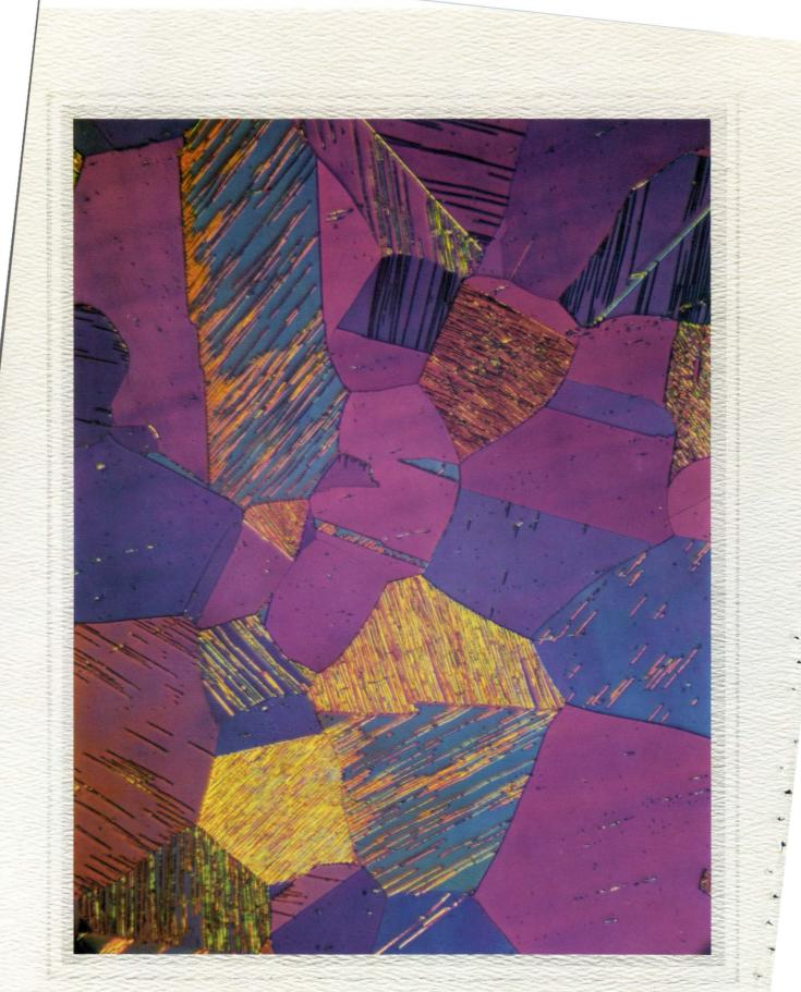
Specimen: Austenite (6% manganese, 1% carbon, 93% iron). Rolled, quenched in brine from 2000°F. Etched with Vilella's reagent. Original magnification:  $100 \times .$
