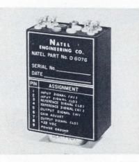
A miniature, solid state a-c amplifier-demodulator performs in extreme operational environments with the accuracy of laboratorytype instruments. It weighs less than 6 oz and occupies only 2.5 cu in. The unit operates either as an a-c to d-c converter or as a phasesensitive synchronous detector for gyros, synchros, and linear variable differential transformers.
