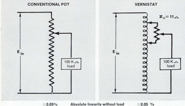
0.60% ±0.65% Load error Absolute linearity with load ±0.05 % 0.011% ±0.061%
