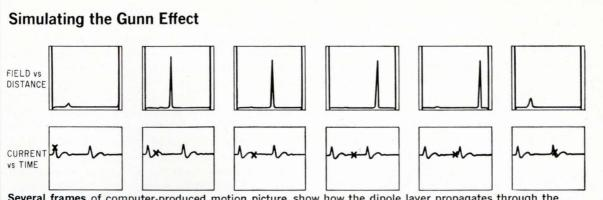
Several frames of computer-produced motion picture show how the dipole layer propagates through the sample after being nucleated at a point where the doping is 10% lower than the doping throughout the rest of the sample. The X's on the current curve show the current at the instant which is pictured in the field distribution plot. The time between frames is about 0.6 nanosecond. The repetition frequency is 680 megahertz.
