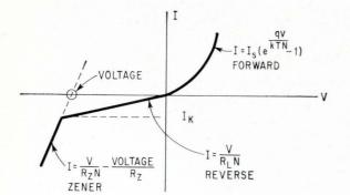
**Typical characteristic** current versus voltage curve for a zener diode. Plot is broken into three parts with each part represented by an appropriate current-voltage equation.
