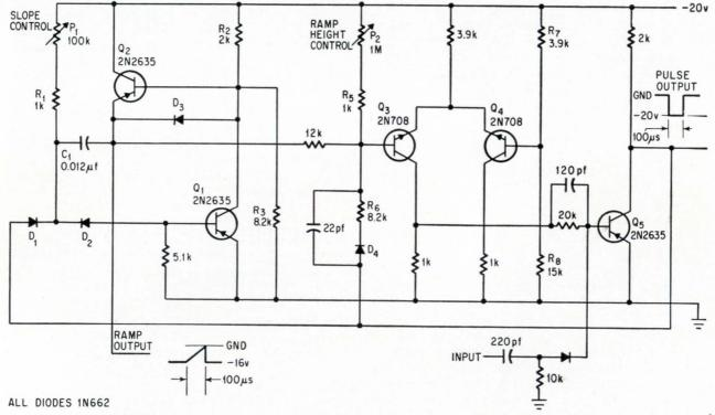
**Transistors Q**<sub>1</sub> and **Q**<sub>2</sub>, together with P<sub>1</sub>, R<sub>1</sub>, C<sub>1</sub> and associated components, make up the Miller-effect ramp generator. The remainder of the circuit, including Q<sub>3</sub>, Q<sub>4</sub>, and Q<sub>5</sub>, is a differential Schmitt trigger that can terminate the ramp at any point.
