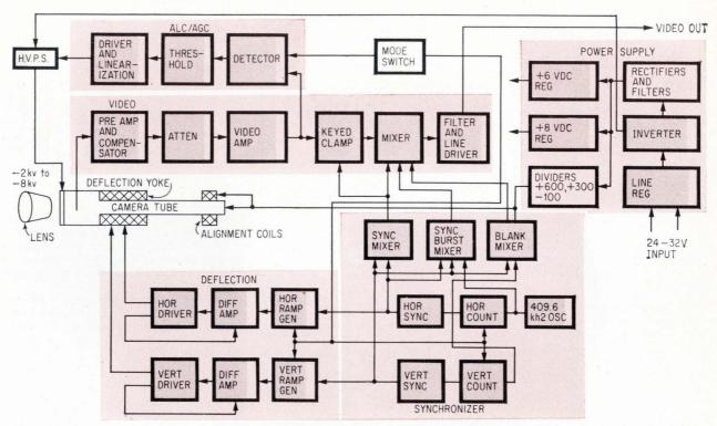
**Camera's five major sections** are shown in color in the block diagram above. Shaded portions indicate the percentage of integrated circuitry. Deflection circuits generate the waveforms to scan the tube. Camera's signal is controlled by the automatic light control and automatic gain control (ALC/AGC) circuit. Video signal is fed to S-band transmitter after amplification and mixing with synchronizing and blanking signals.
