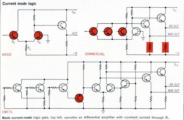
Basic current-mode logic gate, top left, operates as differential amplifier with constant current through R<sub>1</sub>. At the top right, commercial version has emitter-coupled input gate. Added emitter-follower stage provides inverted (NOR) output. Logic swing is boosted in the bottom circuit, current-mode complementary transistor logic, CMCTL, and only one supply voltage is needed, through the use of pnp transistor.
