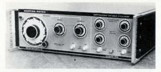
Precision oscillator provides continuously variable frequency output while maintaining the output voltage constant within  $\pm 0.01\%$  over the range. The frequency range is indicated by the multiplier dial to the right of the larger dial, which is coupled to the range-changing system.
