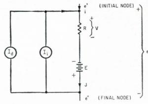
A circuit branch is defined from the initial node to the final node with each branch containing a nonzero R-parameter. The dependent current source is represented by  $I_d$  and  $I_1$  is the independent current source.
