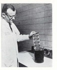
mixtures of high-purity organic solvents and activating ingredients. The nonflammable liquids remove resist films quickly and completely without causing damage to delicate surfaces.
