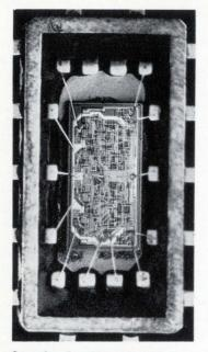
**Complex functions** like this will be part of the Series 54 line. First product will be a quadruple binary latching circuit with four flip flops on a chip.
