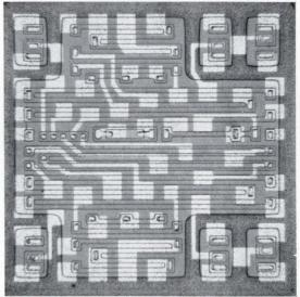
The shortest route to a new IC is Norden's Master Dice Breadboard technique. Each Master Dice contains all the elements, in monolithic integrated form, to perform a variety of analog and digital functions. All you do is tell us your circuit requirements, and we ship you an IC stitched to your specifications. *Glastrate* dielectric isolation of active elements is built in, insuring high performance.
