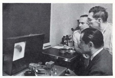
**Researchers study** X-ray motion picture taken with new Picker equipment. Image, of main trunk of a coronary artery, is magnified three times (photo on left). Top photo shows same section enlarged only  $1\frac{1}{2}$  times, the best that could be achieved previously.
