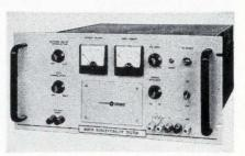
modulation-modes-random Two noise and external input-are available in a solid state 5 amp d-c power source that has output voltage adjustable from 18 to 37 v. The instrument is designed for electromagnetic compatibility testing and can simulate abnormal power supply conditions for checking equipment performance.
