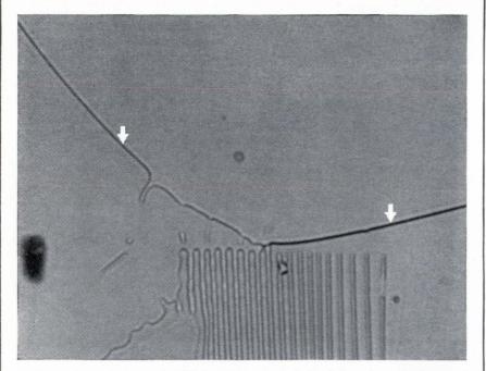
Bell Laboratories' model (200x) permits physical simulation of a <u>eutectic phase</u> <u>diagram</u> for an alloy such as lead-tin. Diagram relates liquid proportions (horizontal scale) to temperature (vertical).
