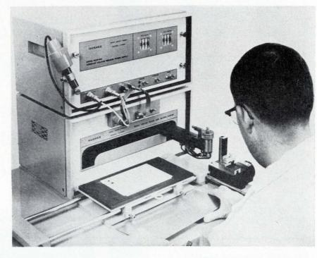
Machines that automatically feed and place flatpacks on printed circuit boards haven't panned out, largely because girls with tweezers excel at gently handling the fragile IC packages.
