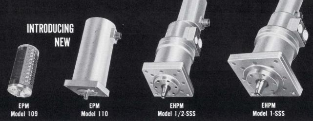
Electric Pulse Motors (EPM's) Models 109, 110 and 111 are stepper motors of excellent gualifications based on originality of both construction and drive circuit. In particular, newly introduced Models 110 and 111 feature large output torque sufficient to directly drive small size machine tools, various machines with relatively small load, etc.
