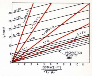
Trade off between system logic delay,  $t_p$ , and interconnection lengths between IC's. Delay resulting from IC is  $t_e$ , while delay caused by the interconnecting media is  $t_1$ . The line lengths are normalized for relative permittivity and permeability of unity.
