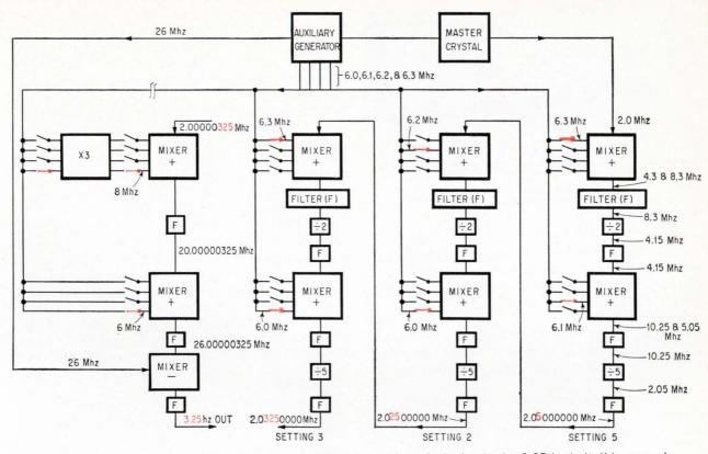
**Decade modules** mix signals produced by crystal oscillator to produce desired output—3.25 hertz in this example. Selecting the desired frequency closes various switch-contacts to feed the proper slave frequencies into mixer. Decimal portion (in color) of each decade's output is shifted one digit to the right as it progresses.
