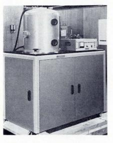
A fully automatic high-vacuum evaporator for producing thin film components can reach to pressures of less than  $5 \ge 10^{-8}$  torr in a 20-inch diameter bell jar. Fast cycling time is achieved with liquid nitrogen and a 1900-liters-per-second oil diffusion pumping system. The pumping system is made fail-safe with an interlocked automatic valve control.
