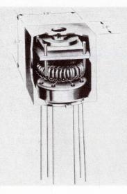
Typical of a line of miniature LC circuits is this phase detector packaged in a square can—3/8 in. square and 1/2 in. high—mounted on a standard 6-pin, TO-5 glassto-metal-sealed header. A recent application has been in a monopulse radar system for weapons control, in which it detects the output phase difference between two 60-Mhz input signals emitted from an i-f amplifier.
