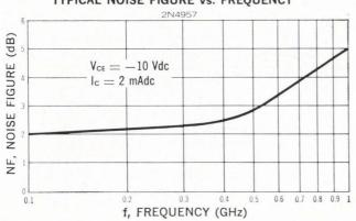
**TYPICAL NOISE FIGURE vs. FREQUENCY**
