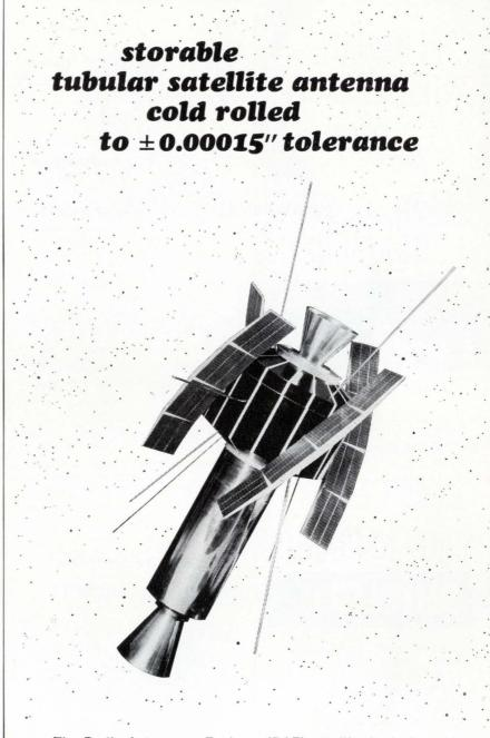
The Radio Astronomy Explorer (RAE) satellite is designed to give NASA an electronic map of the galaxy. Four reel-stored antennae of the RAE satellite consist of 2-in.-wide beryllium-copper strips over a tenth of a mile long. These antennae are made with furled metal strip produced by Hamilton Precision Metals, rolled to a thickness of 0.002'' and held to a tolerance of  $\pm 0.00015''$ .
