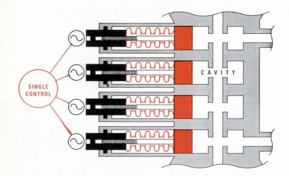
The secret of remarkable tunability for communication klystrons is Sperry's exclusive bellows-type tuner. Replacing the old-fashioned, short-life diaphragm, the bellows gives you longer tuner life and greater
