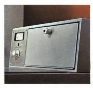
An integral exposure meter removes guesswork—lets you turn every film into a properly exposed photomicrograph with optimum contrast, high resolution. Within arm's reach is the built-in desiccator cabinet—a moisture-free area for safe storage of normal size and most frequently used specimens.
