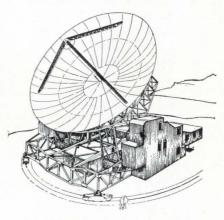
**British dish.** To tie into the Intelsat 3 satellite system, Goonhilly Downs ground station in Cornwall next year will have a new terminal with a 90-foot diameter stainless steel antenna.
