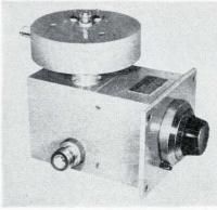
Designed for telemetry and general receiver applications, an integrated package contains a preselector, balanced mixer, and an adder network. It can also monitor individual crystal current.
