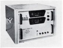
An automatic test set makes possible accurate measurement and visual readout of transfer time and bounce time of electromechanical relays. The equipment offers a clearly visible, in-line decimal readout in milliseconds of operate time (or release time) and bounce on two separate displays.
