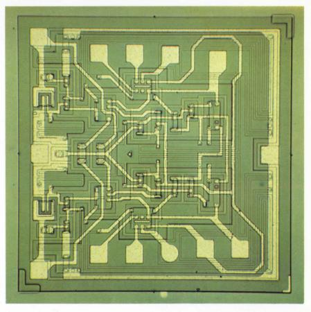
Master-slave flip-flop in new lowpower TTL line, series 54L, will be introduced by Texas Instruments at the IEEE show and convention.
