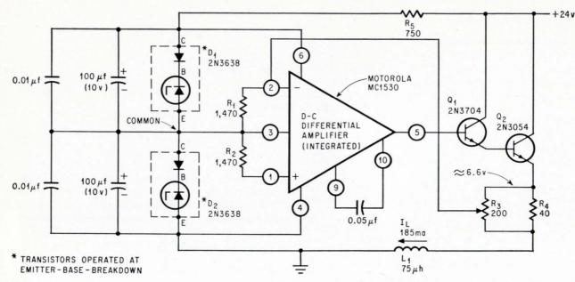
**Rising load current**,  $I_{L_r}$  raises the potential at pin 2 of the integrated amplifier. Pin 2 is the inverting input, so the higher voltage decreases the base current to transistors  $Q_1$  and  $Q_2$ , reducing  $I_{L_r}$ .
