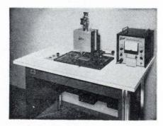
Joining flatpacks to p-c boards becomes a quick and easy operation with a semiautomatic solder reflow machine. It is designed for medium
