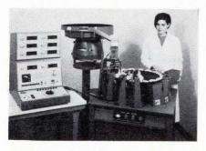
Testing and classifying diodes and rectifiers on production lines and at incoming inspection stations is done with a family of instruments. Designed for application with fast
