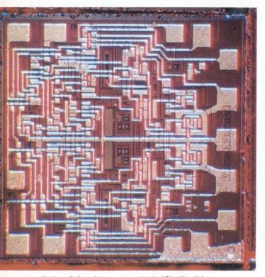
**Rules of thumb** in custom logic IC's like this one from Fairchild are: maximize functional circuits per unit area, minimize separate isolation areas, and use transistors in preference to passive elements.
