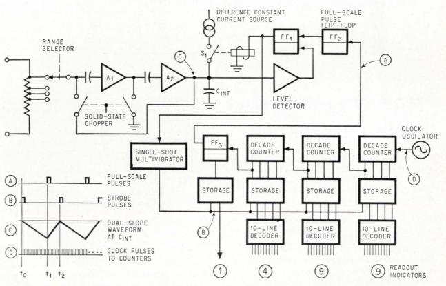
To measure voltage, multimeter measures the time required for the constant-current reference to discharge the integrating capacitor to zero volts after it has been charged to an initial value by an input voltage. The level detector senses the moment when  $C_{\rm int}$  reaches zero volts and generates a strobe pulse to transfer the count from the counters to the readout and restart the measurement cycle.
