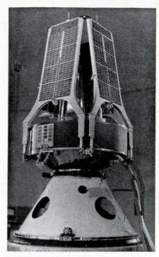
Folded solar-cell panels on all-French satellite D-1A open out when spacecraft goes into spin-stabilized orbit. Cone-shaped structure below satellite is instrument package for trajectory data telemetering, separates from satellite 13 minutes after lift-off.
