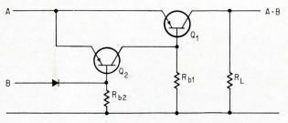
Signal-powered AND gate needs signal B to take  $Q_2$  out of saturation, which permits  $Q_1$  to saturate and allows signal A to pass to output.
