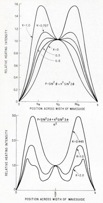
among the various modes. Such calculations can be made if two conditions are assumed; that the load has uniform predictable boundaries and that all of its properties are isotropic and independent of temperature.
