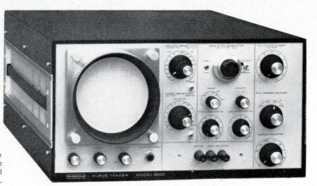
Calibrated controls beside curve-tracer screen provide unambigµous readout of vertical and horizontal sensitivity. Fairchild's tracer can be operated under test in a pulsed condition. Power devices can therefore be tested without dissipating excessive power since the duty cycle is about 10%. Also, elaborate heat sinks are not required to test power transistors in this way.
