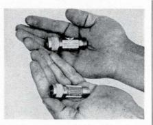
A series of fixed coaxial attenuators, with either 10 or 20 db nominal value, are substantially flat in attenuation vs frequency characteristic from d-c to 12.4 Gc. Model 8491A attenuators are individually swept-frequency tested for attenuation and swr. Exact attenuation at 0, 4, 8, and 12.4 Gc is recorded on the label. Accuracy of attenuator
