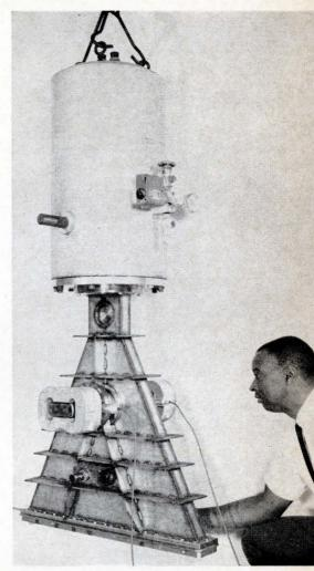
Ford physicist Allen Turner makes adjustment on electron-beam gun developed by company to cure paint on wood, metal and plastic. The process may be adapted for producing printedcircuit boards and multilayer boards.
