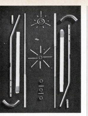
Some electronic parts such as cathode sleeves can be made only from thin-wall tubing. Other parts such as contact fingers for RF connectors may be machined from bar stock, but it is faster and cheaper to fabricate them to specification from thin-wall tubing.
