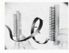
A thin, flexible, ribbon-like laminar busbar named Flexi-bar can be formed, twisted and bent to fit the requirements of electronic rack equipment circuitry. It has the ability to interconnect nonsymmetrical terminations and relieve the tolerance assemblage buildup of rack and panel connectors.
