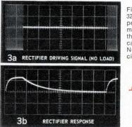
Figure 3a shows a 10-kHz tone burst of 32-cycle duration. Scope scales are 2 V per major vertical division and 2 ms per major horizontal division. Figure 3b shows the resulting output waveform across the capacitor. Scope scales remain the same. Note how easily the time constants of the circuit can be determined.
