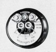
Model 705 Sensitrol—highly sensitive; surface or flush mounted; single or double, fixed or adjustable contact; ranges as low as 0.5-0-0.5  $\mu a$ .
