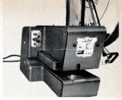
Automatic machines can stake contacts to printed circuit boards at rates of up to 1800 an hour
