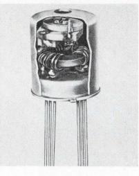
Series MTLC tunable circuits are complete networks housed in a TO-5 outline enclosure. Typically, these miniature circuits consist of toroidal transformer, a Modutrim variable ceramic capacitor, and Uniceram fixed ceramic capacitor all within the same enclosure.
