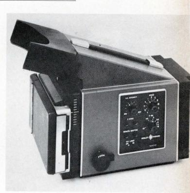
Timing circuits of camera can vary shutter action throughout range of speeds in oscilloscope work.
