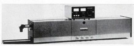
Molecular gas laser with continuous-wave infrared output has a variety of potential applications, including welding, surgery and communications.
