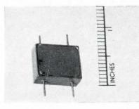
The QHM series of microminiature quadrature hybrid couplers is designed for use with high-density electronic equipment or plugged
