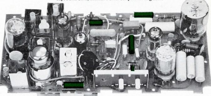
The new Admiral "Playmate" is America's first 9" portable TV with a tube chassis. It weighs only 12 pounds because components were selected not only for reliability, but also for savings in size and weight. That's why Admiral Corporation chose capacitors of MYLAR\*polyester film.
