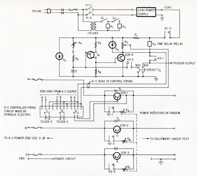
**Resistor R**<sub>1</sub> is varied to change the voltage-dip duration. The three SCR's, SCR-1, 2 and 3, are turned off to achieve a 100% dip while the resistors,  $R_A$ ,  $R_B$  and  $R_c$ , can be switched into the circuit to attenuate the dip's magnitude.
