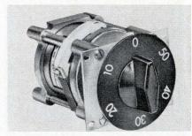
For the frequency range from d-c through 1,200 Mc and attenuation between zero and 50 db, this line of precision turret attenuators offers electrical characteristics of pull-and-turn attenuators three times their price, according to the manufacturer. An important packaging consideration for the design engineer is that each module occupies less than a 3-in.-cube space on an equipment rack or in a testunit chassis.
