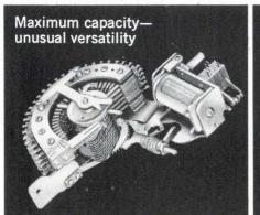
TYPE 45 ROTARY STEPPING SWITCH. Larger capacity: up to twelve 25-point levels, eight 50-point levels. For any DC voltage up to 110, or 115 volts AC with rectifier. Can be impulsecontrolled or self-interrupted. Available with normally open or normally closed circuits (Type 45NC). Also available as prewired, hermetically sealed units.
