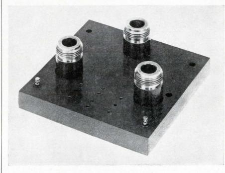
A coaxial diode switch, originally developed on special order for a customer building an airborne identification-friend-or-foe system, is now being marketed commercially. Microwave Associates, Inc., has designated the eight-ounce switch type MA-8306-2L21N and claim it can handle more power than any other switch of the same size and operating at the same frequency.
