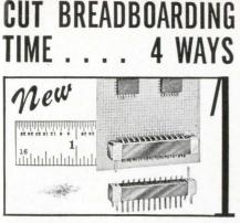
New MICRO PLUGBORDS with subminiature connectors. The .042'' or .025'' dia. holes on .1'' or .05'' centers allow greater packaging density than possible before with prepunched boards. Available also without connectors and in copper clad epoxy glass.
