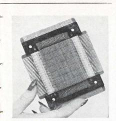
Scratch-pad memory for Gamma 140/ 141 computers uses Permalloy-plated wires as magnetic elements, woven wires for the matrix.
