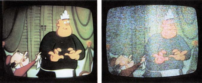
**CATV** system feeding a tv receiver in a poor reception area provides an excellent color signal (left) while high-gain outdoor antenna feeding an identical tv set in the same room produces a noisy picture.
