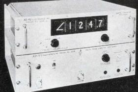
Type 524A2 with indicator. Computer alone (bottom panel) can produce analog output to drive recorder and d.c. digital voltmeter. Price \$965.
