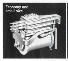
CLASS Z RELAY. Small and lightweight, but designed for service where flexibility is most important. Provides adequate coil volume to permit slugging for long operate and release timing. Four types for DC, one for AC, and two with snap-action contacts.
