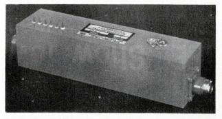
Ferrite phase shifter with reciprocal and latching properties is switched in  $22\frac{1}{2}^{\circ}$  increments by low-power pulses.
