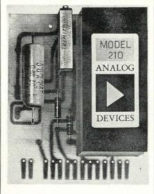
A chopper-stabilized operational amplifier, now available in the same price range as premium differentialtype operational amplifiers, gives an order-of-magnitude voltage-drift improvement and two orders-ofmagnitude better current-drift performance. (D-c drift determines circuit accuracy, establishes the smallest input signals that can be resolved).
