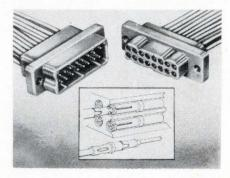
Quadricon connectors, available with rectangular or trapezoidal mating arrangements, provide MIL performance at commercial prices. They offer the reliability of a onepiece insulator, the convenience of crimp-on snap-in contacts, and the economy of a one-piece insulator that requires no shells, brackets, or other mounting hardware. Performance characteristics include low-insertion force, low-contact resistance, high current and voltage ratings and high-insulation resistance.
