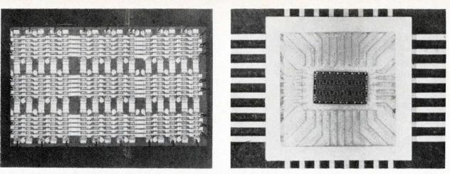
Array of identical diodes gives multifunction capability to integrated circuit. Left photo shows 225-diode matrix in unpackaged detail. At right, it is housed in 32-lead flatpack.
