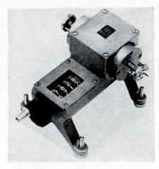
Series 528 direct-reading phase shifter is available in the standard waveguide bands from 12.4 to 110 Gc. This precision instrument, with integral stand and adjustable legs, consists of two quarter-wave plates separated by a rotary halfwave plate in circular waveguide. Rotation of the center section produces a phase shift equal to twice the angle of rotation.
