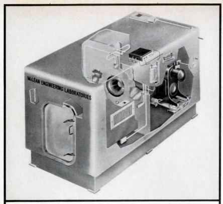
Come in and use any of McLean's modern "lab" facilities any time! They're at your disposal without cost. This Air Flow Test Chamber, for instance, is for new product development and quality control and testing. Provides sure knowledge of pressure drop and air flow requirements to cool specific loads.
