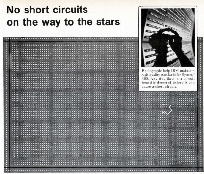
Although it is too small to be seen in this reproduction, the original radiograph revealed a tiny imperfection (arrow) in the circuit board. The radiograph thus served as a guide for repair and saved rejection of the entire costly board.
