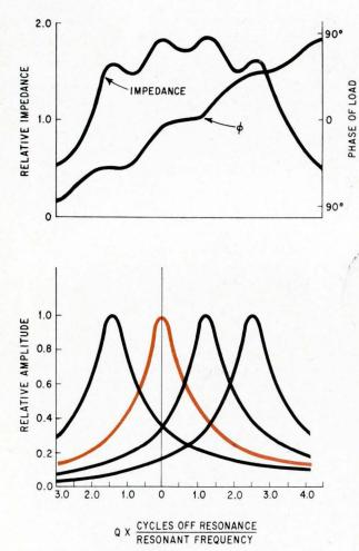
Adding universal response curves of several cavity resonances vectorially, lower sketch, results in a smoother conductance curve, top, which is the frequency characteristics of the cavity.
