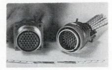
A Class K connector has been developed that is capable of withstanding MIL-C-26500 environments, in addition to meeting flame requirements of MIL-C-5015. The series 238 connectors are for use in missiles, ground support equipment and engine firewalls in high performance jet aircraft. The new K units will also withstand short time exposures up to 800°C, thermal shock cycling from -55° to 260°C and are resistant to moisture, ozone and corrosion type environments.
