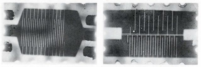
Thin-film resistors of the type made at the VEB Ceramics Works in Hermsdorf. Film with a resistivity of 300 ohms per square has been scribed to form a 100,000-ohm resistor (left). The two resistors at the right have values of 5,000 and 50,000 ohms and were cut from 200-ohm film. The lines, scribed with an electron beam, are 30 microns wide.
