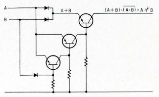
**Exclusive OR gate** is one of the many complex logic circuits that can be built with transistors operating in the common-base configuration.
