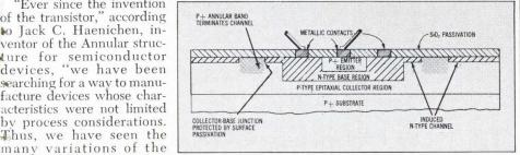
**PNP Annular Transistor Structure**
