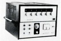
Model AV10 a-c voltage standard features a continuously variable internal oscillator with a range of 38 to 11,000 cps. Its output voltage range is 0 to 511.110 volts rms. The unit has a true absolute accuracy, including one-year stability and temperature effects,  $15^{\circ}$  to  $35^{\circ}$ C, of 0.025%. Harmonic distortion is 0.01% and the solid state, modular unit is convection cooled.
