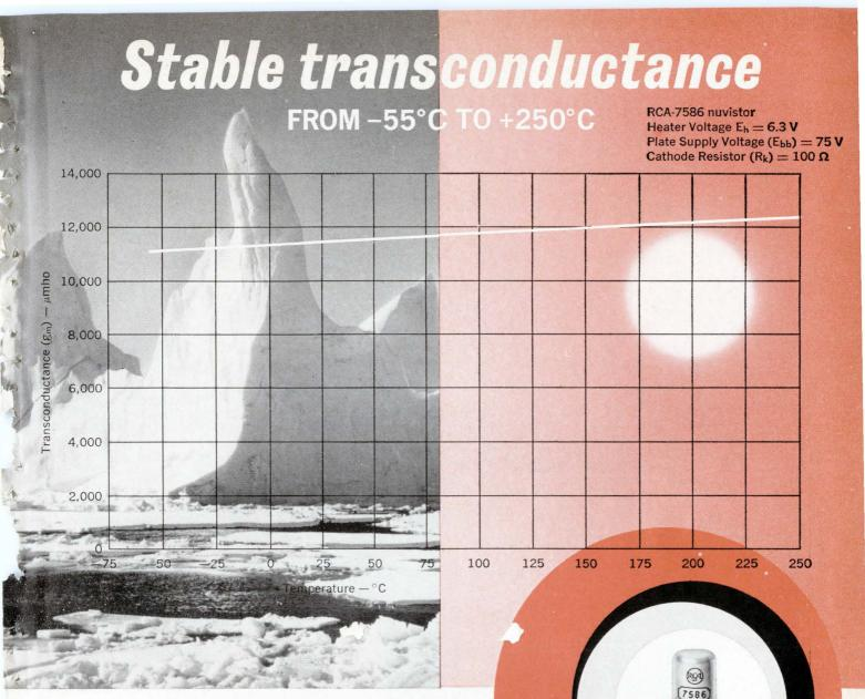
Temperature stability of highly-reliable RCA nuvistors minimizes frequency drift in electronic equipments and permits operation over wider temperature ranges. Change in transconductance per degree change in shell temperature is approximately 4 micromho per degree C.
