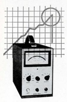
Now you can be specific about the break point in varying voltage, temperature, acceleration, shock pressure, or other quantity being measured. The Model 440A Peak Lok Voltmeter reads and holds the peak signal received over any selected period of time—even pulses shorter than 1 ,us. DC coupling is provided and input ranges are from 0.1 volt to 1000 volts. Output for logging—low impedance 0 to 5 volts with 1% absolute accuracy.
