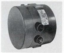
The Duplex Spiral blower provides greater air flow—up to 94 cfm—or greater pressure characteristics up to 2 psig—than the single Spiral blower. It is available in three versions: the SL4 achieves higher pressures by internal ducting of the airflow from the two impellers; the SL5 extends the airflow range; and the SL6 provides an economical source of two independent high pressure air streams, which can be utilized at
