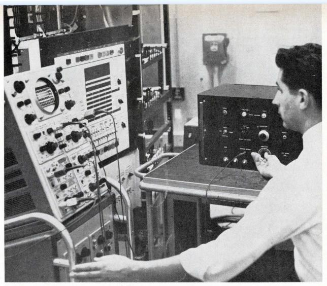
System in the background is subjected to voltage dip from cycle sag simulator, right. The design engineer monitors the simulator's output and a system parameter on oscilloscope.
