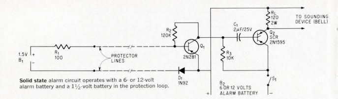
Holding resistor  $R_L$  is required if a conventional alarm bell is used.
