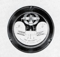
Model 723 Sensitrol—sealed; shielded; internal reset; solder terminals; single or double magnetic contact; ranges as low as 1-0-1  $\mu a$ .
