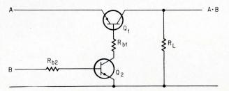
**AND** gate with  $Q_2$  in the base circuit of  $Q_1$  permits a lower voltage at B than at A to function.
