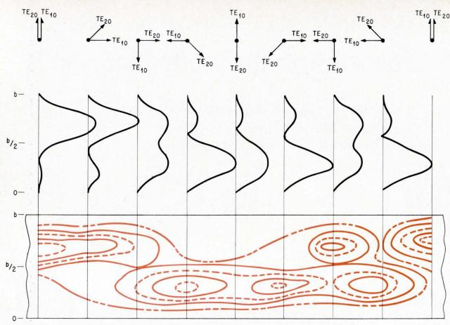
**Development of contours** for the average heating density is shown for a waveguide carrying the  $TE_{10}$  and  $TE_{20}$  modes. Vectors at the top indicate the relative time phase of the two modes in planes perpendicular to the direction of power flow. Heating density (see equation 3) in these planes is shown in center illustration. Contours of equal heating density are shown in bottom drawing.
