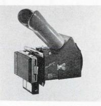
Three new Beattie-Coleman oscilloscope cameras are available. Model MIIA Oscillotron (illustrated) is especially designed for use under severe operating conditions in field test instrumentation. Special locks protect against focus change. An electric shutter permits synchronizing picture with phenomena. It has wide object-to-image recording ratio, 1:1 to 1:05 without special lenses.
