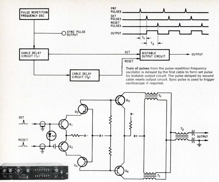
In bistable output circuit, the set and reset pulses are kept from appearing at the output by the differential amplifier, which allows only the difference voltage at the bases of  $Q_1$  and  $Q_2$  to be amplified.
