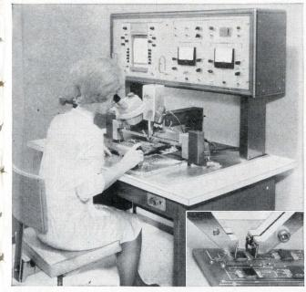
Weltek's new semi-automatic MODEL 900 solders all 14 leads of a flatpack to a p.c. board in just 2 seconds. A proven product, capable of full automation. Send for details.
