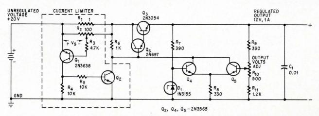
**Current-limiting protection** is added to a series-regulated power supply. The two transistors, shown within the dotted lines, accomplish the protection without degrading the performance of the power supply.
