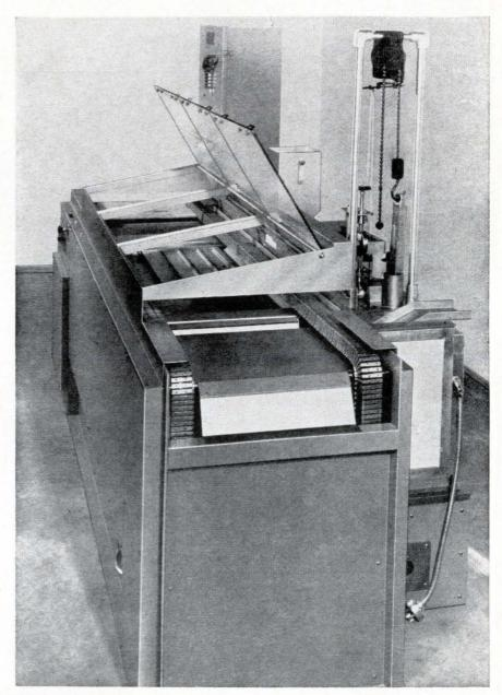
Stainless-steel fingers on wave soldering equipment transport pallets from p-c board assembly line through the wave-soldering process.
