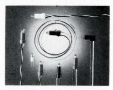
A subminiature incandescent lamp with an integrally molded base, designed for the specific requirements of the computer industry, differs from conventional lamps because it has a nylon base molded to a standard bulb. This replaces not only the separately attached metal base but also the mated socket which it requires.
