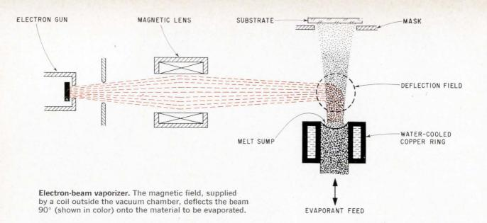
characteristics. An accelerating voltage of 25 to 75 kilovolts is sufficient for thin-film machining. The ability to vary beam characteristics will enable other operations to be performed with the beam.
