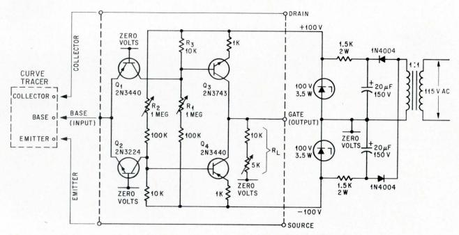
Adapter converts input current steps from curve tracer into output voltage steps for FET gate.
