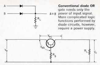
**Transistor in common base configuration** is basic circuit used to perform many logic functions with no power supply. These circuits use only the signal power.
