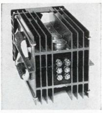
Three basic high-power operational amplifiers are announced. Model OA-111 (illustrated) is an economical high-power operational amplifier with limited frequency response. This basic amplifier module has an output of  $\pm 10$  v with maximum current capabilities of 10 amps. Frequency response is 7.5 kc with a d-c open loop gain of 40,000. Voltage drift is 100  $\mu v$ /hour and peak to peak noise is less than 50  $\mu$ v.
