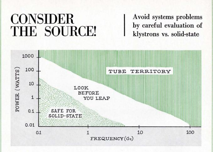
A premature stampede to solid-state for microwave power sources can cause serious problems for system designers. This is the major finding of recent Sperry studies which objectively compared solid-state sources with klystron oscillators.
