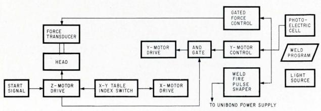
**Pushbutton microwelder** is controlled by an optical reader. A film pattern of the weld locations and the assembly being welded are placed on a table that moves the assembly under the welding head and pauses each time a weld is to be made.
