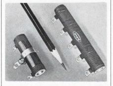
Two commercial resistor styles adjustable and tapped power wirewounds—are now available. The HLA (adjustable) and HLT (tapped) series have the added precision and load-life stability made possible by a multilayer silicone coating. They replace vitreous enamel tapped and adjustable resistors.
