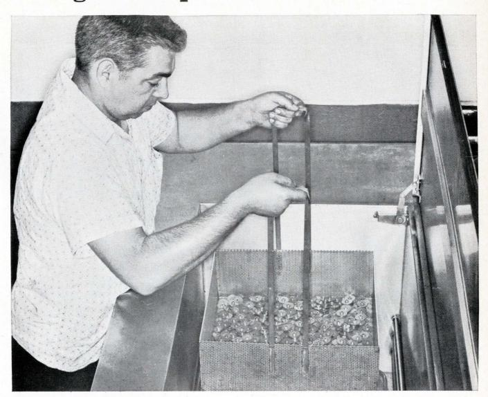
Powder Metal Products, Inc., St. Marys, Pa., makes gears, bushings and bearings for motors in phonograph turntables, car heater fans and other fractional horsepower equipment. All types of soils—even microscopic remnants of grease, oil, ash and metal particles—must be completely removed to insure trouble-free, noiseless operation. Standard degreasing couldn't do the job alone.
