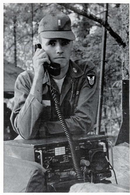
**The war in Vietnam** has created a growing demand for communications equipment such as this AN/VRC-12 jeep-mounted radio being used by the First Air Cavalry Division. Companies making such gear are actively seeking engineers. tickets, open offers, not even a salary decision."
