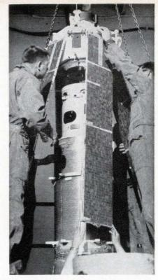
**Navigation Satellite** is attached to the Scout fourth stage for spin-balancing.
