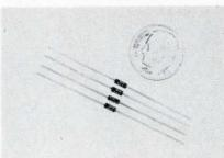
The EE-1/20 precision resistor conforms to all requirements of MIL-R-10509F and MIL-R-55182B, styles RN50 and RNR50, respectively, and features high-density molded environmental protection over a subassembly of rugged cap and lead construction. It measures 0.068 in. in diameter and 0.156 in. in length. Leads, 0.016 in. in diameter and 1 in. in length, are available in tinned copper, gold-plated dumet, or bare nickel.
