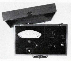
VAW meter is a multirange, multifunction instrument that is moved from the current to voltage mode by a single knob which switches the precision shunt in or out of the circuit. The power measurements are made with both the shunt and multipliers in the circuit; the coil current is proportional to the product of the applied voltage and current.
