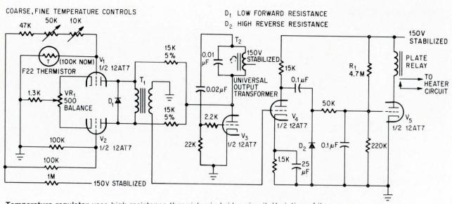
**Temperature regulator** uses high-resistance thermistor in bridge circuit. Variation of its resistance unbalances chopper circuit, generating pulses to control heater circuit.
