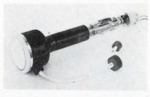
A 3-inch diameter, magnetic deflection, high voltage focus crt is available with over 100 million glass fibers in the useful screen area to carry the light from the phosphor screen to the faceplate surface. Fiber optics insures maximum recording of the crt's light output by direct contact to lightsensitive material.
