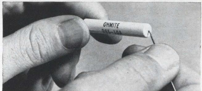
**BEND THE LEAD** at the resistor body! There's no damage. Conventional (dipped) vitreous-enameled resistors have a meniscus at this point which ruptures, damaging the coating. Series 99 (molded) have no meniscus.
