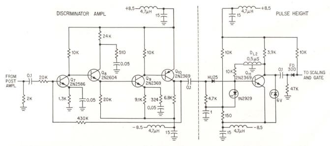
DISCRIMINATOR AMPLIFIER feeds pulse height circuit. Tunnel diode at input to pulse height circuit does not pass small pulses or low level noise—Fig. 4
