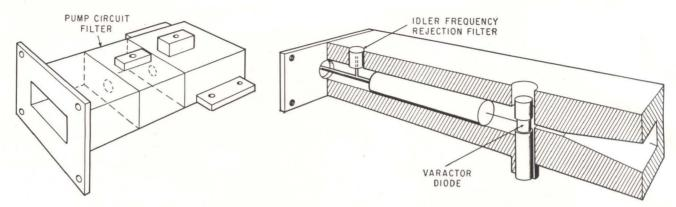
PUMP circuit with isolation filter (left) was necessary to provide isolation within the designed package. Signal circuit with idler rejection filter is shown at right
