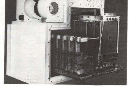
FEEDBOX equipment for operation at 400 Mc
