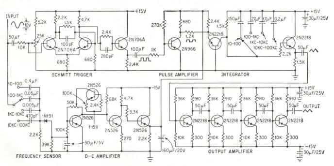
CIRCUIT of the triangular-wave generator uses 14 transistors—Fig. 2
