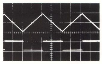
WAVEFORM is measured at the output of the amplifier for 500 cps. Scale is: vertical—5 v per cm and horizontal—500  $\mu$ s per cm—Fig. 4
