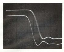
Upper trace shows step response with 100% sampling efficiency; lower with 20%. Rise times are 80 ps and 50 ps, respectively; sweep speed, 50 ps/cm.
