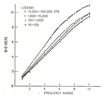
OUTPUT VOLTAGE of the frequency sensor is linear, except at the upper frequency range—Fig.  $\bf 3$
