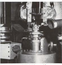
unique 1.2 MW TEST SET is used for high-power rf amplifier test of water-cooled ML-6696. Tests are programmed from remote control console.
