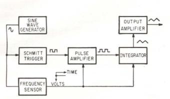
TRIANGULAR-WAVE generator uses a frequency sensing circuit to keep amplitude constant—Fig.  $\bf 1$
