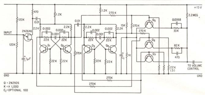
SOLID-STATE stepping switch performs all the functions of a conventional stepping relay using low-cost silicon transistors. The unijunction transistor threshold detector combines the two functions of level detection and trigger pulse generation
