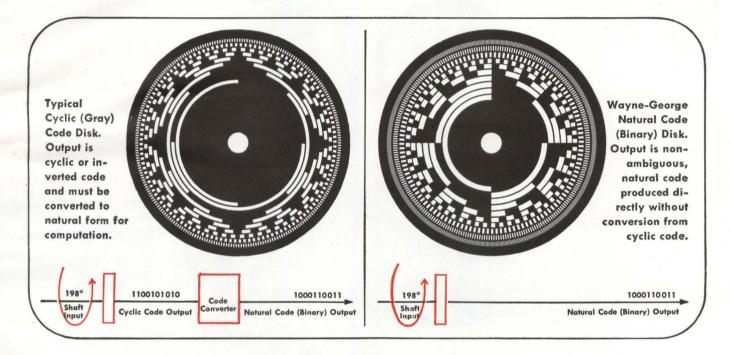
Only Wayne-George offers a complete line of optical shaft-angle encoders providing direct, non-ambiguous natural code outputs without code conversion. The new DIGISEC® and "N" Series DIGISYN® encoders completely obsolete encoders using inverted or cyclic (Gray) codes and their conversion equipment.
