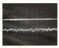
Upper trace shows noise of typical 188A at 10 mv/cm; lower at 1 mv/cm.
