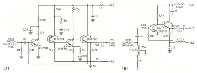
CURRENT PREAMPLIFIER (A) is a-c coupled from multiplier phototube and to following or post amplifier. Feedback holds gain change to  $\pm$  5 percent over temperature range. Post amplifier (B) uses delay line for pulse shaping—Fig. 3
