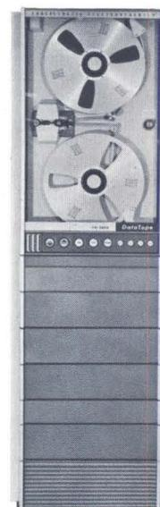
**VR-2800** is a wide band system for use in laboratory environments with Direct and FM electronics. Bandwidth of direct recording/reproducing is 100 cps to 200 kc; 0-20 kc with wide band FM techniques. The full 7- or 14-channel system, with 6 speed operation and plug-in electronics, can be packaged in a single, six-foot EMA cabinet. Bulletin 2800VS.
