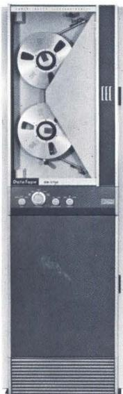
**DR-2700** is a high speed Vacuum-Buffered Digital Magnetic Tape System designed for on-line and off-line digital computer usage. A complete 16-channel digital write and read system can be housed in the unit's 72-inch-high RETMA cabinet. Outstanding reliability has been proven in critical military applications and in IBM compatible installations. Bulletin 2700S.
