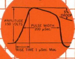
Toroidal pulse transformer, 150 V, 200  $\mu$ Sec. @ 400 PPS. Molded in epoxy, 3 windings, low leakage, less than 1  $\mu$ Sec. rise time;  $-40^{\circ}\text{C}$ . to  $+85^{\circ}\text{C}$ .; output voltage within 1%. MIL-T-27A;  $1\frac{1}{8}$  sq. x  $\frac{3}{4}$ "; 1.5 oz.
