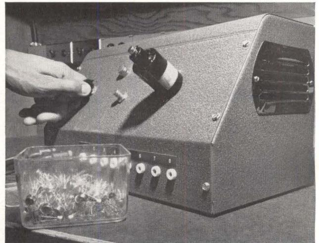
**TESTING** Fairchild designed and built special instruments (shown above) to test electrical performance of the finished units. Samples of each batch are also submitted to Fairchild's environmental quality assurance test programs. Fairchild's Planar\* process results in high, economical yields even after this thorough testing procedure.
