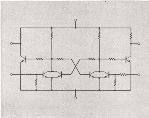
**SCHEMATIC** Engineers at Litton Industries' Guidance and Control Systems Division in Woodland Hills, California, designed this complex toggle circuit for use in the digital computer section of a high reliability control system. Working closely with Fairchild personnel, they learned that their circuit could be mass produced as a microcircuit—completely integrated within a single chip of silicon.
