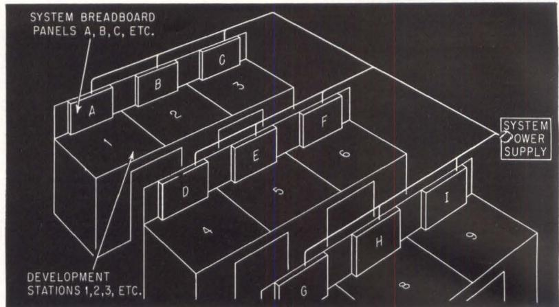
**SYSTEM BREADBOARD** technique uses a common power supply for all breadboards to quickly spot mutually interfering black boxes under development—Fig. 3
