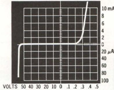
Trace of new GPD-1 shows its extremely low leakage current, sharp breakdown voltage, and low forward voltage drop. GMD-1 planar micro-diode produces identical trace.
