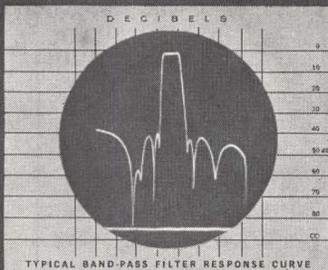
This extremely accurate log amplifier enables exact measurements of attenuation in networks, filters, amplifiers, and other devices exhibiting dynamic operating ranges down to 90 db. Write for complete technical data.
