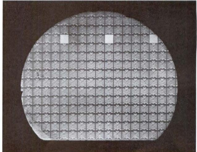
**MULTI-DIFFUSION** Next, the processing of silicon wafers was begun: etching and triple diffusion followed by deposition of the evaporated metal-over-oxide intraconnections\*. Fairchild's Planar\* process was utilized: a protective layer of silicon dioxide is grown into the wafer *before* any junctions are formed. Production begins after several trial diffusion runs in which run-to-run variations of performance parameters are established.
