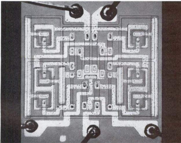
**FIVE WEEK DELIVERY** By December 20, 1962, five weeks after receiving firm specifications, Fairchild delivered an initial shipment to Litton—50 *production* microcircuit toggles—seven weeks before the promised date. The microphotograph above is the finished circuit mounted in a TO-5 can with cap removed. Actual size of the chip is .060" square.
