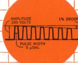
Output to Klystron, 5  $\mu$ Sec. pulses in groups of pulse trains at high rep rate. Droop 1% over pulse trains. 30 KV W.V., 43 KV hipot;  $-53^{\circ}\text{C}$ . to  $+85^{\circ}\text{C}$ .; MIL-T-27A;  $4\frac{1}{4}$  x  $5$  x  $6\frac{3}{4}$ ";  $11\frac{1}{2}$  lbs.
