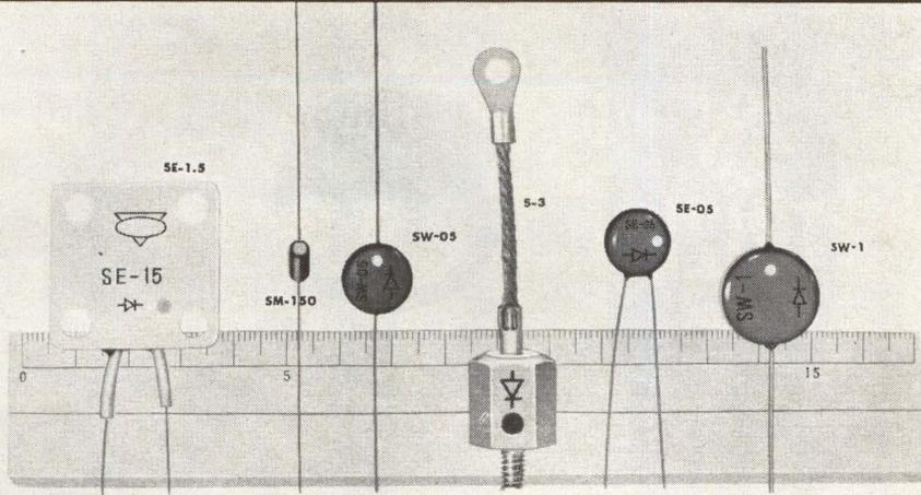
**SE-1.5:** Available in 4 physical configurations. PIV: 400V-1000 Volts. Max. AC input voltages (RMS) of 280, 420, 560 and 700 Volts. Max. Reverse Leakage Current (PIV)  $10\mu\text{A}$ . Max. Average Rectified Current (Single-phase, half-wave) 1.5A. Surge Current (for 1 cycle) 20A.
