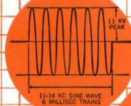
Sonar sine wave pulse output transformer. PP 4-65A's, 11-14 KC flat. Pri. 11 KV; 28 KV hipot. Spark gap protected. Sec. 1500 V. @ 800 $\Omega$ , 60 millsec on, 6% duty cycle. MIL-T-27A;  $-65^{\circ}\text{C}$ . to  $+85^{\circ}\text{C}$ .;  $6$  x  $6$  x  $8\frac{1}{2}$ ", 13 lbs.
