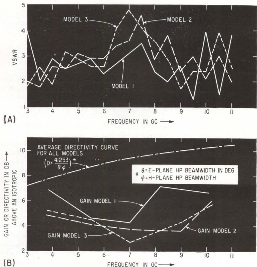
FORWARD GAIN and directivity for all models (A) and plot of vswr for the same three antennas (B)—Fig. 4
