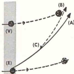
Redirecting vehicle from destination (A) to (B) in vicinity of Venus required flight correction at point (C) by applied jet propulsion of short duration. The vehicle's maneuvers prior to corrective propulsion were based on initial proper sun reference via the photoconductive sun sensors.
