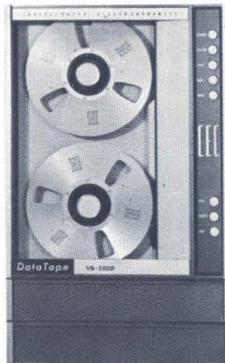
**VR-3300** is a wide band system for use in applications where portability is desirable. Bandwidth of direct recording/reproducing is 100 cps to 200 kc; 0-20 kc with wide band FM techniques — or twice the bandwidth of standard telemetry records. Features include 6 speeds and all solid state electronics. Bulletin 3300VS.
