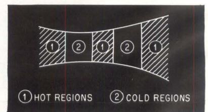
**MHD GENERATOR** suggested by Centre d'Etudes Nucleaires would have heated slugs of gas acting as electrical pistons
