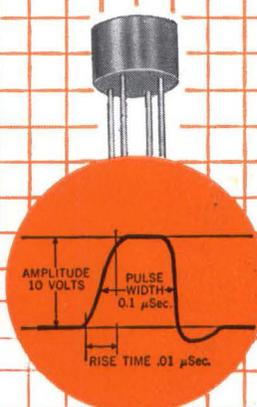
Ferrite core blocking oscillator transformer, 0.1  $\mu$ Sec.  $\pm 10\%$  @ 200 KC PPS. 2 windings, rise time .01  $\mu$ Sec. Epoxy case. MIL-T-27A;  $\frac{1}{16}$  dia. x  $\frac{1}{4}$ ", .07 oz.
