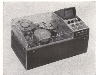
MINIATURE video recorder uses micro-tv set for monitoring. Set, built by Victor Co. of Japan, is for nonbroadcast applications and records 64 minutes on 1,800 feet of 1-inch tape by the two-head method
