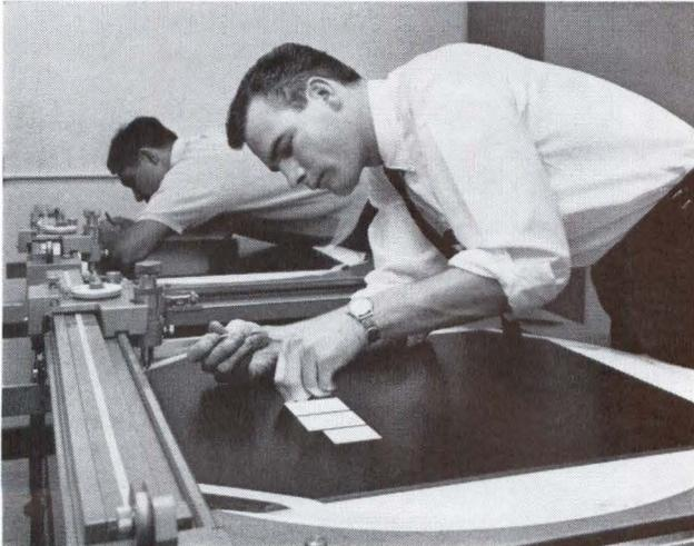
**MASK MAKING** From Litton's pre-tested circuit, Fairchild engineers designed and made the masks used to photo-etch precisely indexed patterns for the multi-diffusion process. Fairchild's highly developed photo-optical techniques are the result of five years experience in producing semiconductor devices, including two years of microcircuit production.
