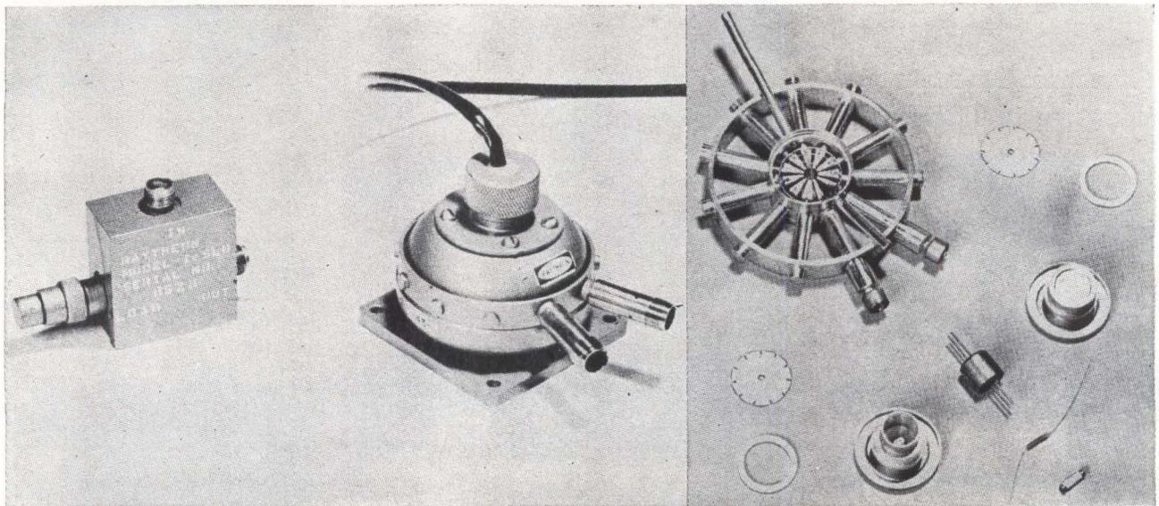
NEW 25-watt c-w S-band Amplitron with companion stripline circulator. Basic anode assembly of QK997 with parts necessary to complete vacuum envelope is shown at right—Fig. 1
