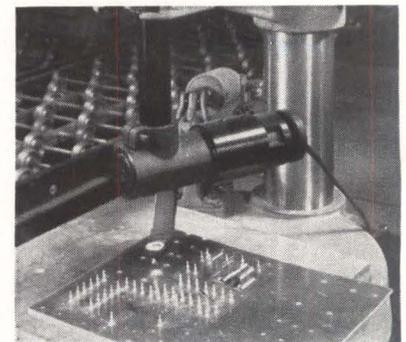
*TERMINAL BOARD just prior to having three target holes located and drilled. Target-hole radius of 0.003 inch is centered by cross-hair reticle in comparator, which is struck by a point of light*
