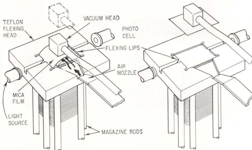
TOP FILM in input magazine is separated from others, after being picked up by vacuum head, using flexing and air blast flutter techniques simultaneously. Light and photo cell are part of system maintaining top of film stack just below flexing lips—Fig. 1
