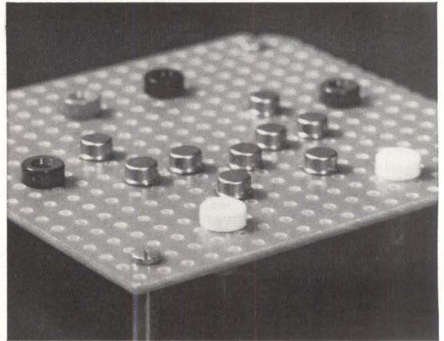
**BREADBOARD** Using microcircuit design components from Fairchild, the Litton project team built a breadboard of the circuit. With this they accurately determined the electrical characteristics of the circuit before committing the single-chip version to production. With design and specifications thoroughly proven, Litton gave Fairchild the production order on November 14, 1962.
