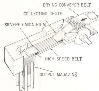
*KINETIC ENERGY imparted to mica films by stacking mechanism overcomes effect of film's light weight and static friction so that films can be uniformly stacked—Fig. 3*
