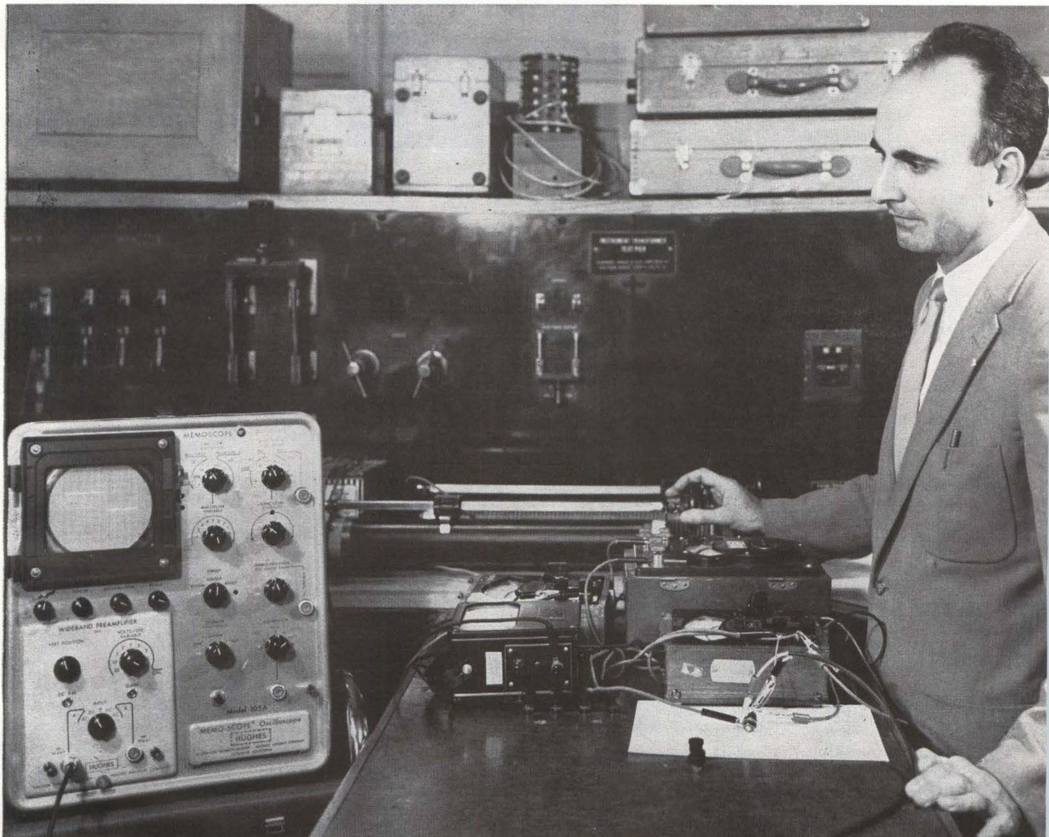
*GATE TURN-OFF switch under test has the same physical configuration as a silicon-controlled rectifier*
