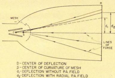
**DEFLECTION** demagnification from a slightly negative spherical mesh makes a new closed-structure crt useful at high frequencies, S. Slade of Hewlett-Packard reported last week at the Cleveland Electronics Conference. Conventional post-accelerator tubes, using bands or helices, trade scan to intensify brightness because of the converging action of the lenses formed. The mesh, followed by a radial field, overcomes this limit at a sacrifice of screen current and some enlargement of spot size
