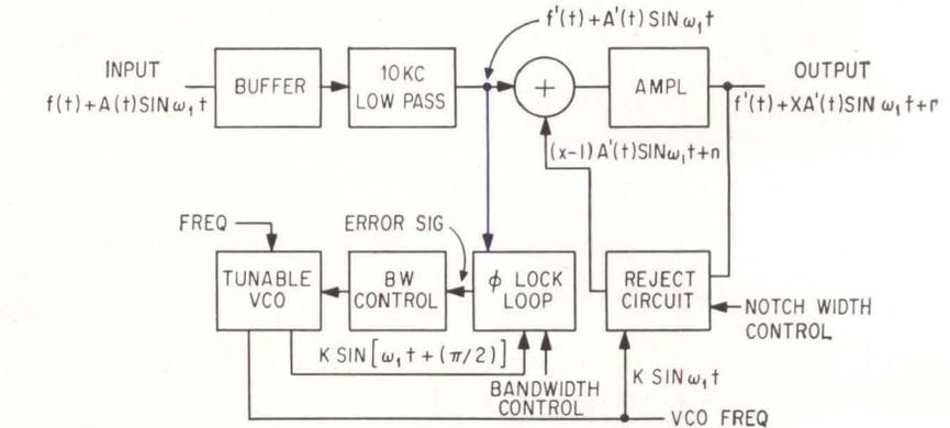
from 5 cps to 5 Kc and notch bandwidth adjustable to more than 30 cps. A simplified block diagram is shown in the sketch. The vco is tuned to the desired rejection frequency and the phase-lock loop acquires the signal. Once locked, the loop generates two sine waves of the frequency to be rejected. These are in quadrature to each other. One
