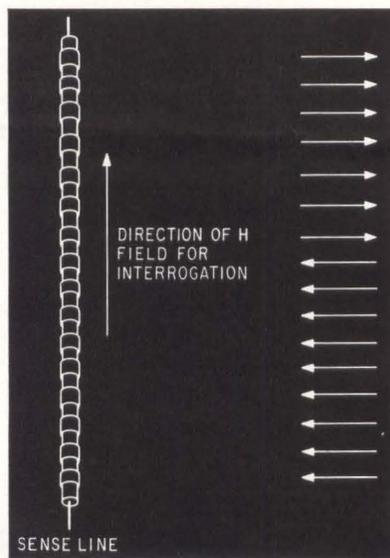
**SELF-ADAPTIVE SYSTEM** described by G. R. Henderson and A. J. MacMillan, of Northrop, uses gain-storage device to weight inputs (top, left). In the two-aperture MAD device (left, center) storage-gain is accomplished by controlling the ratio of set-flux A to blocked flux B and thereby the readable flux available when switching leg C. Next diagrams show a basic thin-film adaptive device and a cylindrical assembly constituting an elemental adaptive system
