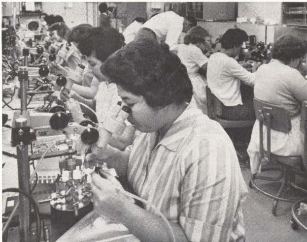
**ASSEMBLY LINE** Final production wafers were then diced to separate individual circuits. A single wafer produces approximately 200 Microcircuits—each incorporating six transistors and 12 resistors. The circuit chips were mounted with leadwires attached, capped and electrically tested in accordance with standard procedure. One of Fairchild's microcircuit production lines was used.
