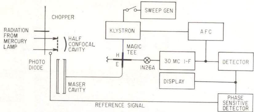
ATTEMPT TO DETECT stimulated emission in far ir of  $10^{-12}$  will be made with ammonia maser oscillator described by D. C. Laine of Keele University, England. If successful next step will be to determine feasibility of device for ultramicrowave oscillator
