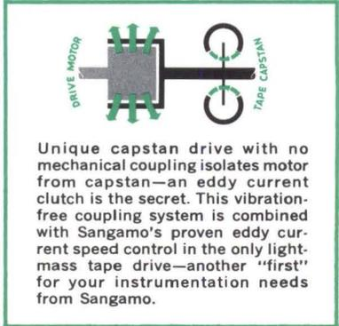
Unique capstan drive with no mechanical coupling isolates motor from capstan—an eddy current clutch is the secret. This vibration-free coupling system is combined with Sangamo's proven eddy current speed control in the only light-mass tape drive—another "first" for your instrumentation needs from Sangamo.
