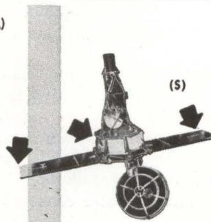
Throughout the life of the craft, prior and subsequent to mid-course correction, the sun sensors (S) signalled error-correcting commands to the stabilization jets for pitch and yaw control, thus keeping the solar cell banks properly oriented for maximum power output.
