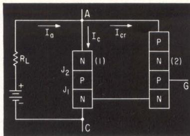
**TURN-OFF GAIN** can be increased by combining the gate turn-off switch with a transistor—Fig. 3
