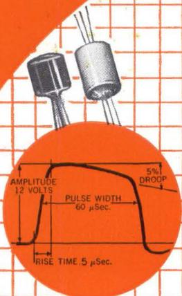
25 KC pulse transformer, DO-T or DI-T configuration. Pulse width 60  $\mu$ Sec. Rise time less than 0.5  $\mu$ Sec. Secondary C.T. balance each side to within 1% to ground. MIL-T-27A, GR 4. Size: DO-T,  $\frac{3}{16}$  dia. x  $\frac{13}{32}$ " wt. 1/10 oz.; DI-T,  $\frac{3}{16}$  dia. x  $\frac{1}{4}$ ", wt. 1/20 oz.
