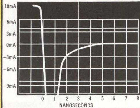
Trace of new high speed GPD-5 shows its very fast recovery. GMD-5 planar micro-diode produces identical trace.
