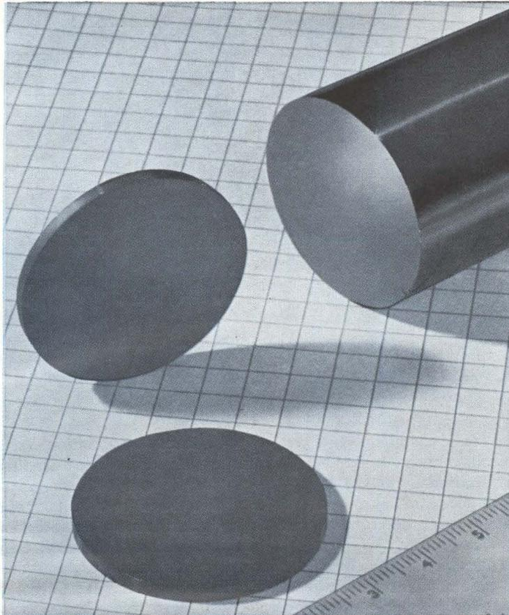
**Now...to help cut your costs, speed production...40 mm dia. float-zoned silicon crystals!**
