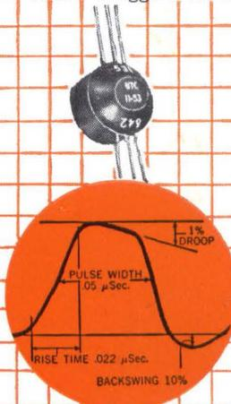
Special precision miniature pulse transformers. Designed in our standard stock mold to your specs. Checked and precisely adjusted in your tube or transistor blocking oscillator circuit. Sizes:  $\frac{3}{8}$  dia. x  $\frac{3}{8}$ ", 1 gram;  $\frac{1}{4}$  dia. x  $\frac{1}{16}$ ", 4 grams;  $\frac{5}{8}$  dia. x  $\frac{3}{8}$ ", 6 grams.
