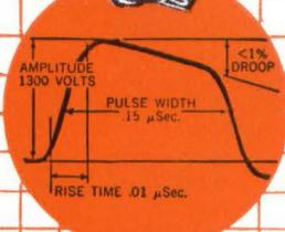
Output to 2J42 magnetron. Input 1300 V-50 ohms. Output 6.5 KV to 1200 ohms and .6A. bifilar filament winding. .15  $\mu$ Sec., 1000 PPS. Trigger winding. MIL-T-27A GR 5;  $1\frac{1}{2}$  x  $2\frac{1}{2}$  x  $2\frac{3}{4}$ ", 10 oz.
