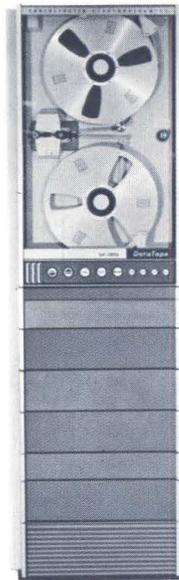
**GR-2800** is solid state, a fully integrated recorder/reproducer system. A single standard 19-inch EMA rack with a 64-inch-high opening contains the complete 14-channel record and reproduce system. The one cabinet can mount 28 amplifiers (operating in Direct, FM or PDM modes), capstan power amplifier, and tape-speed control servo. Direct record response is 100 cps to 100 kc; FM response is 0-10 kc. Bulletin 2800S.
