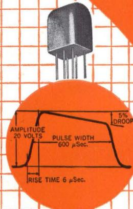
600  $\mu$ Sec. coupling transformer for printed circuit application. 3 windings, mu metal case for extreme shielding. Z=20 K  $\Omega$ , 10 V. MIL-T-27A; standard UTC MIL case;  $\frac{1}{8}$  x  $\frac{3}{64}$  x  $\frac{1}{16}$ " h., .2 oz.
