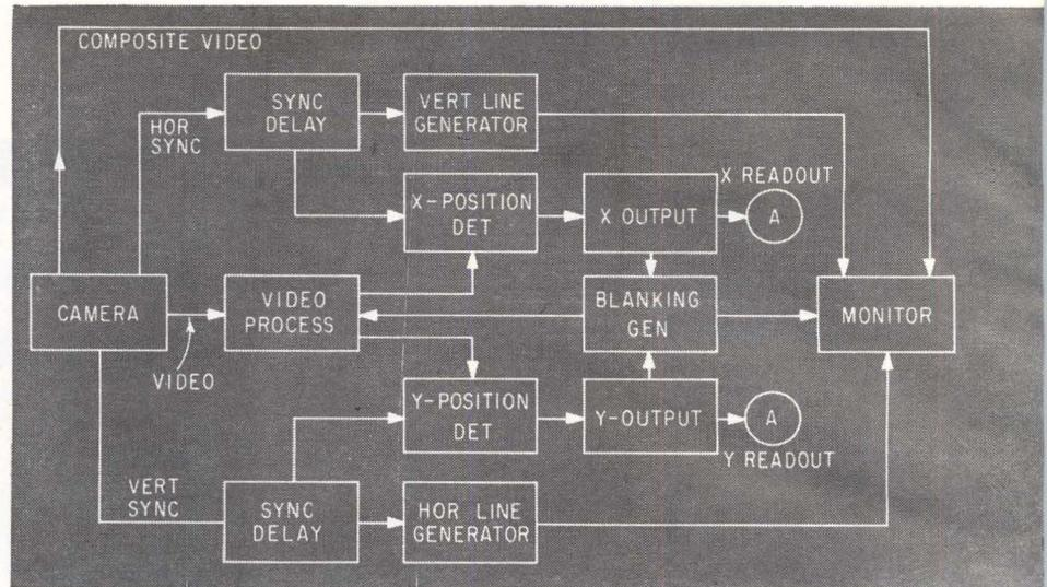
TRACKER CIRCUITS most of which use general-purpose transistors in straightforward designs, such as flip-flops, amplifiers and one-shots—Fig. 1
