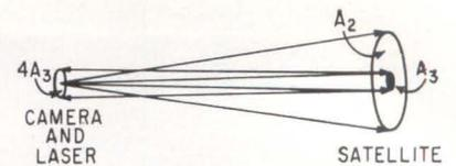
*LASER BEAM calculated to diverge and cover an area  $A_2$  at the satellite, whose effective area is  $A_1$ . Area of the reflected beam at camera position will be  $4A_3$ —Fig. 4*
