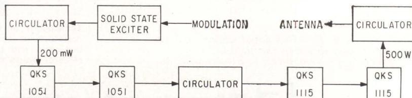
THREE-LEVEL stages would be practical when higher gains are required. Amplitron stages for above system could be 60 percent efficient in S-band—Fig. 3
