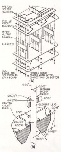
EXPLODED VIEW of module shows assembly details (A). Close-up of soldered joint assembly shows how needed rigidity is supplied by countersink configuration that provides conical shape of solder mass (B)—Fig. 2
