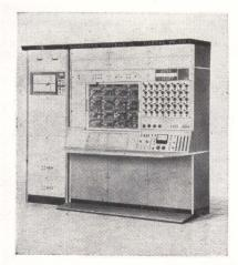
computing equipment. The 100-v level makes possible a dynamic range of 10,000 to 1 with computing accuracies of 0.01 percent at the lower range of the time scale. Although high packing density reduces parasitic capacitances and allows high computing frequencies, the highest range of computing frequencies requires operation at verylow impedance and voltage levels.
