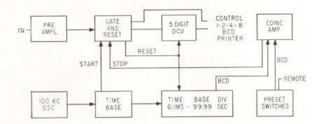
well as a 1-2-4-8 BCD 5-digit printer output. One example of use is determining fluid flow rate. If a transducer provides 250 pulses per gallon of flow, and n equals gallons per minute, then 250n could be displayed if the counter is gated for 60 seconds. Therefore, n could be displayed directly if the counter is gated for 60/250 seconds, or 0.24 second. Better resolution could be
