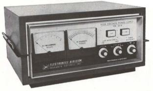
PSR Series, pictured above offer these important features: Range 5 to 30 KV, 2 to 30 MA • Regulation ± .05% • Ripple .1% RMS • Completely Solid State Circuitry • Light Weight • Rack Height 8%" maximum • Dry Insulation • Overload Protection • Reversible Polarity • Simplified Controls; coarse and fine voltage, ON-OFF meter reversing switch • Triple-Range Kilovoltmeter and Milliameter. Write for New 1963 High Voltage Bulletin.
