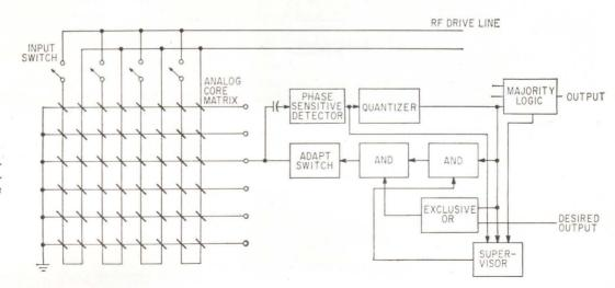
ADAPT LOGIC required to perform adaptations with inputs of one and zero-Fig. 5
