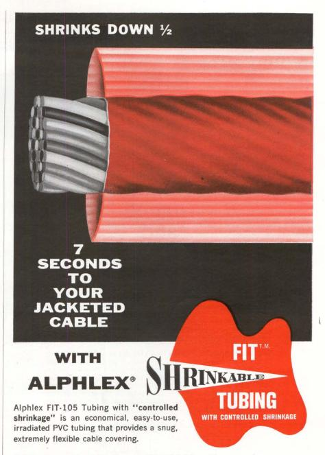
Cable cores may be pulled through FIT-105 Tubing with ease and shrunk down to form a jacket with all the qualities of the finest extruded plastic jackets. The tubing is supplied in expanded form and in continuous lengths and shrinks 50% upon application of heat (325°F). Heat may be applied through the use of the Alpha Heat Gun, or other heat sources. FIT-105 conforms to MIL-I-631C (105°C).
