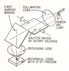
HOT-ENERGY SPOT is generated by optical soldering system and selectively applied to portions of joint soldered—Fig. 3
