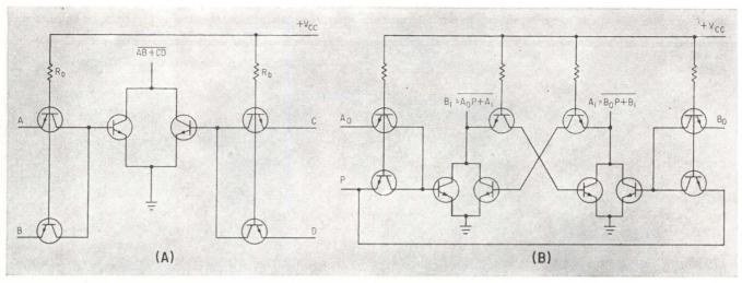
COMBINED TTL and DCTL (direct-coupled transistor logic) parallel gates leads to NOT-AND-OR circuit (A). TTL gated flip-flop (B) is designed for minimum logic delay—Fig. 2
