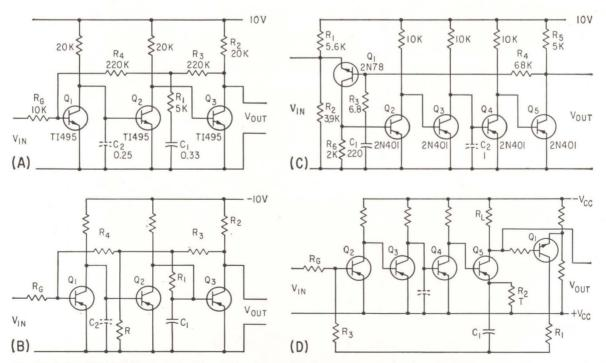
CURRENT DERIVED stabilization (A), Shunted-base current-derived stabilization (B). Circuit with bridge derived stabilization (C) has component values worked out in text, alternative version of bridge stabilized circuit (D)—Fig. 1
