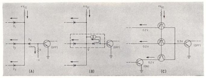
LOW LEVEL diode-transistor-logic (DTL) NAND gate (A) and a possible ideal solution (B). Development of TTL is shown (C)—Fig. 1
