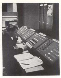
CONSOLE provides operating controls and selected readout
