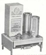
MGFO OSCILLATOR contains MG fork and vacuum tube circuitry
