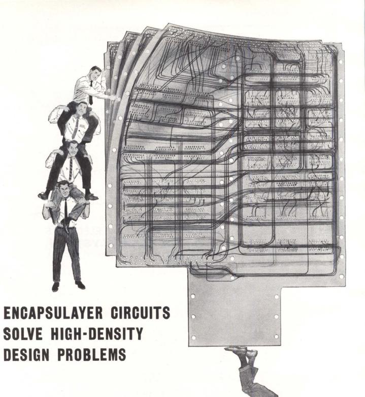
"Encapsulayer" is Photocircuits' multilayer printed circuit—an advanced new technique embodying great technical advantages. Thin printed circuit layers are stacked over each other-laminated together in registry to make one integral board. Plated-through holes' provide interconnections be-tween layers, interlinking all layers' circuitry with each other and board surface. Some advantages?
