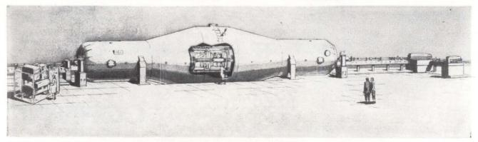
HIGH VOLTAGE Engineering Corporation's \$3-million 20-Mev tandem Van de Graaff accelerator, purchased during the last two months by the National Science Foundation and AEC for nuclear structure research at Rochester, Minnesota and Yale Universities, will produce stabilized and homogeneous accelerated ion beams at currents up to 25 microamperes, weighs 187 tons
