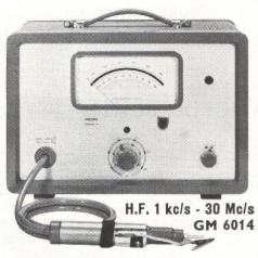
Range (fsd) 1 mV - 30 V -80 dB to + 32 dB Input impedance without attenuator 1 M $\Omega$  - 50 k $\Omega//7$  pF with attenuator 50 M $\Omega$  - 2 M $\Omega$ //2 pF Accuracy 3% Calibration voltages 30 mV and 3 V
