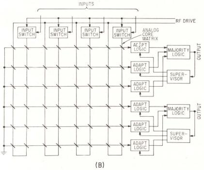
ADAPTIVE SYSTEM that classifies 4-bit patterns into four catagories (A), and the manner in which the cores can be arranged in a matrix (B)—Fig. 3
