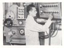
ROTARY dial switches on spindlehead-mounted console control precise boring operations
