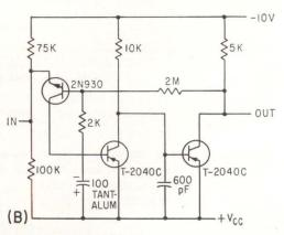
BAND-PASS AMPLIFIER (A) drives recorder in 0.2 to 5-cycle range; wideband amplifier with 60 db gain (B) uses Philoo T-2040 C transistors for frequency range 1 cycle to 1 Mc—Fig. 2
