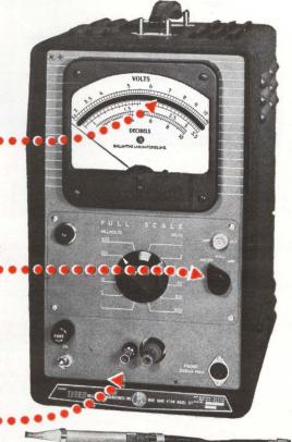
Cathode follower probe has high input impedance of 10 M  $\Omega$  -7 pF
