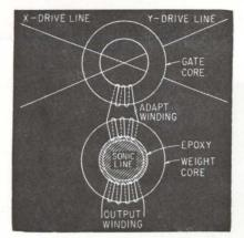
COUPLING of a magnetostrictive component to its gate core-Fig. 4
