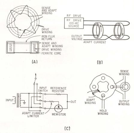
TWO FORMS of magnetic integrators. In (A), the flux level is altered by pulsing the output winding. In the second harmonic generator (B), the flux level is altered by passing d-c through the output winding. Bridge arrangements (C) for operation of the memistor or MAD—Fig. 2
