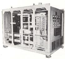
Typical construction of 600 KW, 250 volt dc power supplies designed by Acme Electric for use at Brookhaven National Laboratory. Similar units furnish the reliable power for other nuclear research installations at Cambridge, Argonne, Oak Ridge.
