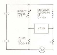
ductance variation with d-c current. The sketch shows how any inductance between 0.0005 and 10 H can be determined. This sketch shows a choke, with d-c superimposed and requires only a vtvm, a 25-w a-c amplifier, a low-ripple 1 to 10 ampere d-c supply and the Digibox unit. (305)
