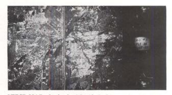
STRIP MAP obtained with side-looking radar illustrates high resolution. Map is made with antennas looking left and right, seam indicates aircraft line of flight
