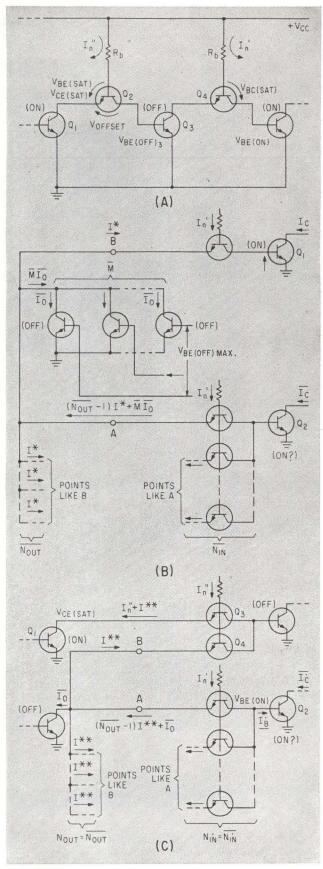
TWO TTL stages (A) with symbols used in the fan-out equations. Worst case circuit (B) where drive current is drained from Q2 because of base voltage differences of inverter transistors of the same fan-out family. Base current (C) drained away from Q2 adds to collector current of Q1. Question mark indicates that under worst case conditions, Q: may not actually be on-Fig. 4
