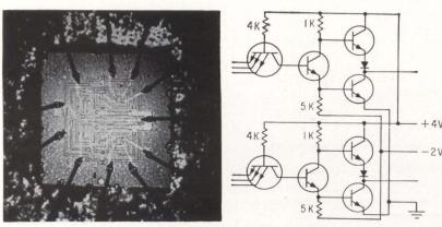
TYPICAL of the family of modified transistor-transistor integrated logic blocks introduced last week by Sylvania (see p 8, March 15) is this dual NAND gate. Propagation delays are 8 or 11 nsec depending on whether dissipation per stage is 15 or 7 mv. The block shown uses a Darlington-type circuit to increase fan-out to 25 and cascode connection at output to drive 50-pf capacitive loads
