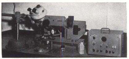
OPTICAL soldering equipment includes carbon-arc lamp energy source and positioning jig for holding modules to be soldered
