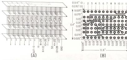
INTERCONNECTION of circuit elements in modular configuration using lead wires and circuit boards is determined using overall orientation layout (A) and printed circuit layout (B)—Fig. 1
