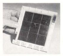
EXPERIMENTAL solar converter was successfully tested under actual space conditions
