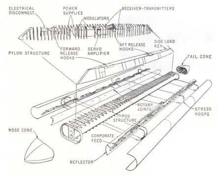
ANTENNA POD and electronics pylon of side-looking airborne radar, in exploded view. A series of 32 slotted-waveguide arrays are used as a line source feed for each of the two roll-stabilized antennas. Air Force system operates at X-band, with 240-Kw peak power
