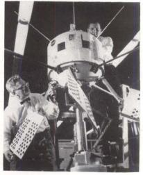
ENGINEERS EXAMINE test model of the S-52 satellite, a joint U. S.-United Kingdom project to measure galactic noise, ozone distribution and micrometeoroids. Westinghouse Electric is building it for NASA; British scientists will provide instrumentation
