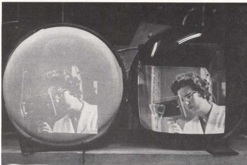
HIGH CONTRAST obtained from a transparent phosphor tube is shown above, right, compared to conventional cathode-ray tube, left, photographed in bright ambient light. Developed at Hirst Research Centre of the General Electric Co. in Wembley, Middlesex, England, the phosphor is vacuum-deposited on the tube faceplate. Tube is then baked to render the screen luminescent, and the phosphor is then coated with a black backing to absorb extraneous light and conceal the hot cathode.
