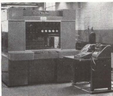
HYDRAULIC, pneumatic and electrical components are combined in automatic wire-wrap machine produced by Gardner-Denver. Complete installation includes machine, card-reader and machine control cabinet
