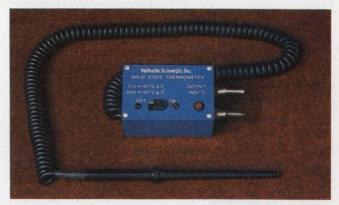
This temperature probe with a solid-state-junction thermal sensor generates an EMF of 1 mV/°C. It can be used with the Valhalla Model 4440 digital multimeter or any other DMM with a 200-mV full-scale range and autopolarity for indicating negative temperature. It can measure from -50 to 150 C.
