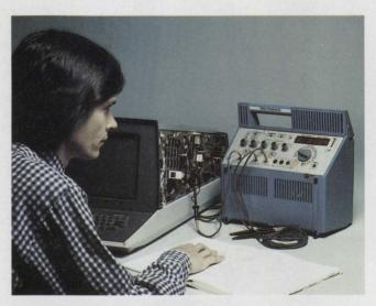
**Diagnostic decisions:** After the Tektronix 851 tests other equipment, it can help test itself. Just plug in the probes, step through the function switch and read the display.
