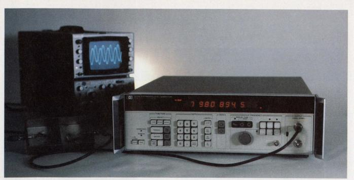
Frequency and amplitude in an HP 3335A are controlled by a microprocessor. Ten front-panel settings can be stored and recalled from the internal memory. A 200-Hz
