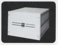
**HP 9414A Matrix Switch** provides maximum flexibility for high-density, high-performance switching, allowing any UUT pin to be switched to any instrument in the ATE system. The 16-input Matrix Switch can be configured in 30-pin increments (UUT pins) up to 120 pins, expandable to 240 pins.
