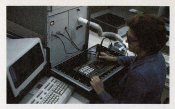
A software simulator generates programs capable of testing 360 points on a UUT approximately 10,000 times a second on the DTS-70 from HP. Boards containing 220 MSIs can be tested with programs that an experienced person can prepare in about two weeks.
