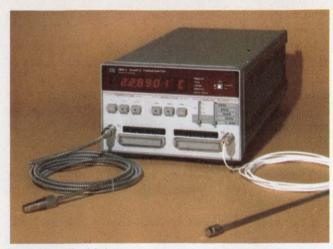
**Exceptionally high accuracy** is provided by HP's Model 2804 quartz-crystal thermometer. Temperature range is -50 to 150 C and resolution is 0.0001 C.
