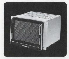
**HP 9412A Modular Switch** provides high-density, multi-function switching of signals up to 10 MHz. The built-in interface panel eliminates the massive cabling normally found in ATE switching configurations and significantly improves signal performance. The 9412A accommodates five types of switch cards in any combination up to a total of 25 cards.
