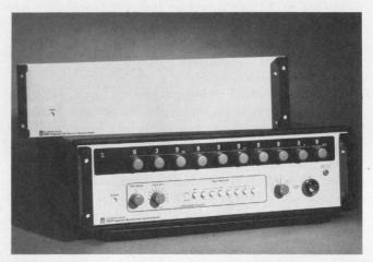
GenRad's 1062 frequency synthesizer switches frequency in 50  $\mu$ s. One-hundred data points in a digitally swept system can be scanned in 45 ms, with a 400- $\mu$ s dwell time for each measurement.
