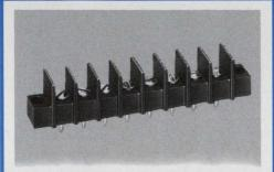
NEWLY DESIGNED "C" SERIES TERMI-NAL BLOCKS Your quality products deserve the best of the blocks—the Curtis Connection. Compact, break-resistant "C" blocks for control and electronic circuits are made from high-impact thermoplastic. Rigid, immovable molded-in insert prevents breaking of P.C. solder joints. High barrier design meets full 300 volt clearances required by UL 1059. 1 thru 26 terminals. Curtis Industries, Inc., 8000 W. Tower Ave., Milwaukee, WI 53223. Phone (414) 354-1500.
