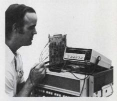
Many companies are streamlining field service of microprocessor-based products by troubleshooting to the component level with the 5004A signature analyzer.
