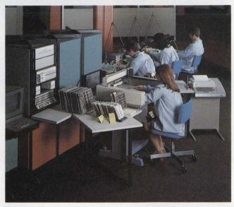
Teradyne's L125 Circuit Diagnostic System has two major configurations—one for digital boards, one for mixed analog-digital boards. By following instructions from the CRT, the operator works with the system's guided probe.
