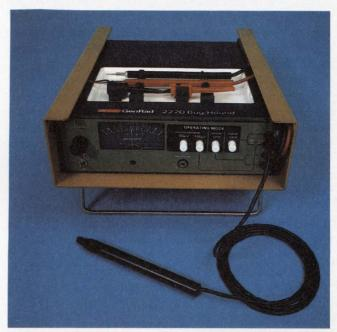
GenRad's current-tracing 2220 Bug Hound isolates faults on known-bad cards. The probe's LEDs and audible alarms pinpoint shorts, opens, bad ICs, and other troubles.
