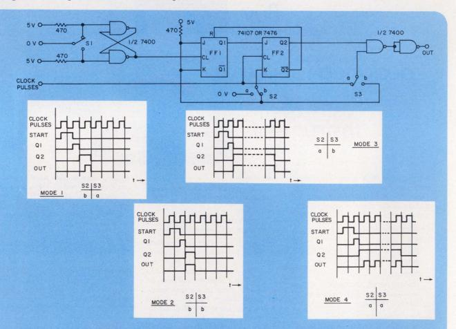
Four modes of testing can be obtained by setting switches  $S_2$  and  $S_3$  in the four possible position
