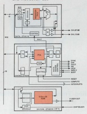
The basic chip set consists of a data-manipulation chip containing an 8-bit ALU and 26 8-bit registers. The 16 registers can be set up to act as program counter, stack pointer, accumulator and general-purpose 8 or 16-bit registers. A typical minimal system consists of a data chip, a control chip, two to four ROM chips, a clock generator and buffers.
