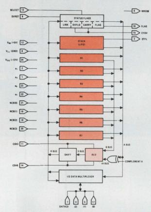
The architecture of the IMP processor family is split into three basic chips. On the RALU are all the RAM registers, counters and control logic (including the ALU). The CROM holds the microprogram for the macroinstructions while the interface logic circuit provides the flags, condition-jump controller, program counter and program-counter stack. All circuits interface directly via MOS level buses and require a four-phase nonoverlapping clock.
