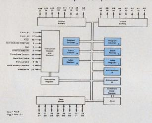
A minimum system for the MC6800 will typically consist of the processor, some ROM and RAM, a clock circuit and some I/O circuits. All lines except the clock lines are TTL compatible and the address bus, data bus and R/W line also have three-state capability. The 6800 has two accumulators, but all stack space is in the user-supplied RAM—there are no auxiliary registers on the processor chip.
