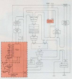
The 16-bit memory-to-memory architecture of the 9900  $\mu Ps$  permits flexible register files to be set up in memory. A minimal system consists of the CPU, a clock generator and the necessary memory.
