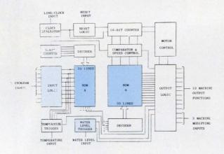
The architecture of the 7150 uses two ROMs to control the various output functions. There is no ALU since no data manipulation is required. However, there are two analog inputs to the processor that are used with an on-chip difference amplifier to form a temperature sensing circuit.
