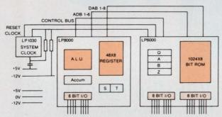
The architecture of the Series 8000 is based on a three-chip set—the CPU, ROM and clock generator. In the processor is an 8-bit ALU, a 48 × 8 register file, a four-word address stack and eight bidirectional I/O lines. The 8-bit data bus and 6-bit control bus combine to provide a 14-bit memory address.
