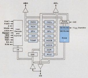
The architecture of the MC6802 resembles that of the MC6800 except that the 6802 includes the stack and the clock oscillator on the chip. A minimum system requires just two chips—the MC6802 MPU and the MC6846, a combination ROM and I/O timer.
