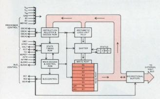
The architecture of the CP1600 family processors starts with a 16-bit parallel ALU and an eight-word general-purpose register file that is directly accessible by the processor. All lines are TTL compatible except for the clock lines, and the 16-line bus has three-state capability.
