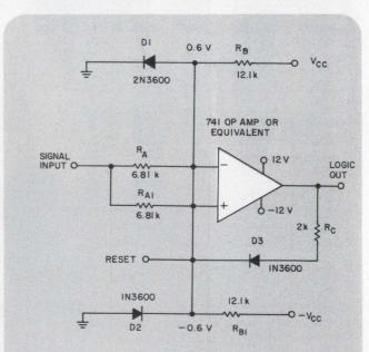
A positive analog input provides a positive logic-level output that remains after the signal passes. Similarly, a negative input provides a remembered positivelevel output.
