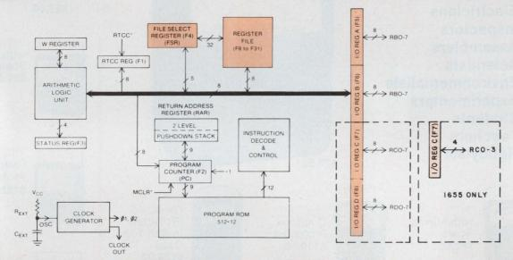
The PIC 1655 differs from the 1650 only in the number of I/O lines. All lines are TTL compatible. There are four 8-bit parallel ports on the 1650 as well
