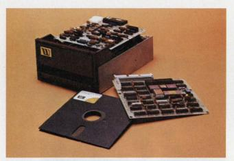
**Dual-index and file-protect sensors** permit recording of data on both sides of a microdiskette on the Wangco Model 82 Micro-Floppy. Up to four units can be daisy-chained on a single bus.
