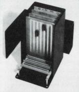
A new pc card case with optional heat sinking and/or blower accommodation. "TEKARD" cases receive standard 4.5" wide pc cards, as made by many manufacturers. The connector rails have up to 37 mounting positions, spaced on .200". Five extruded shapes are available in three lengths, allowing 45 "off the shelf" kits.
