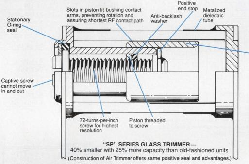
Non-rotating design assures .0002" max. dielectric clearance for greatest capacitance
