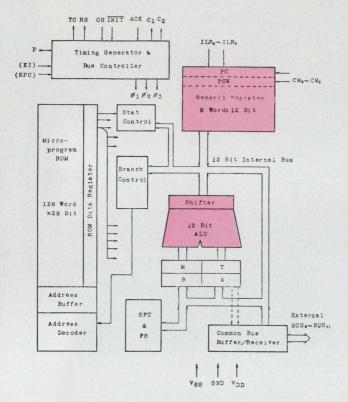
12 bits Data word size: Address bus size: 12 bits 4096 words Direct addressing range: Instruction word size: 12 bits Number of basic instructions: 21 Shortest instruction/time 6.6 µs (Load register): Longest instruction/time (Divide): 104 µs 0.63/2 MHz Clock frequency (min/max): 3/Internal Clock phases/voltage swing: Dedicated I/O control lines: None 36-pin DIP Package: 5 V/140 mA Power requirements: -5 V/35 mA
