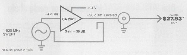
These applications are only the beginning. TRW RF linear hybrids can revolutionize design after design...with incredible performance at unbelievable prices. Let us prove it. To get complete data sheets, send us the coupon.
