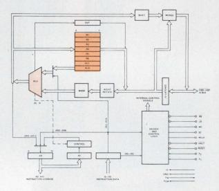
The architecture of the 8X300 is designed so that several operations can take place simultaneously—shift, merge, rotate and mask. A minimal system contains the 8X300, some memories and several 8-bit I/O ports. All lines are TTL compatible and the 8-bit interface bus has three-state capability.
