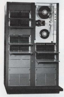
Besides this 28-track model, Bell & Howell's Data-tape Division, Pasadena, CA, supplies 42-track digital instrumentation recorders with packing densities of 33,000 bpi, data throughput rates of 150 Mbits/s, and error rates of one bit in 10-billion.
