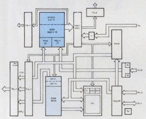
The architecture of the uCOM-42 is designed directly for the electronic cash register market and keyboard controllable appliances. The I/O structure handles an  $8\times4$  keyboard, an 8-digit LED display and peripherals. The on-board RAM can also be expanded off the chip. All I/O lines are TTL compatible and all outputs can handle up to -35 V.
