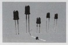
Ultra high Brightness in LED has been achieved in a new and unique process developed by "STANLEY ELECTRIC" of Japan in which continuous liquid growth of Multilayers of Ga Al As compound is deposited on Ga As substrate in the crystal gowing phase. Ultra bright LED's made this material exhibit 60 to 80 mcd at IF 20ma. Samples and literature available from A.C. INTERFACE, INC., 2925 College Ave., #A-1, Costa Mesa, California 92626, (714) 979-9830.
