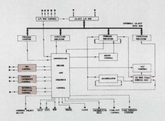
The architecture of the F100-L uses a multiplexed data and address bus. However, to simplify the handling of data many of the bus control functions are handled by support chips. The processor performs all of its ALU operations in a serial mode—the ALU is only 1 bit wide. An external clock is required and a clock rate of up to 20 MHz is possible. All lines are TTL compatible.
