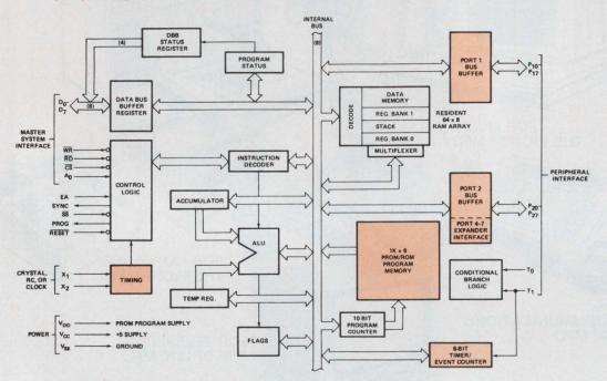
Since the device is a complete microcomputer, it can function as a stand alone unit. Of the 18 I/O lines, 2 are for input only, and 16 are input-output
