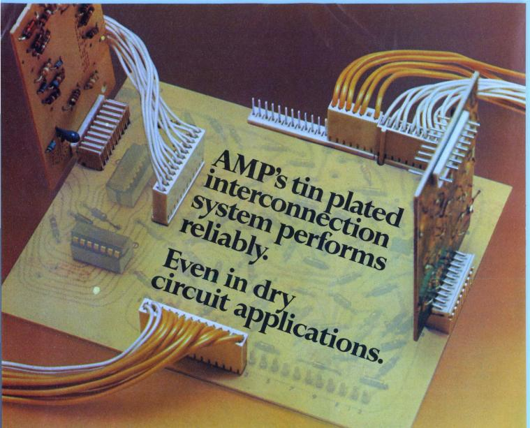
Because our Commercial Interconnection System (CIS) features a unique, high pressure, redundant, metal-to-metal contact design, tin plating can be used instead of gold. A choice of fork-type-contacts provides mating forces from 400 to 1,000 grams for maximum application flexibility. And the posts assure positive wiping action for clean contacts and extended stability.
