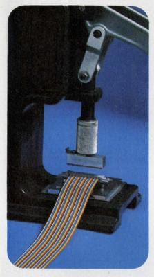
There's no costly investment to make in equipment or training. All you need are two locator plates and the Scotchflex manual or pneumatic assembly press. You can start mass terminating assemblies quickly and economically. No special operator skills are required. Rejects and reworking are greatly minimized.
