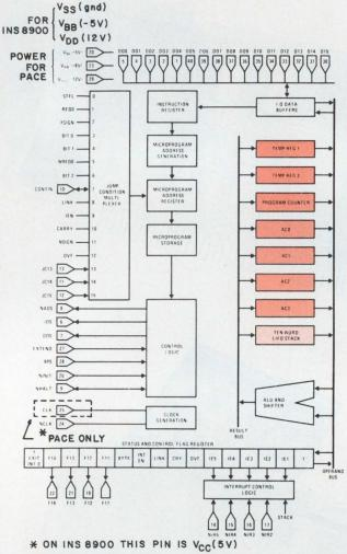
The architecture of the INS8900 and the PACE provides a 10-word stack as well as four general-purpose registers and an independent 16-bit status and control flag register. There is also a six-level vectored priority interrupt system built into the chip. However, an external single-phase clock must be supplied. A minimal system consists of the CPU, a clock and some memory.
