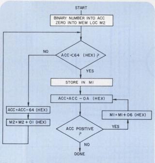
When the binary-to-BCD conversion is complete,  $M_1$  contains the tens and ones digits within a single byte in BCD, while  $M_2$  contains the hundreds digit.
