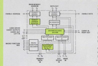
A minimal system for the Series 3000 is hard to define since the user determines the processor word length and the amount of microprogram storage needed. A typical 16-bit machine application, though, might require about 25 to 35 devices. The processor's architecture revolves about the ALU and 11 general-purpose registers. All operations are controlled by the function bus, which accepts the microprogram control words and selects both operands and the ALU operation to be performed.
