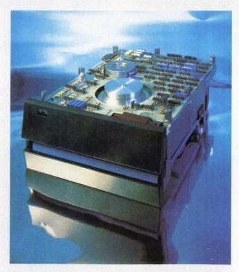
This double-sided, double-density IBM-compatible May-flower 700 from MFE measures 30% smaller than competition, and multiplies media life by four. Dc-motored 750 version claims a high 10,000-h MTBF and low power—30 W. The 700 and the 750 are the first floppy products of MFE, an established cassette builder.
