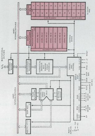
The architecture of the MCS-40 processors is almost identical except for the expanded stack and scratch-pad areas of the 4040 as compared to the 4004. A minimal system typically requires three chips—the CPU, a clock generator and a memory circuit.
