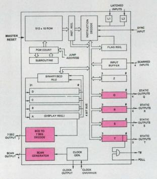
The stand-alone processor has scanned inputs and decoded outputs: seven input lines, 16 output lines, and LED segment driver outputs. All lines are compatible with TTL or CMOS logic families. In addition to the 512  $\times$  10 bit on chip ROM, the 1872 has a 32  $\times$  4 bit scratchpad RAM and on-board clock generator.
