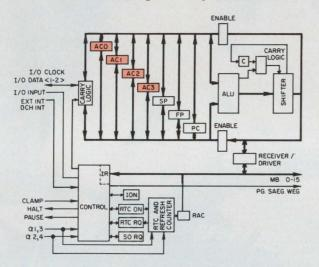
Included in the basic chip set are the mN601 microprocessor, mN640 clock driver and the mN629 I/O transceiver. All I/O lines are decoded for I/O interfacing and are not available for control purposes. The lines are open-collector TTL compatible. Four 16-bit registers in the CPU can act as source or destination accumulator.
