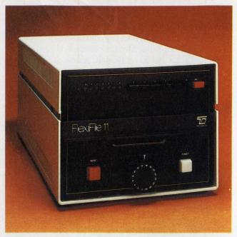
is triple the industry standard, though the 8-in. medium affords only 32 tracks, 98 kbytes of storage and 40 kbytes/s transfer with 100-rpm operation.
