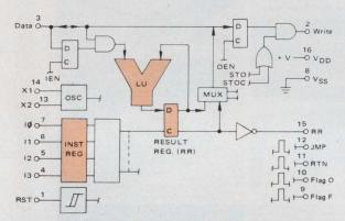
A minimum system consists of the processor, an external memory, program counter, 8-channel data selector and an 8-bit addressable latch. Instruction lines are TTL compatible and the 1-bit bi-directional data line has three-state capability. On-chip there are three 1-bit registers that are directly addressable, and the clock oscillator.
