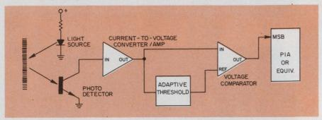
**Bar coded programs** are illuminated by a LED and sensed by a phototransistor. The pulse produced by the transistor is amplified and fed to a comparator. An adaptive threshold circuit that is used as a reference for the comparator helps eliminate noise. The output of the comparator then goes to a peripheral interface adapter (PIA) and then to the computer.
