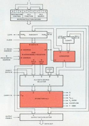
A minimal system is hard to pin down since the word size can be set to any size. However a typical number of circuits would be between 40 and 60. The high-speed ALU in the 2901A can perform its operations on two 4-bit input words, one from a two-input multiplexer and the other from a three-input mux.
