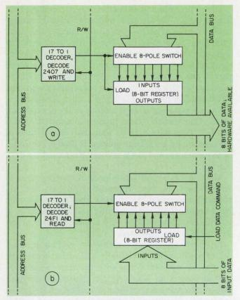
4. Output (a) and input (b) ports provide the means for communicating with the outside world. In "a," address 2407 and a WRITE command load the data bus into a register. In "b," data are loaded into the register. Address 24F1 places them onto the data bus.
