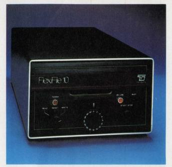
Seeking guaranteed interchangeability of diskette media, Tri Data departs from industry standards with its floppy drives for the Flexifile 10 (left) and 11 (right). Track width
