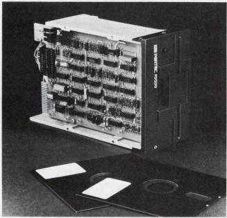
A micro-sized drive (top) from MPI is the only minifloppy to use a metal-band actuator. Its track-to-track time is 5 ms. Pertec's micro-sized floppy (bottom) boasts the same dimensions, mounting holes, interface signals, and voltage requirements as the Shugart SA400.
