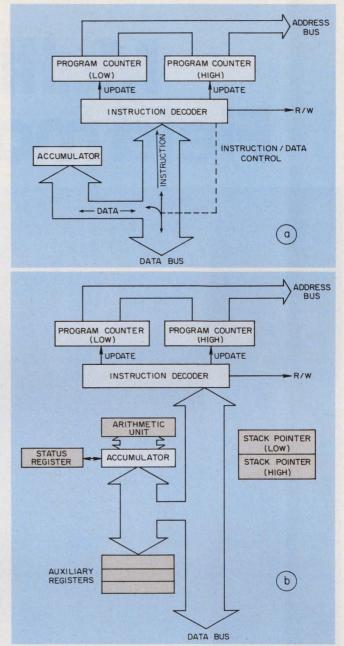
5. A simple microprocessor consists of just a few basic blocks (a). A more realistic  $\mu P$  (b) includes a few "frills" that make it operational.
