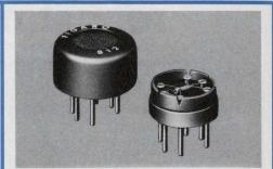
FIGARO GAS SENSOR TGS is a gas sensitive semiconductor. When combustible gas is absorbed on the sensor surface, a marked decrease of electrical resistance occurs. Major features of the sensor include high sensitivity, long term reliability and low cost. The applications are: GAS-LEAK ALARM, AUTOMATIC FAN CON-TROL, FIRE ALARM, ALCOHOL DETEC-TOR, etc. Figaro Engineering Inc., North America Office-3303 Habor Boulevard, Suite D-8, Costa Mesa, Calif. 92626 Tel: (714) 751-4103 Telex: 678396
