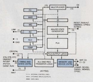
The architecture of the IM 6100 resembles that of the PDP-8 minicomputer. Signals are available that can help create a front panel so that the processor can be manually controlled. The processor's onboard crystal-controlled clock can be driven by an external source.
