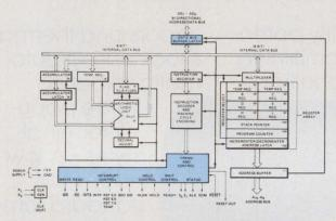
The basic architecture of the 8085 is the same as that of the 8080A. The only differences are the built-in clock generator, the built-in system control circuit and the multiplexed address/date bus structure to make available several pins for additional control.
