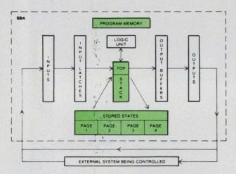
The Sequential Boolean Analyzer consists of a program memory that holds a set of Boolean functions that define system operation as well as 30 input buffers that are latched at the start of the evaluation of Boolean equations, and four pages of 30 stored-state flip-flops which can be grouped to emulate counters and shift registers. Also included are a logic unit that can perform the logic functions and a stack that holds a set of Boolean values used to evaluate the input equation.
