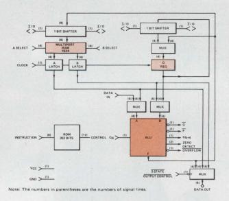
The architecture of the 5701/6701 bit slice includes a 16 word x 4 bit dual-port RAM as well as a 36 instruction ALU and a single 4-bit working register that can be used as a second accumulator or as an extension to permit an 8-bit result. On the chip are also some microprogrammed ROMs that determine the operation of the ALU for each incoming instruction.
