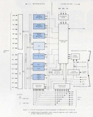
The architecture of the MCS6500 permits all registers to accept data from the data bus and transfer data back and forth since they are all connected to the same internal bus. A minimal system consists of the CPU and some memory (for a 651X system you also need a clock generator).
