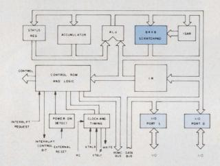
The architecture of the 3850 CPU provides a distributed format, thus permitting simple system expansions. The processor contains a 64 byte scratchpad RAM and 16 I/O lines. Any program storage unit added to the system brings 16 I/O lines, a counter/timer and other features depending on the version. All I/O lines are TTL compatible and the data and address buses have three-state capability.
