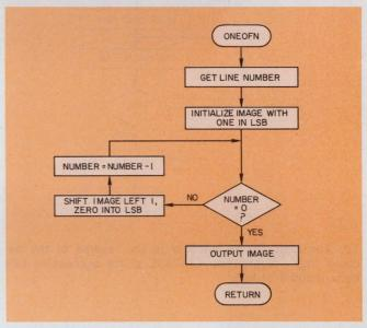
9. The algorithm ONEOFN illustrates operation of a "one-of-N" decoder. The number of available lines, N, is usually 8, 10, or 16.
