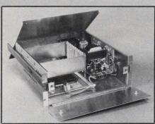
Several Micromodule card cages and a power supply have been added by Motorola to support M6800-based equipment development. Two card cages are available: one with five card slots, the other with 10. Both cages have motherboards that are pin-compatible with all Micromodules and EXORciser modules.
