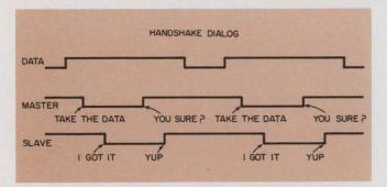
4. The handshake dialog ensures proper signal flow between a "master" and a "slave" device. Usually the CPU is the master for output operations, and the I/O device for input operations.
