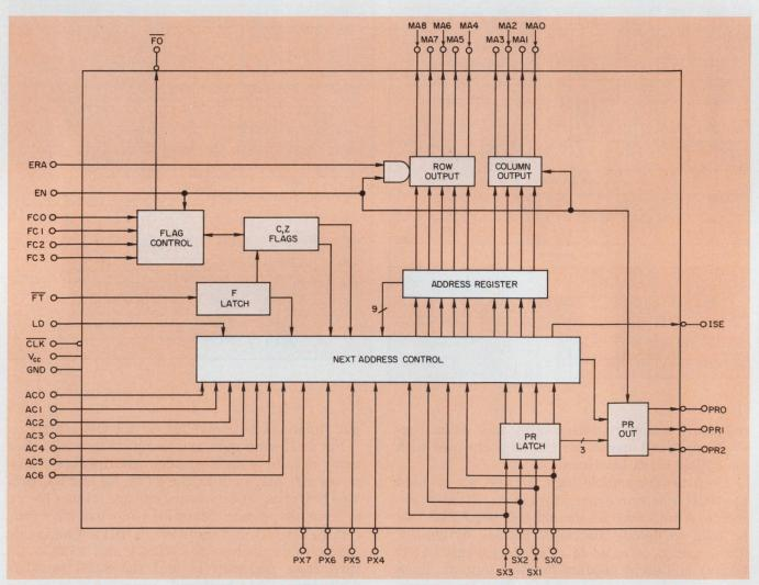
5. Able to address up to 512 words of any length, the 3001 microprogram controller provides its companion
