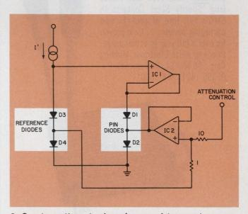
3. Constant attenuator impedance and temperature compensation are attained when the PIN diodes are matched against reference diodes in this arrangement. Op amp  $IC_1$  keeps the voltage drive to both sets of diodes equal, and  $IC_2$  acts as a current-sink control for the PIN diodes and as a temperature compensator.
