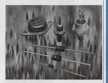
Varo Semiconductor, Inc. is the only manufacturer offering a complete line of Schottky Barrier Rectifiers with 40V PIV rating and 150°C maximum junction operating temperature (T<sub>J</sub>). These Schottkys can simplify your design problems by allowing a greater safety factor in component selection. You are no longer limited to 30V PIV and 125°C max. (T<sub>g</sub>).
