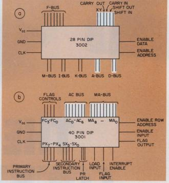
1. Capable of being cascaded to any desired word length, the 3002 two-bit processor (a) comes housed in a 28-pin DIP. Its controller, the 3001 (b), can handle
