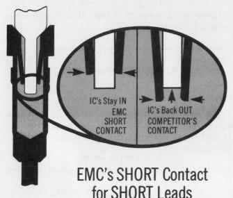
Many newer IC's have shorter or highly tapered leads. If plugged into longer standard terminal contacts, lateral pressure caused by the angle of the contacts vector into a constant potential ejection force. Add a
