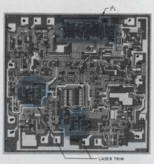
Linear and digital technologies are combined in this high-density variable-slope delta modulator by Motorola. A linear-compatible I<sup>2</sup>L process used in the digital portions of the chip reduces chip size by 5 to 1.
