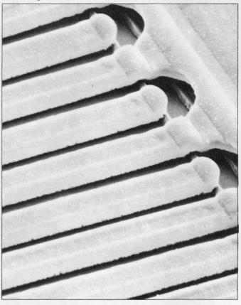
**TRW etchless gold die metalization.** Exact finger definition holds original design values intact, eliminates current crowding and metal migration.
