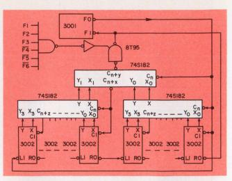
4. To speed up arithmetic processing, the 74S182 look-ahead carry generator can work with eight 3002s to form a 16-bit machine.
