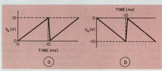
4. Switching operation from p-channel to n charges the sweep from a positive (a) to a negative-going ramp (b). In both instances, the sweep time is 10 ms.
