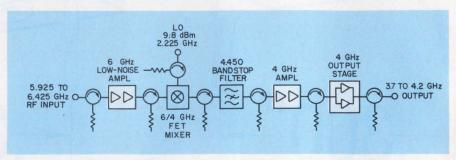
High gain, excellent linearity and low noise figures are provided by galliumarsenide FETs in this satellite-communications receiver.
