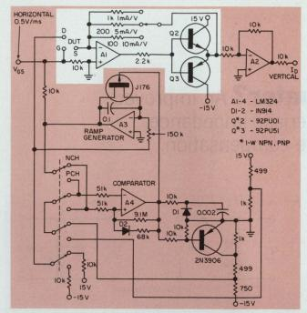
2. Basis of the tracer is a current-to-voltage converter designed around an op amp  $(A_1)$ , one-fourth of a quad. Amplifier  $A_2$  forms a unity-gain inverter, while  $A_3$  and  $A_4$  form the sweep generator. Sweep rate is 0.5 V/ms.
