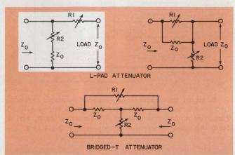
1. L-pad attenuators can provide a constant characteristic impedance,  $Z_o$ , as the attenuation is varied—but only at the input terminals. A bridged-T configuration can keep  $Z_o$  constant at both input and output terminals.
