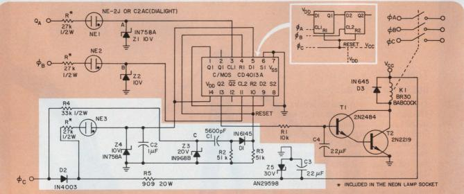
1. The phase-sequence detector circuit derives its supply voltage,  $V_{\rm ec}$  and  $V_{\rm dd}$ , from  $\phi_{\rm e}$ . This factor, together with the neon lamps and zener diodes in the
