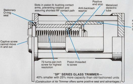
Non-rotating design assures .0002" max. dielectric clearance for greatest capacitance
