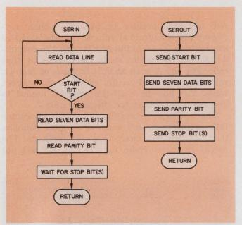
14. The ASCII serial-interface logic consists of two subroutines: SERIN, which accepts serial input, and SER-OUT, which generates serial output.
