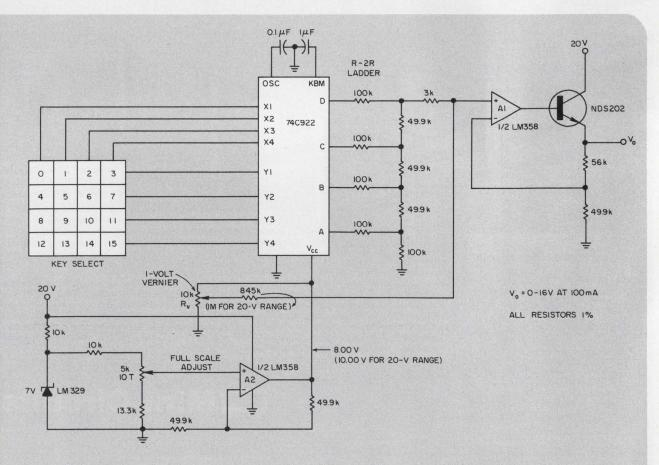
Press a key and the corresponding voltage appears at the output in 1-V steps. A 1-V vernier adjust-
