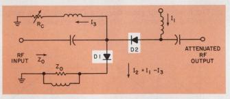
2. A pair of PIN diodes in an L-pad configuration can be used to attenuate rf signals controlled by dc current. Both  $\mathbf{I}_1$  and  $\mathbf{I}_2$  must be varied appropriately to control attenuation and keep  $\mathbf{Z}_o$  constant.
