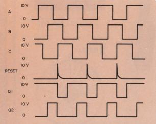
2. Any one of the following correct phase sequences—ABC, BCA or CAB—will produce a train of rectangular pulses at the output  $Q_2$ , in Fig. 1. For incorrect sequences—BAC, ACB or CBA—the output,  $Q_2$ , stays LOW.
