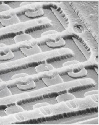
Conventionally-etched die metalization. Etched scalloping in metal fingers produces current crowding and resultant failure through metal migration.
