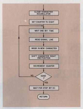
16. Converting a serial character to hex requires that the data bits be assembled in the proper sequence. The least significant bit arrives first.
