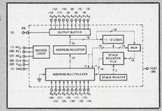
Compared with other available units, the 8X02 provides several advantages. The 1-k addressing capability is not available in other units, nor is the 8X02's subroutine-nesting capability. The controller has a four-way stack-register file and offers conditional nesting
