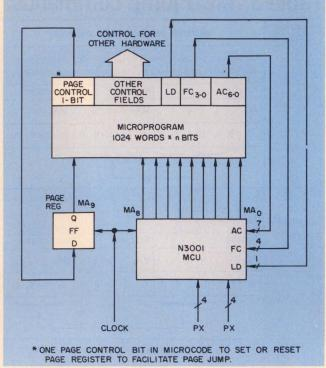
6. If more than 512 words of microprogram memory are needed, the address bus of the 3001 can be expanded by adding an extra flip-flop for paging.
