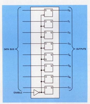
3. A simple 8-bit output port uses latches to store data from the bus. When the output device is ready to receive, the "enable" pulse makes the connection.
