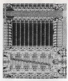
A 92,160-bit CCD memory tolerates faults in single-memory cells because any of the 36 blocks like this one can be disconnected from the circuit, leaving only good cells in operation.
