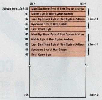
12. The random-access memory needed to hold the log data must be grouped into blocks of five bytes for each error file. Three bytes are needed for the system address, one for the parity and one for the error-count.
