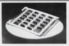
T<sup>2</sup>L Power Distribution—Noise attenuation and highest packaging density for P.C. boards with T<sup>2</sup>L logic are yours with Mini/Bus®, the Rogers way to eliminate the cost of multilayer boards by off-board power distribution. Rogers Corporation, Chandler, AZ 85224. Phone (602) 963-4584. (EUROPE: Mektron NV, Ghent, Belgium; JAPAN: Nippon Mektron, Tokyo)
