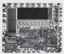
Containing 1024 bytes of UV PROM and 64 bytes of RAM in addition to a full 8-bit  $\mu$ P on a single chip, the 8748 is the first of a new breed of user-programmable microcomputer circuits pioneered by Intel.
