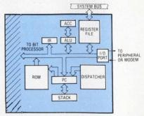
What's better than one  $\mu P$  on a chip? Why two, of course. Combining both a bit and byte-oriented processor on a single chip, Intel has been able to make programmable controllers from the same basic chip.
