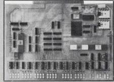
The expanded industrial version permits 16-bit addressing and has 1 kbyte of RAM sockets for 2 kbytes of UV PROM, a ROM containing I/O routines for a teletypewriter as well as a current loop or RS-232 interface, a cassette interface, two parallel I/O ports, and a bus structure that permits simple expansion.
